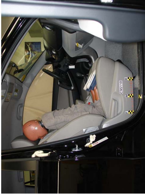
3-Year-Old Unbelted, Middle Seat Track, Position 7
