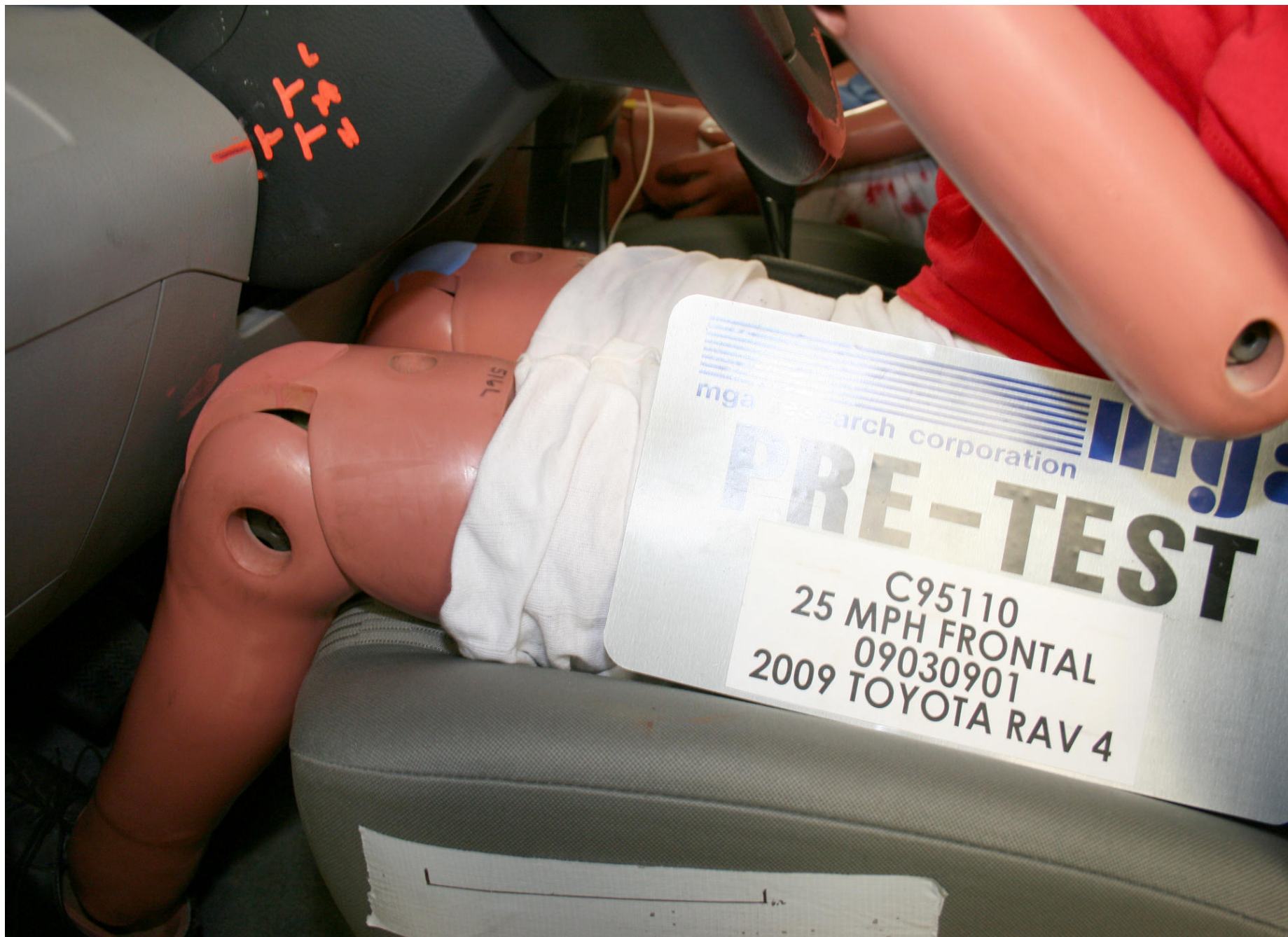
Pre-Test Driver Side Knee Bolster View
