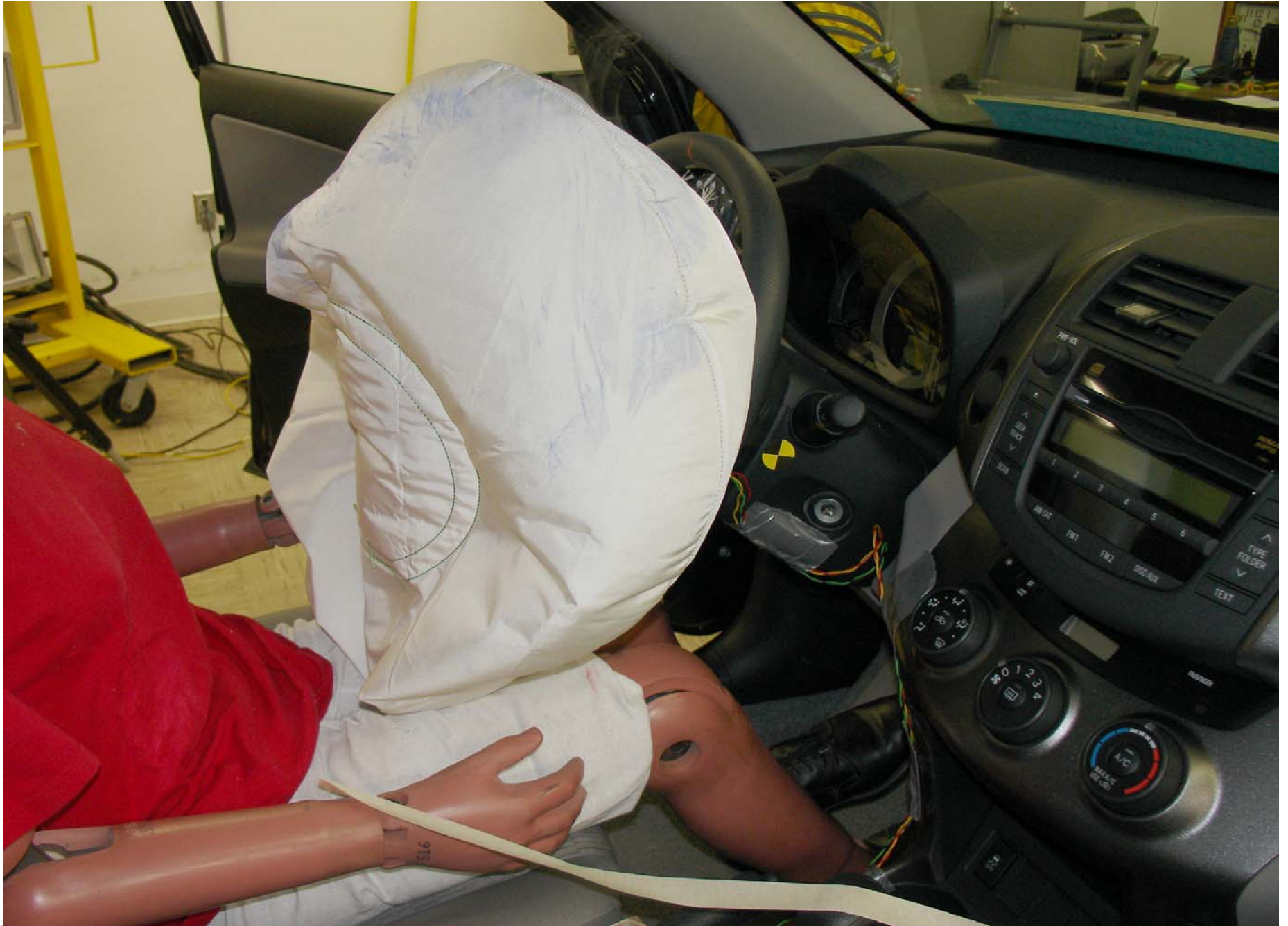
Post-Test 5th Fem. P1 Driver Dummy Airbag Right Side View
