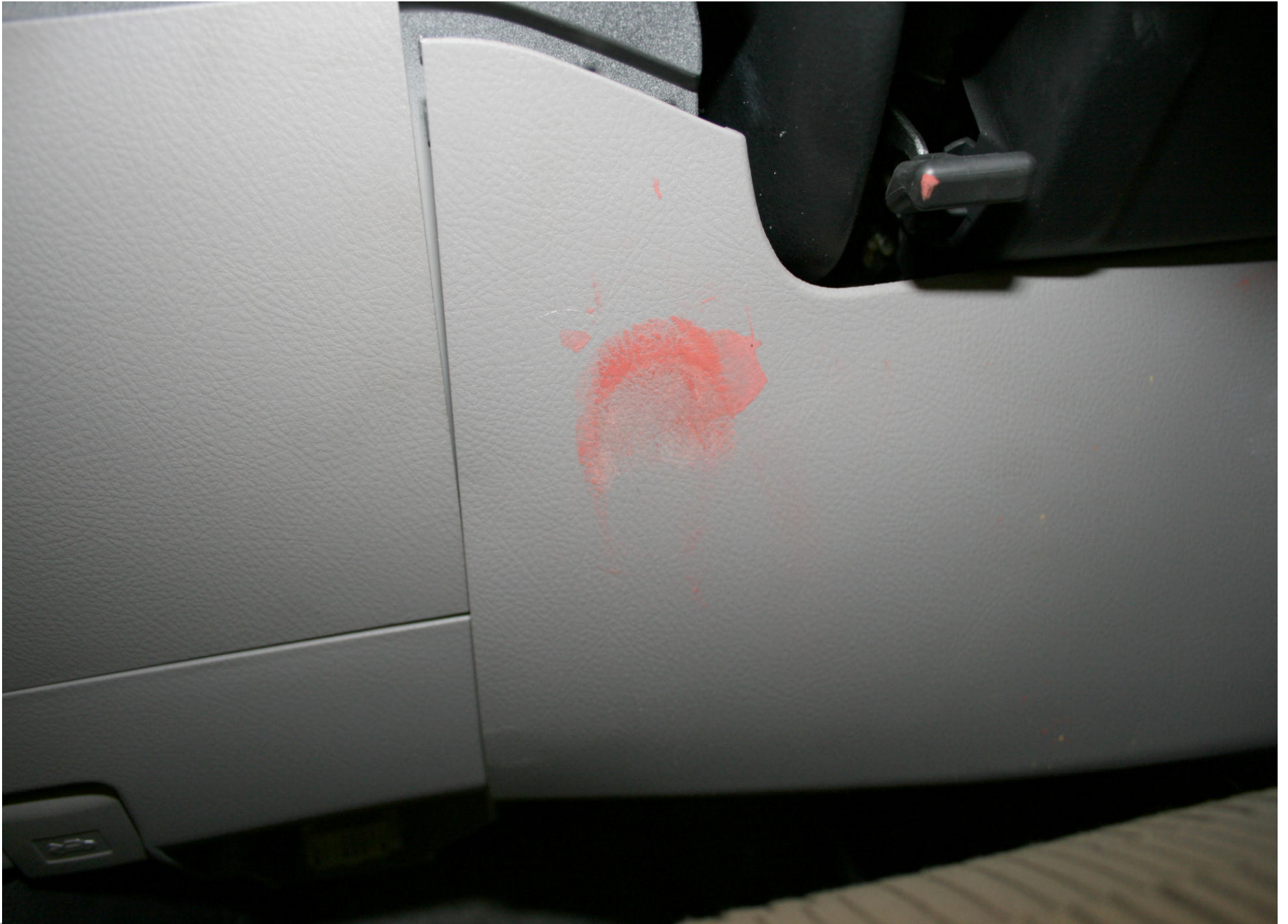
Post-Test Driver Dummy Knee Contact (left side)
