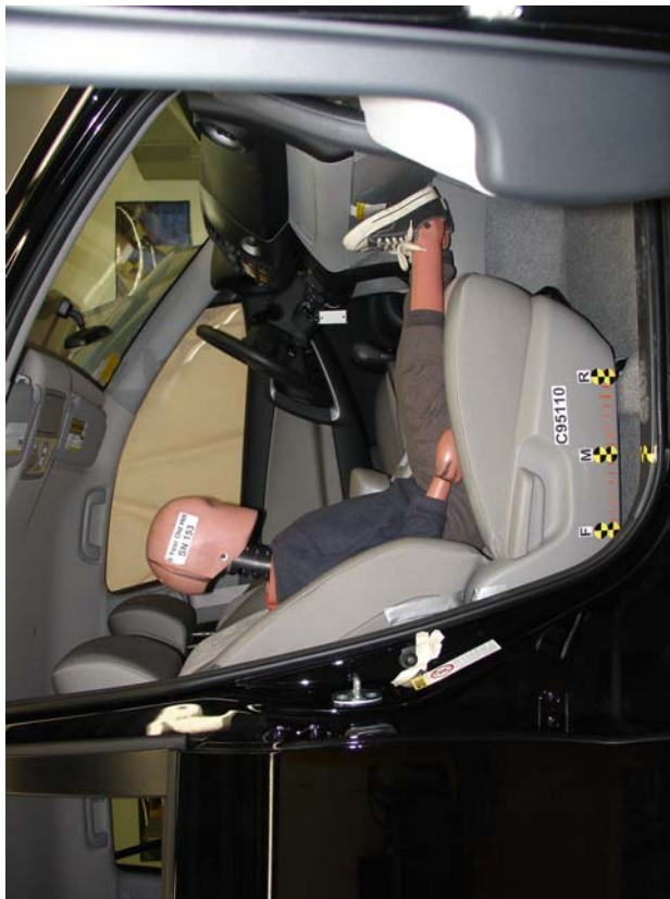
6-Year-Old Unbelted, Middle Seat Track, Position 1
