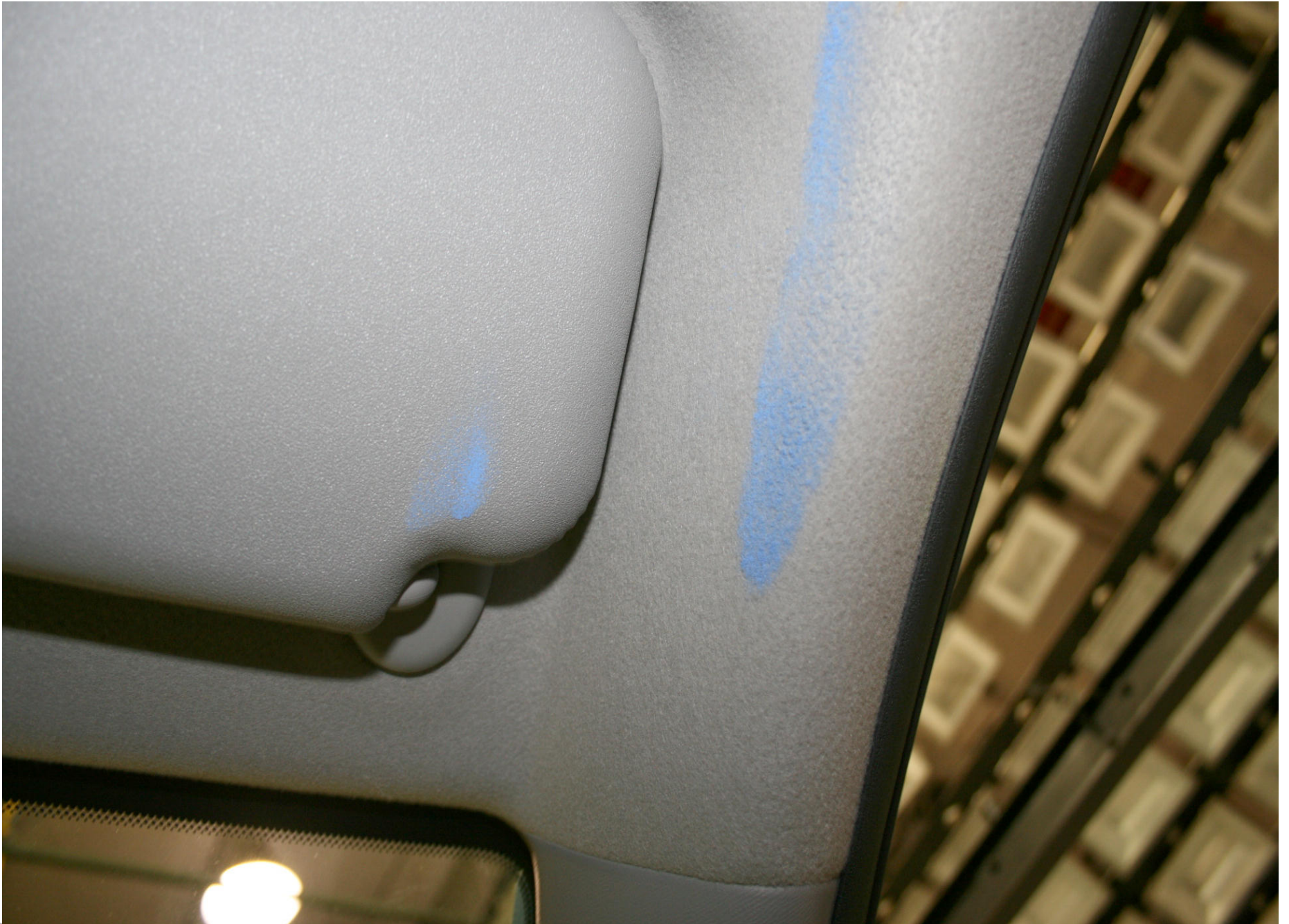
Post-Test Passenger Dummy Head Contact (a-pillar, visor)
