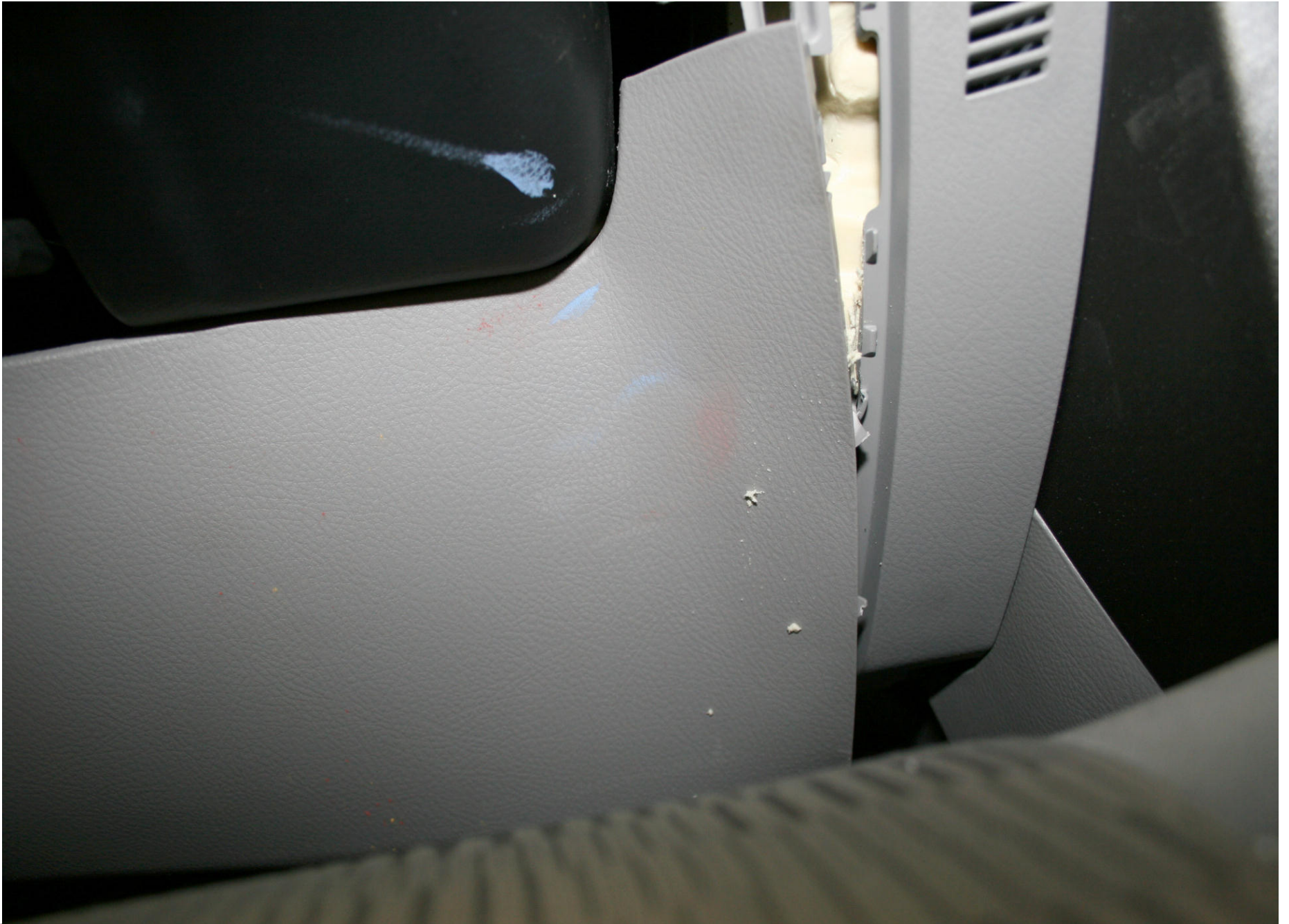
Post-Test Driver Dummy Knee Contact (right side)
