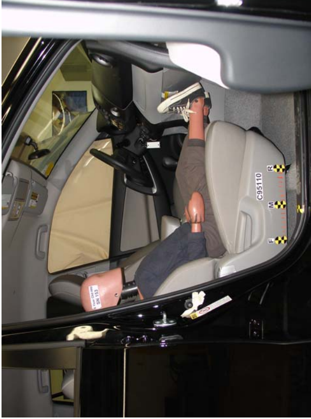
6-Year-Old Unbelted, Forward Seat Track, Position 2
