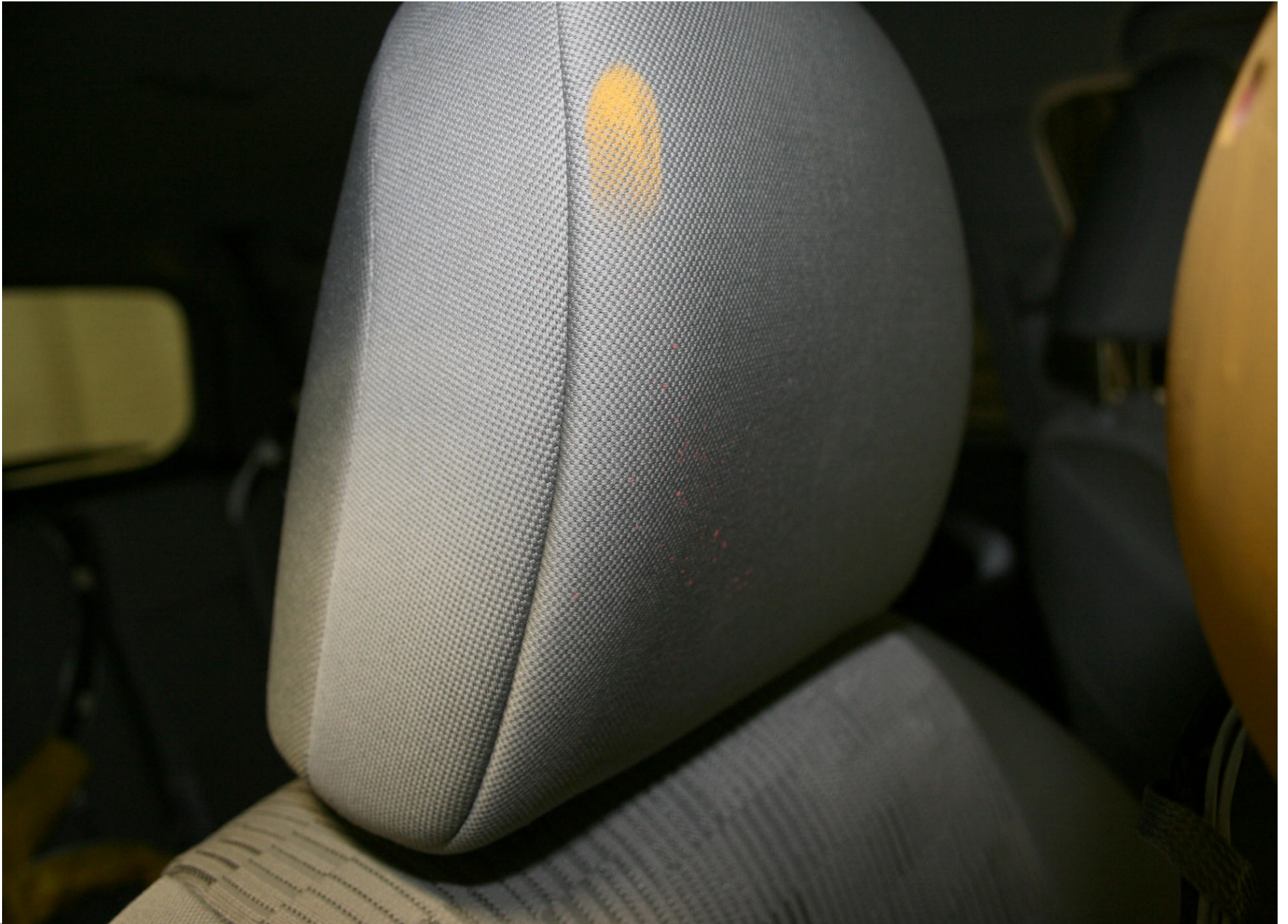
Post-Test Passenger Dummy Head Contact (headrest)
