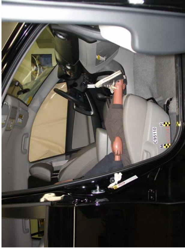
6-Year-Old Unbelted, Rearward Seat Track, Position 2
