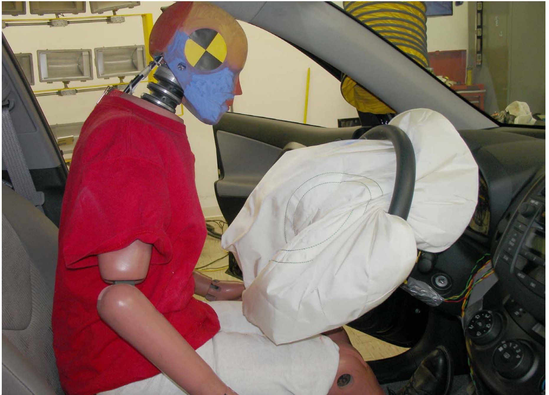
Post-Test 5th Fem. P2 Driver Dummy Airbag Right Side View
