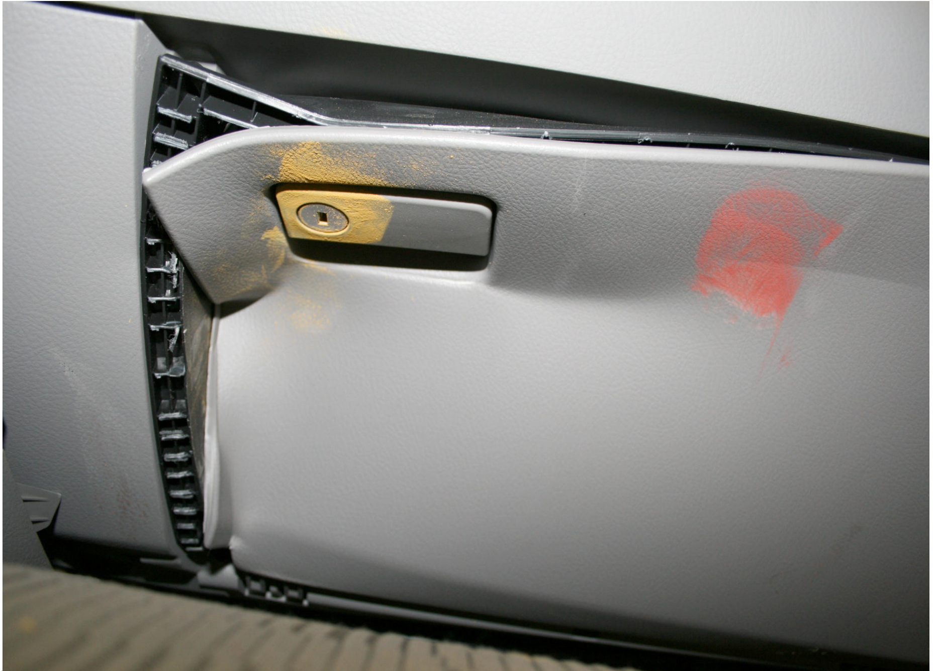
Post-Test Passenger Dummy Knee Contact
