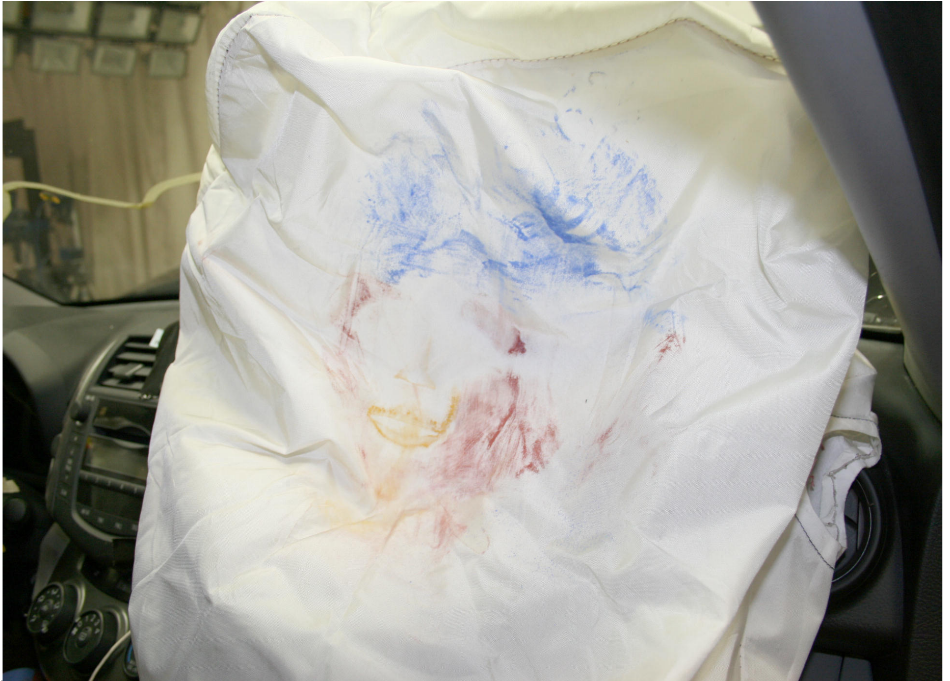
Post-Test Passenger Dummy Airbag Contact
