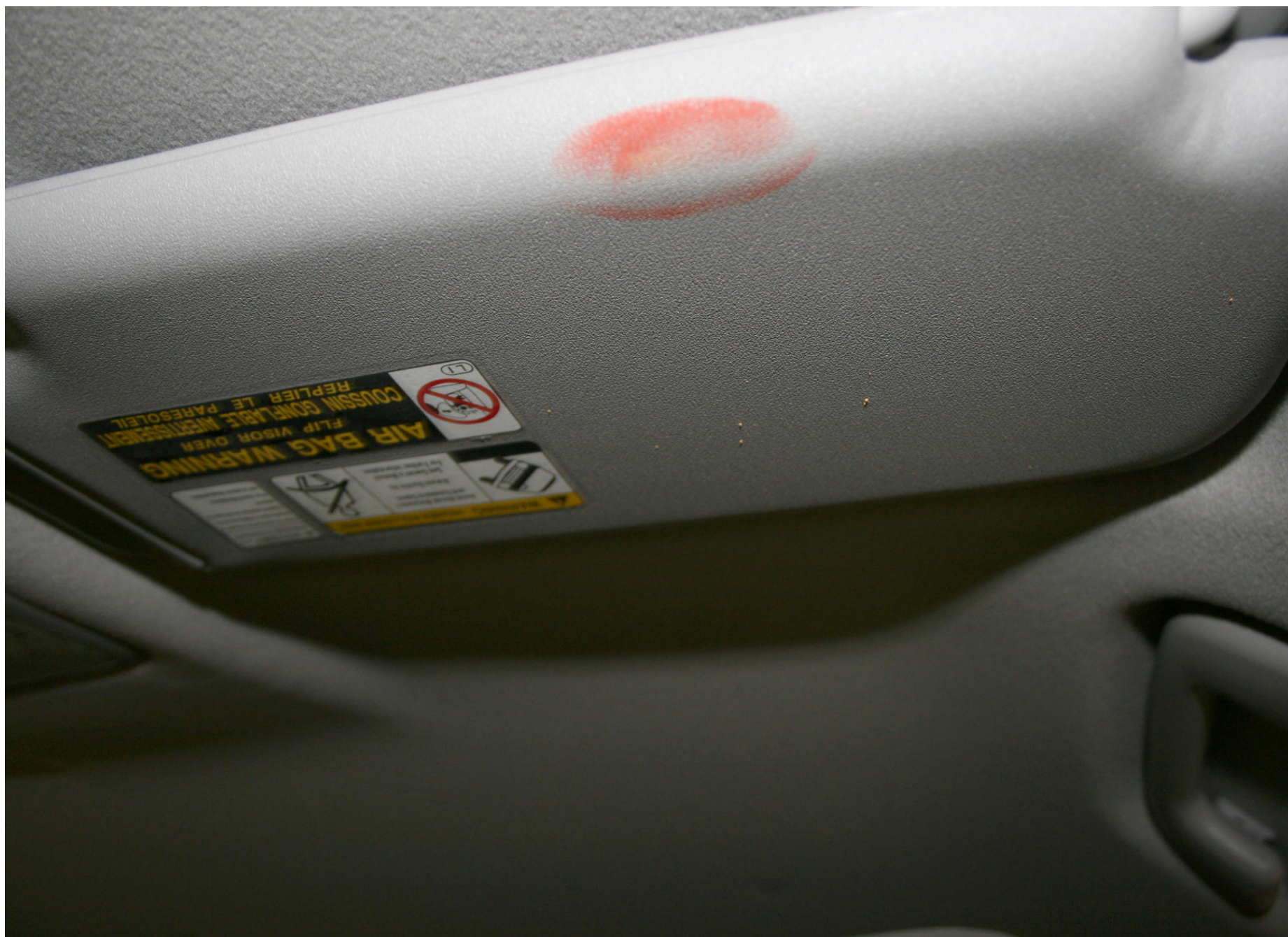
Post-Test Driver Dummy Head Contact (visor)
