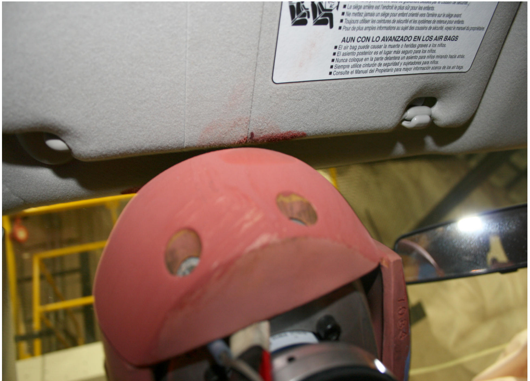
Post-Test Driver Dummy Head Contact (visor)
