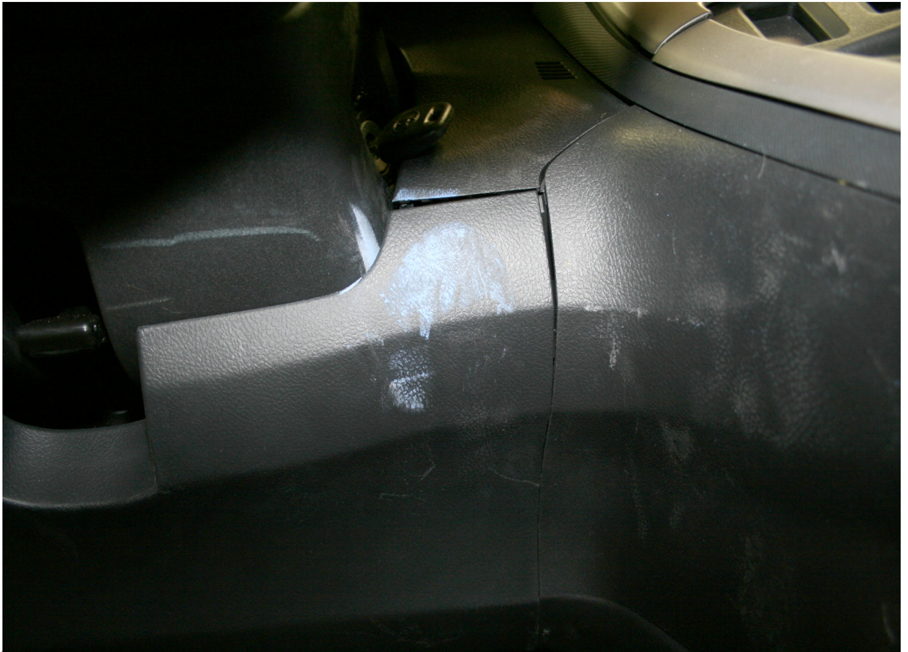
Post-Test Driver Dummy Knee Contact (right side)
