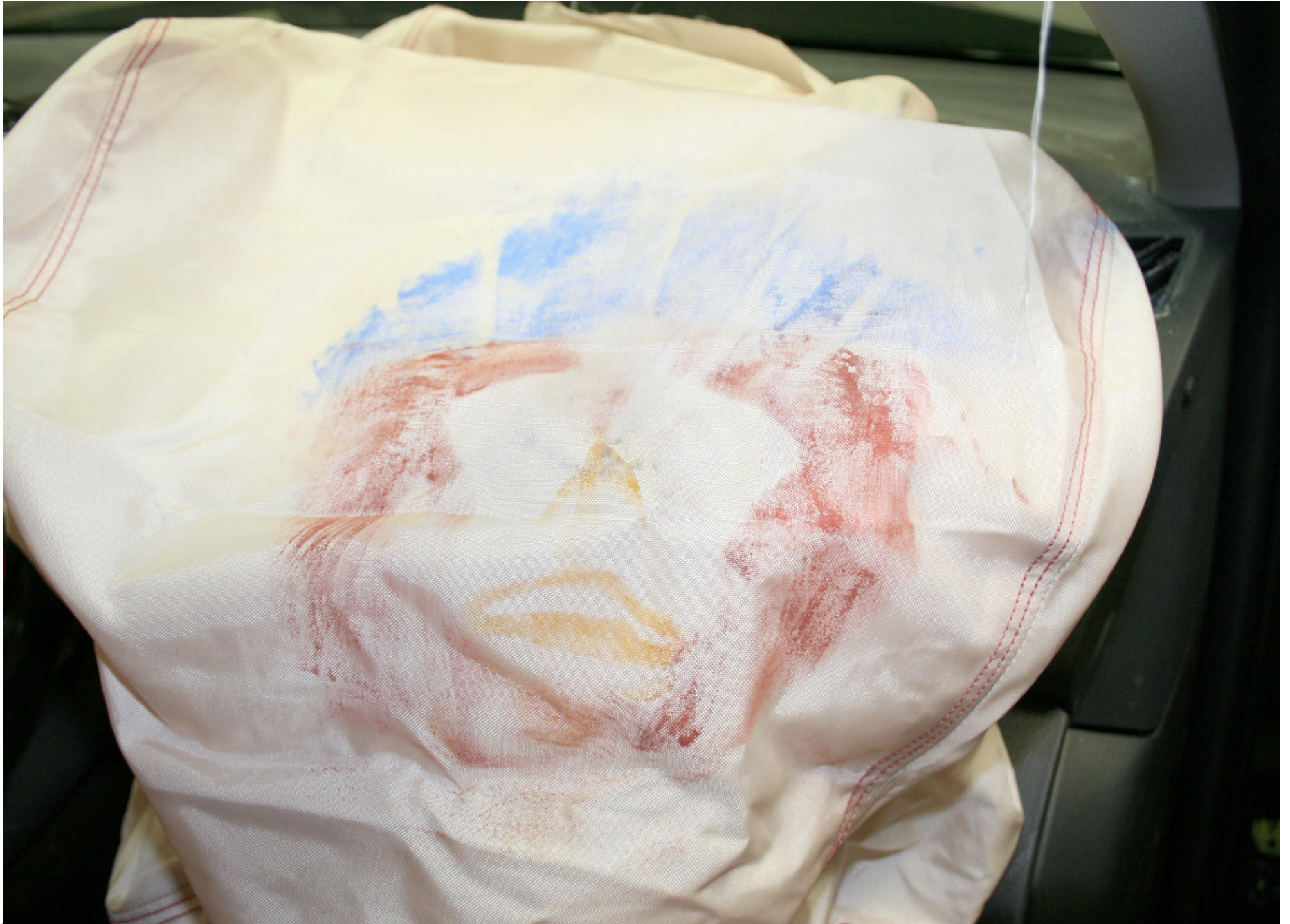
Post-Test Passenger Dummy Airbag Contact
