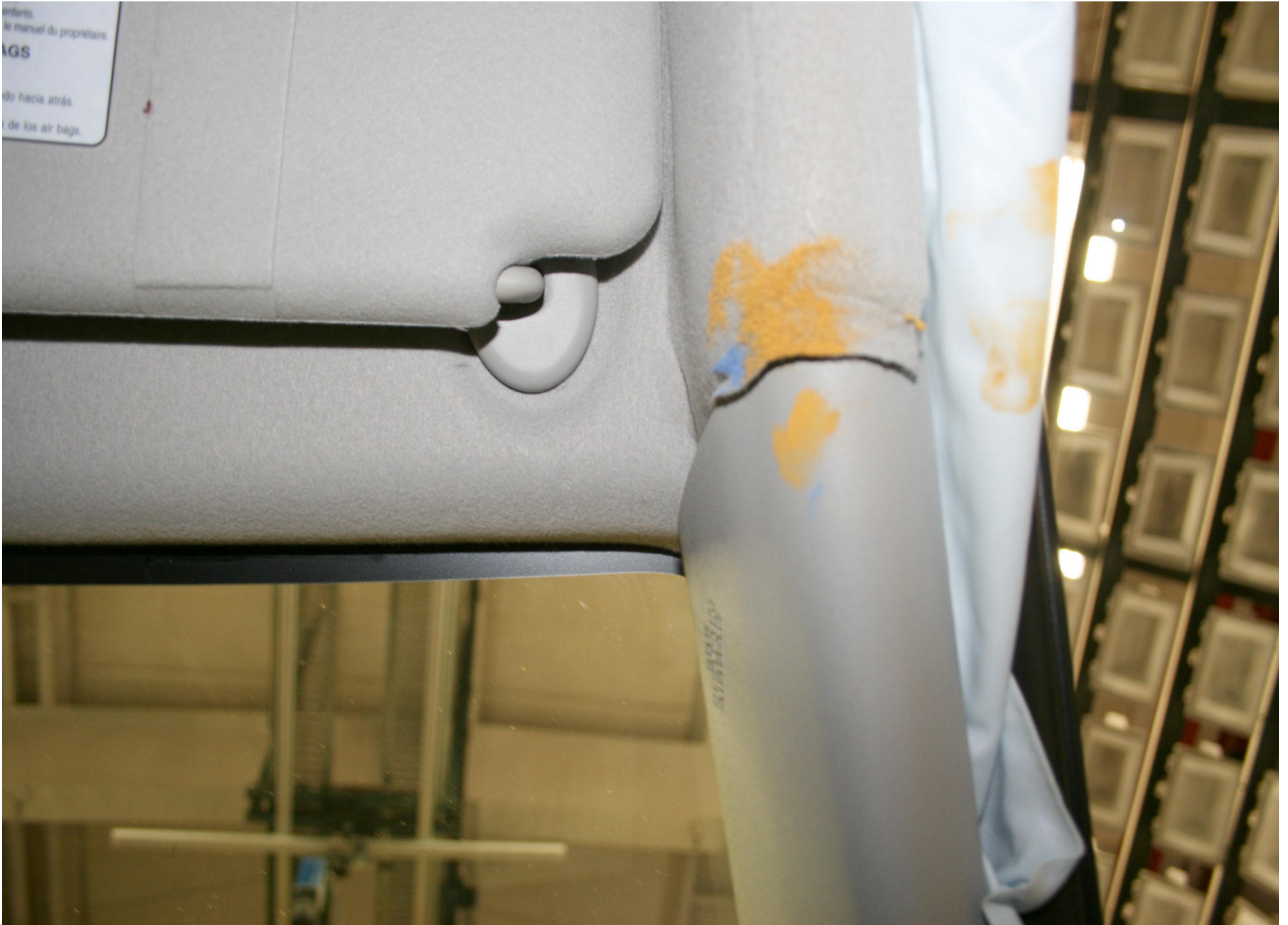
Post-Test Passenger Dummy Head Contact (C-pillar)
