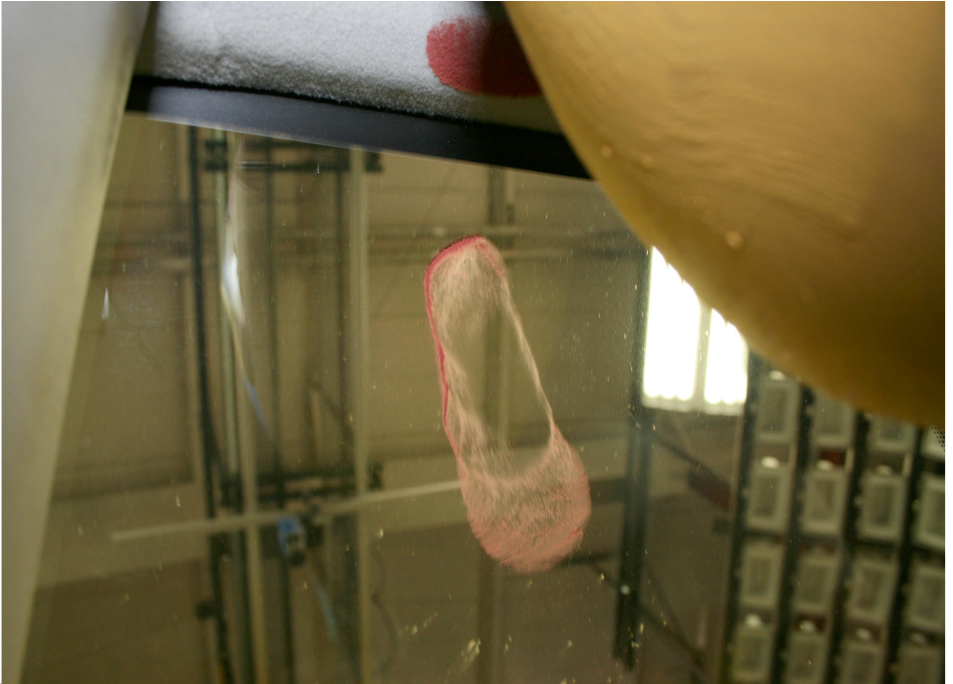
Post-Test Driver Dummy Head Contact (windshield)
