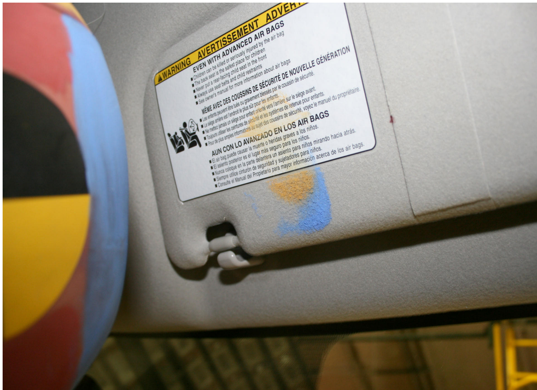
Post-Test Passenger Dummy Head Contact (visor)
