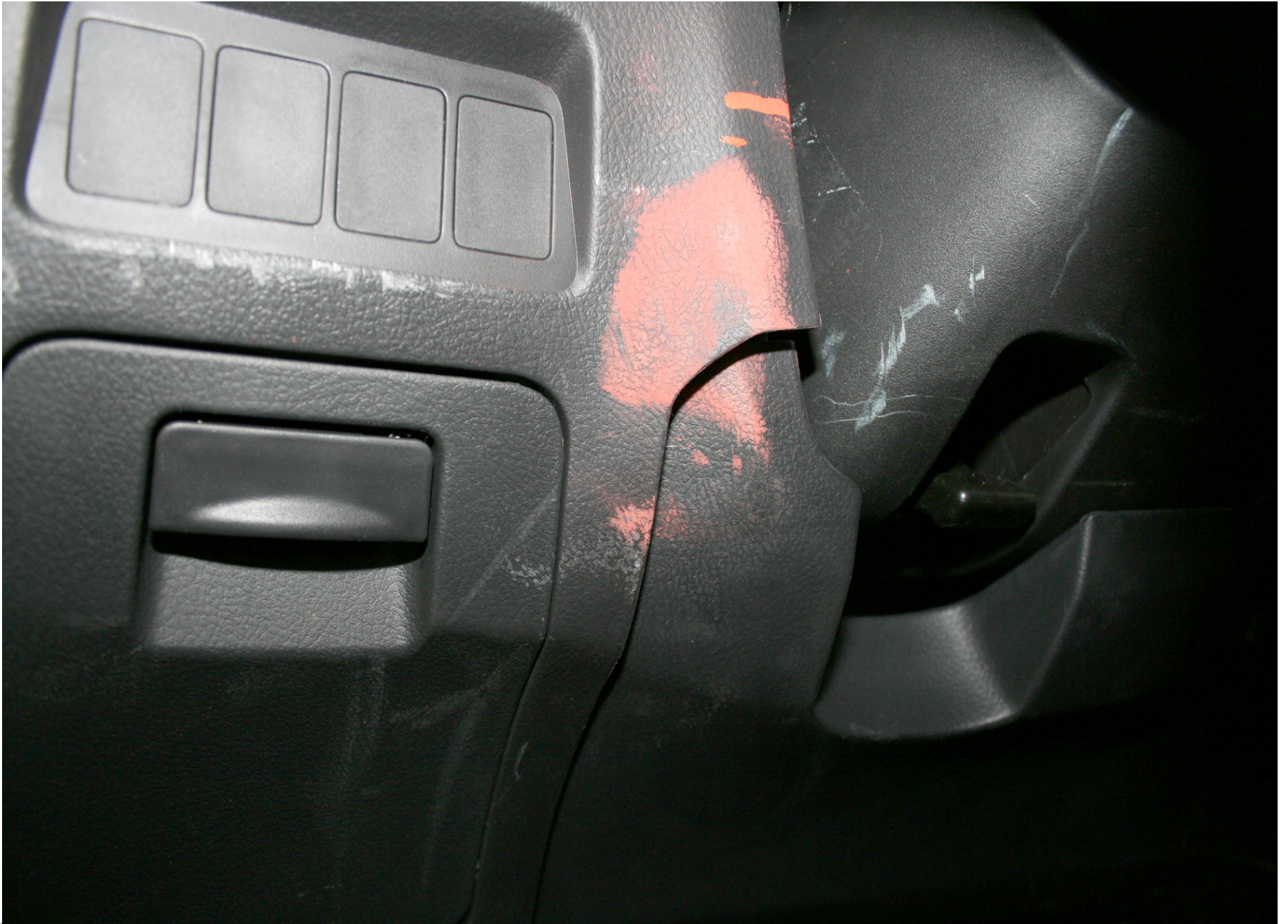
Post-Test Driver Dummy Knee Contact (left side)
