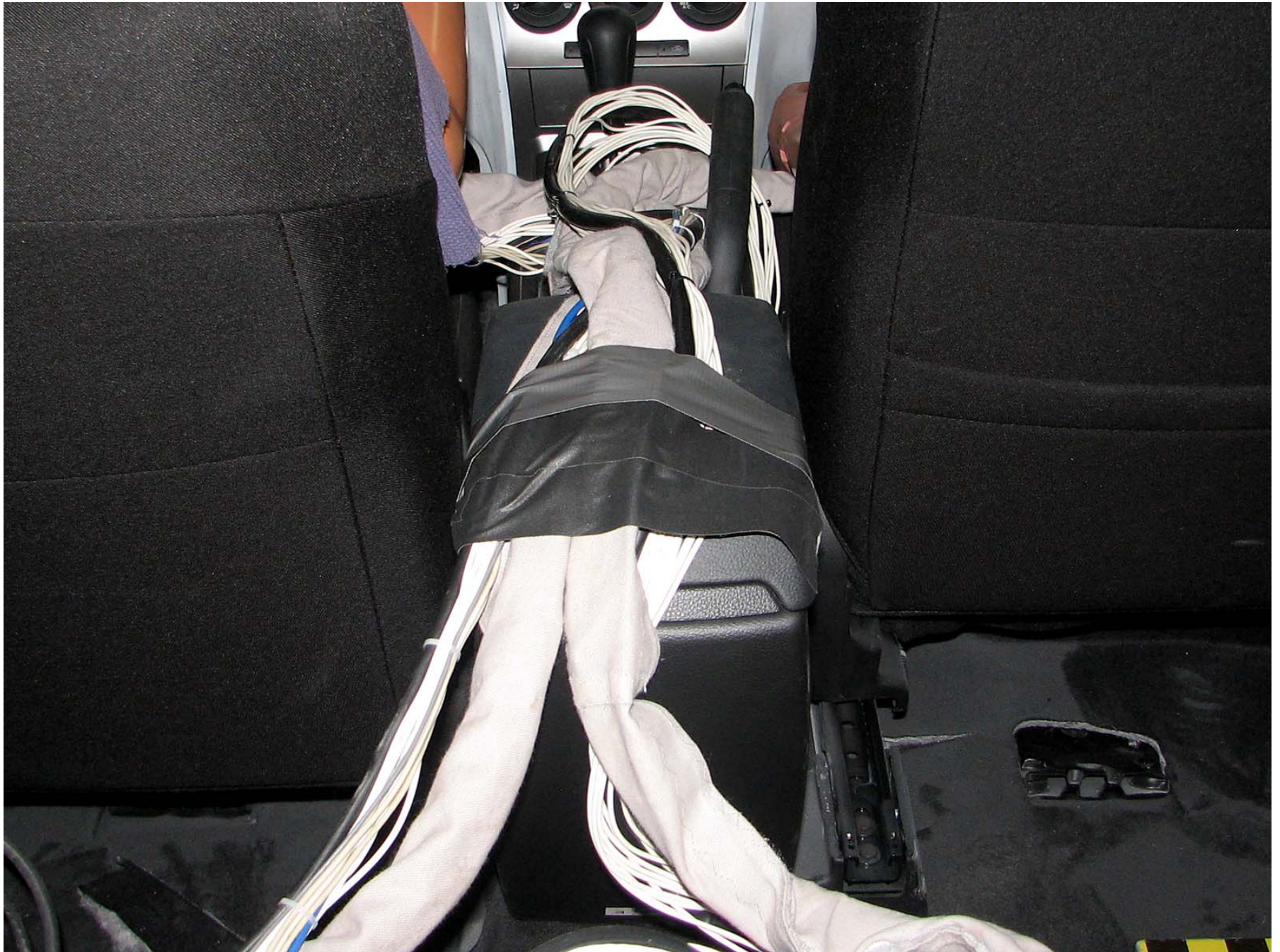
Figure A-26: Pre-Test Dummy Cable Routing
