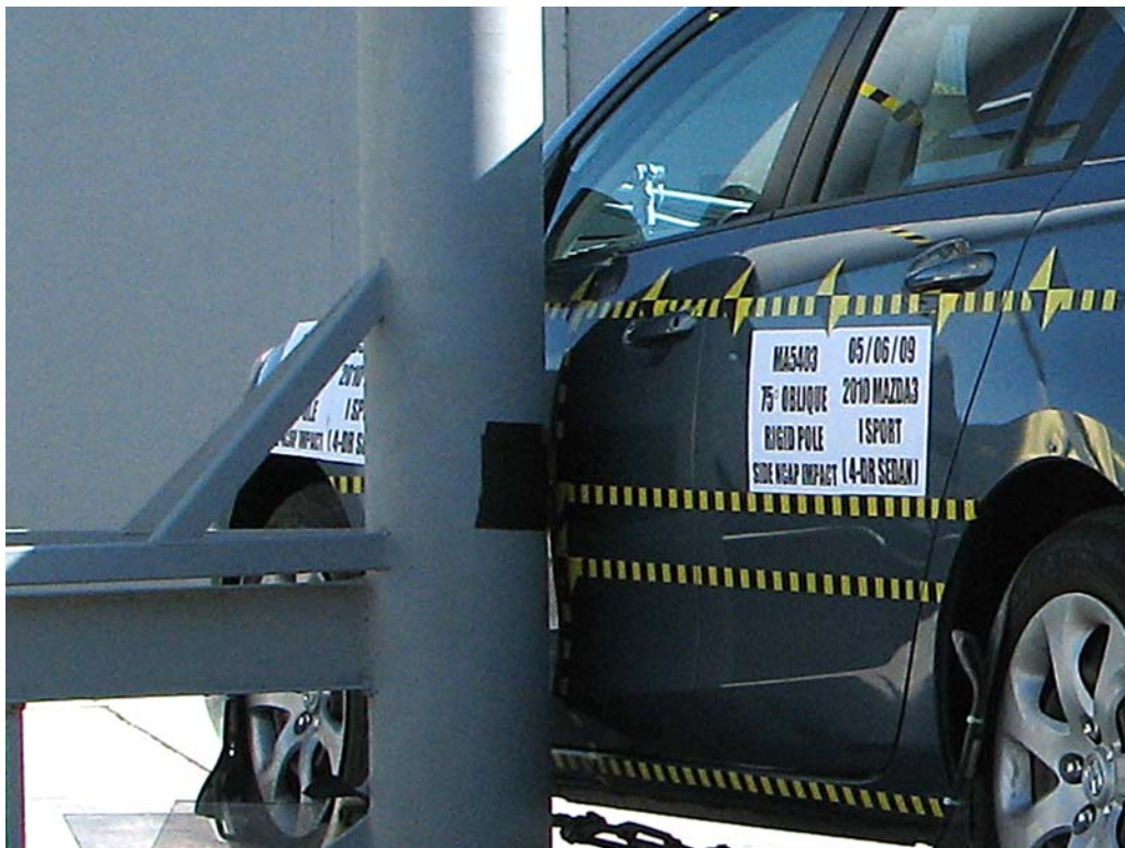
FIGURE 18. Pre-Test Right Side View of Pole Positioned Against Vehicle
