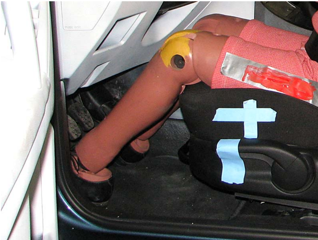
FIGURE 26. Pre-Test Placement of Dummy Feet
