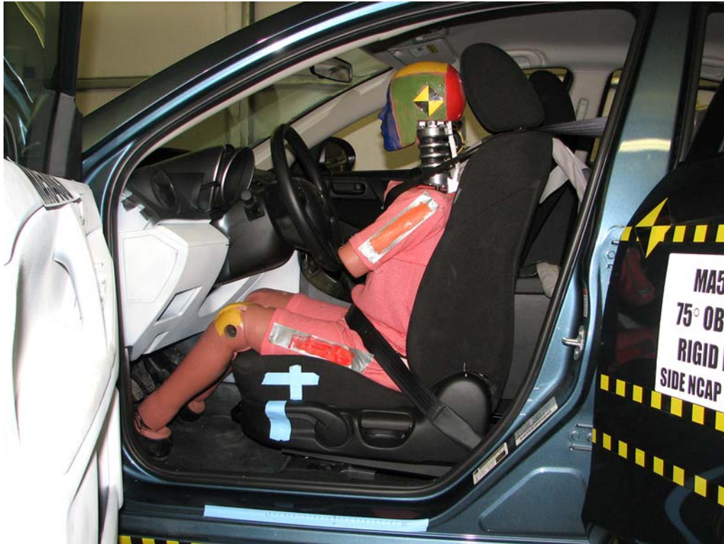
FIGURE 23. Pre-Test Left Side View of Dummy Showing Belt, Chalking, and Contact Switches (Door Open)
