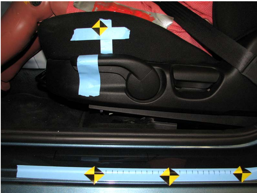
FIGURE 28. Pre-Test Close-Up Left Side View of Driver Seat Track Showing Seat Positioning
