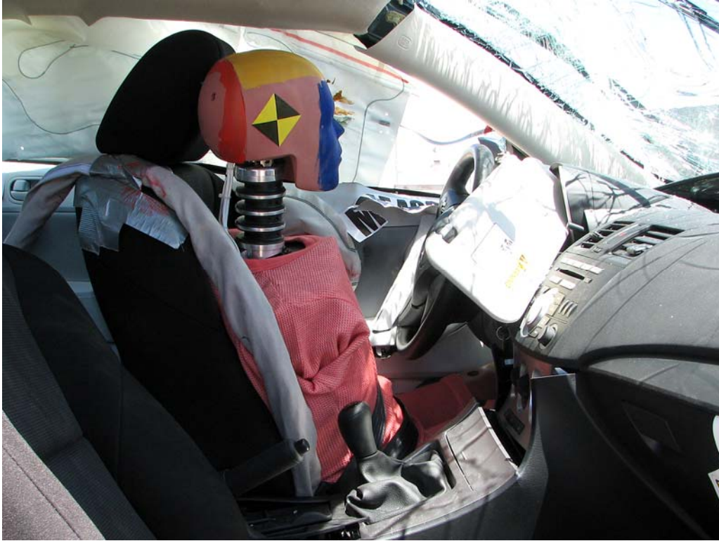
FIGURE 33. Post-Test Right Side View of Dummy and Front Seat Occupant Compartment (Through Window with Dummy)
