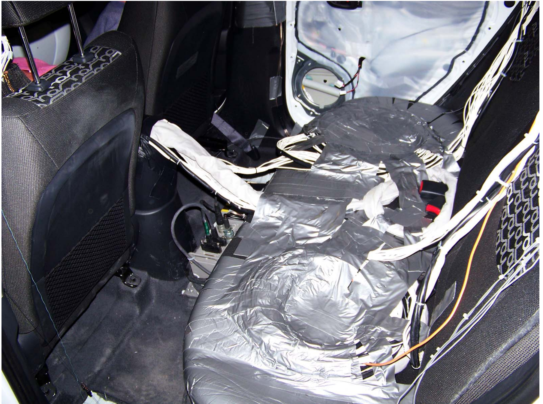
Figure A-26: Pre-Test Dummy Cable Routing
