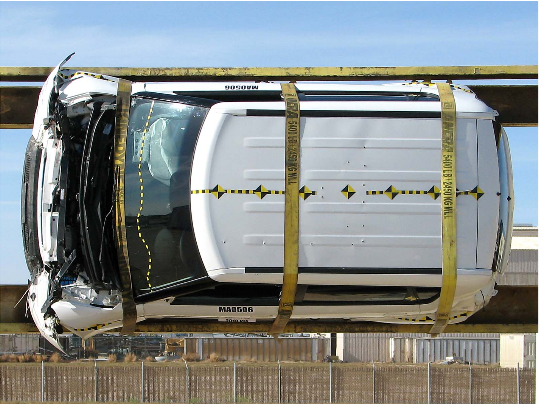
Figure A-68: Vehicle at 90° on Static Rollover Device
