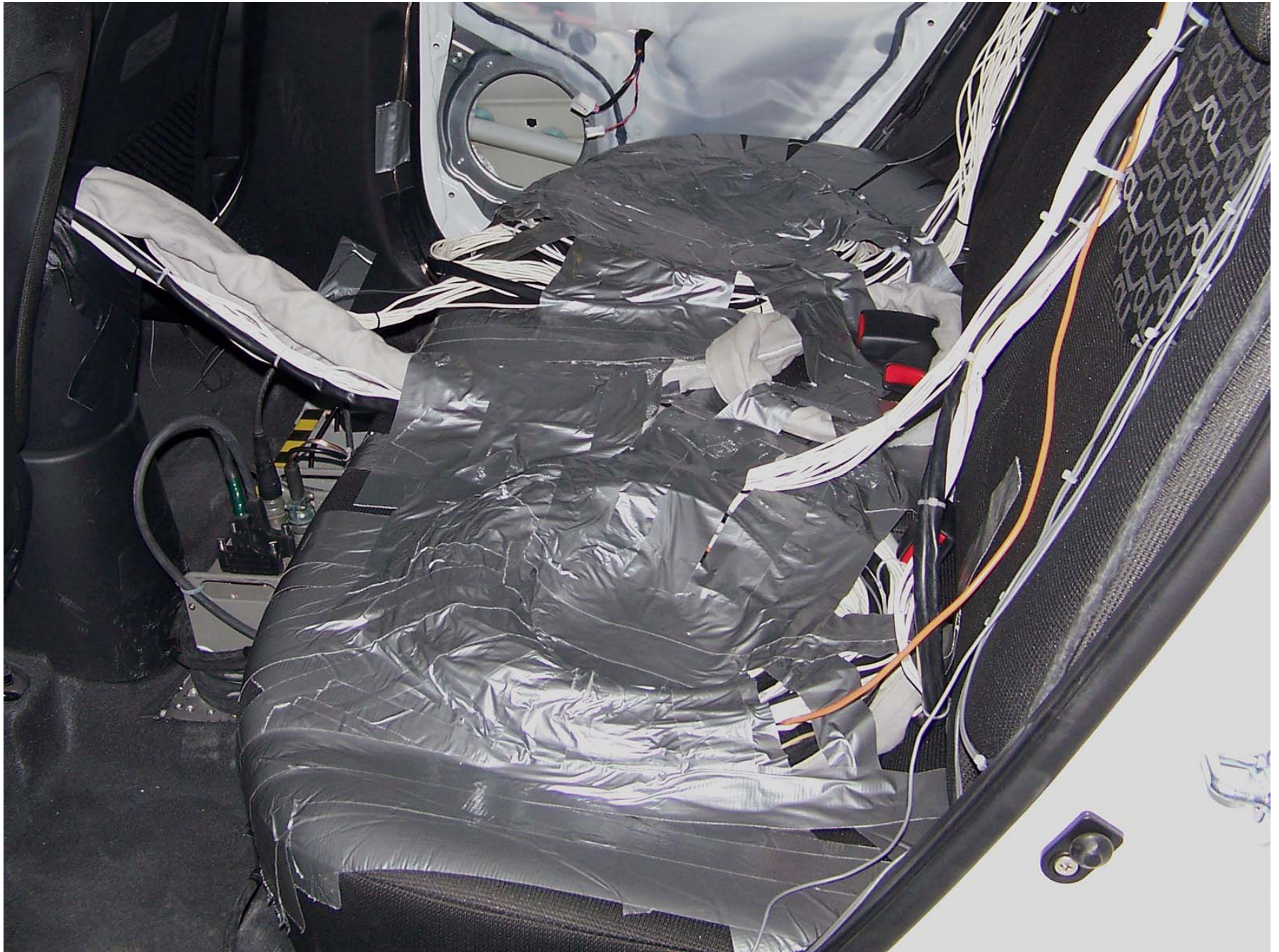
Figure A-27: Post-Test Dummy Cable Routing
