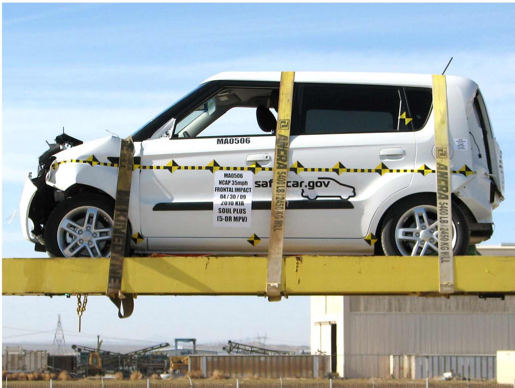
Figure A-71: Vehicle at 360° on Static Rollover Device
