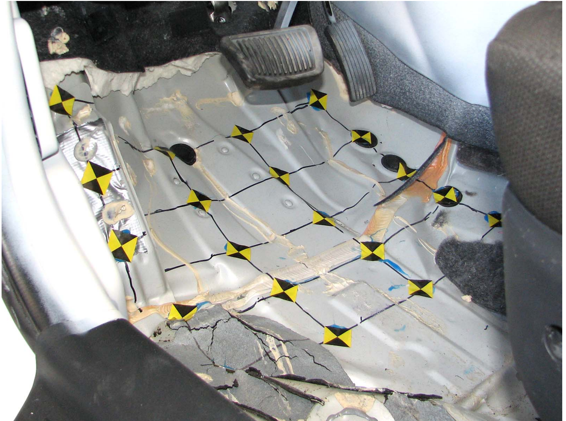
Figure A-41: Post-Test Driver's Side Floorpan
