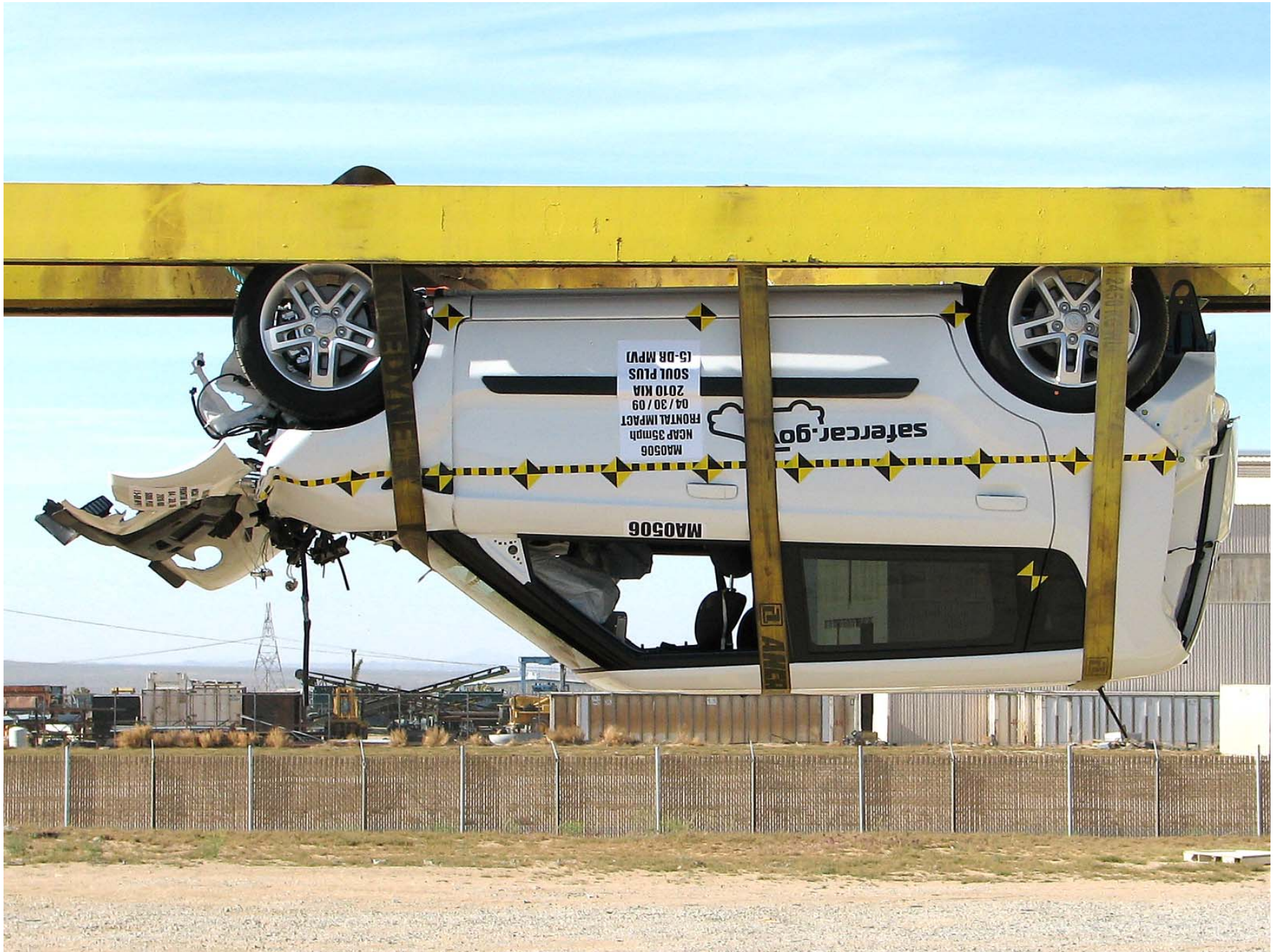
Figure A-69: Vehicle at 180° on Static Rollover Device
