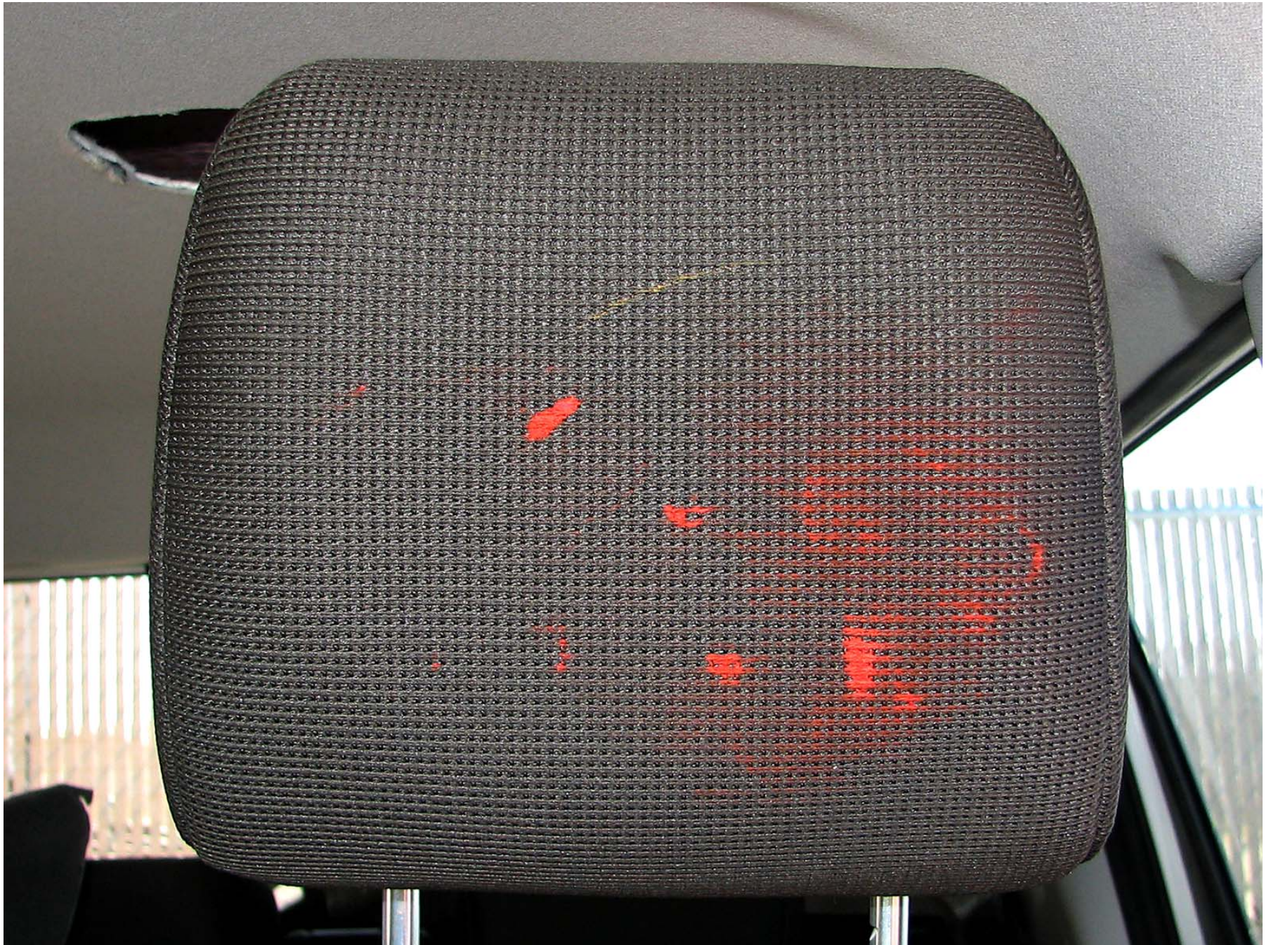
Figure A-44: Post-Test Driver Dummy Contact with Headrest
