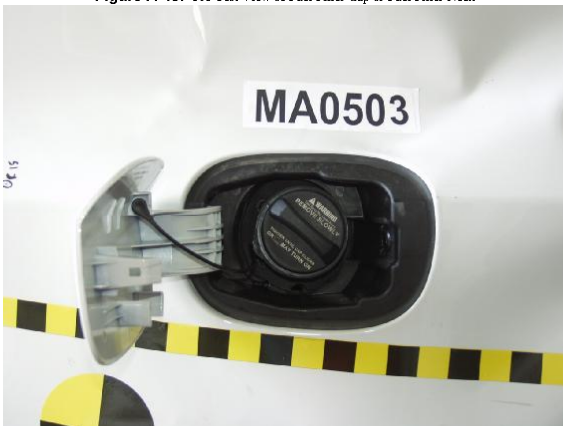
Figure A-46: Post-Test View of Fuel Filler Cap or Fuel Filler Neck
