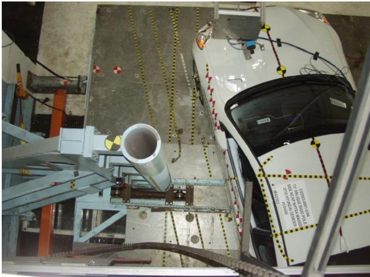
Figure A-15: Pre-Test Overhead View of Test Vehicle and Pole
