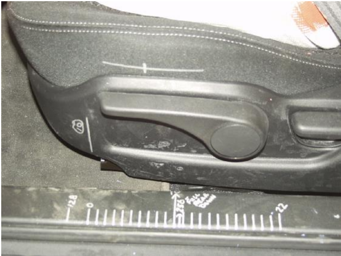
Figure A-35: Pre-Test Close-Up Left Side View of Driver Seat Track Showing Test Position (should include detent or millimeter markings)
