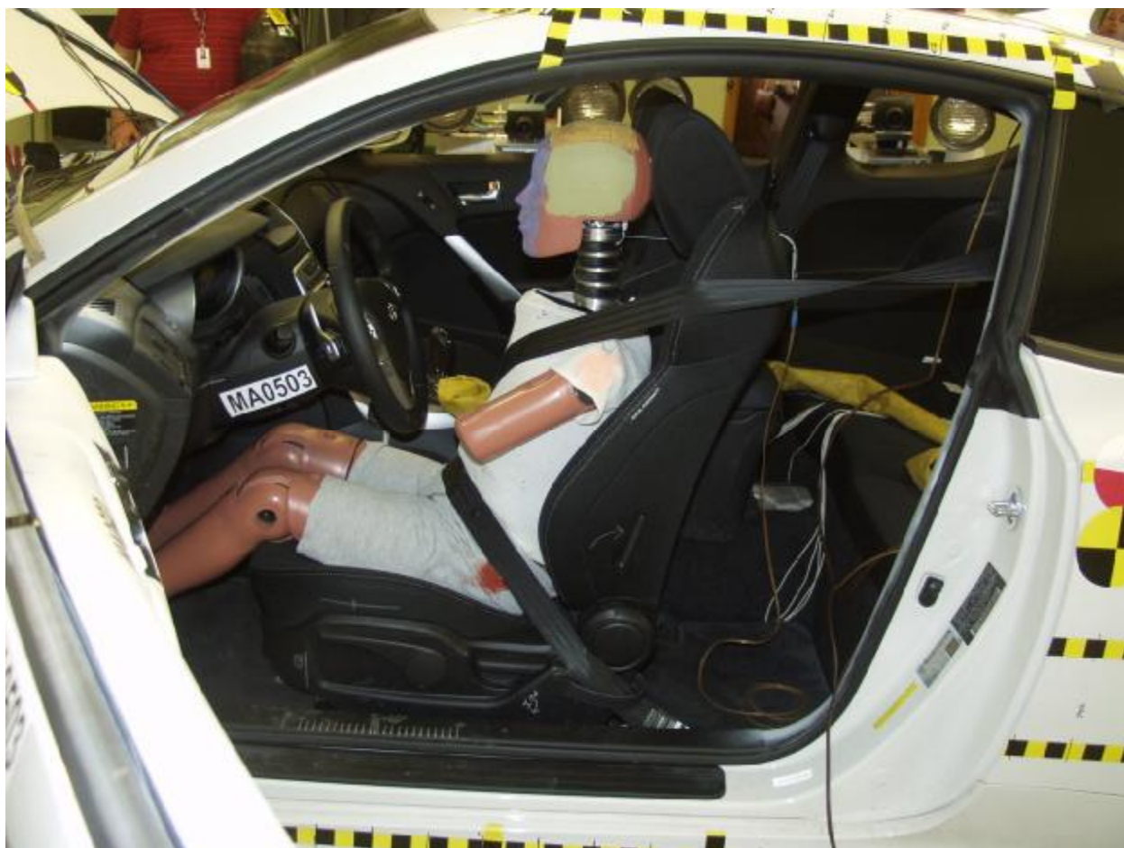
Figure A-23: Pre-Test Left Side View of Dummy Showing Belt, Chalking, and Contact Switches (Door Open)
