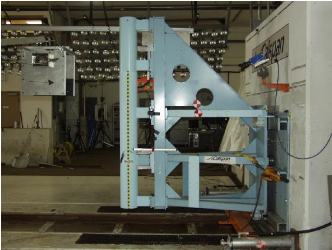
Figure A-45: Pre-Test Pole Barrier Side View
