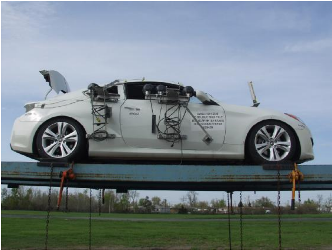
Figure A-45: FMVSS No. 301/305 Rollover 0°
