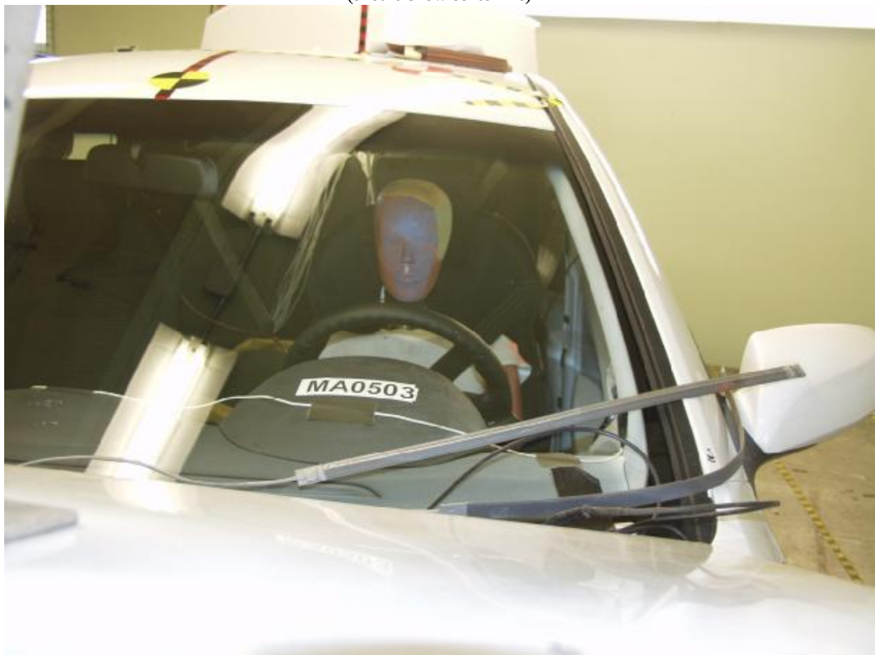
Figure A-27: Pre-Test Frontal View of Dummy Head and Shoulders in Relation to Head Restraint
