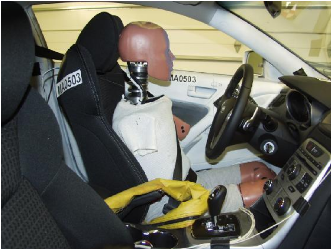
Figure A-41: Pre-Test Right Side View of Dummy and Front Seat Occupant Compartment (Through Vehicle with Door Open)
