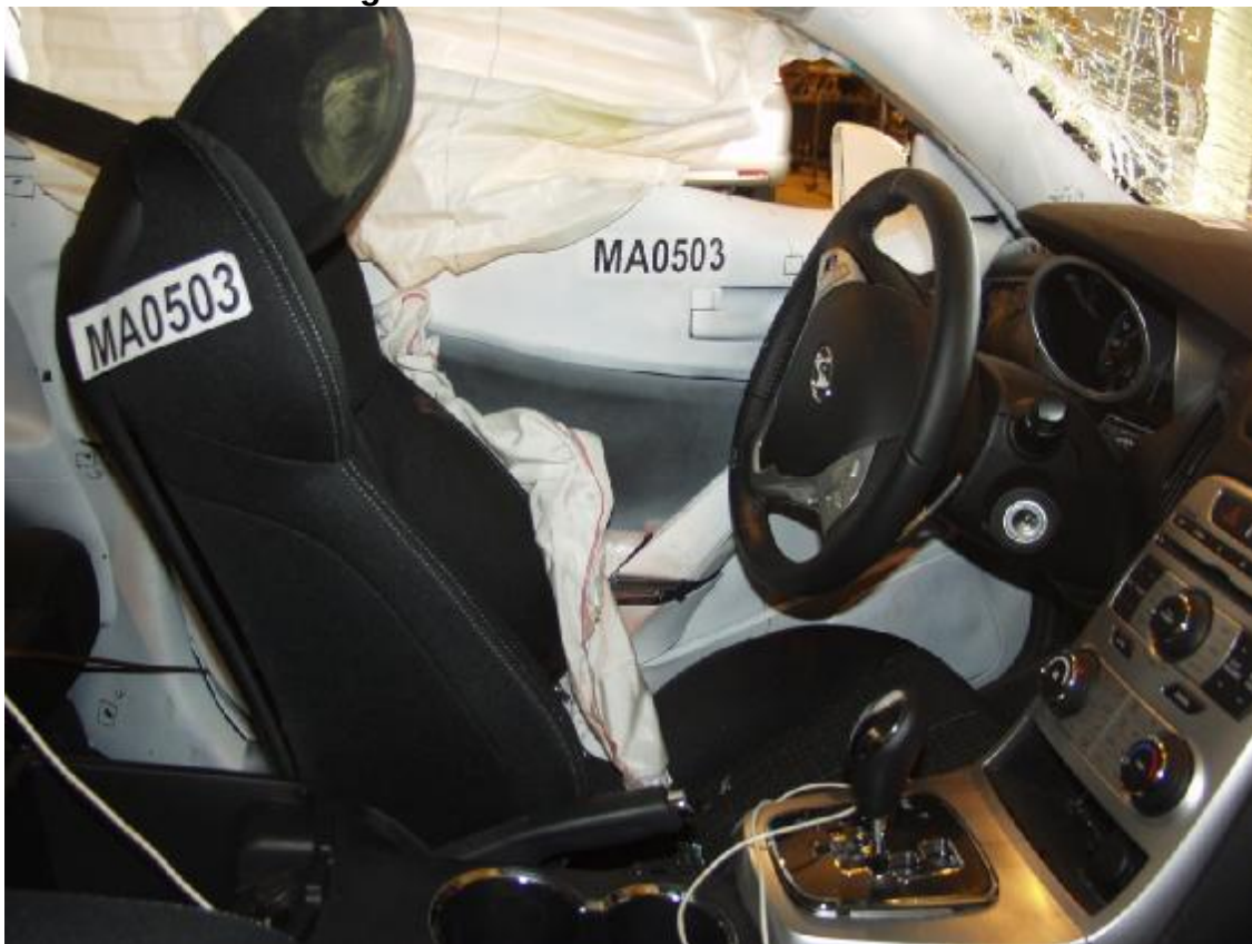
Figure A-44: Post-Test Inner Door Panel View Showing Dummy Contact Location
