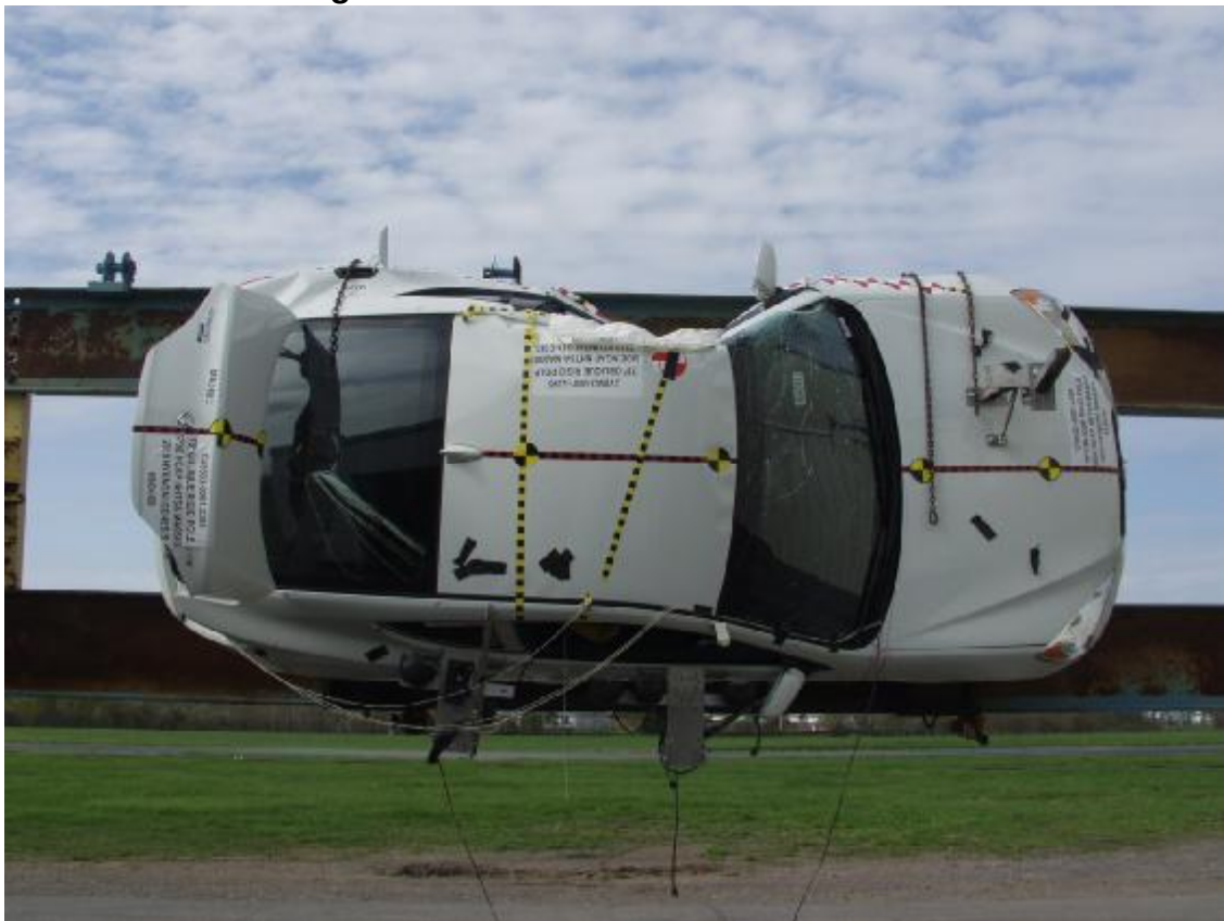
Figure A-46: FMVSS No. 301/305 Rollover 270°
