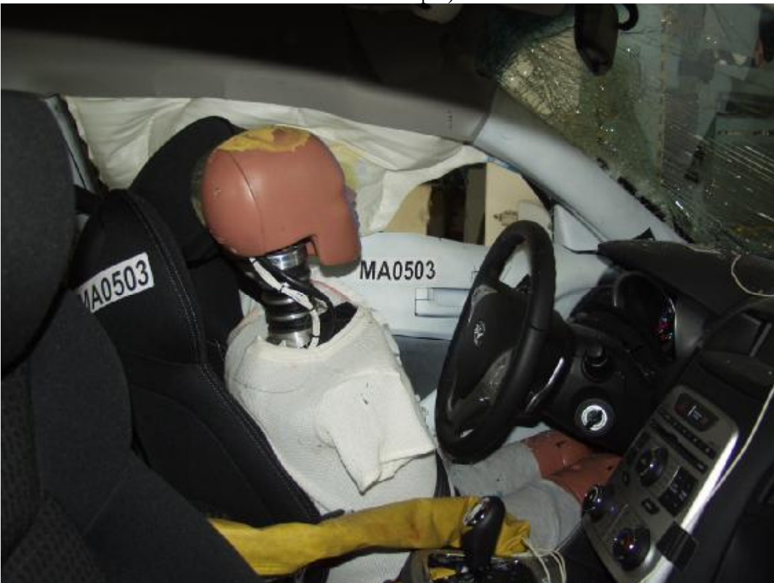
Figure A-42: Post-Test Right Side View of Dummy and Front Seat Occupant Compartment (Through Vehicle with Door Open)
