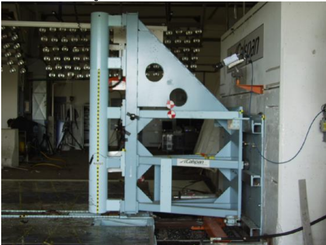
Figure A-46: Post-Test Pole Barrier Side View
