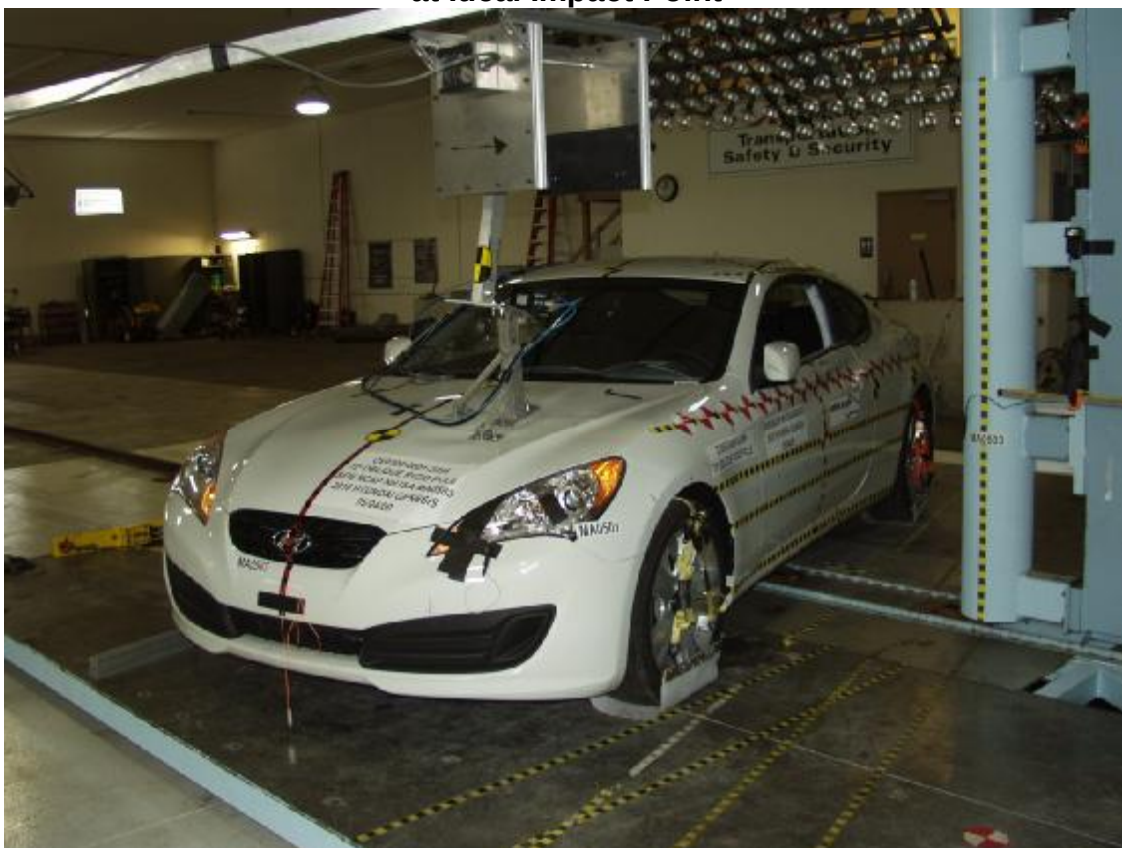
Figure A-18: Pre-Test Right Side View of Pole Positioned Against Side of Vehicle at Ideal Impact Point
