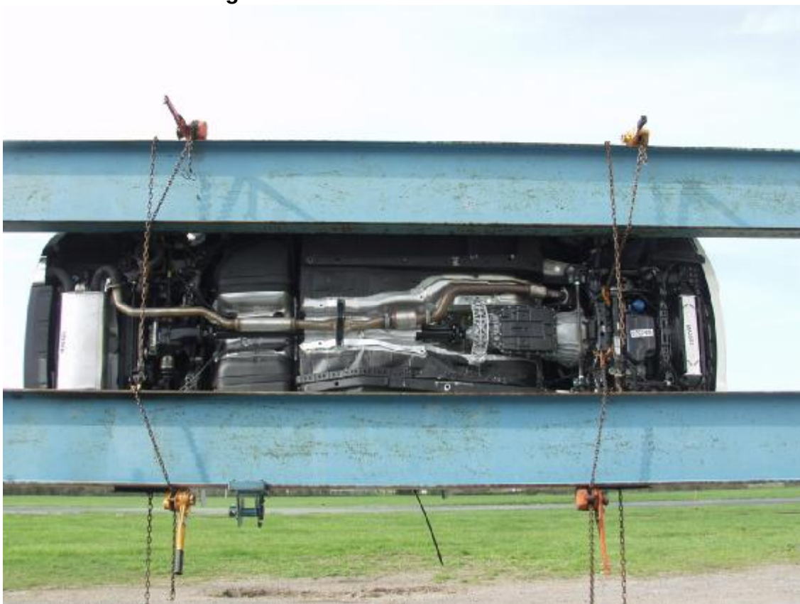
Figure A-46: FMVSS No. 301/305 Rollover 90°
