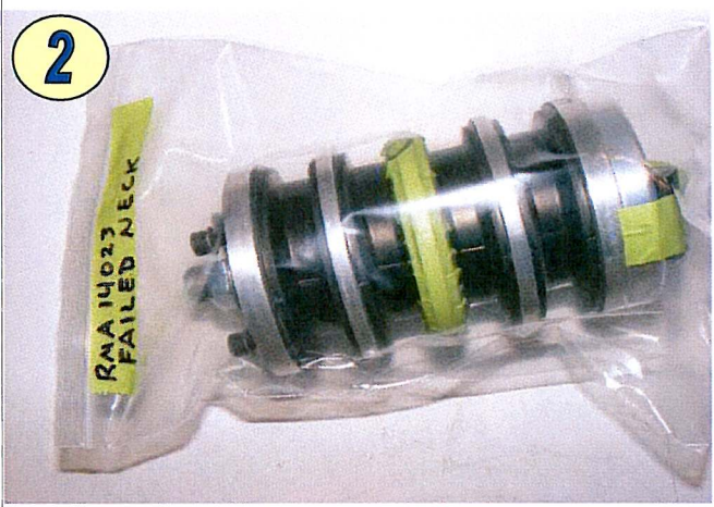
Failed Certification - Neck S/N = 705
