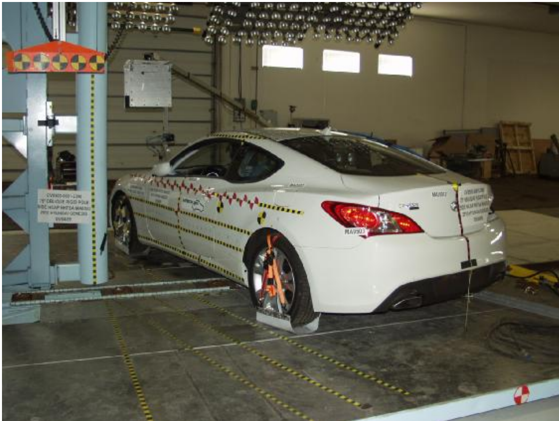
Figure A-17: Pre-Test Left Side View of Pole Positioned Against Side of Vehicle at Ideal Impact Point
