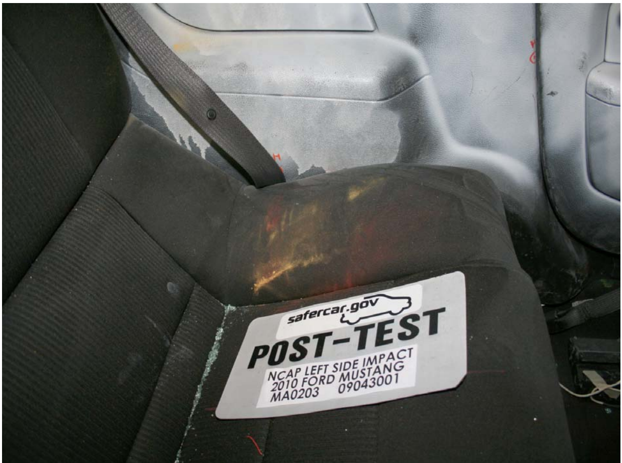
Post-Test Passenger Dummy Lower Torso Contact
