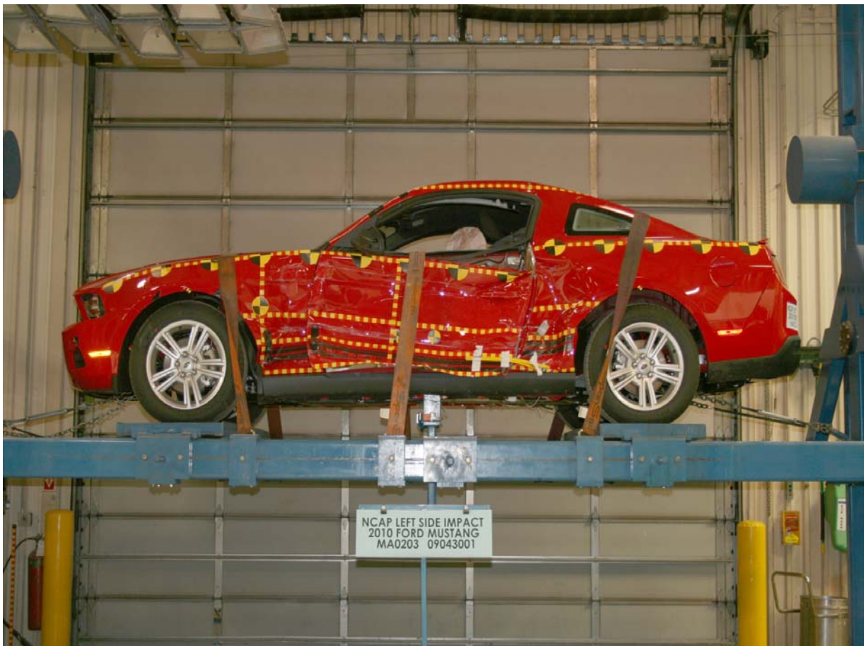
Vehicle on Rollover Device (360 Degrees)
