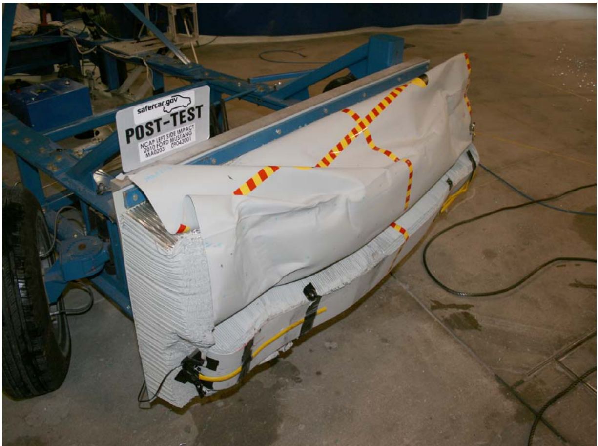
Post-Test Right Side View of Deformable Barrier
