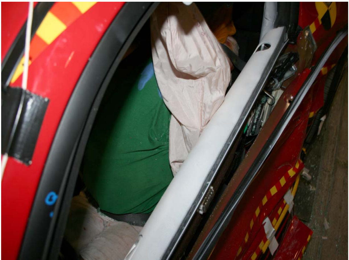
Post-Test Driver Dummy Clearance From Door
