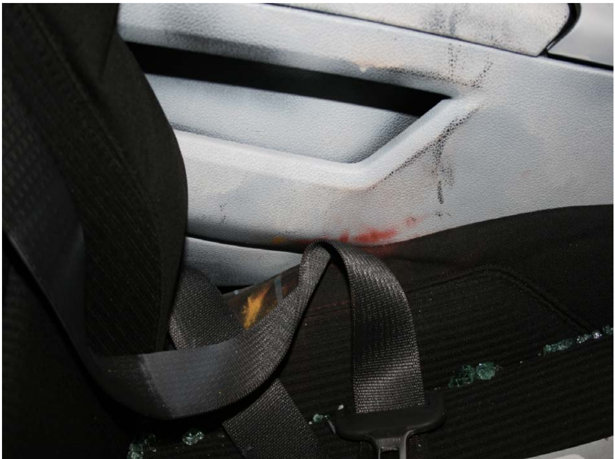
Post-Test Driver Dummy Lower Torso Contact
