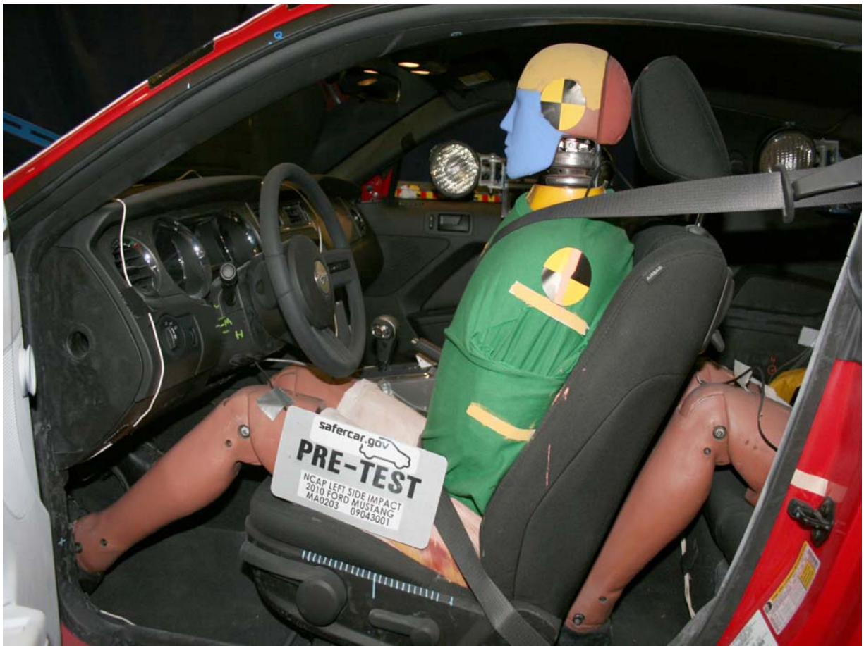
Pre-Test Driver Dummy (Door Open)
