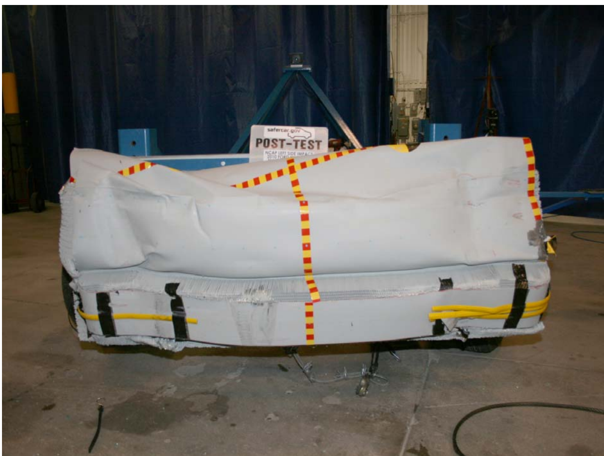
Post-Test Front View of Deformable Barrier
