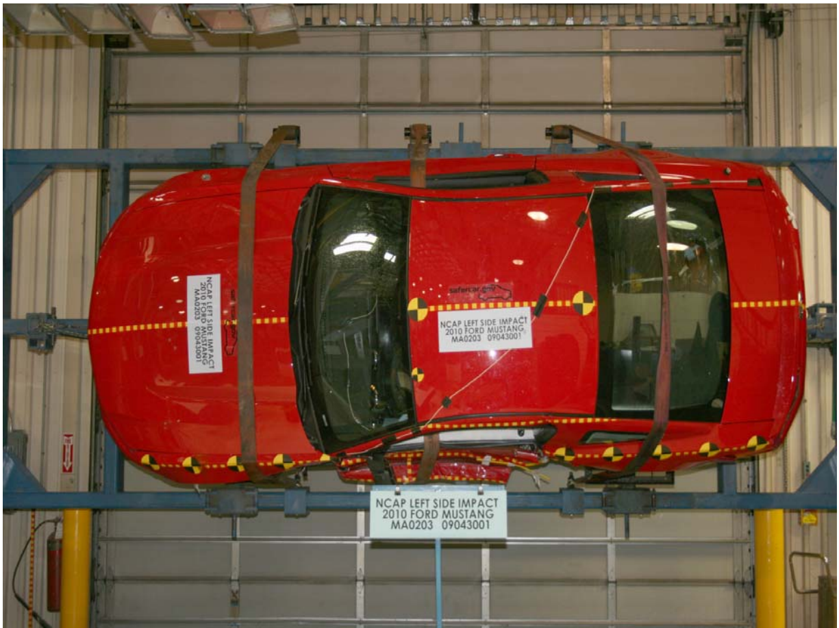
Vehicle on Rollover Device (90 Degrees)
