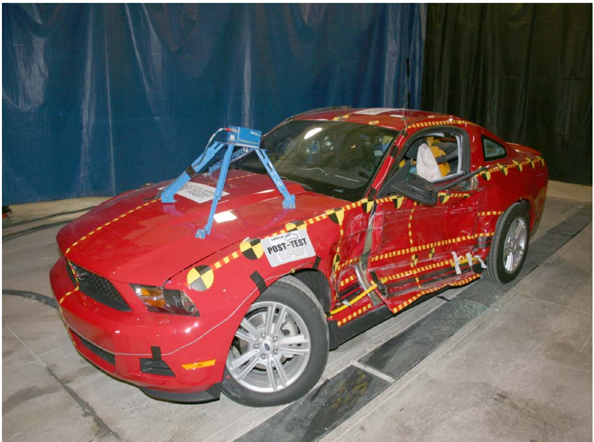
Post-Test Left Front \frac{3}{4} View
