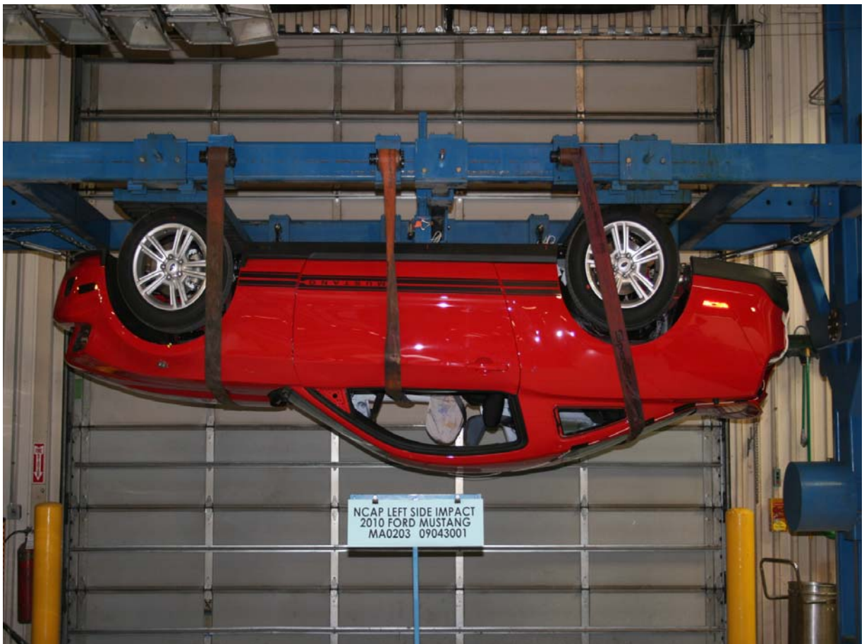
Vehicle on Rollover Device (180 Degrees)
