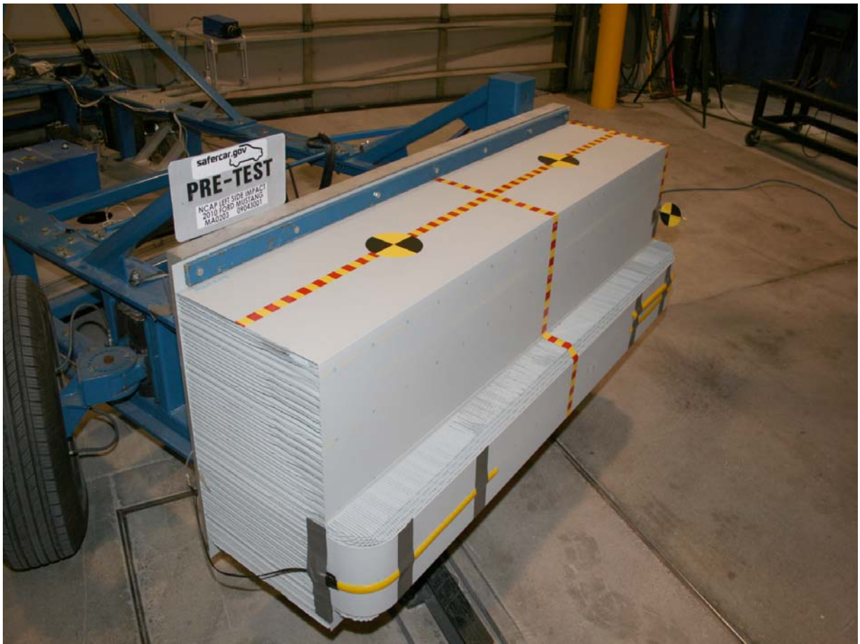
Pre-Test Right Side View of Deformable Barrier
