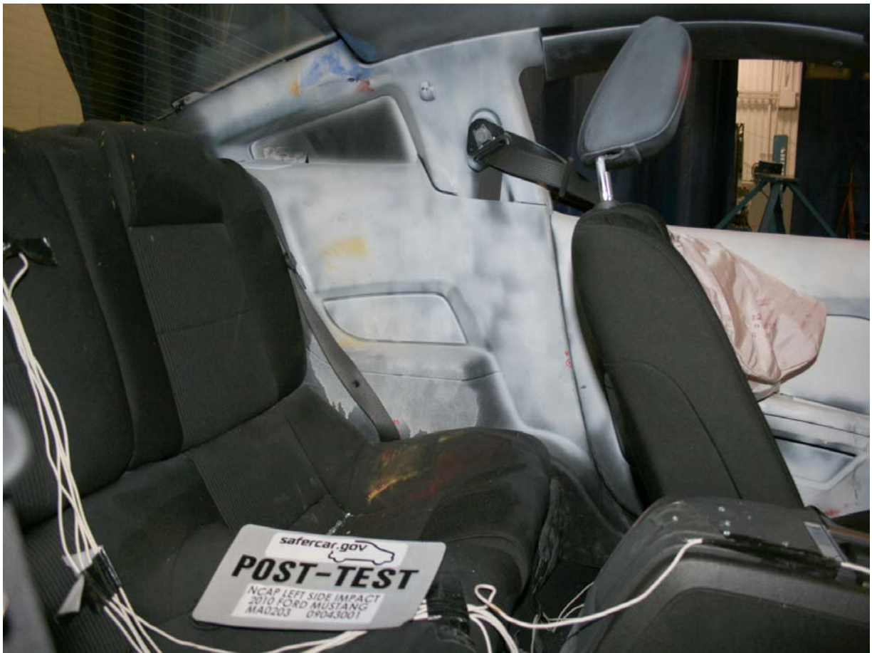
Post-Test Passenger Dummy Contact
