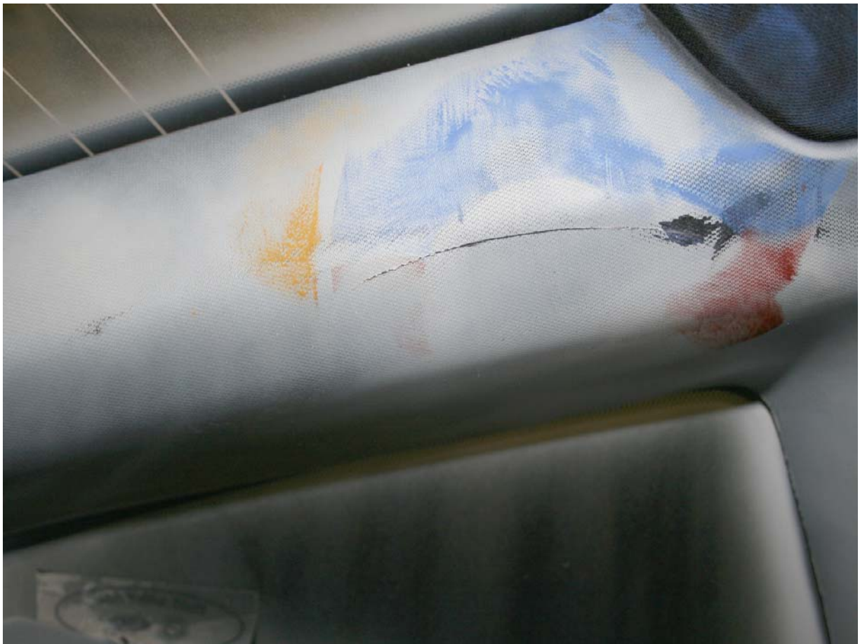
Post-Test Passenger Dummy Head Contact View 1
