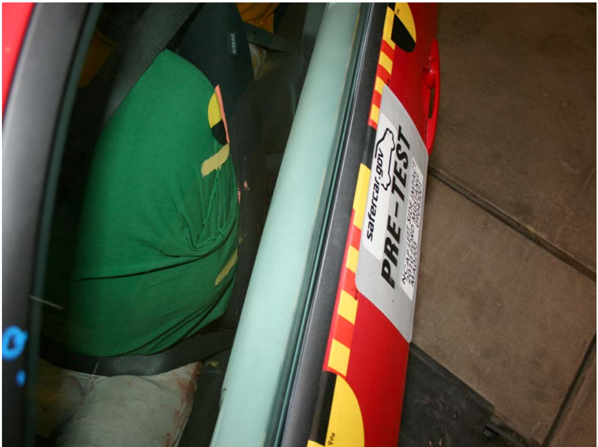
Pre-Test Driver Dummy Clearance From Door
