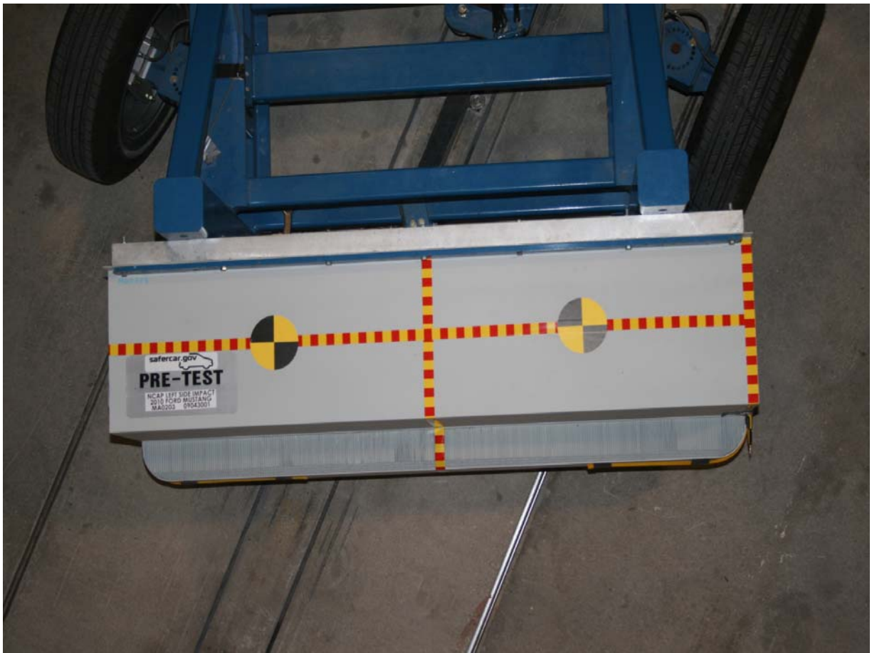
Pre-Test Top View of Deformable Barrier
