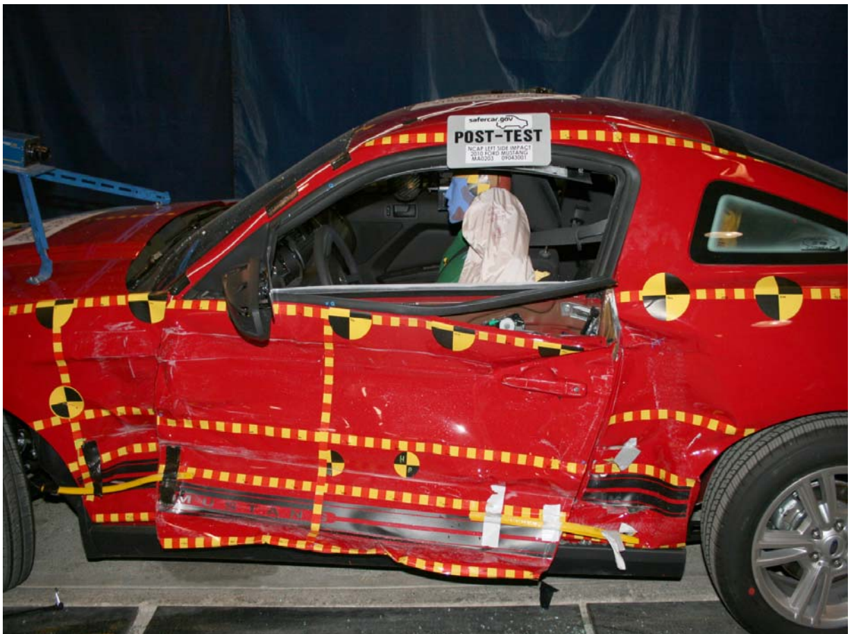
Post-Test Left Side Impact Close-up
