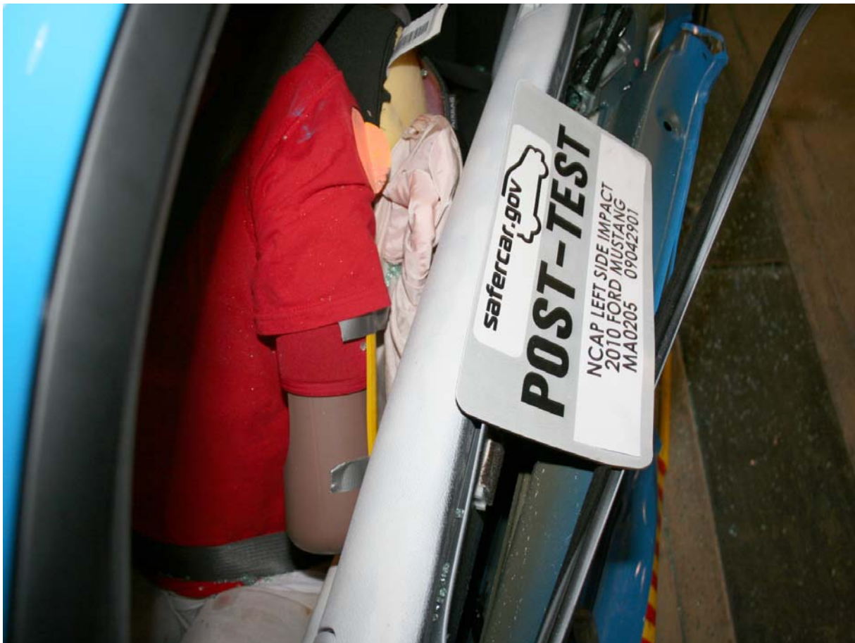
Post-Test Driver Dummy and Door Clearance View
