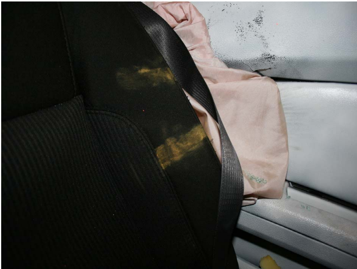
Post-Test Driver Dummy Door Contact View
