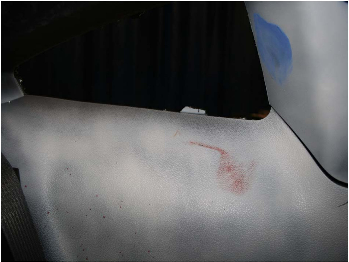
Post-Test Passenger Dummy Head Contact View 2
