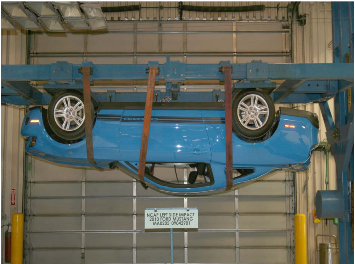
FMVSS No. 301/305 Rollover 180 Degrees
