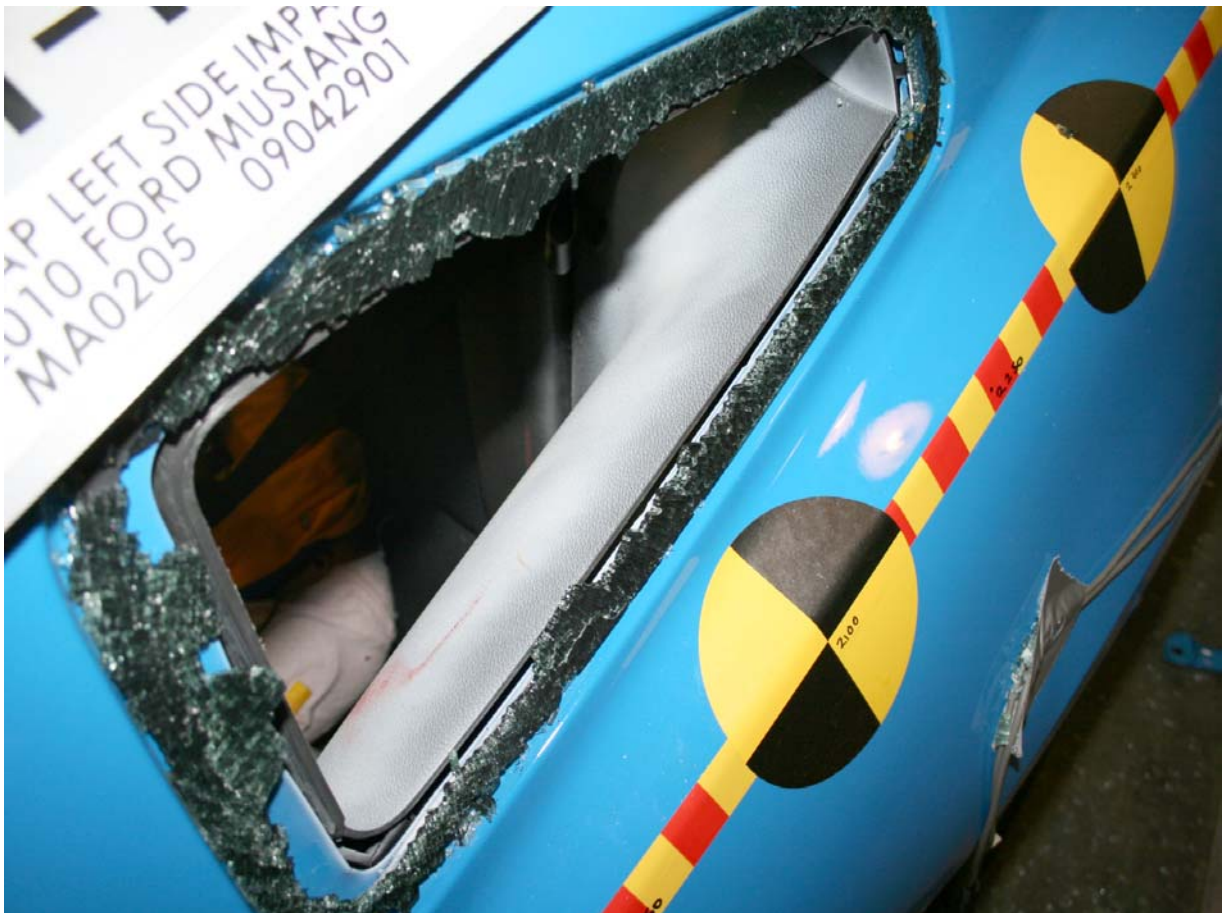
Post-Test Passenger Dummy and Door Clearance View
