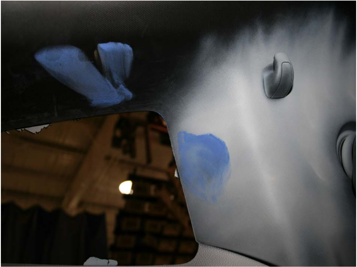
Post-Test Passenger Dummy Head Contact View
