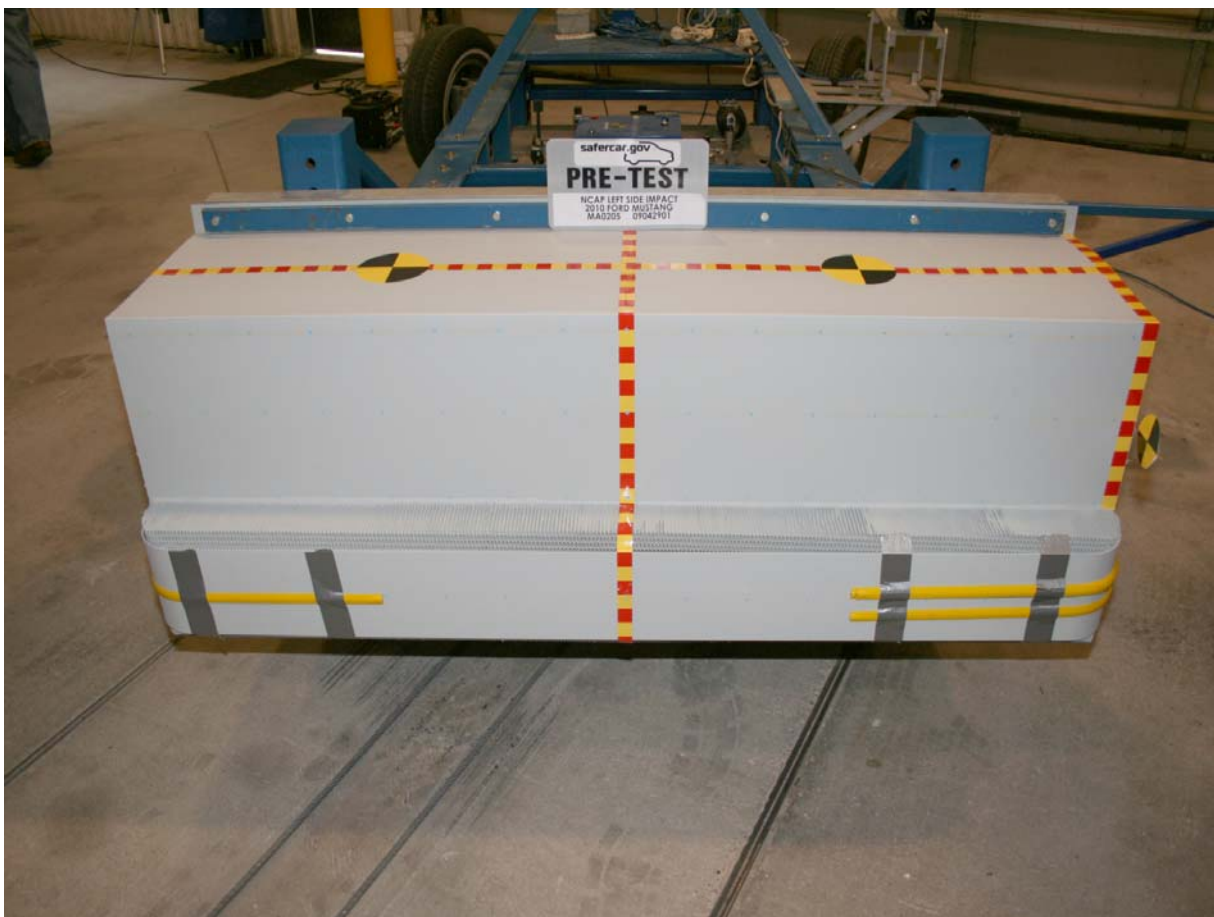
Pre-Test Front View of MDB Impactor Face
