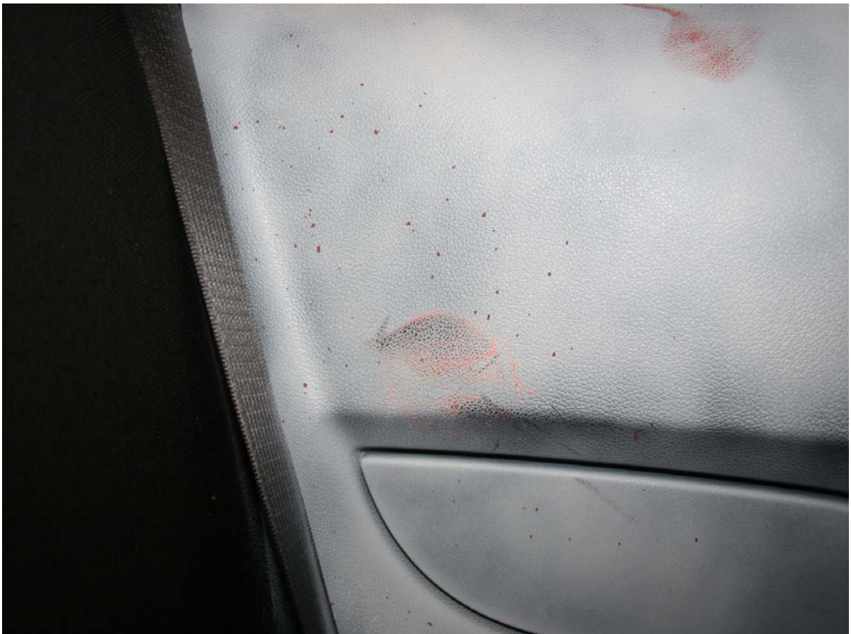
Post-Test Passenger Dummy Door Contact View
