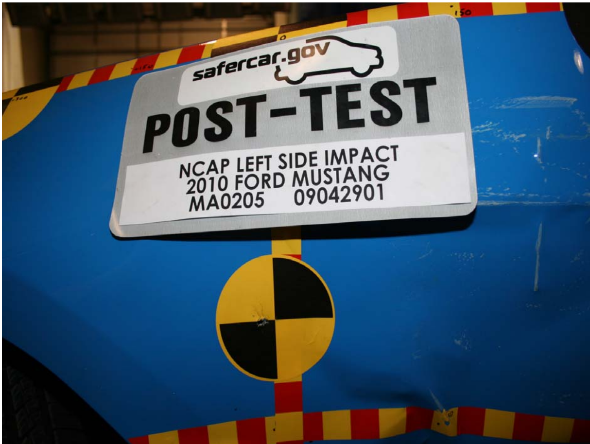
Post-Test Close-Up View of Impact Point Target Showing Impact Point Location
