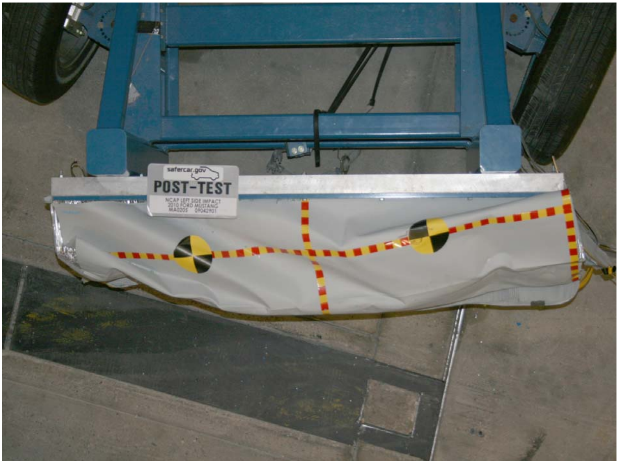
Post-Test Top View of MDB Impactor Face
