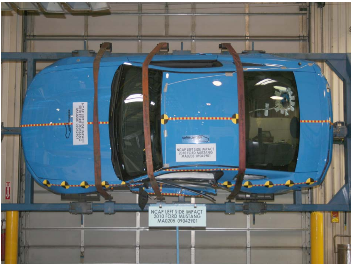
FMVSS No. 301/305 Rollover 90 Degrees
