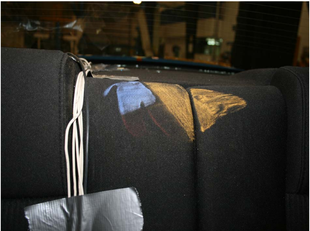
Post-Test Passenger Dummy Head Contact View 3
