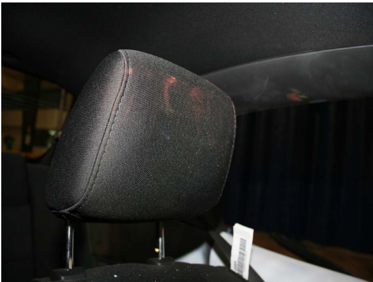
Post-Test Driver Dummy Head Contact View
