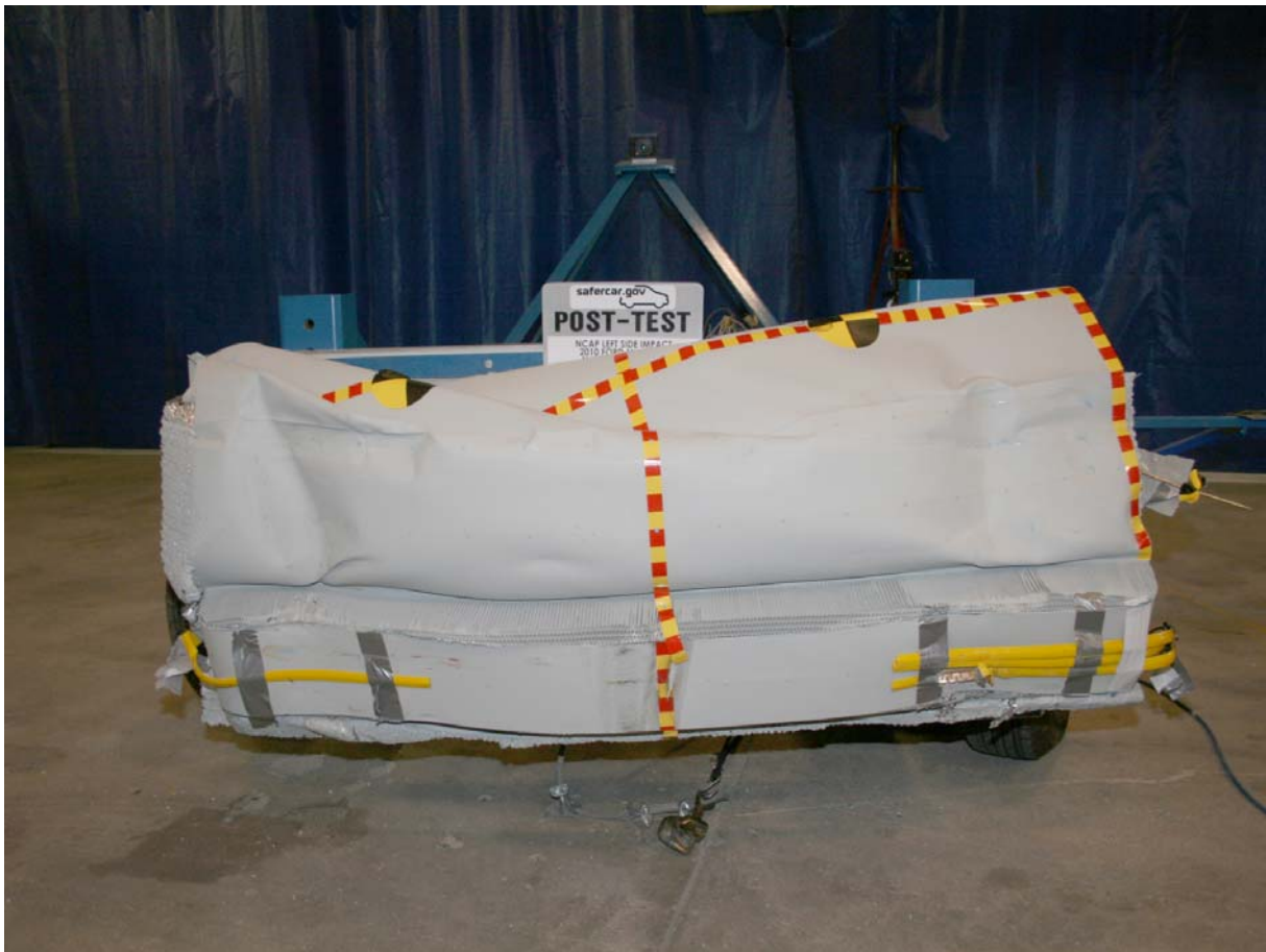
Post-Test Front View of MDB Impactor Face
