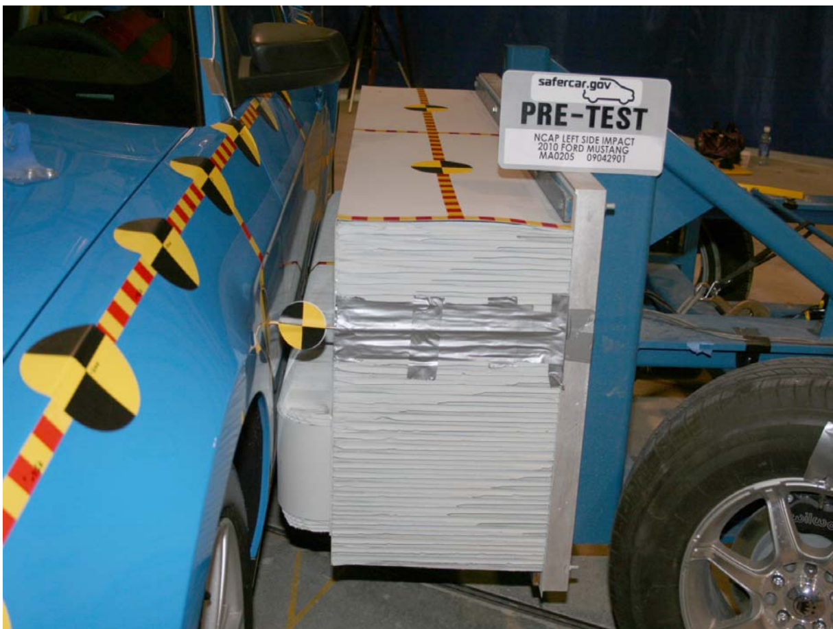
Pre-Test Left Side View of MDB Positioned Against the Side of the Test Vehicle at the Ideal Impact Point
