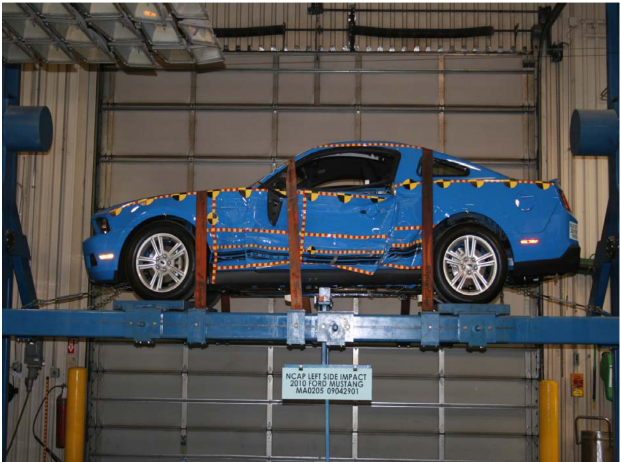
FMVSS No. 301/305 Rollover 0 Degrees
