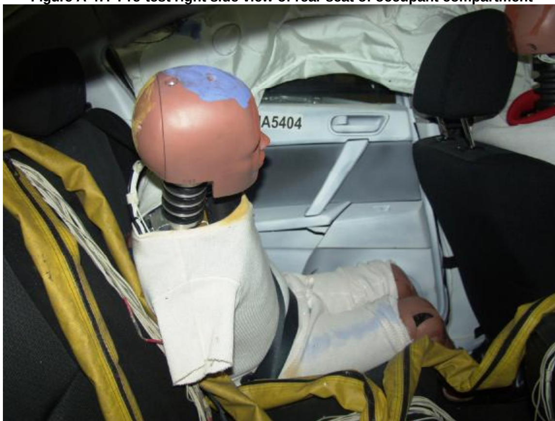
Figure A-48: Post-test right side view of rear seat of occupant compartment
