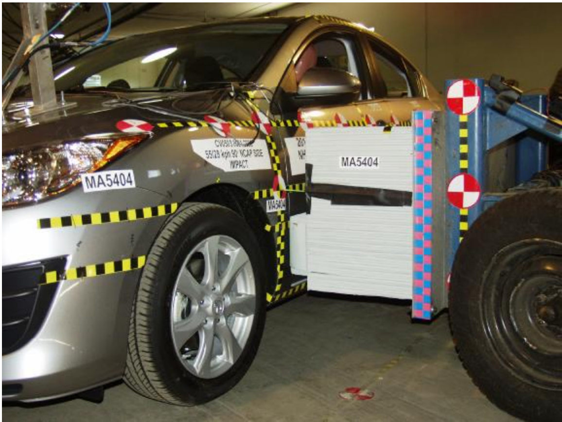
Figure A-17: Pre-test left side view of MDB positioned against vehicle
