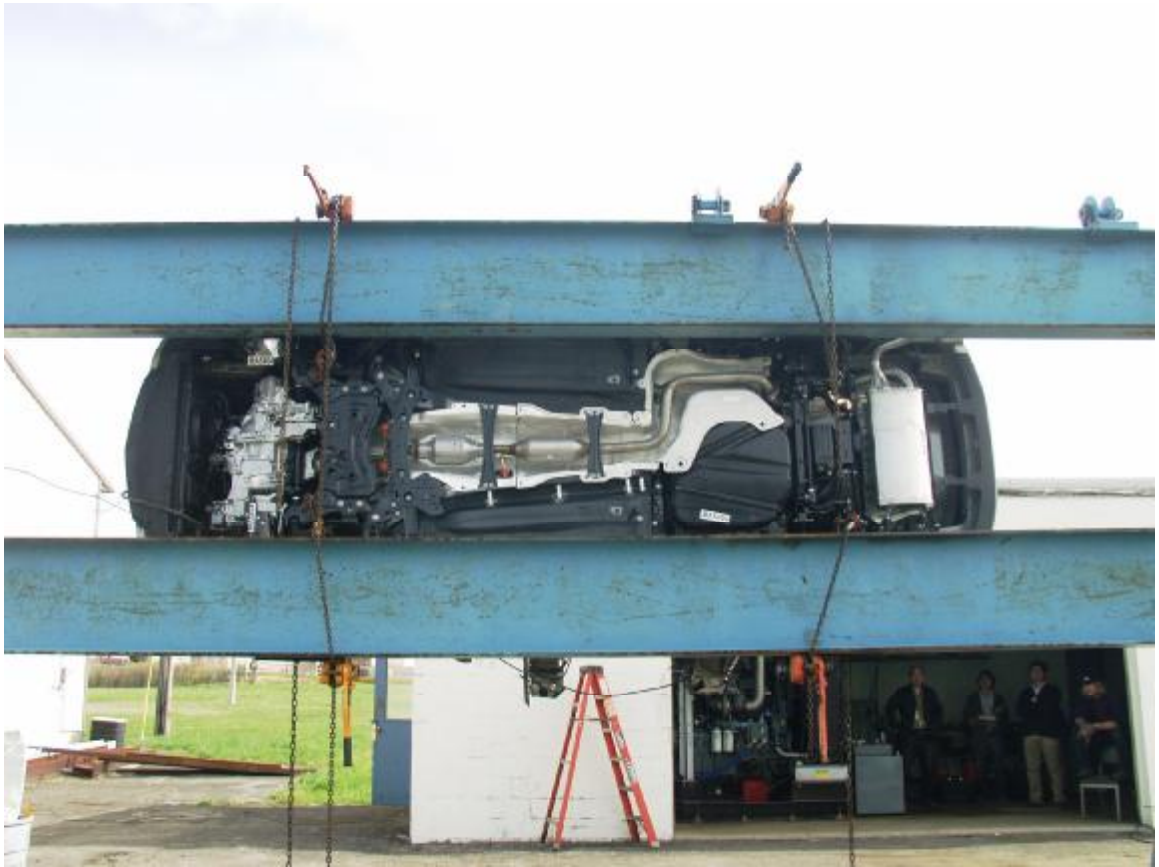
Figure A-65: FMVSS 301/305 rollover 90°
