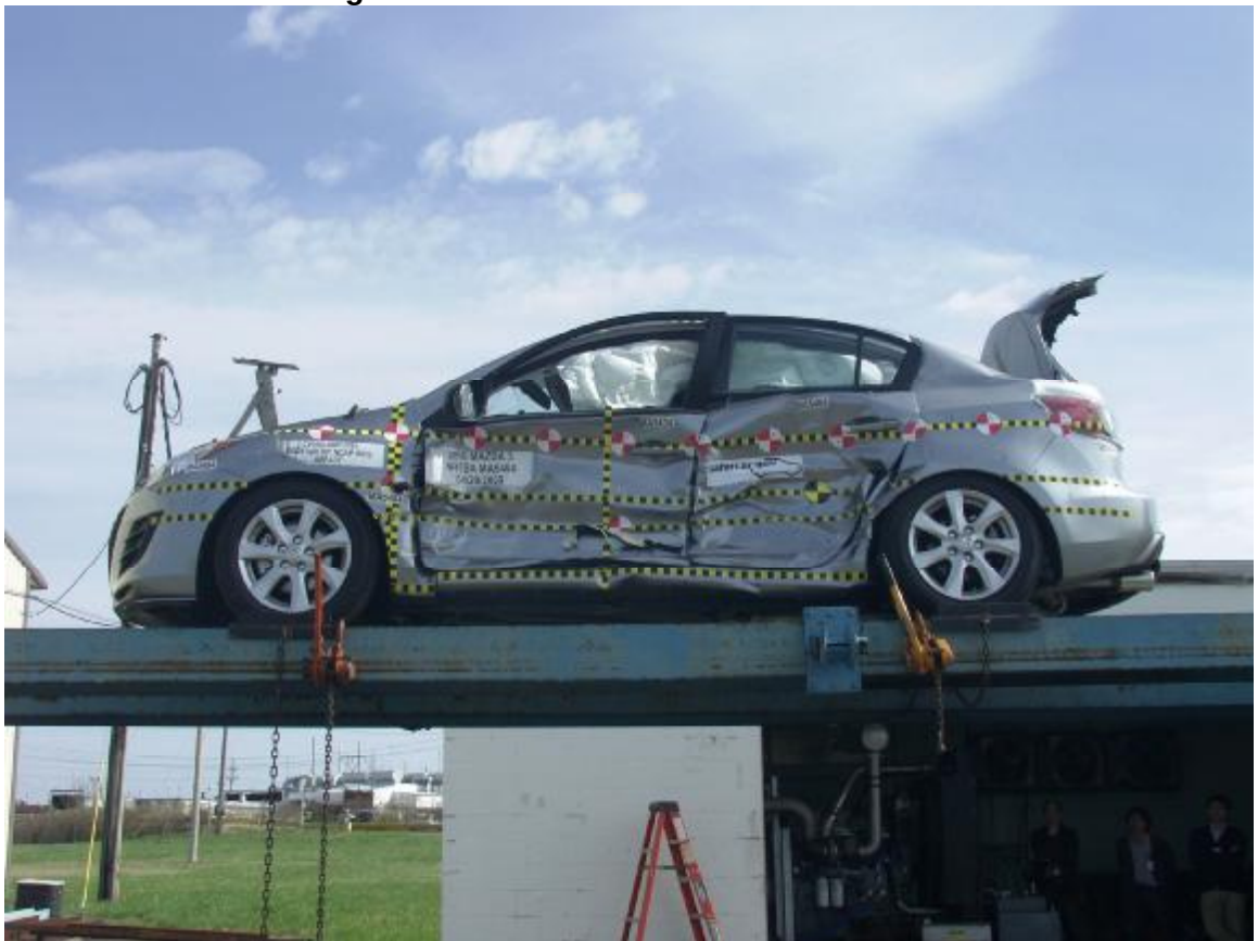
Figure A-68: FMVSS 301/305 rollover 360°
