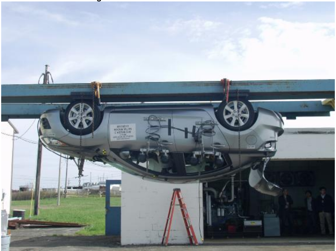
Figure A-66: FMVSS 301/305 rollover 180°
