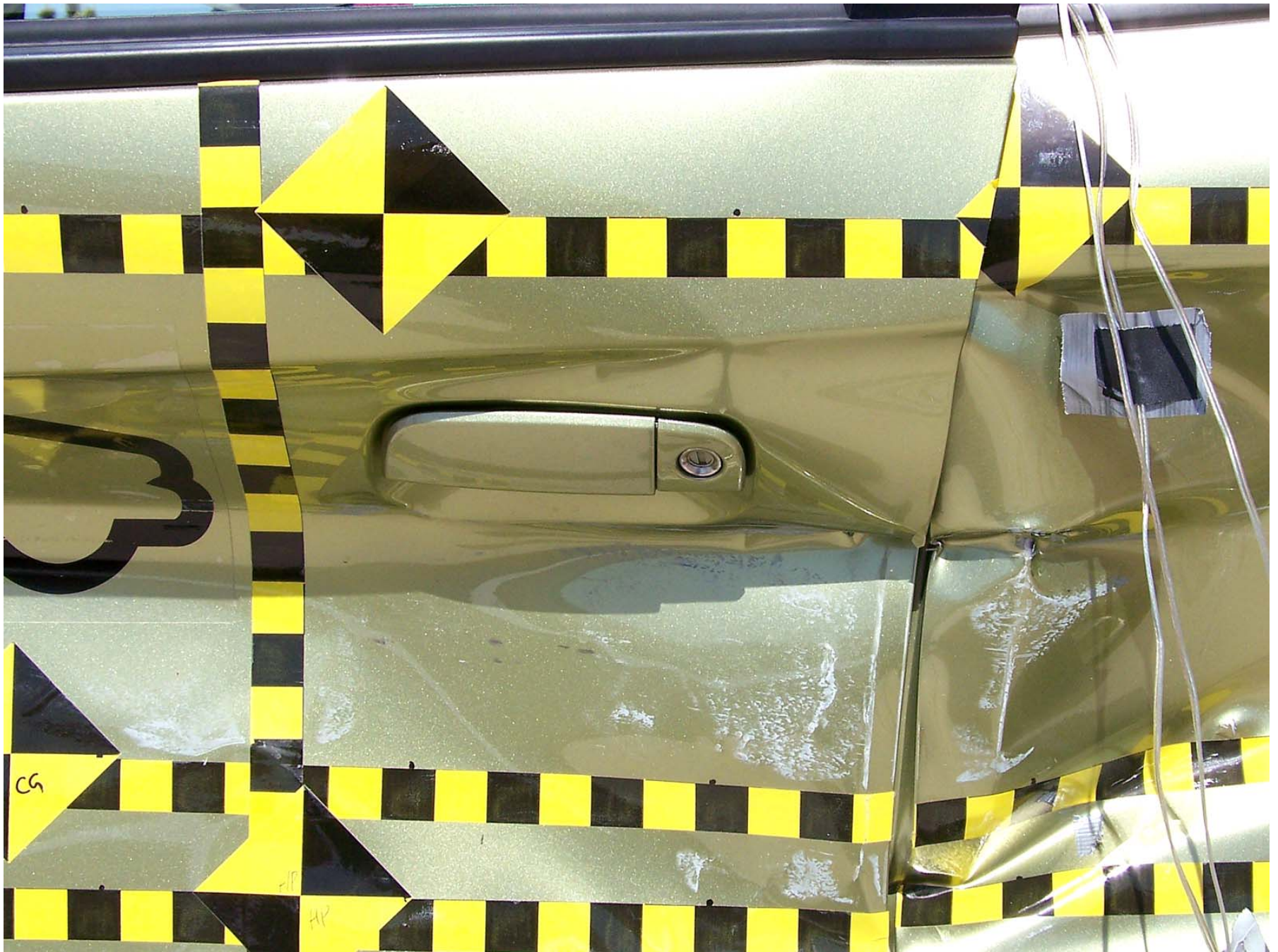
Figure A-22: Post-Test Left Front Door Latch Close-Up (With Door Closed)
