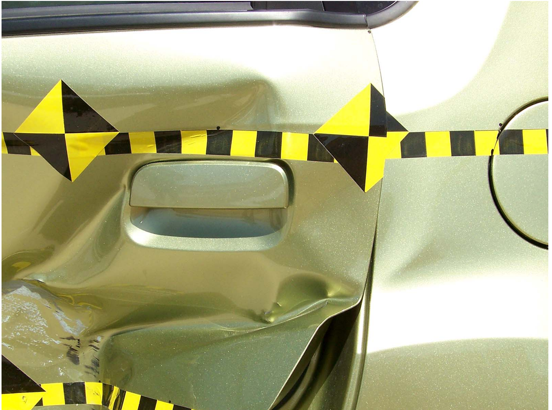
Figure A-24: Post-Test Left Rear Door Latch Close-Up (With Door Closed)
