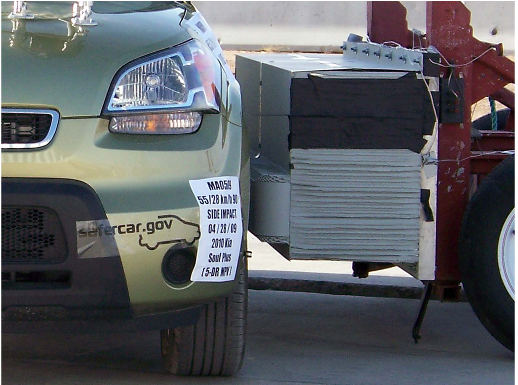
Figure A-17: Pre-Test Left Side View of MDB Positioned Against Test Vehicle
