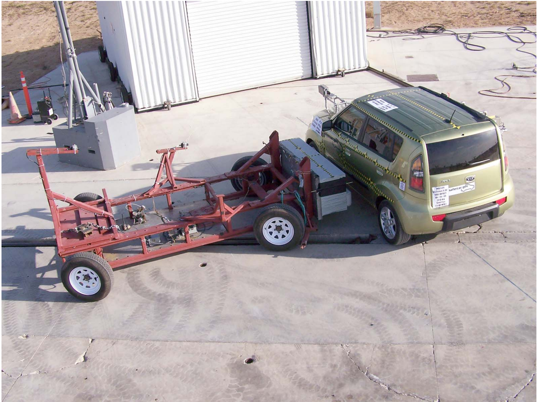
Figure A-15: Pre-Test Overhead View of Test Vehicle with MDB Positioned
