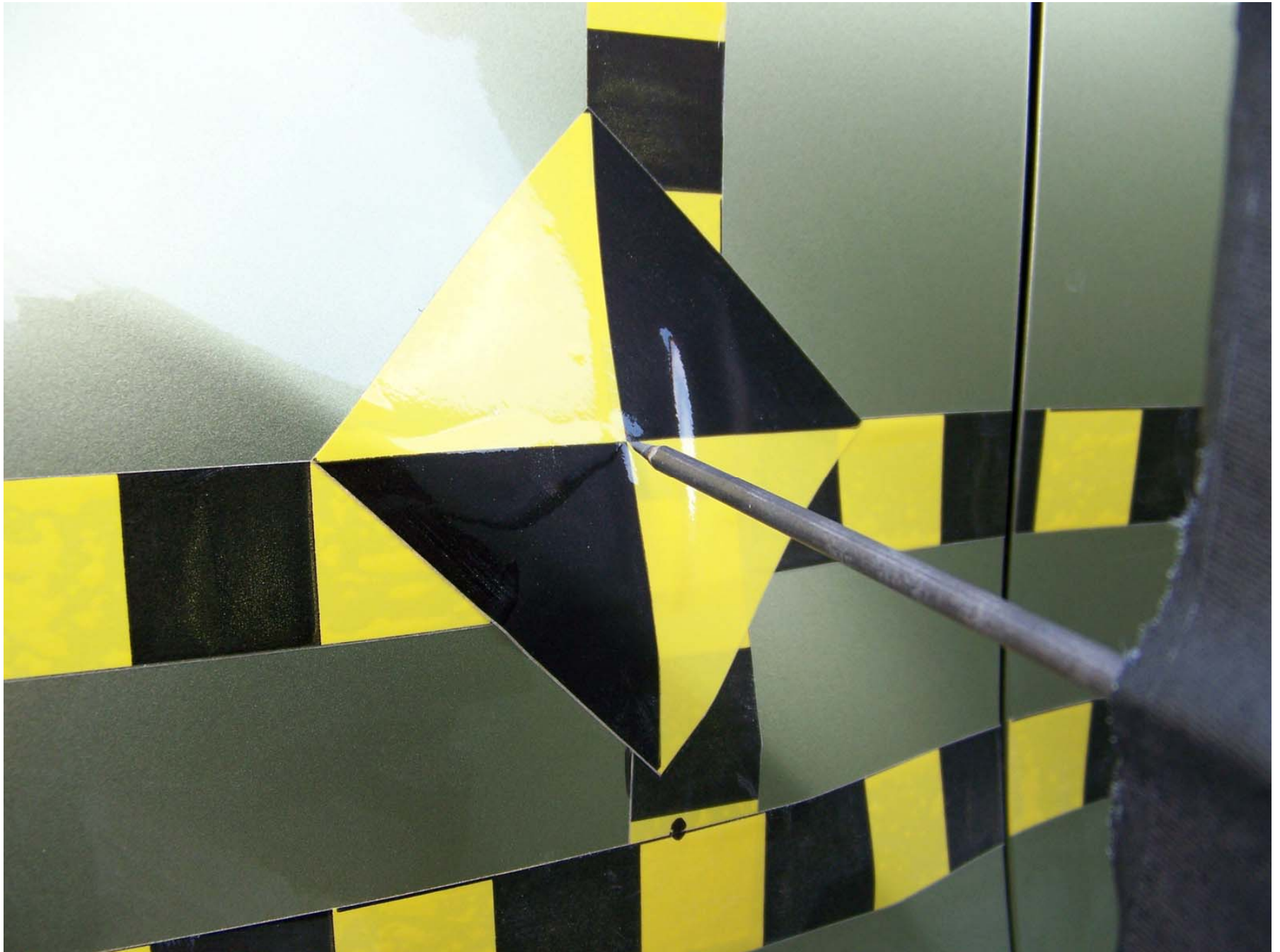
Figure A-19: Pre-Test Close-Up View of Impact Point Target
