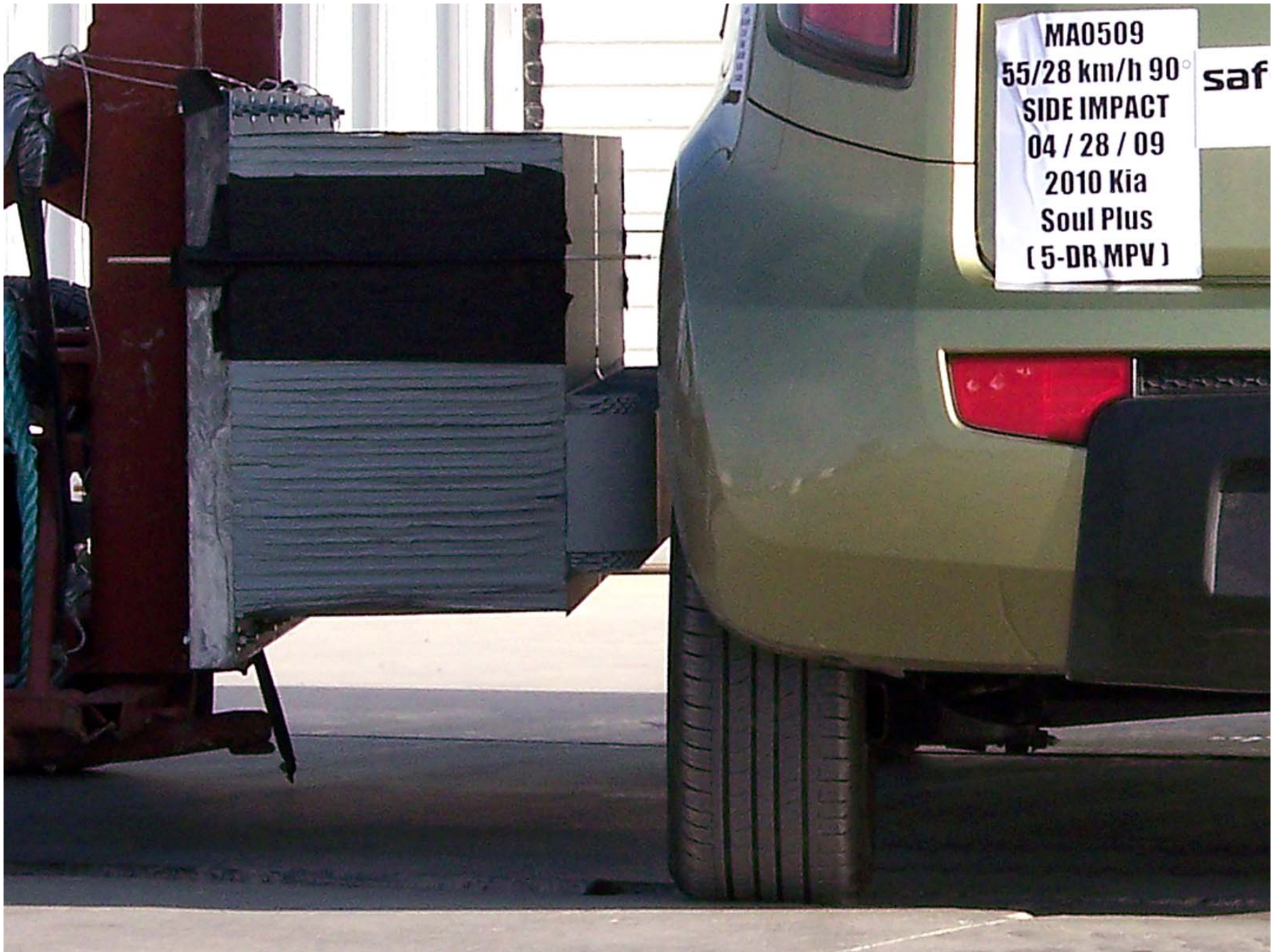
Figure A-18: Pre-Test Right Side View of MDB Positioned Against Test Vehicle
