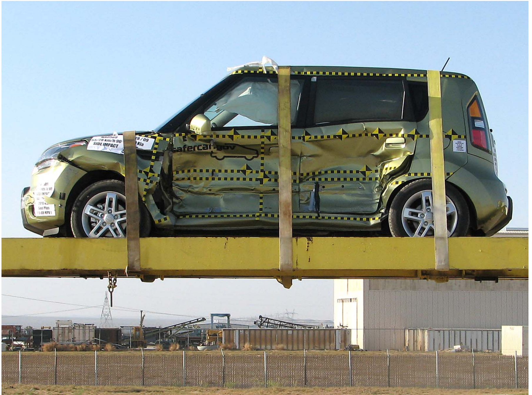
Figure A-64: FMVSS 301/305 Rollover 0°
