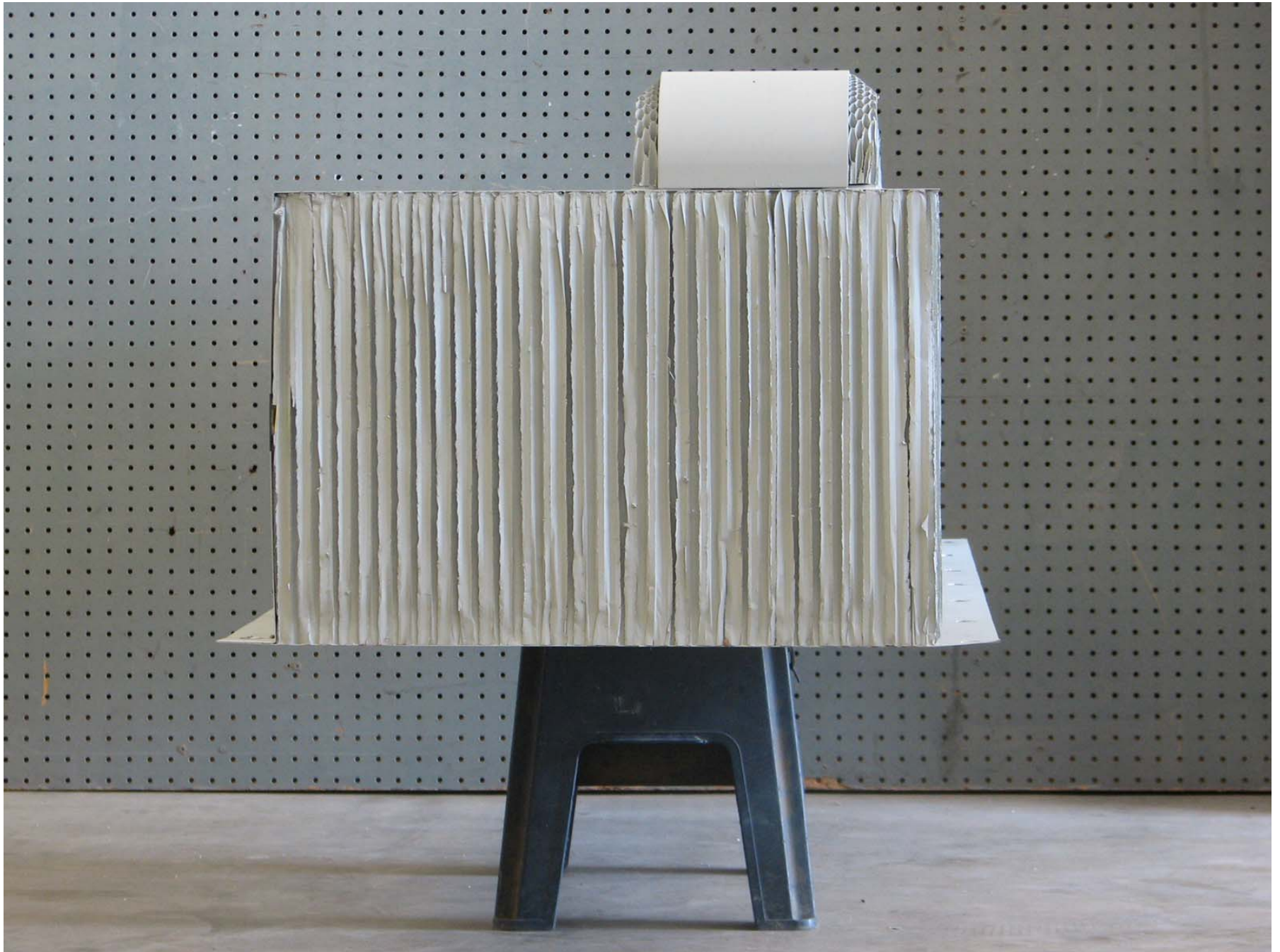
Figure A-61: Pre-Test Right Side View of MDB Impactor Face
