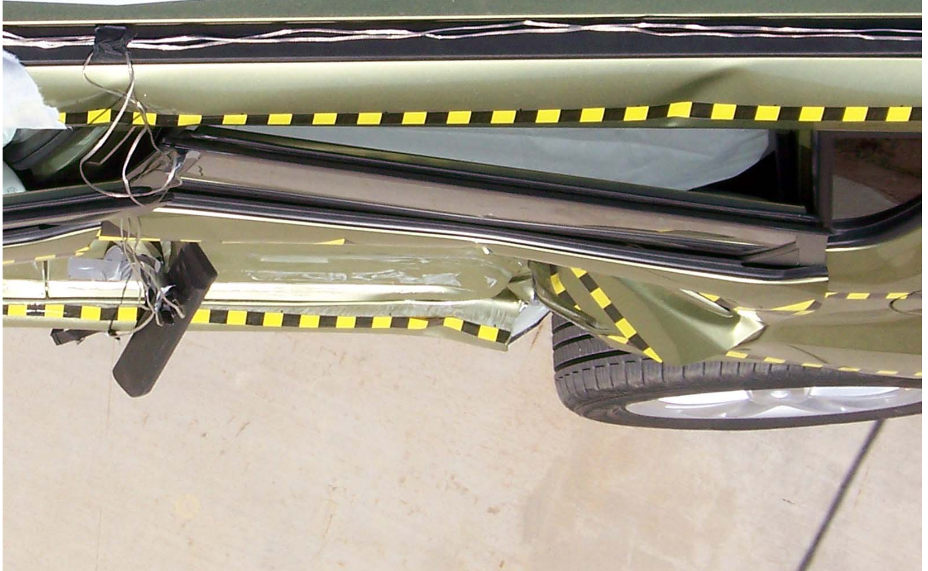
Figure A-46: Post-Test Passenger Dummy and Door Clearance View
