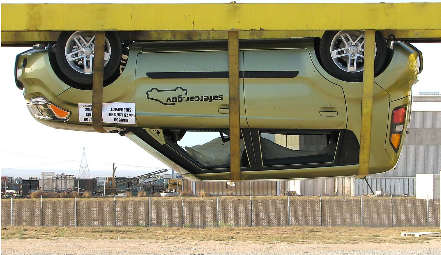
Figure A-66: FMVSS 301/305 Rollover 180°
