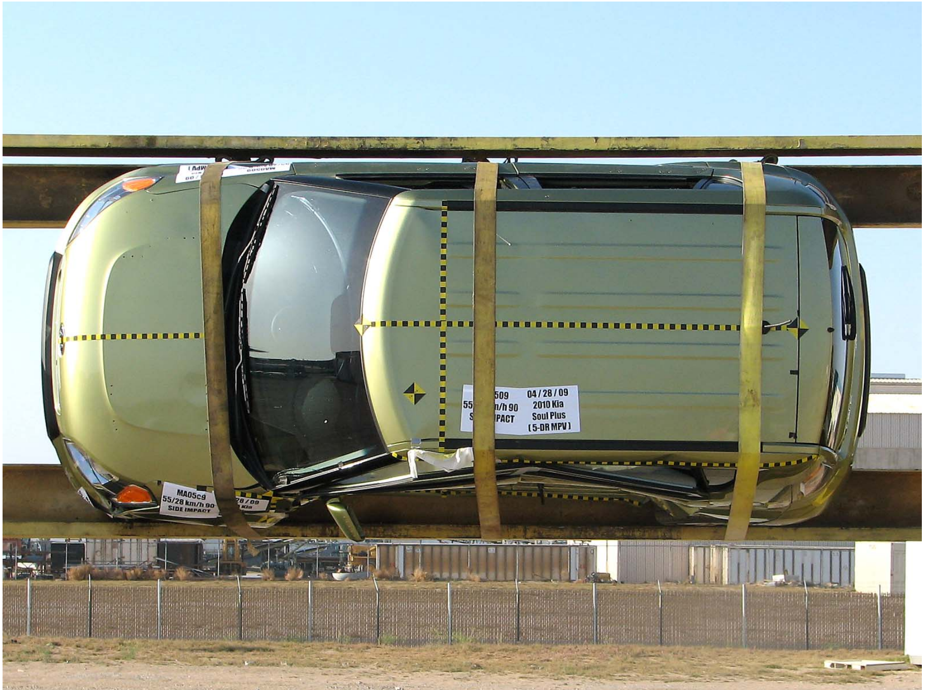
Figure A-65: FMVSS 301/305 Rollover 90°
