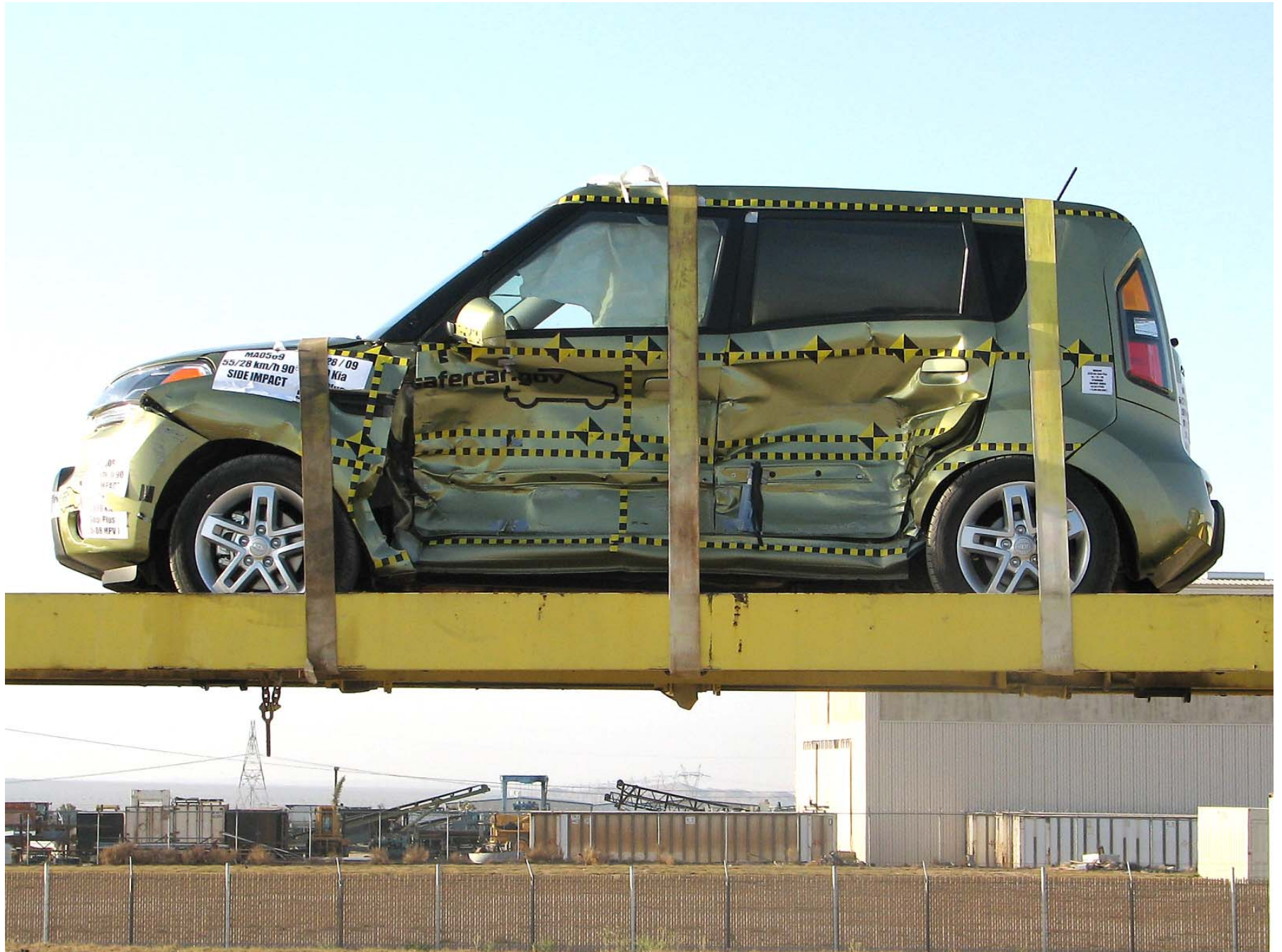
Figure A-68: FMVSS 301/305 Rollover 360°
