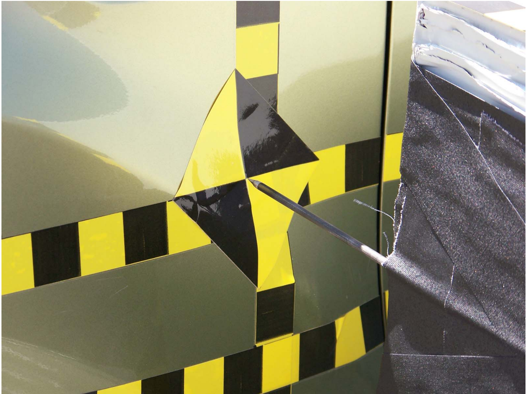
Figure A-25: Pre-Test Left Impact Point
