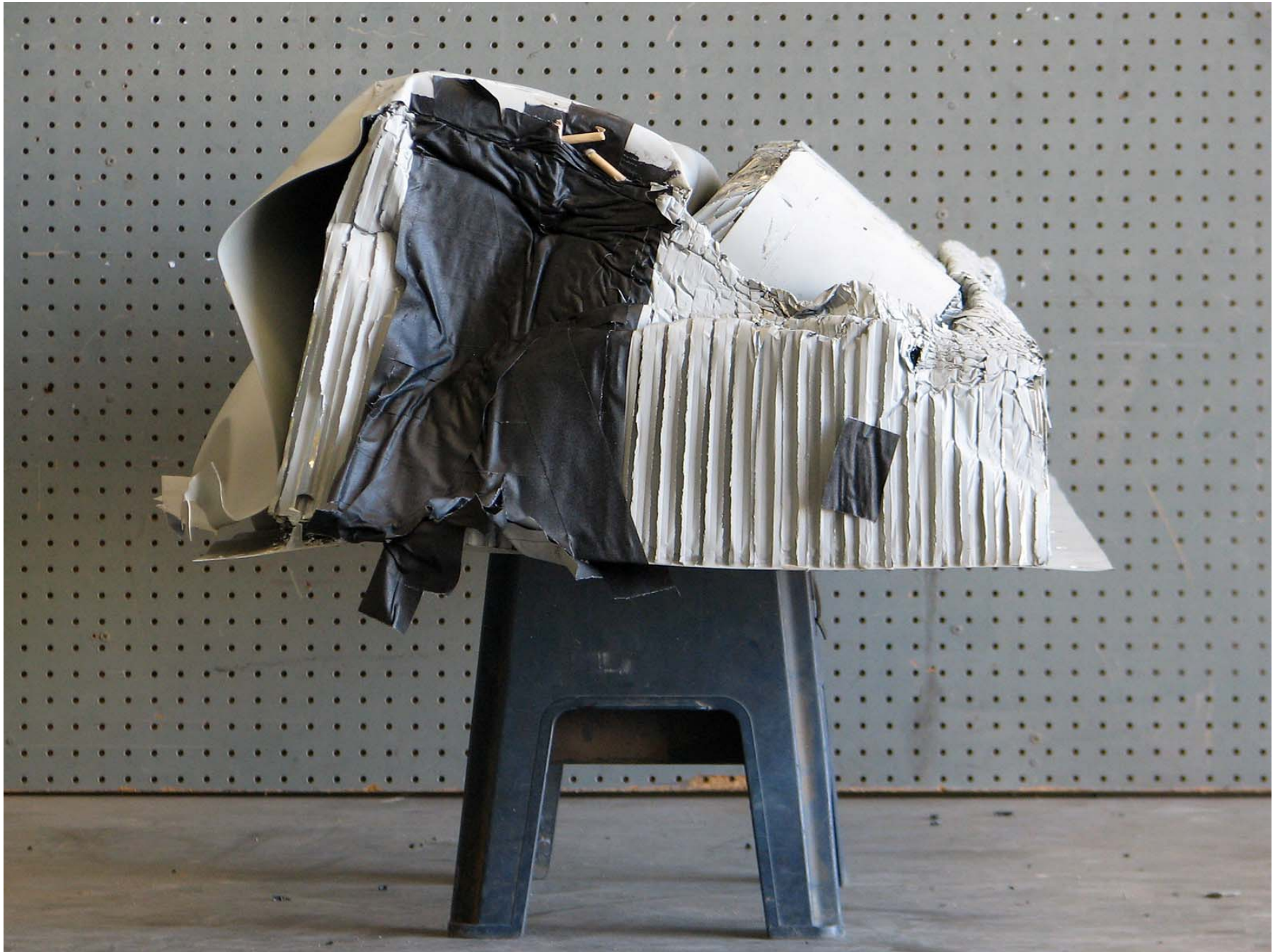
Figure A-60: Post-Test Right Side View of MDB Impactor Face
