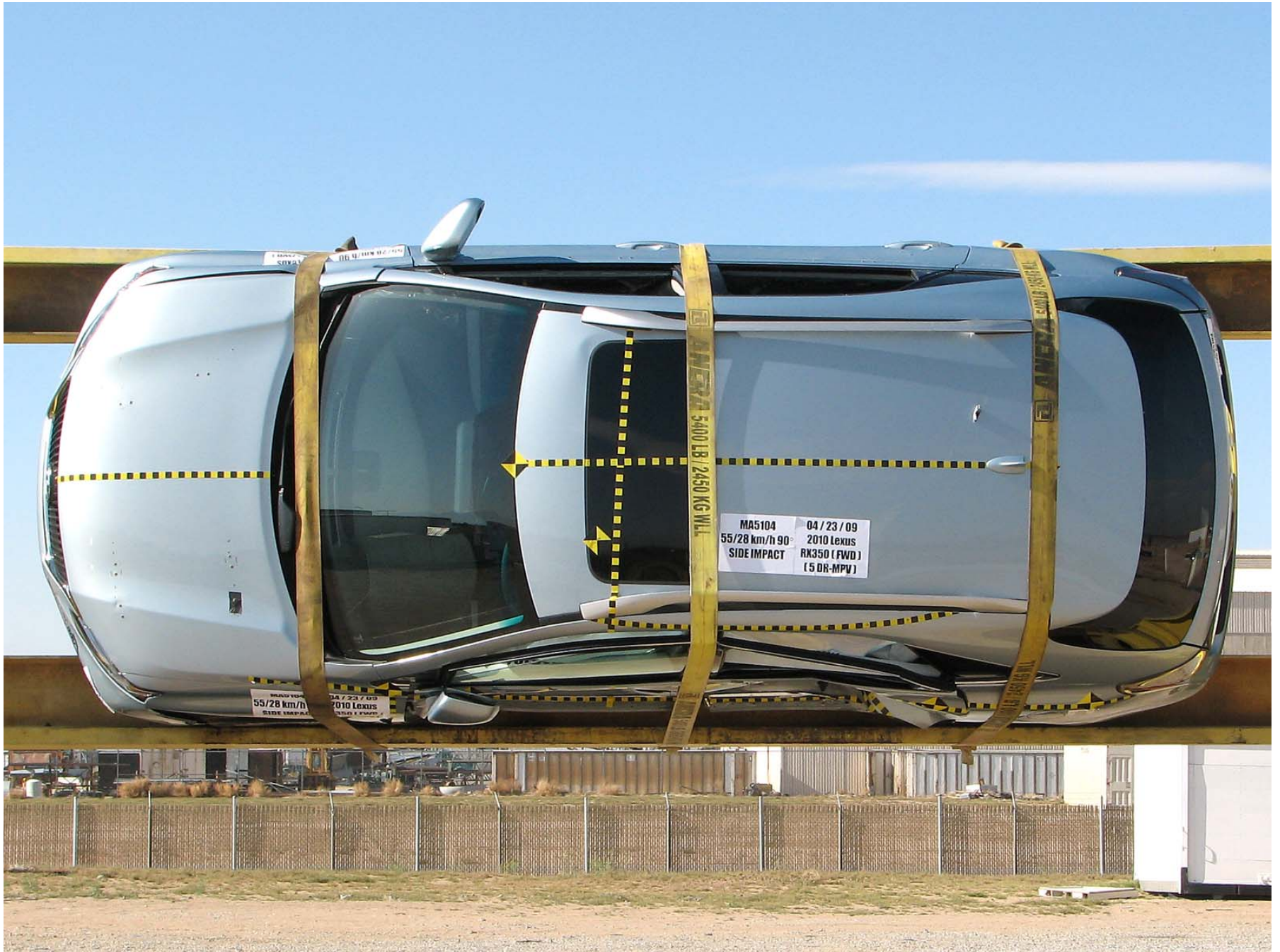
Figure A-63: FMVSS 301 / 305 Rollover 90°
