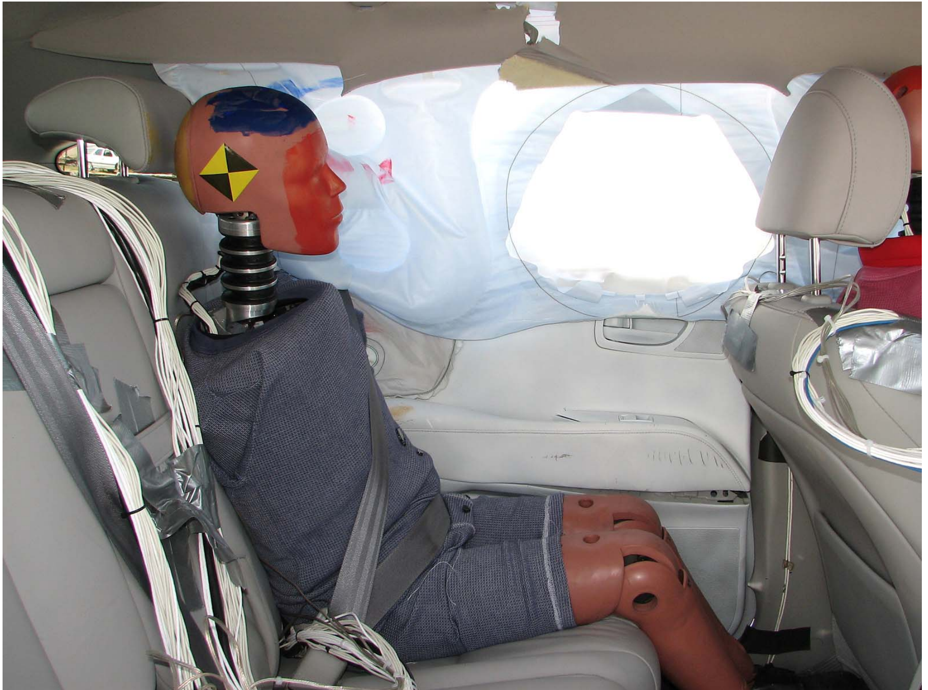
Figure A-46: Post-Test Right Side View of Rear Seat of Occupant Compartment (Through Window with Dummy)
