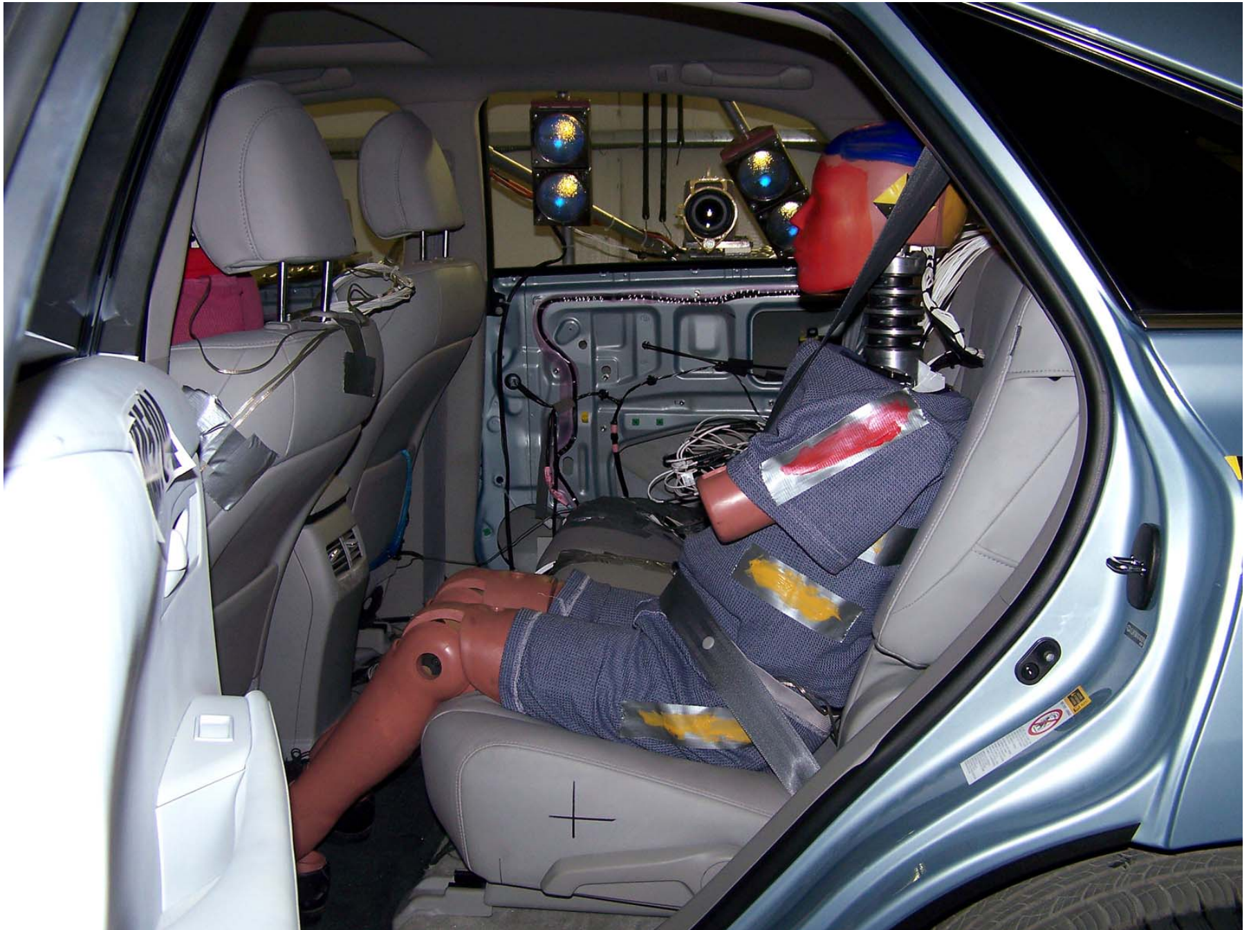
Figure A-39: Pre-Test Left Side View of Passenger Dummy Showing Belt, Chalking, and Contact Switches
