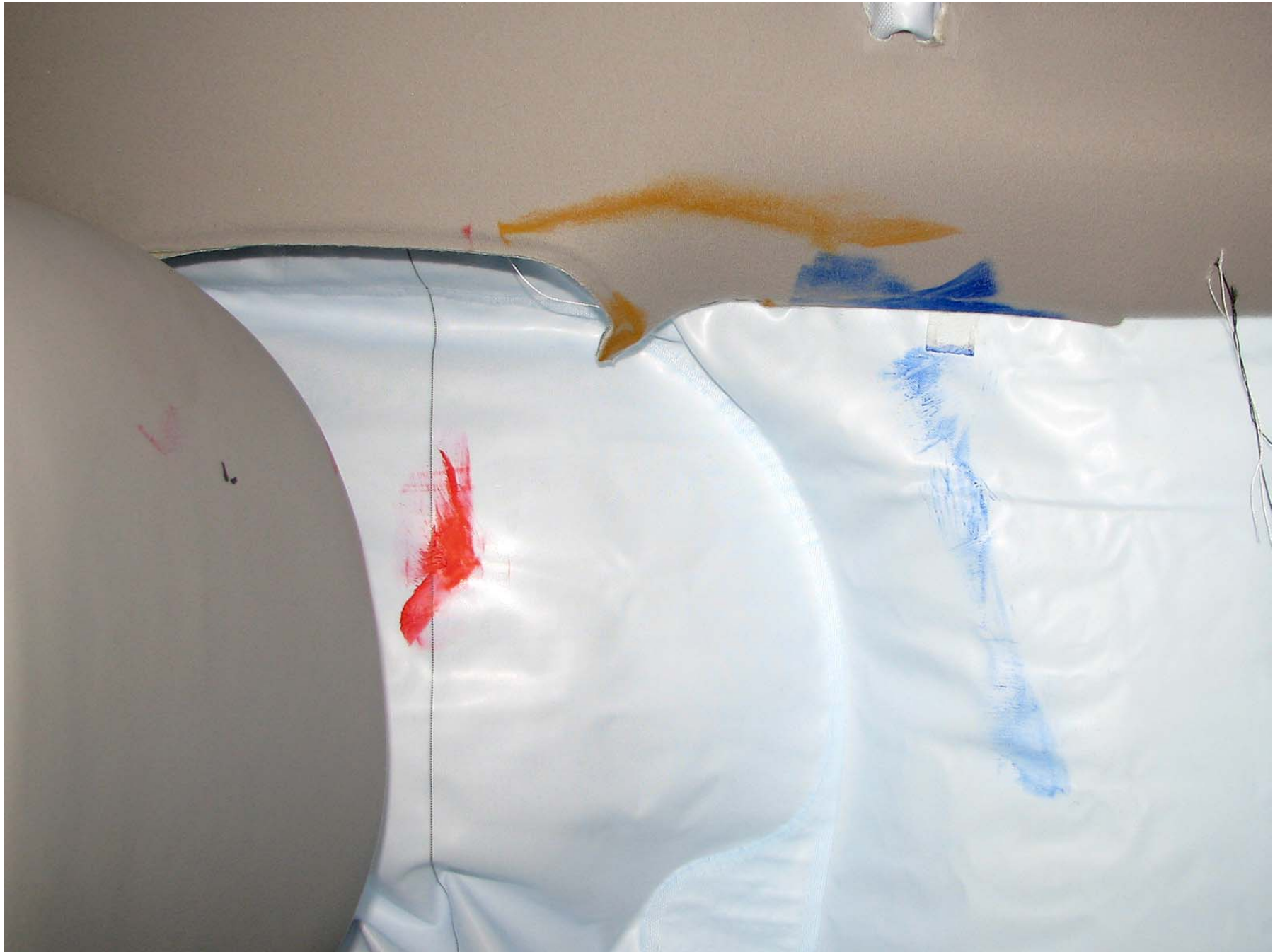
Figure A-37: Post-Test Driver Dummy Head Contact View
