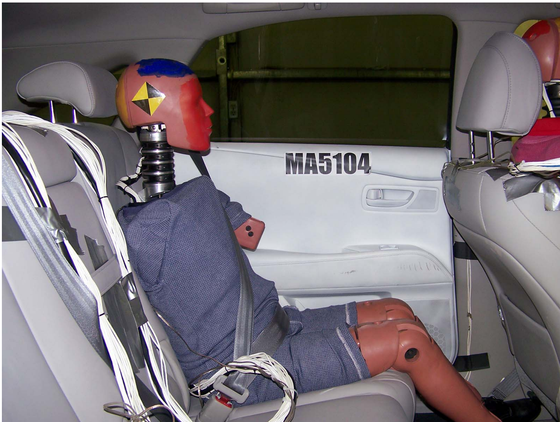
Figure A-45: Pre-Test Right Side View of Rear Seat of Occupant Compartment (Through Window with Dummy)
