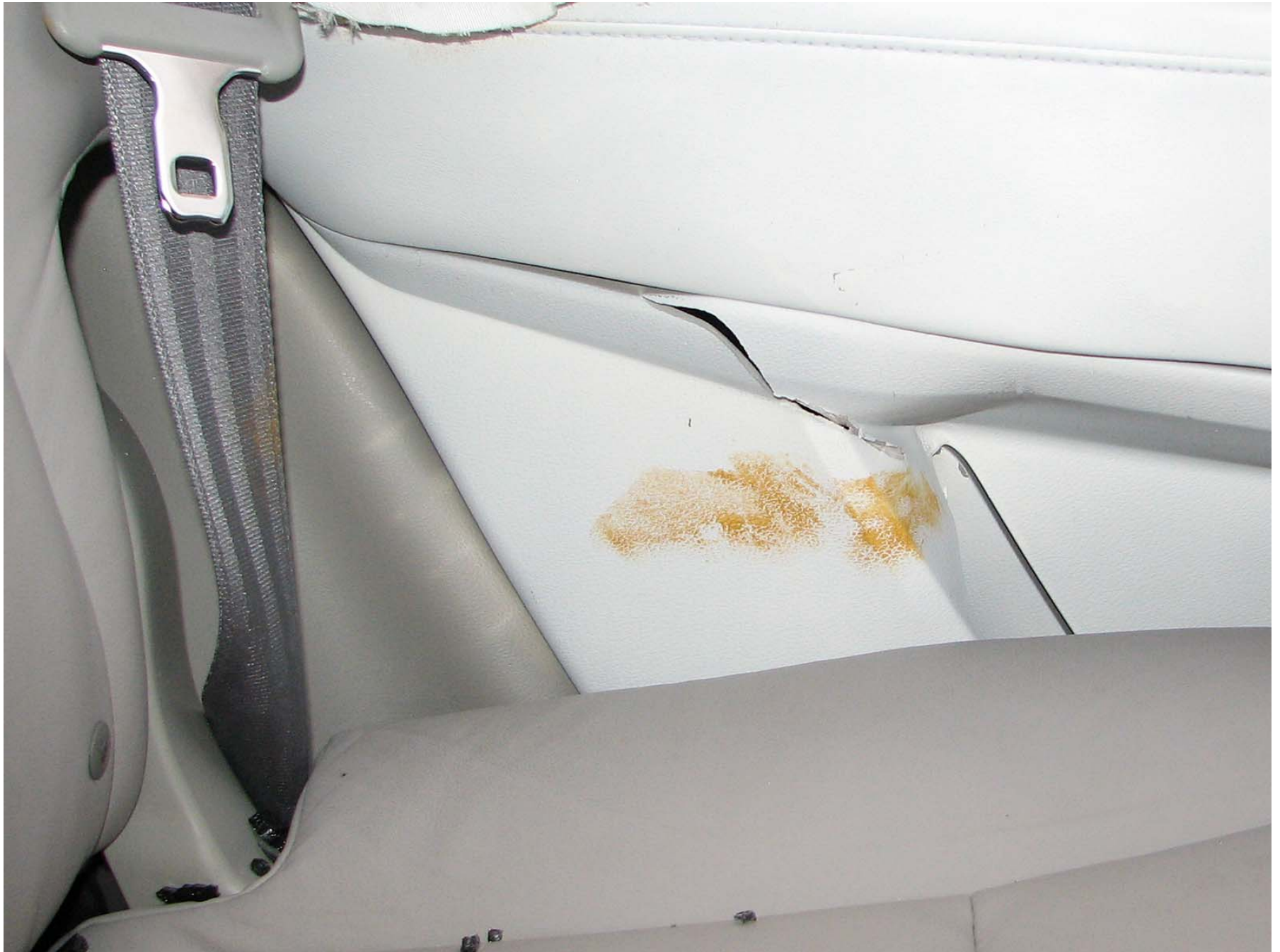
Figure A-50: Post-Test Passenger Dummy Door Contact View
