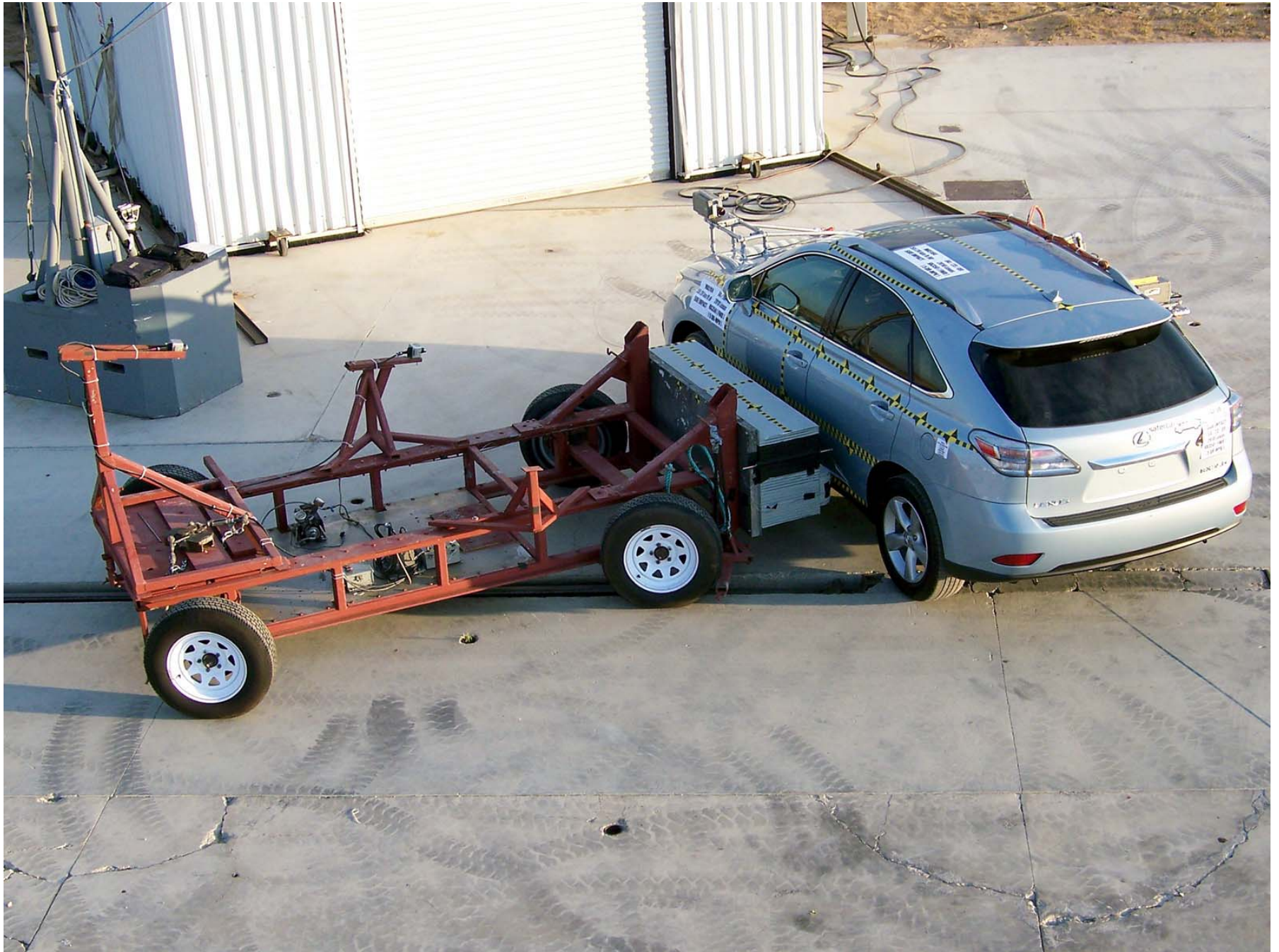
Figure A-15: Pre-Test Overhead View of MDB Positioned Against Impact Side of Test Vehicle at Impact Location
