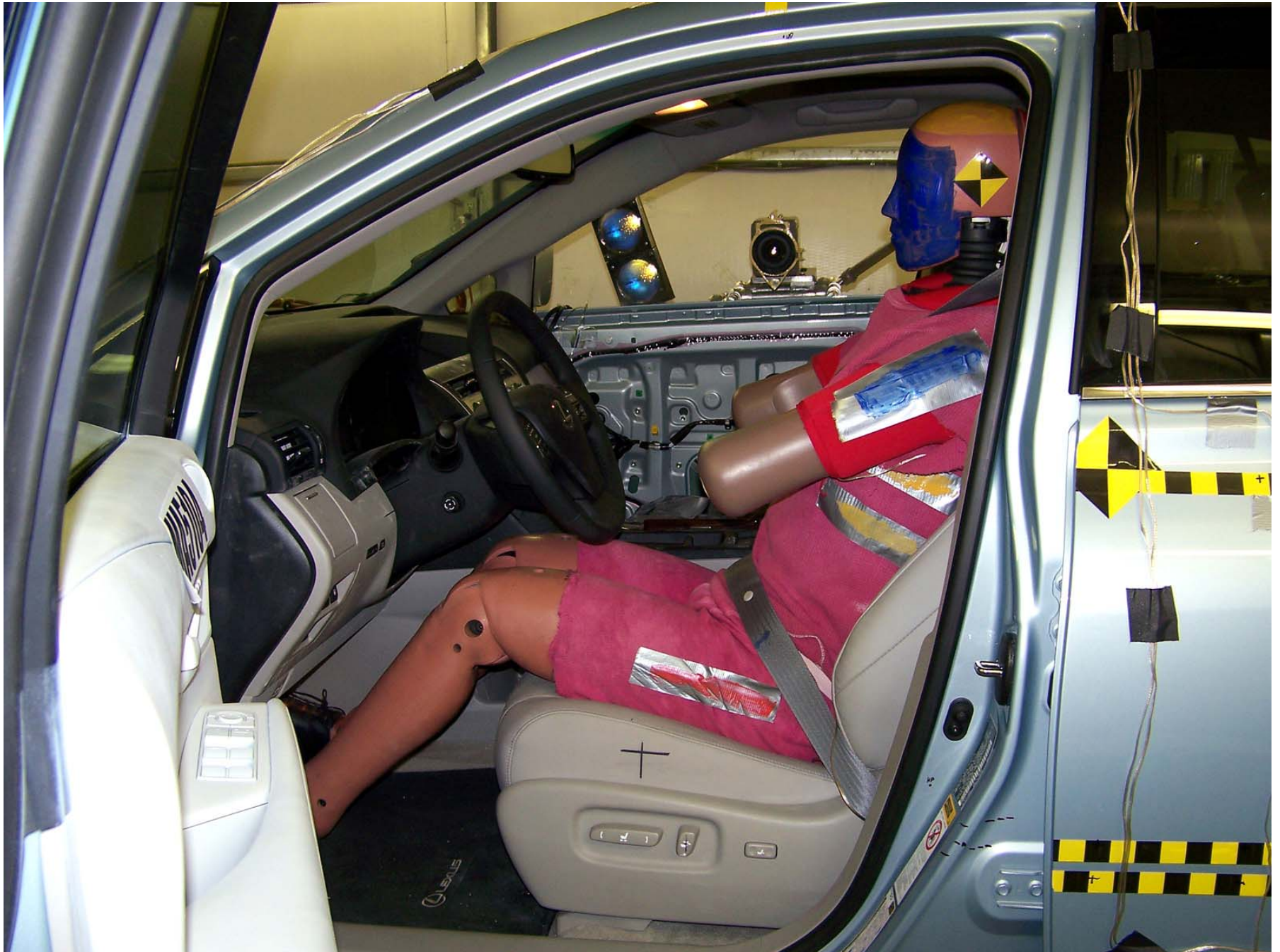
Figure A-27: Pre-Test Left Side View of Driver Dummy Showing Belt, Chalking, and Contact Switches
