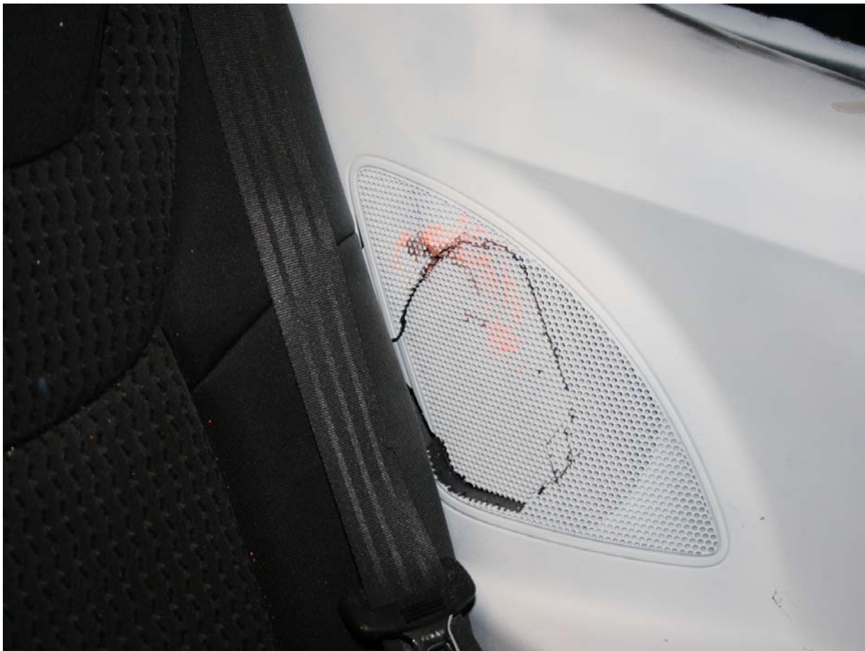
Post-Test Passenger Dummy Door Contact View
