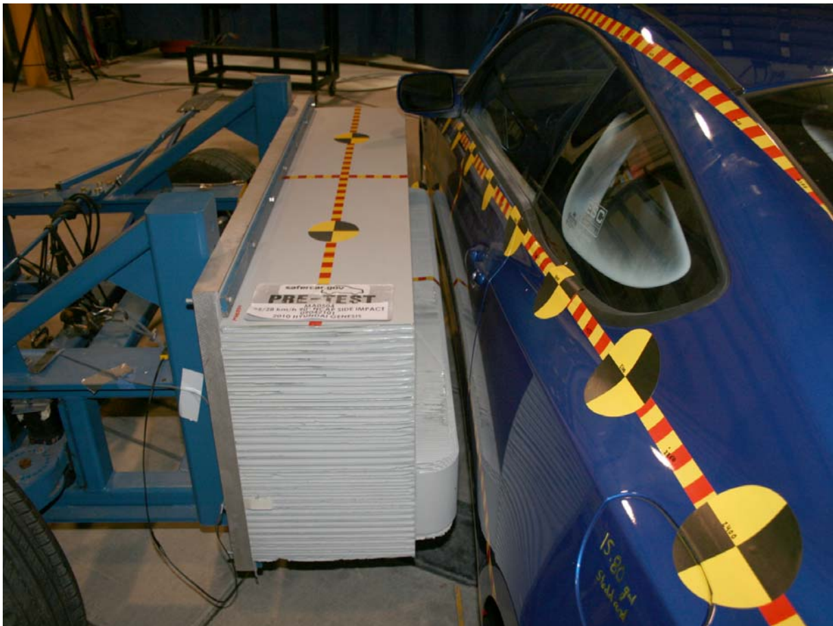
Pre-Test Right Side View of MDB Positioned Against the Side of the Test Vehicle at the Ideal Impact Point
