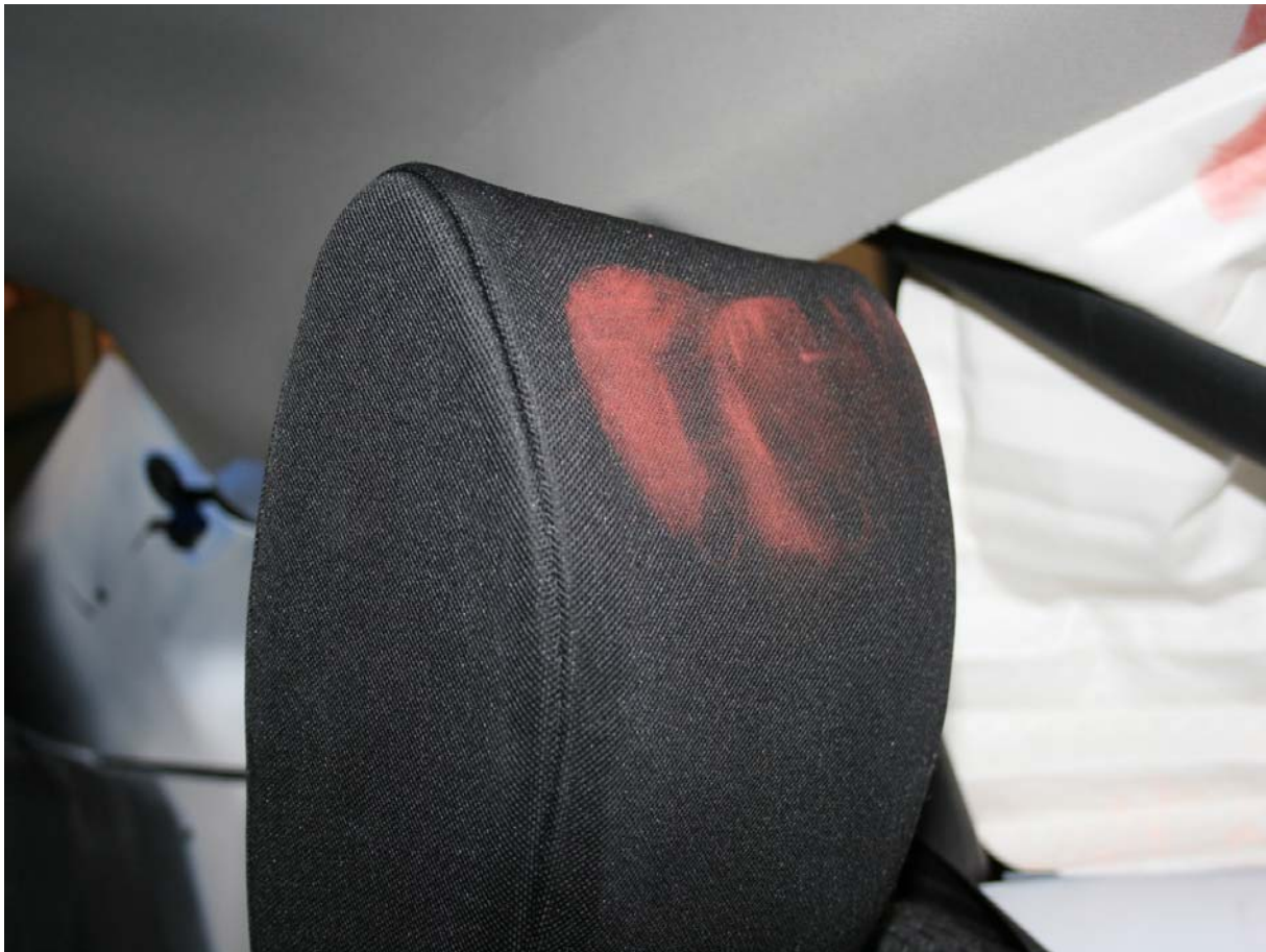
Post-Test Driver Dummy Head Contact View 2
