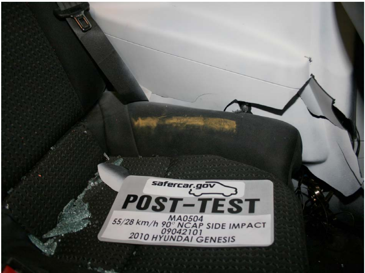
Post-Test Passenger Dummy Door Contact View 2
