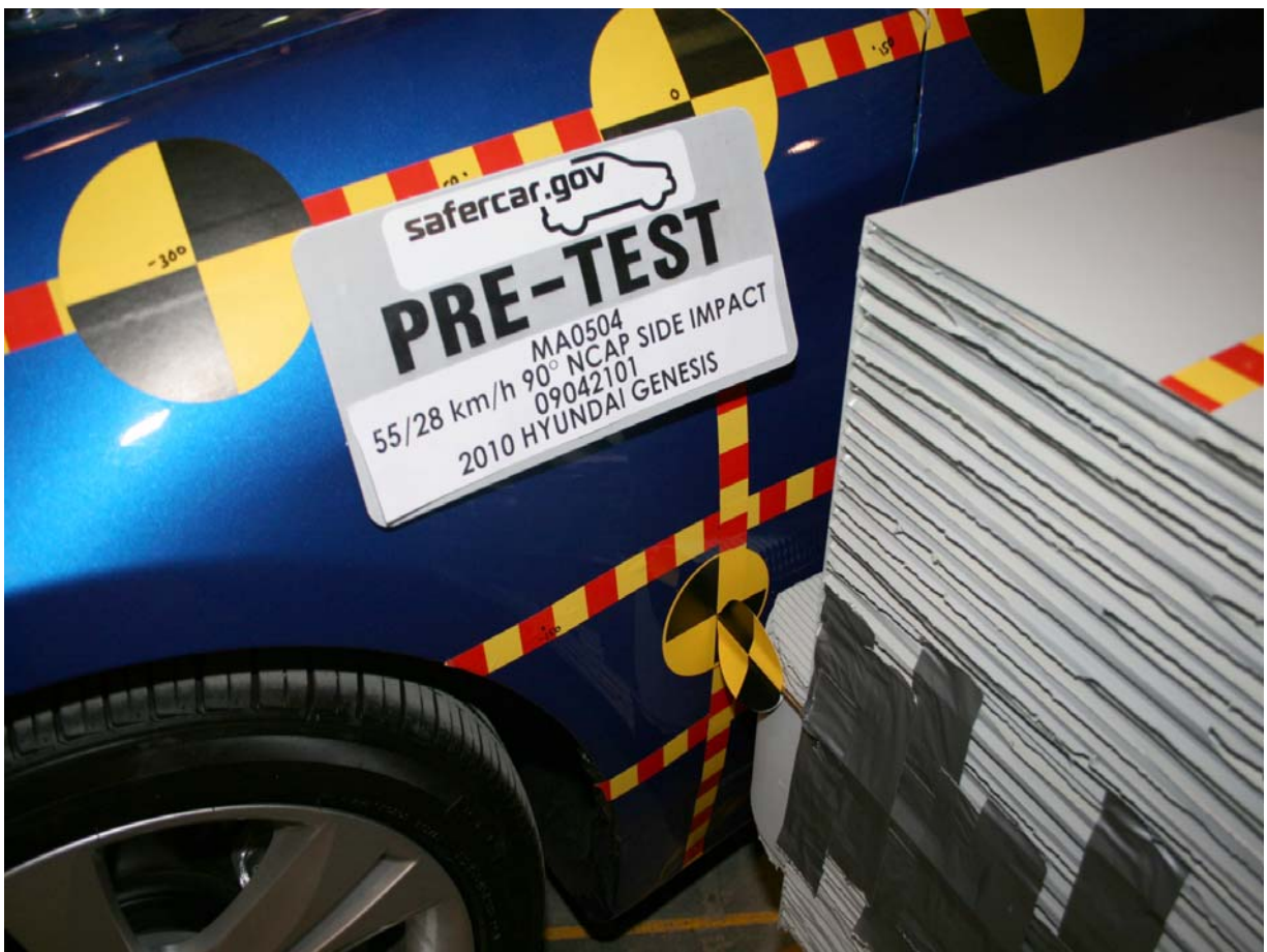
Pre-Test Close-Up View of Impact Point Target
