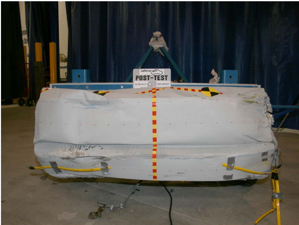
Post-Test Front View of MDB Impactor Face
