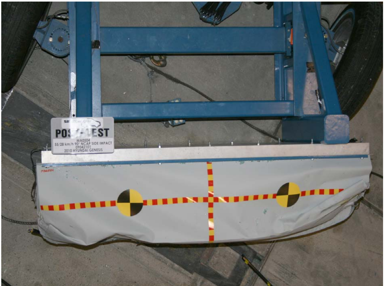
Post-Test Top View of MDB Impactor Face
