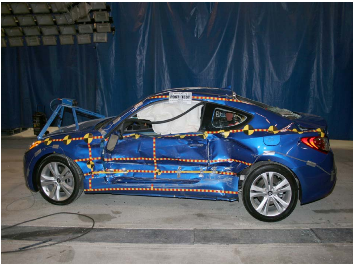
Post-Test Left Side View of Test Vehicle
