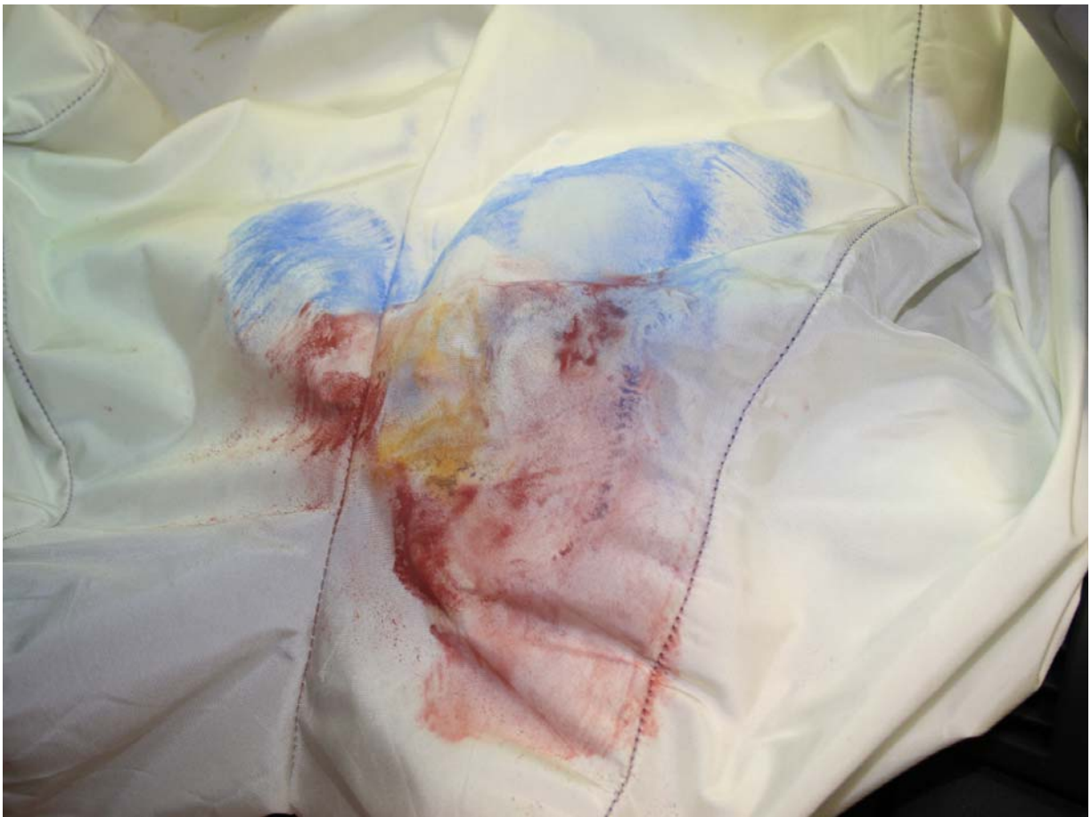
Post-Test Passenger Dummy Airbag Contact
