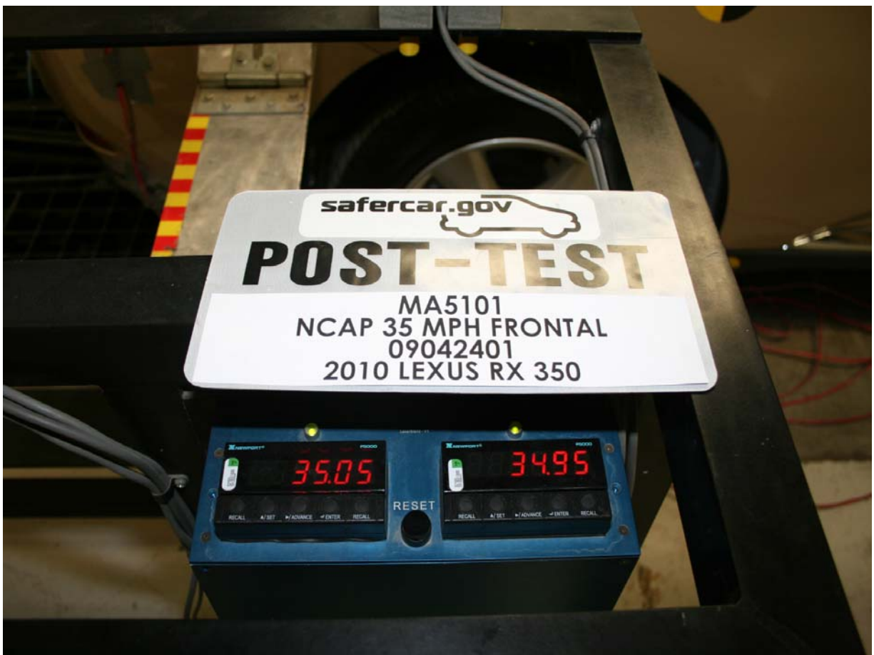
Post-Test Speed Trap Read-Out
