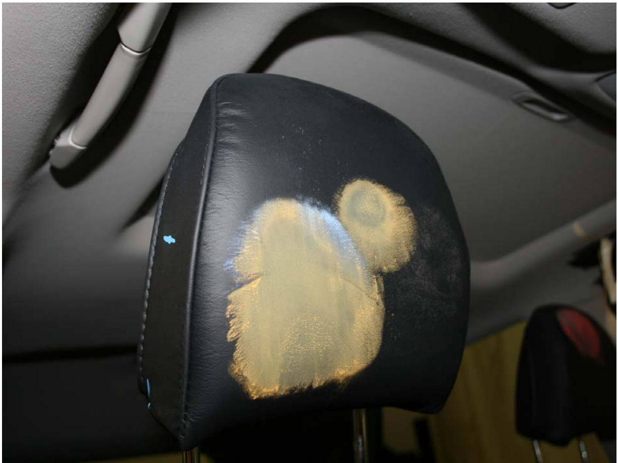
Post-Test Passenger Dummy Head Contact
