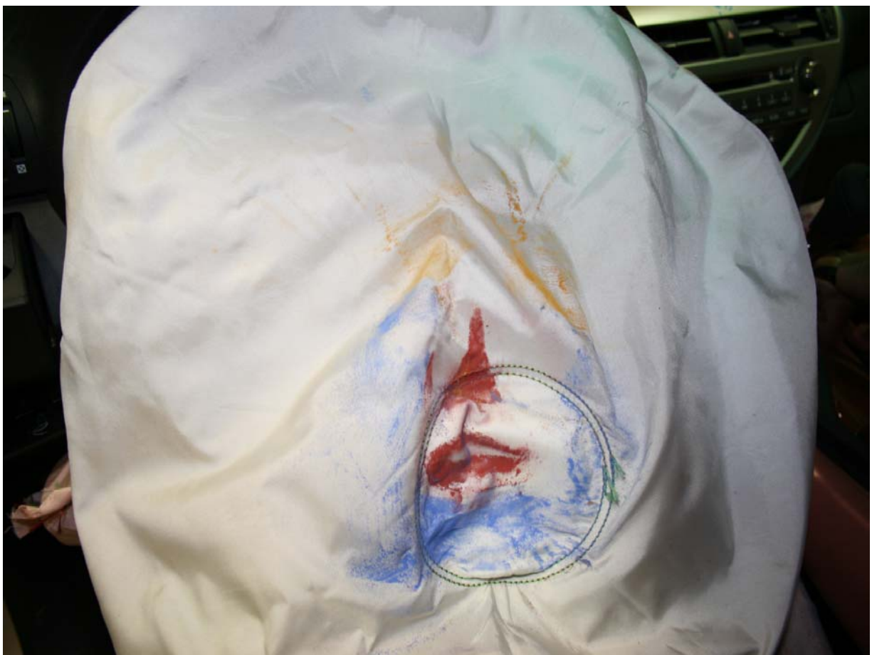
Post-Test Driver Dummy Airbag Contact
