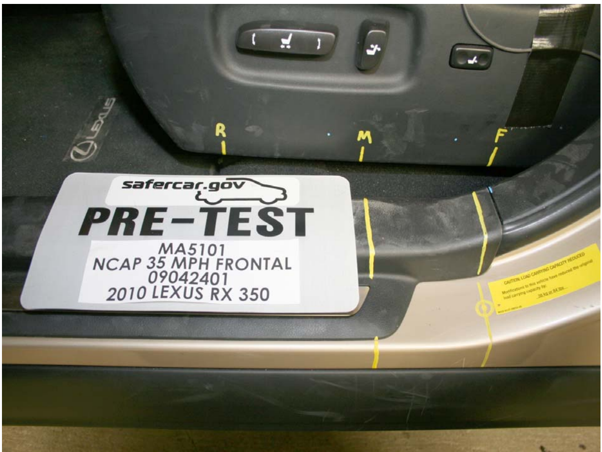
Pre-Test Driver's Seat Fore-Aft Markings
