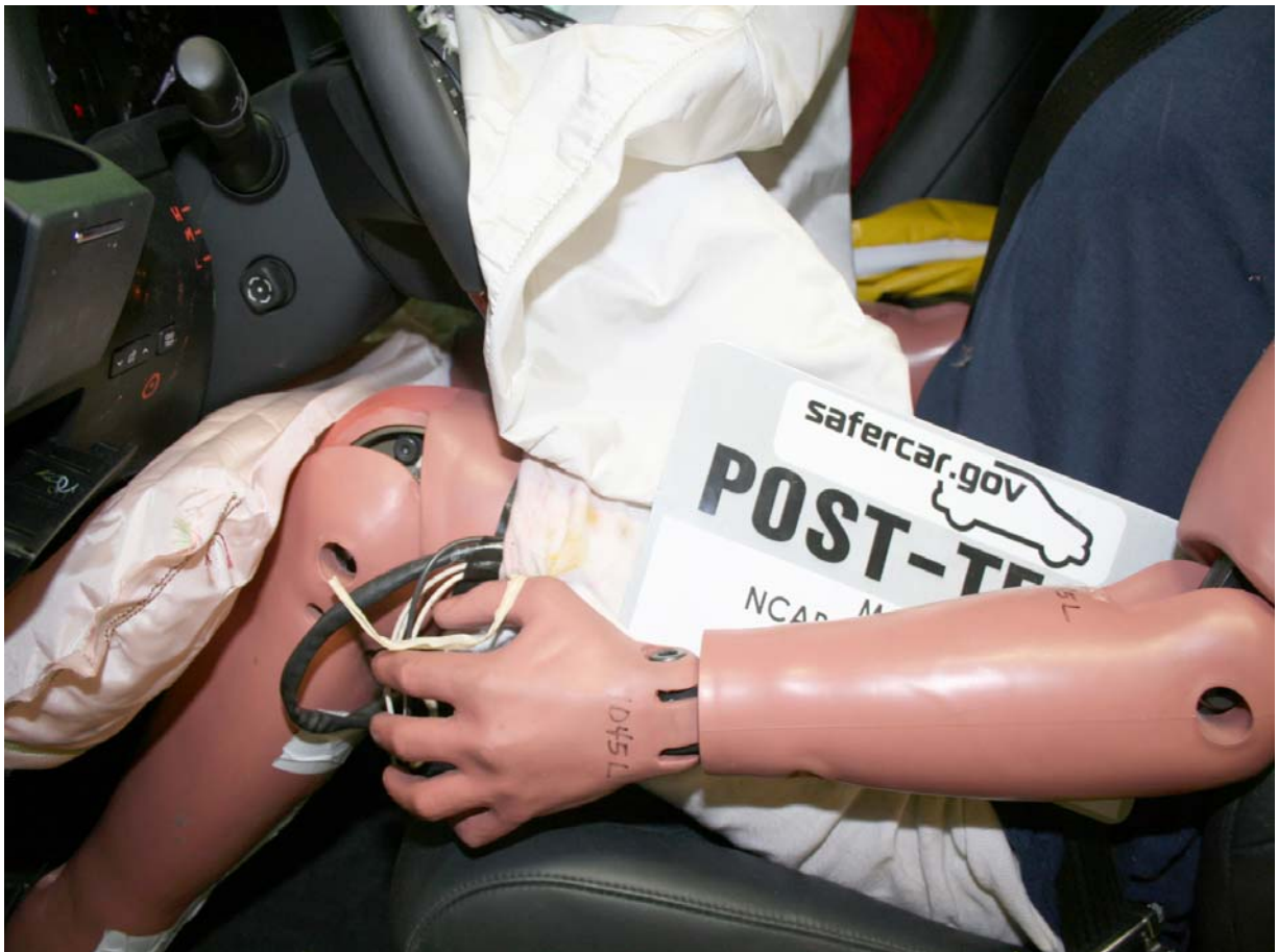
Post-Test Driver's Side Knee Bolster
