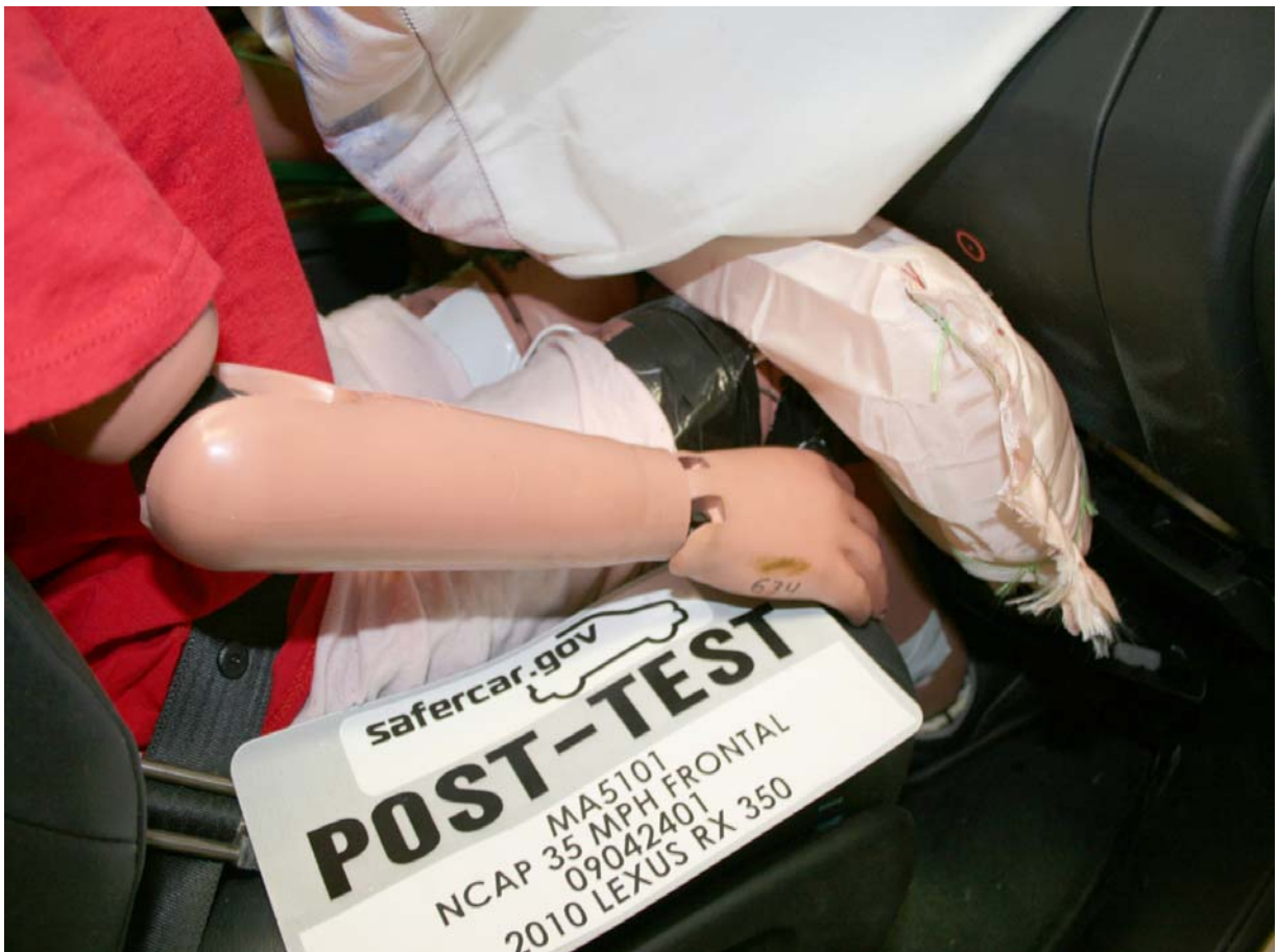
Post-Test Passenger's Side Knee Bolster
