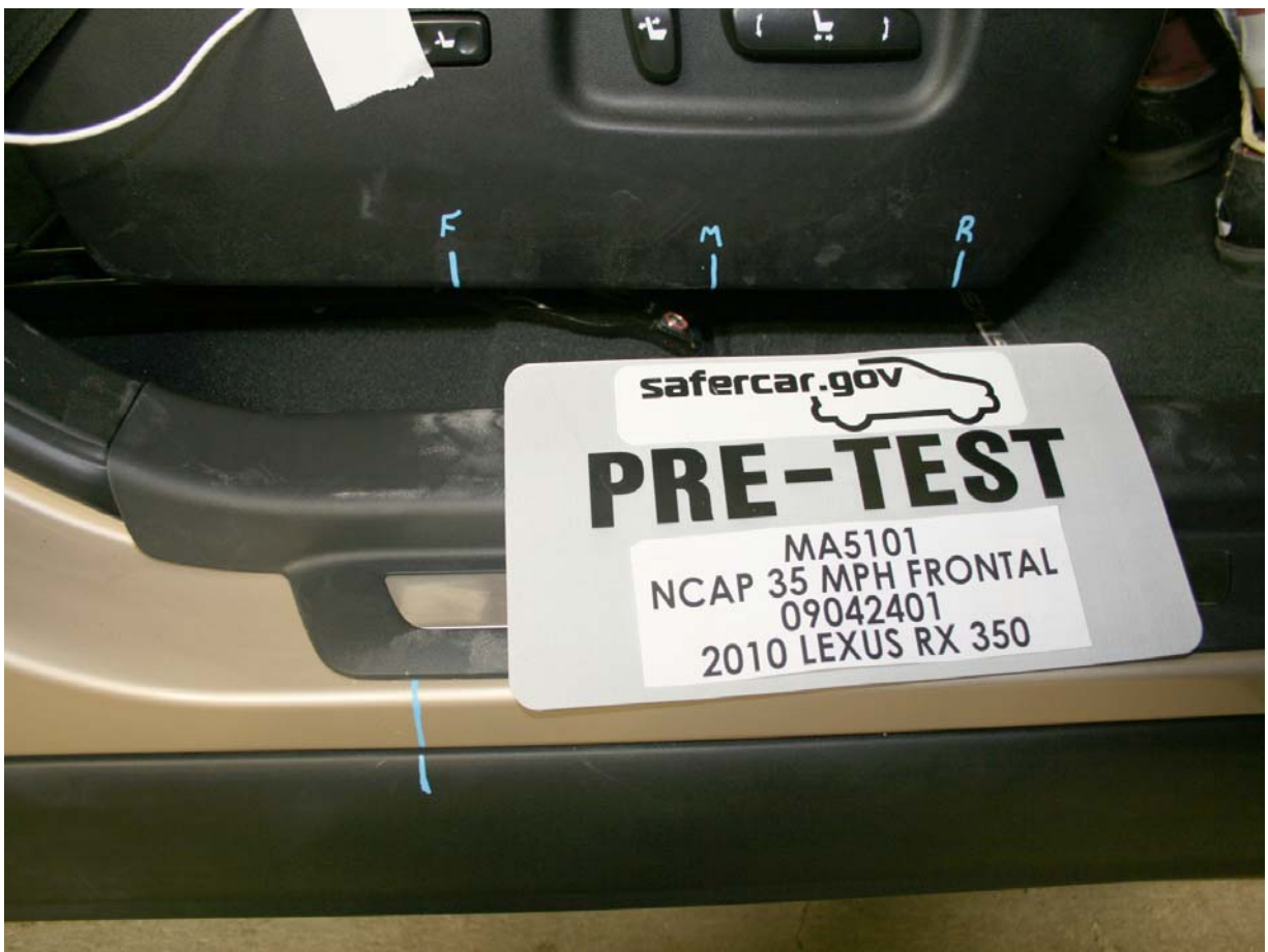
Pre-Test Passenger's Seat Fore-Aft Markings
