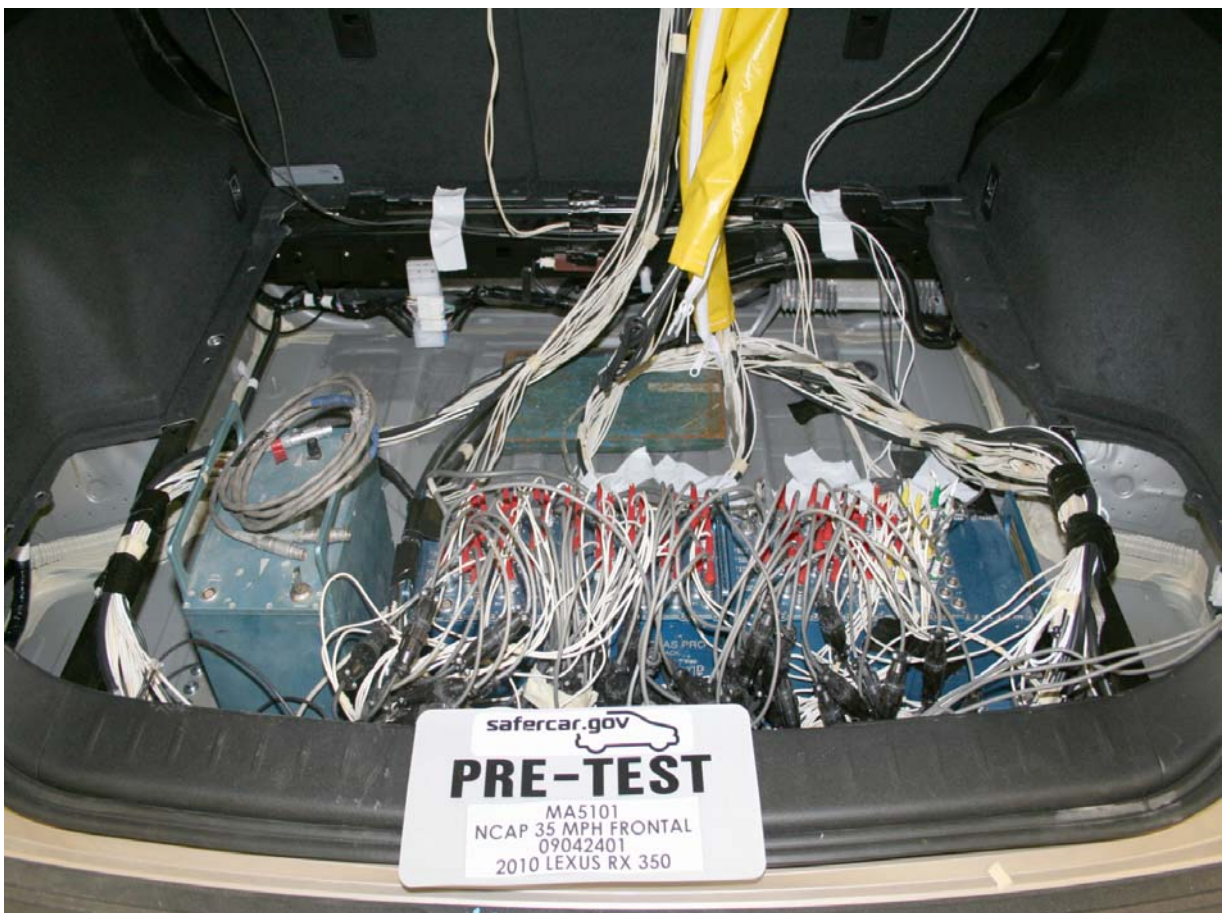
Ballast Installed in Vehicle
