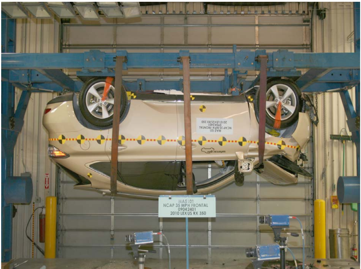
Vehicle at 180 Degrees on Static Rollover Device
