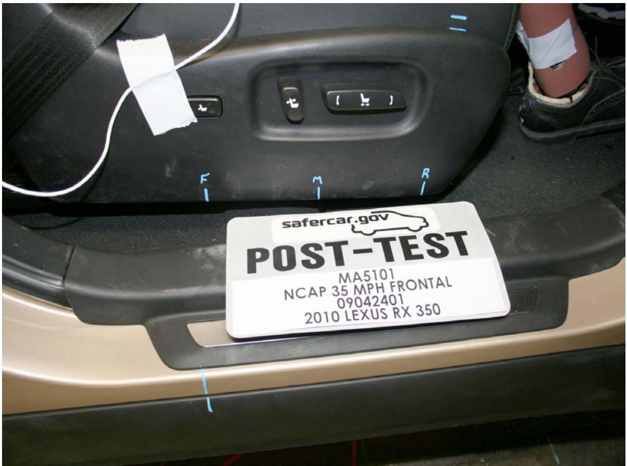
Post-Test Passenger's Seat Fore-Aft Markings
