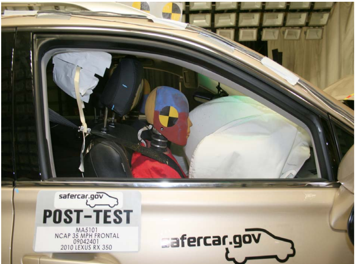
Post-Test Passenger Dummy Window View
