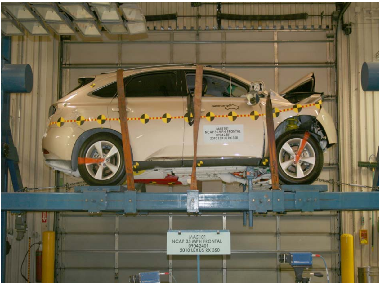
Vehicle at 360 Degrees on Static Rollover Device
