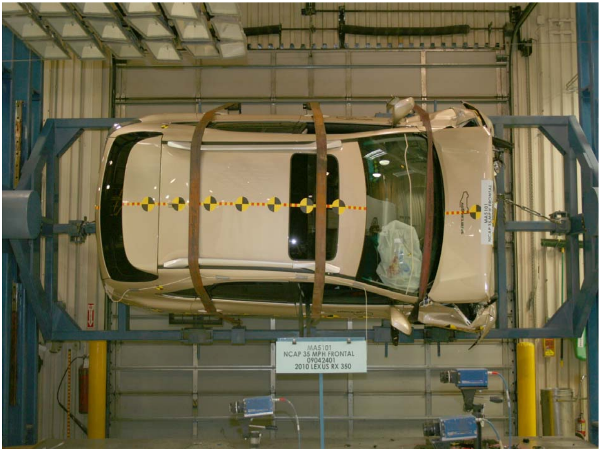
Vehicle at 270 Degrees on Static Rollover Device
