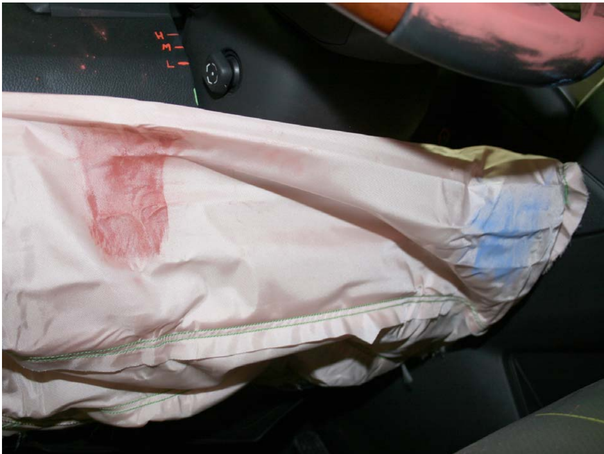
Post-Test Driver Dummy Knee Contact
