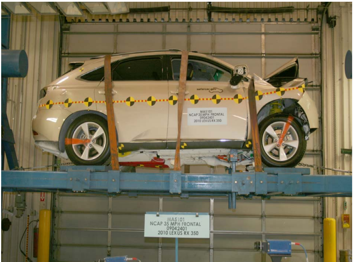
Vehicle at 0 Degrees on Static Rollover Device
