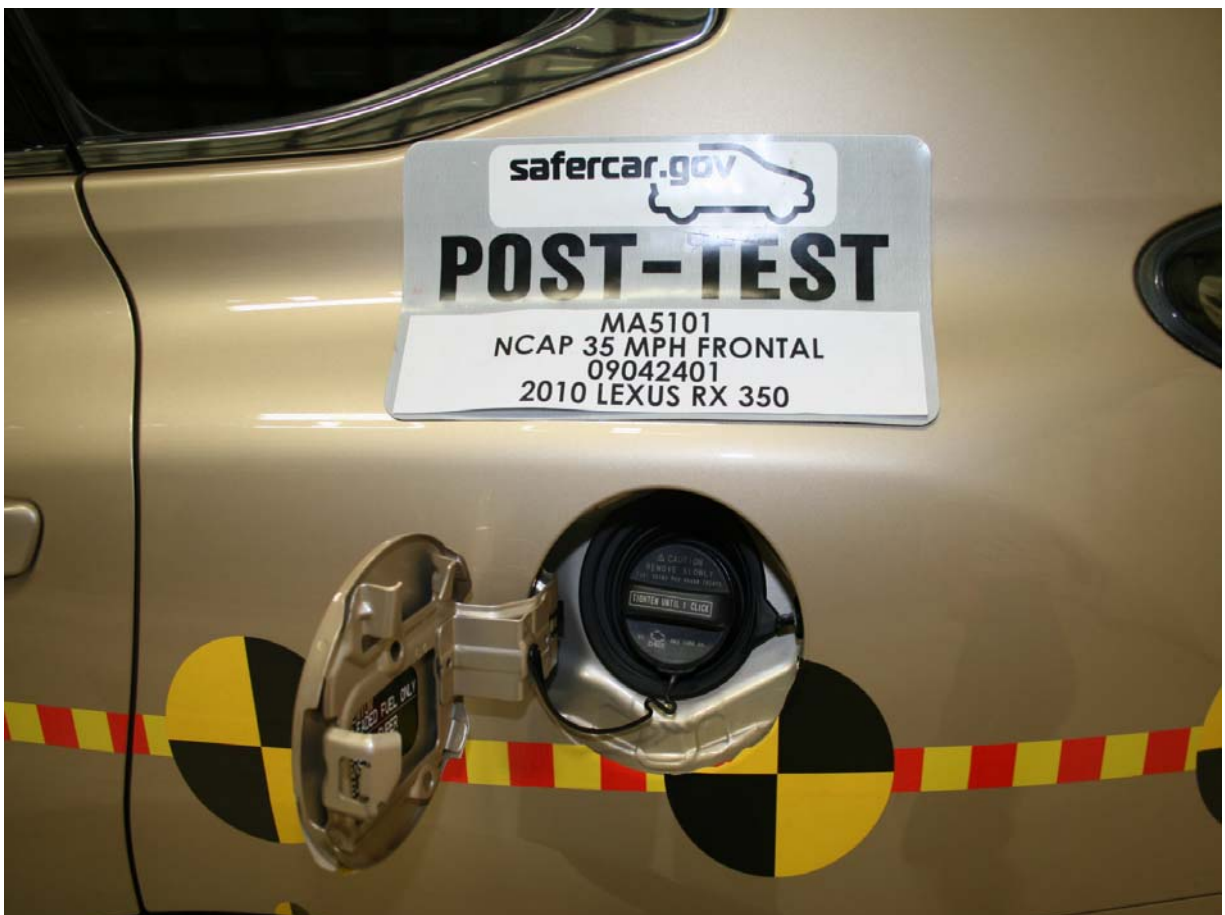
Post-Test Fuel Cap View
