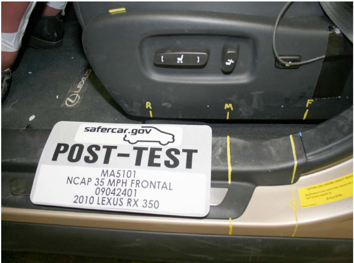
Post-Test Driver's Seat Fore-Aft Markings
