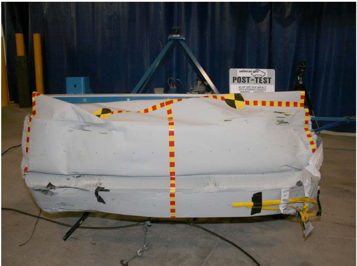
Post-Test Front View of Deformable Barrier
