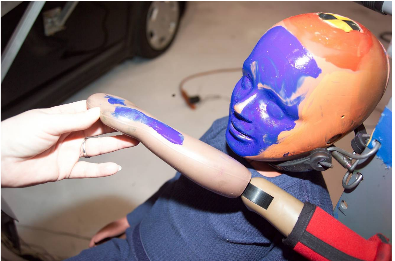
Figure A-95 Post-Test Right Rear Child Dummy Head Contact - View 3
