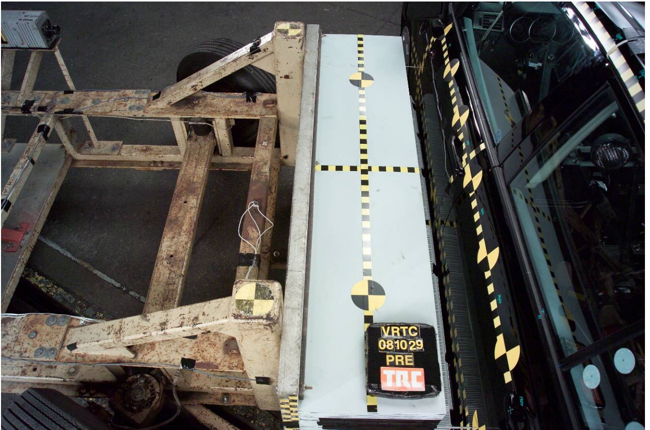
Figure A-45 Pre-Test MDB Alignment Overhead View
