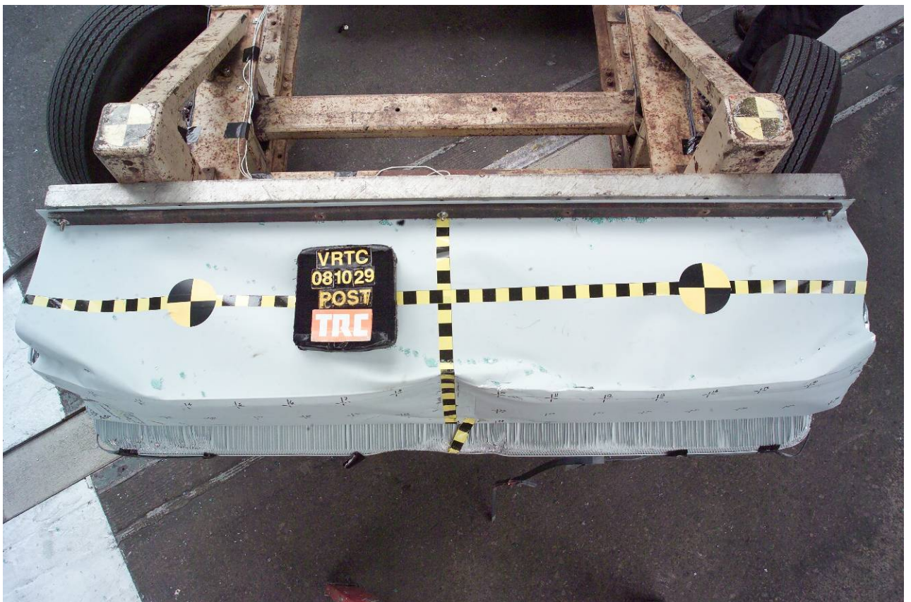
Figure A-30 Post-Test MDB Face Overhead View
