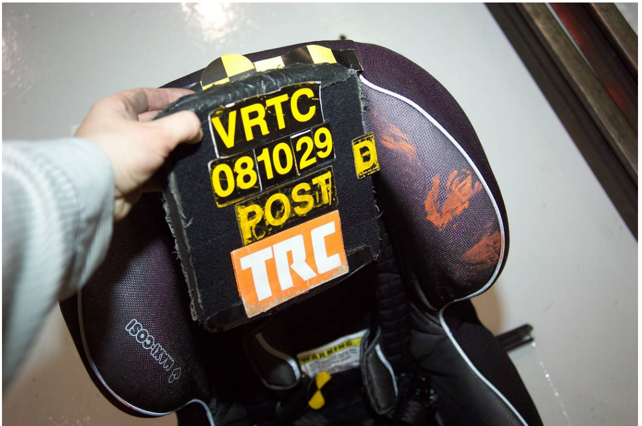
Figure A-88 Post-Test Left Rear Child Dummy Head Contact - View 1
