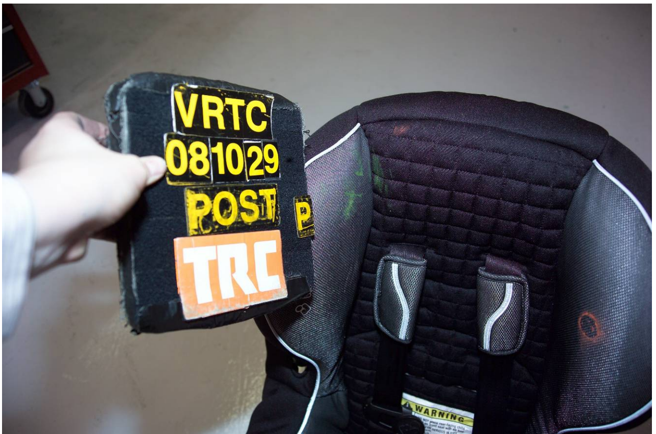
Figure A-94 Post-Test Right Rear Child Dummy Head Contact - View 2
