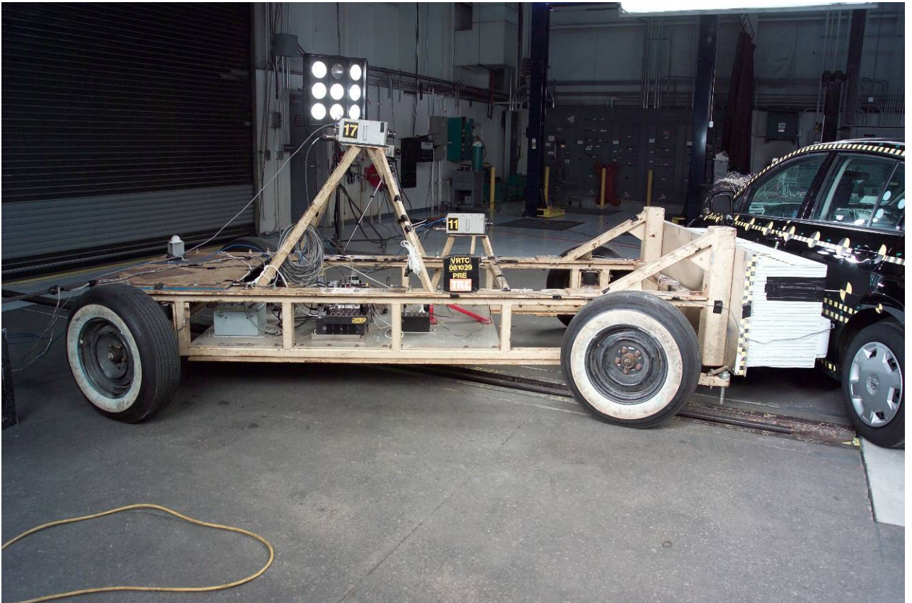
Figure A-43 Pre-Test MDB Right Side Overall View
