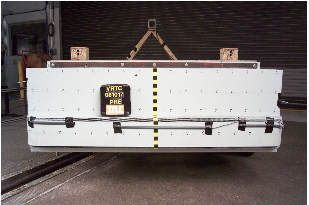
Figure A-23 Pre-Test MDB Face Front View
