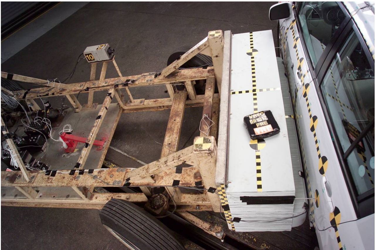
Figure A-45 Pre-Test MDB Alignment Overhead View
