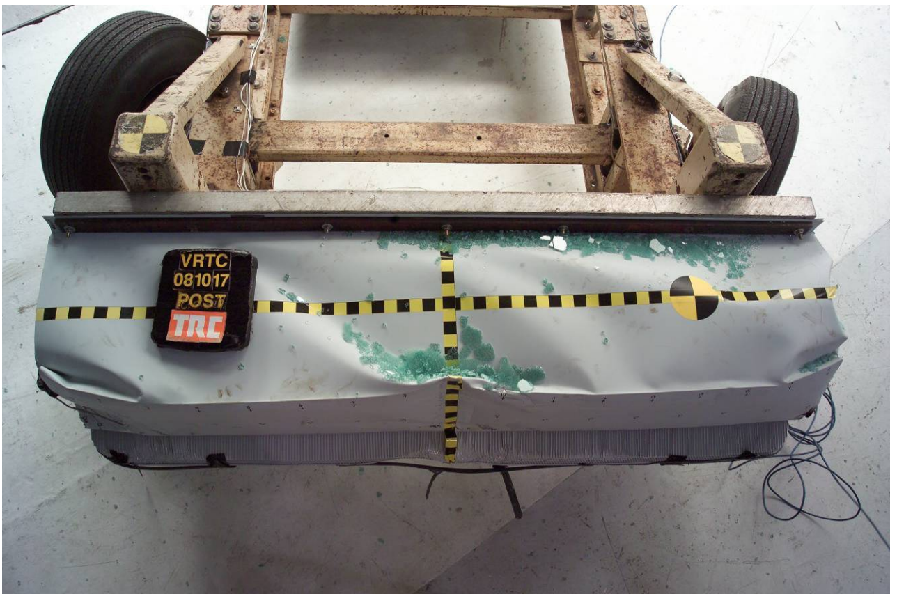
Figure A-30 Post-Test MDB Face Overhead View
