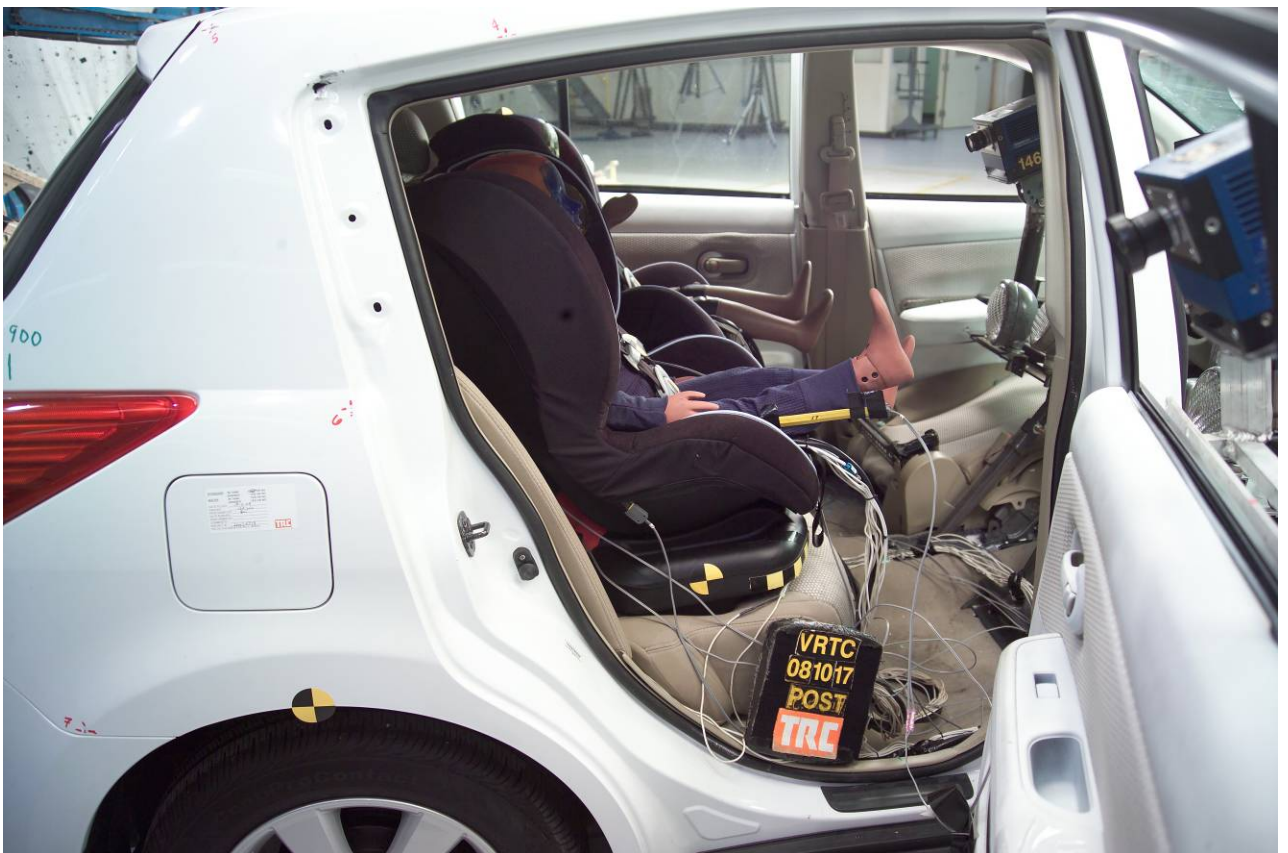
Figure A-64 Post-Test Right Rear Dummy Showing Belts, Chalking, and Contact Switches
