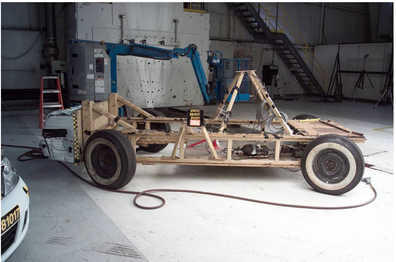
Figure A-42 Post-Test MDB Left Side Overall View
