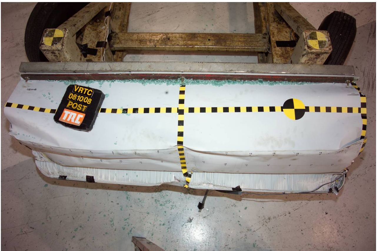
Figure A-30 Post-Test MDB Face Overhead View
