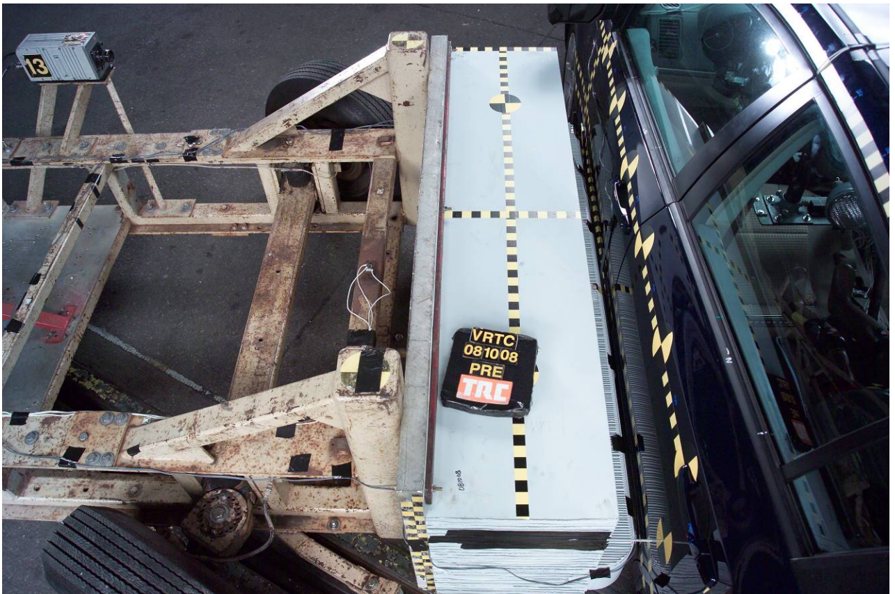
Figure A-45 Pre-Test MDB Alignment Overhead View
