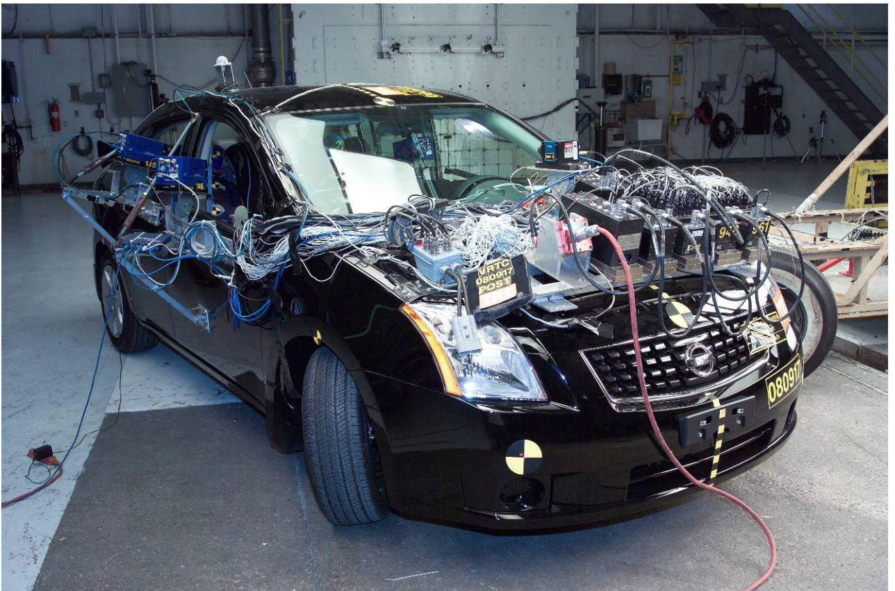
Figure A-16 Post-Test Right Front View
