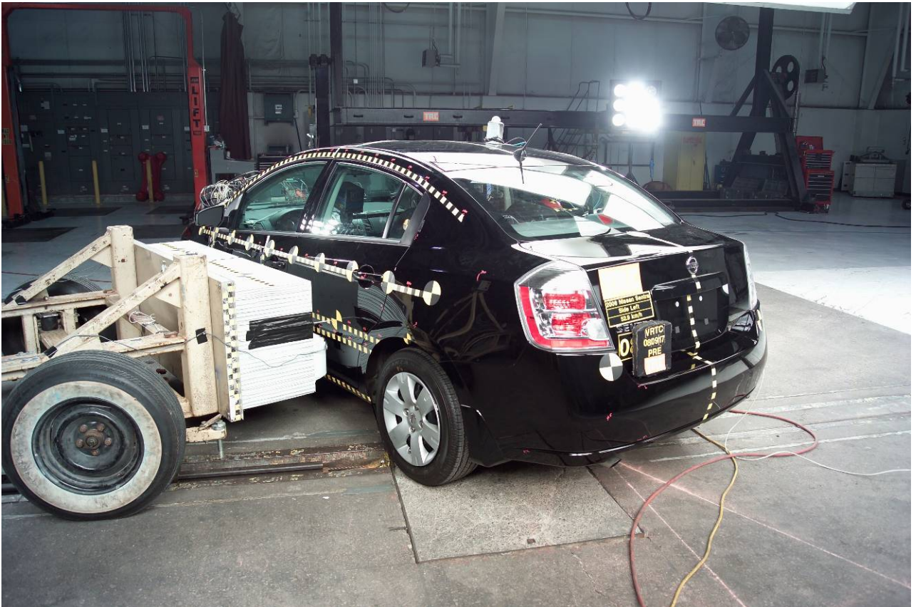
Figure A-37 Pre-Test MDB with Vehicle Right Front View
