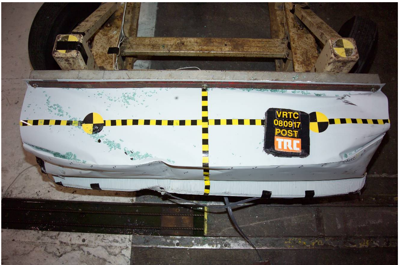
Figure A-30 Post-Test MDB Face Overhead View
