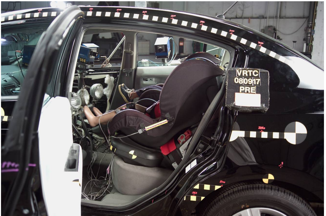
Figure A-52 Pre-Test Left Rear Dummy Showing Belts, Chalking, and Contact Switches
