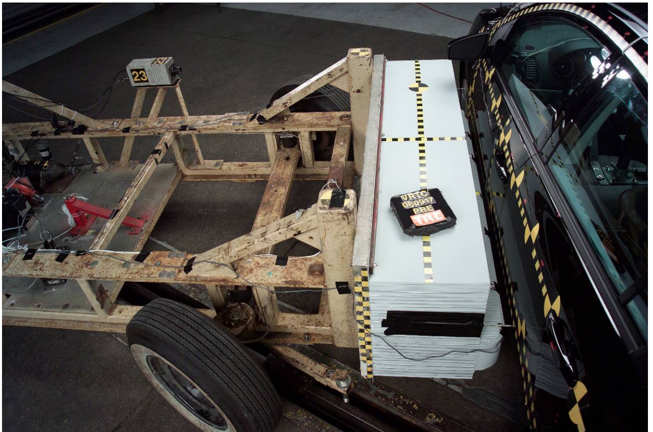
Figure A-45 Pre-Test MDB Alignment Overhead View
