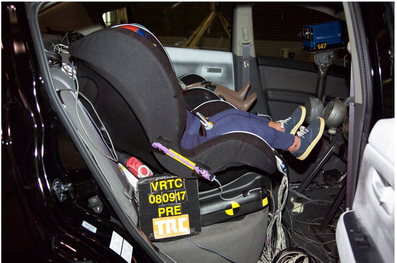
Figure A-62 Pre-Test Right Rear Dummy Showing Belts, Chalking, and Contact Switches
