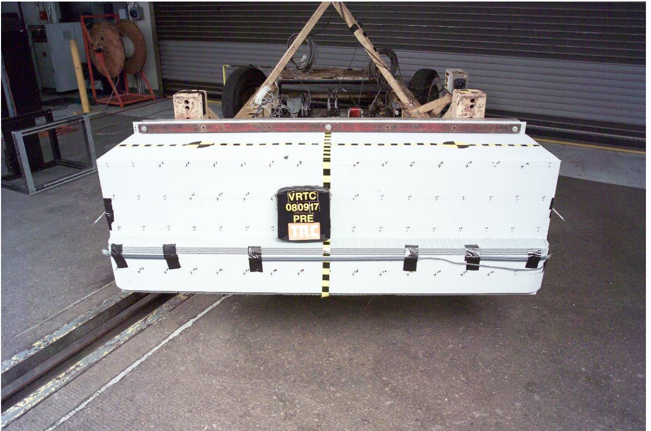
Figure A-23 Pre-Test MDB Face Front View
