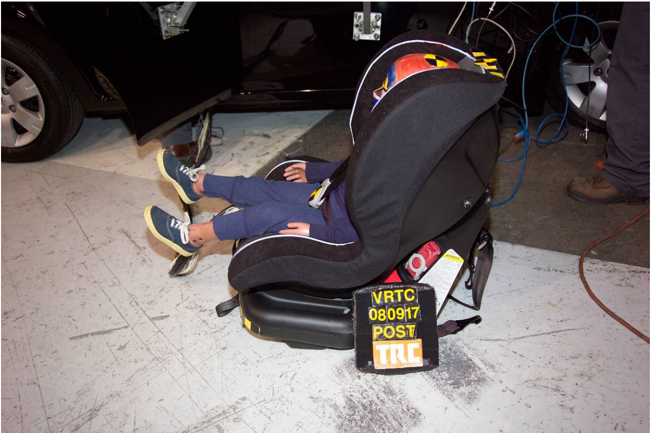
Figure A-79 Post-Test Left Side View of Right Rear CRS
