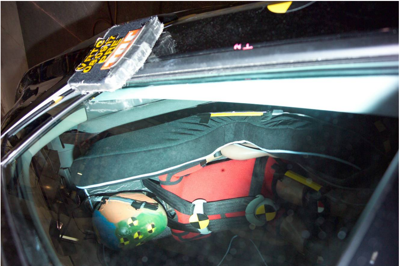
Figure A-50 Pre-Test Left Rear Dummy and Door Clearance View
