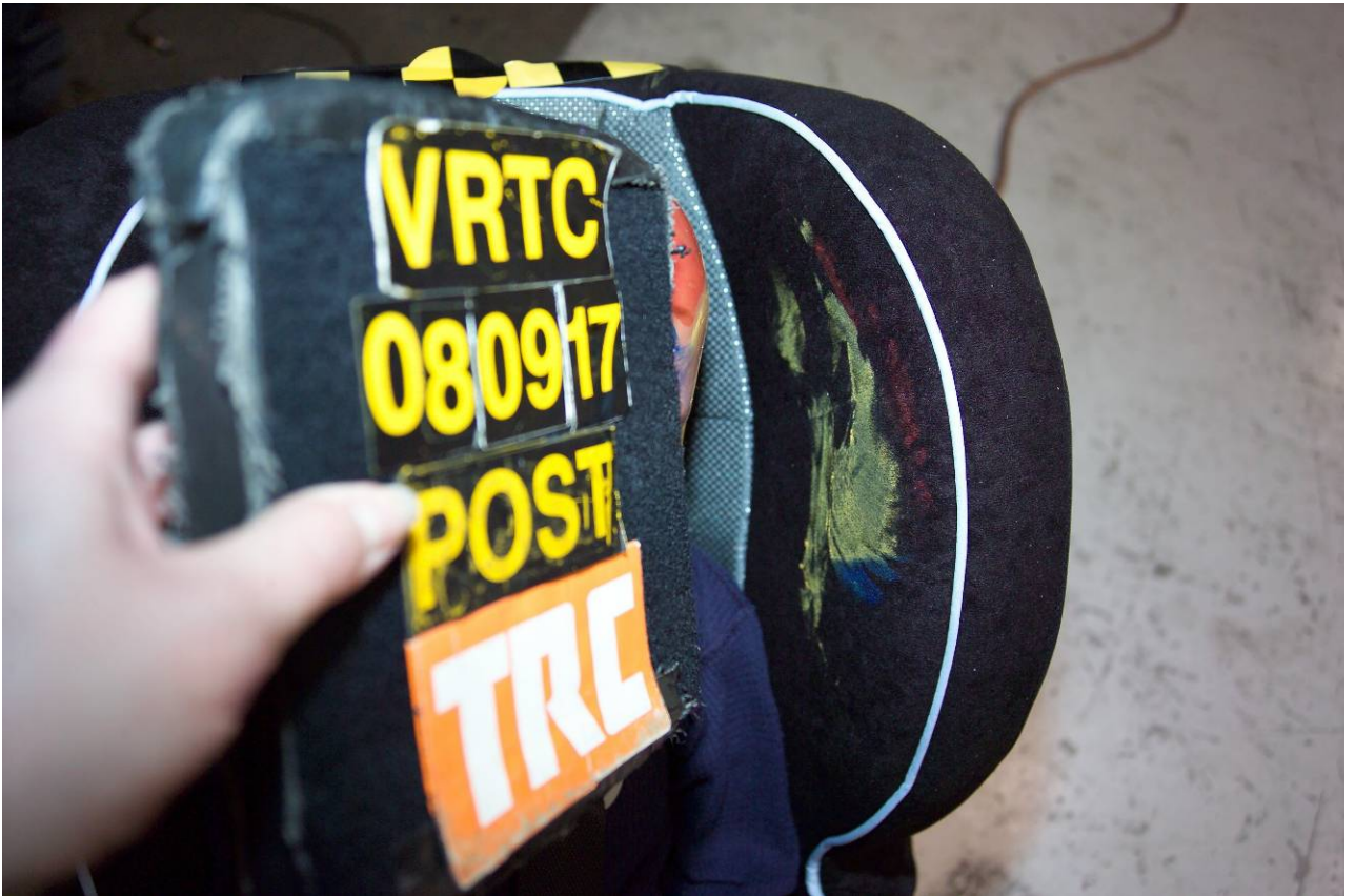
Figure A-95 Post-Test Right Rear Child Dummy Head Contact - View 1
