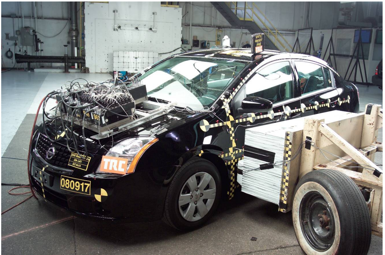
Figure A-33 Pre-Test MDB with Vehicle Left Front View
