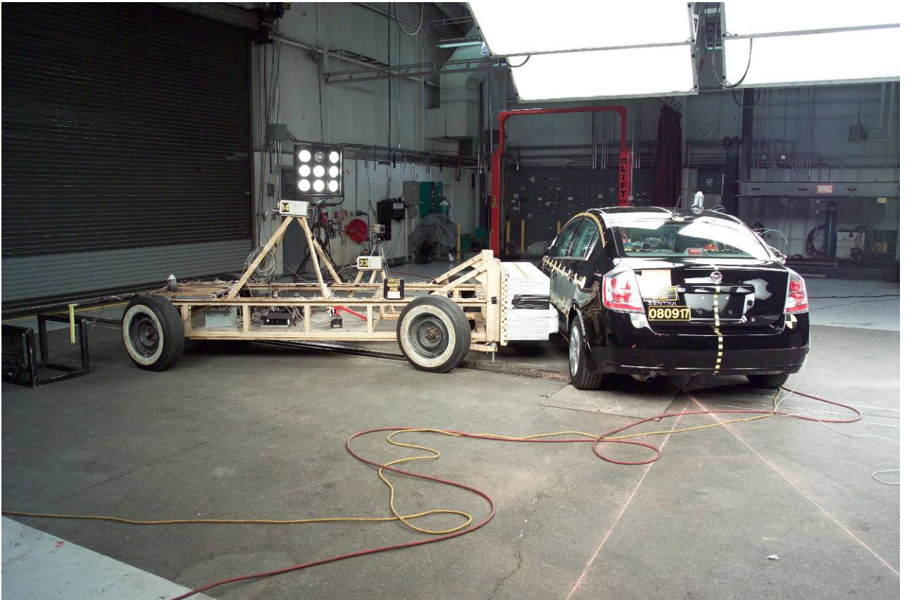
Figure A-35 Pre-Test MDB with Vehicle Right Side Overall View
