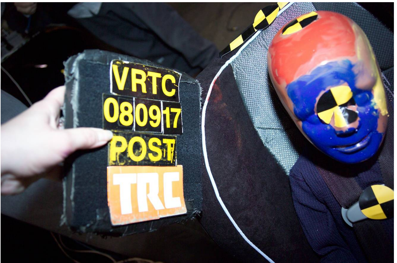
Figure A-96 Post-Test Right Rear Child Dummy Head Contact - View 2
