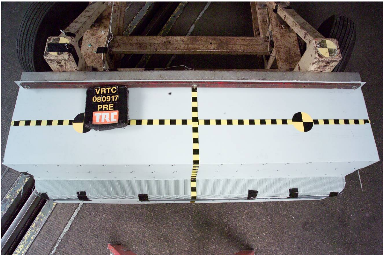
Figure A-29 Pre-Test MDB Face Overhead View
