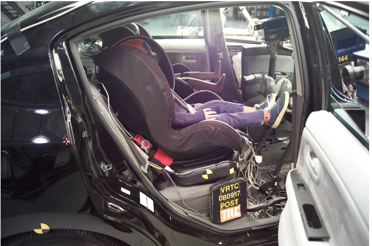
Figure A-94 Post-Test Right Side View of Right Rear Child Dummy
