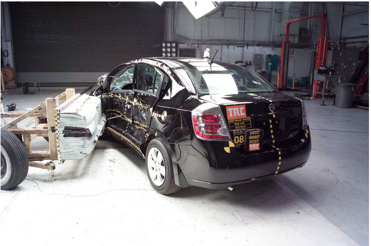
Figure A-38 Post-Test MDB with Vehicle Right Front View
