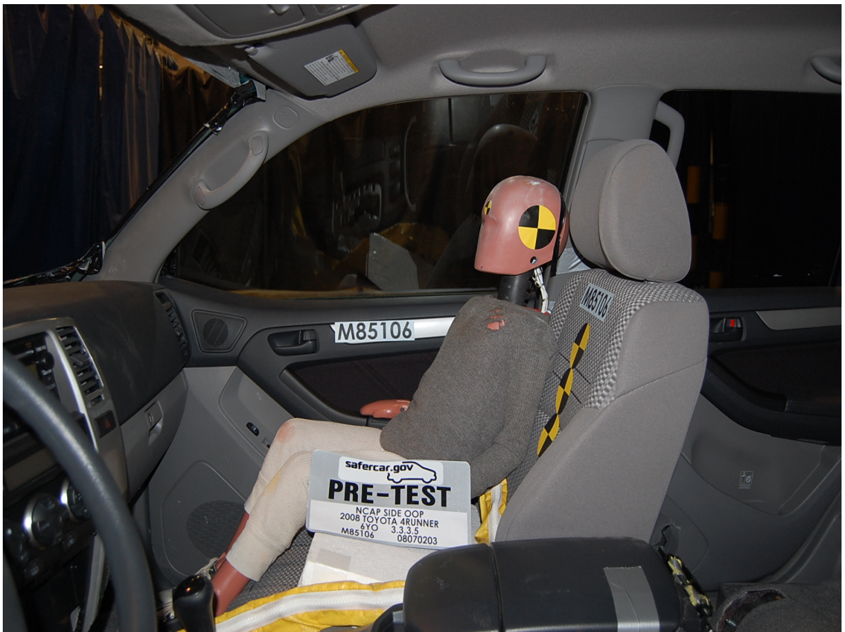
Pre-Test 6-Year-Old Dummy Left Side Closeup View
