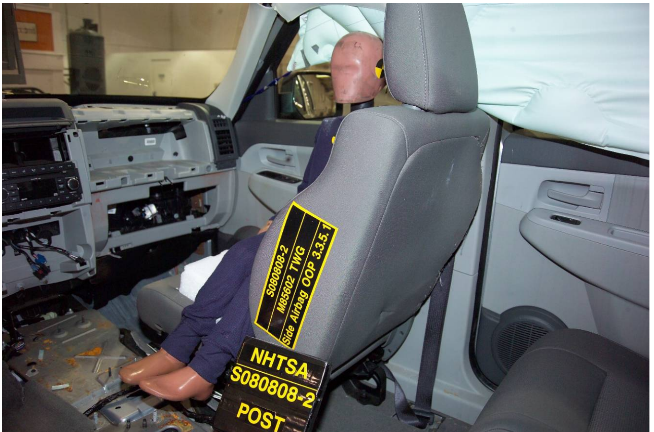
Figure A-18 Post-Test Front SID Rear View
