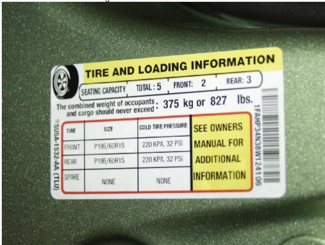
Figure A-4: Vehicle Tire Placard
