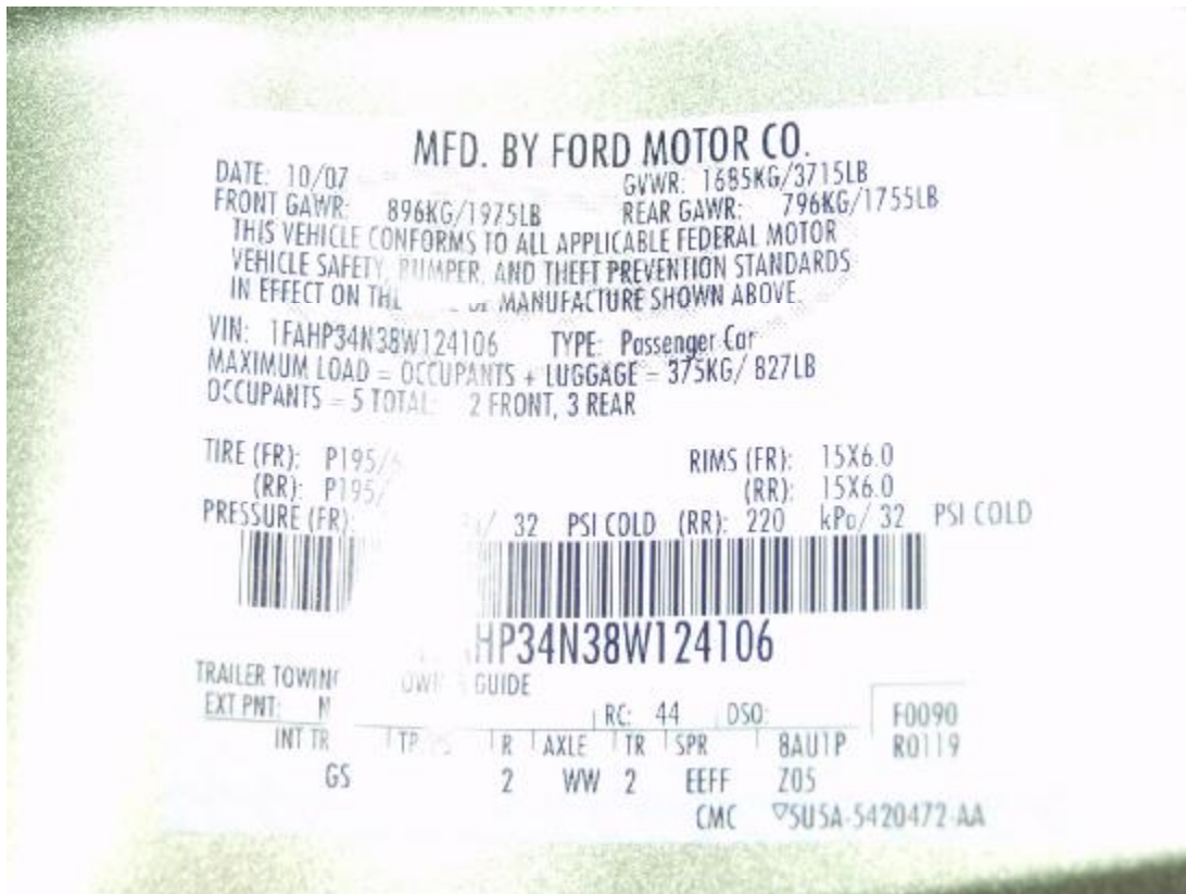
Figure A-3: Vehicle Certification Placard
