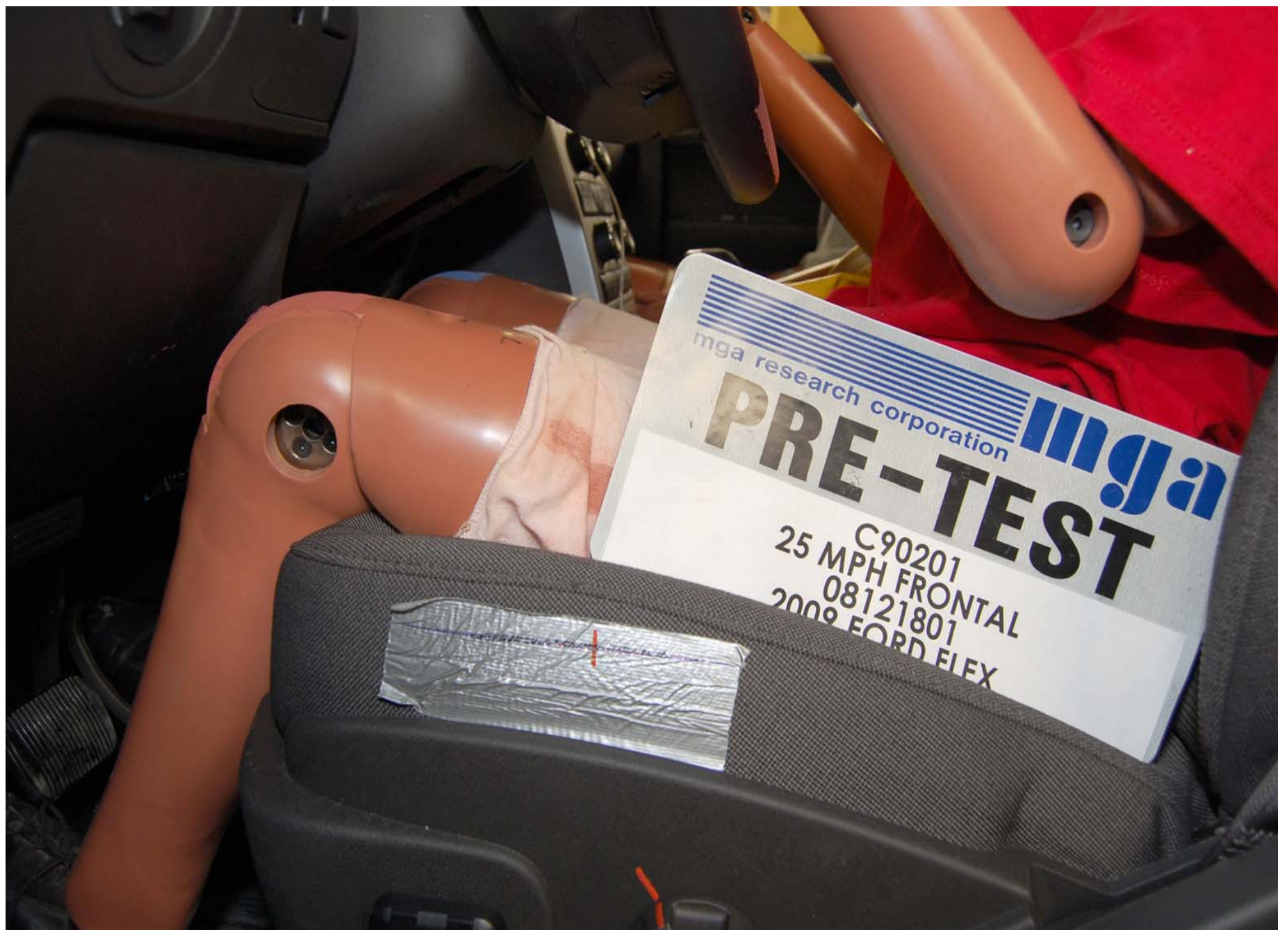
Pre-Test Driver Side Knee Bolster View
