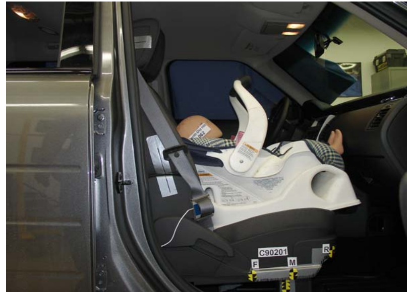
Graco Infant W/ Base Forward Facing Unbelted, Forward Seat Track
