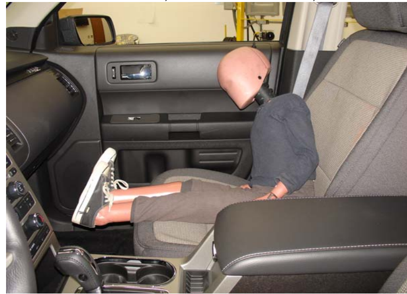
6-Year-Old Unbelted, Rearward Seat Track, Position 4
