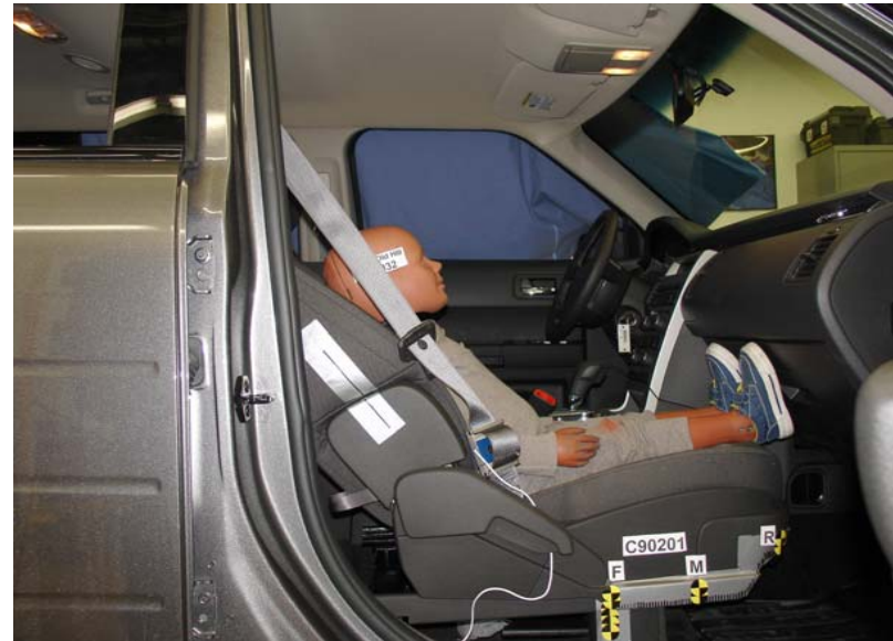
3-Year-Old Unbelted, Forward Seat Track, Position 2
