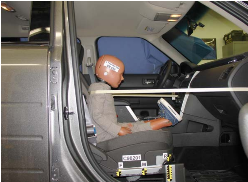
3-Year-Old Unbelted, Rearward Seat Track, Position 3
