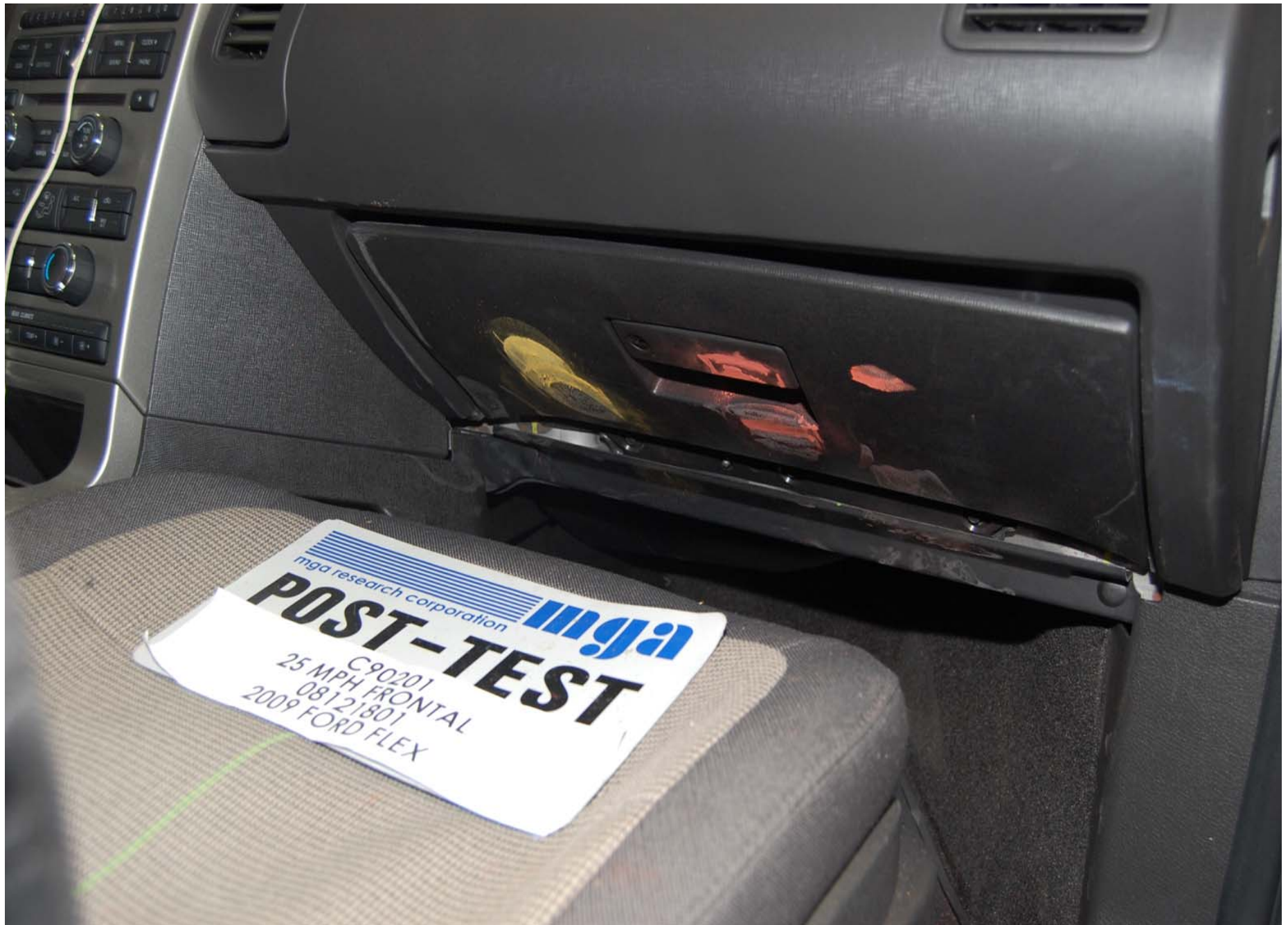
Post-Test Passenger Dummy Knee Contact
