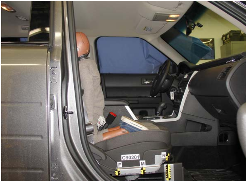
3-Year-Old Unbelted, Rearward Seat Track, Position 7
