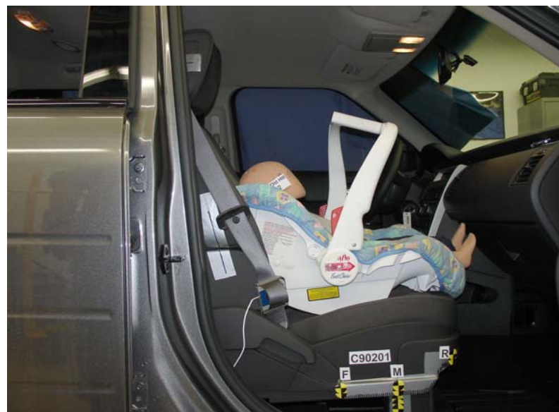
Evenflo First Choice 204 Forward Facing Unbelted, Middle Seat Track
