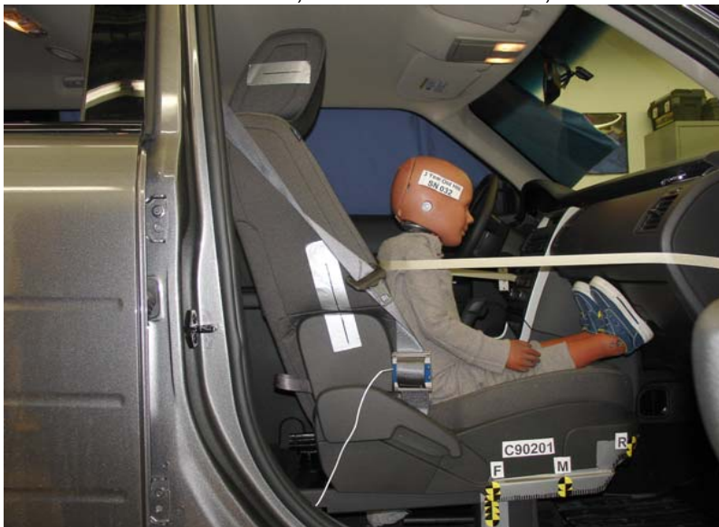
3-Year-Old Unbelted, Forward Seat Track, Position 3
