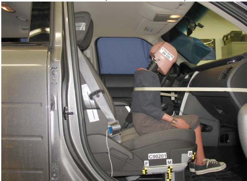
6-Year-Old Unbelted, Middle Seat Track, Position 3
