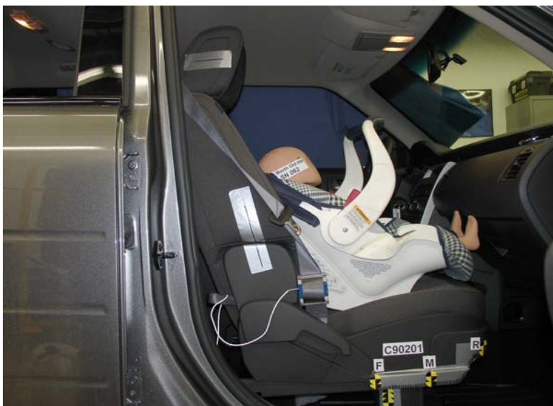
Graco Infant W/O Base Forward Facing Unbelted, Forward Seat Track
