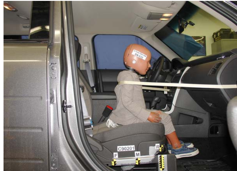
3-Year-Old Unbelted, Rearward Seat Track, Position 4
