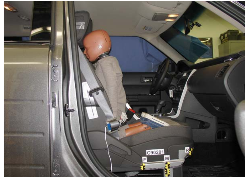
3-Year-Old Unbelted, Middle Seat Track, Position 7
