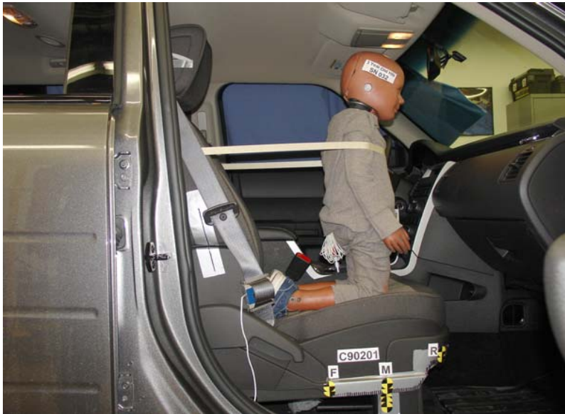
3-Year-Old Unbelted, Middle Seat Track, Position 6
