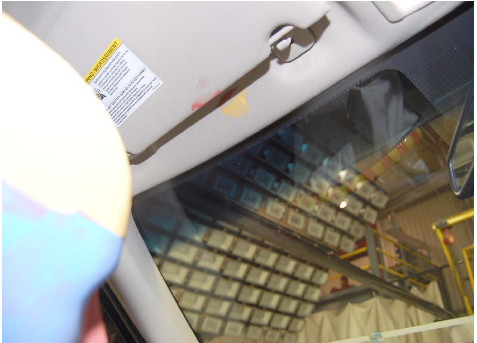
Post-Test Driver Dummy Head Contact (visor)
