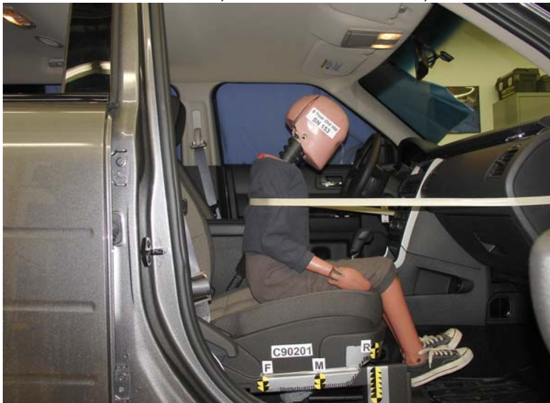
6-Year-Old Unbelted, Rearward Seat Track, Position 3
