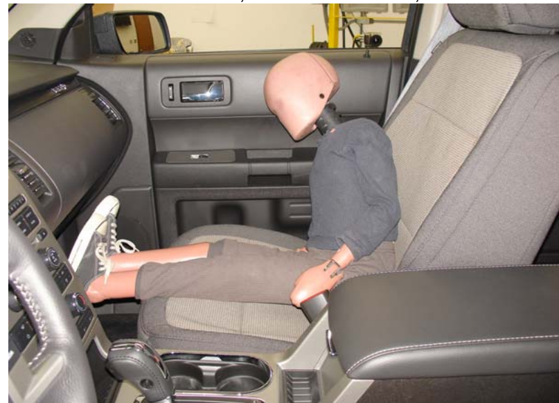
6-Year-Old Unbelted, Middle Seat Track, Position 4
