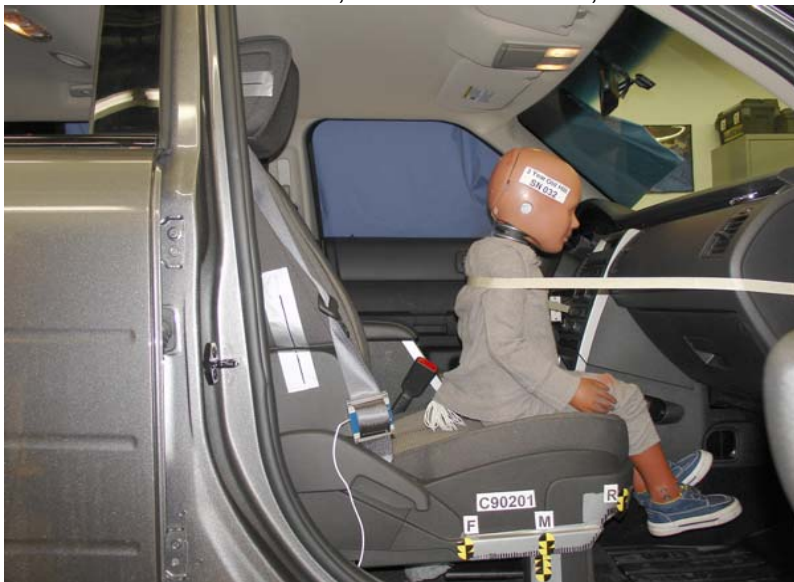
3-Year-Old Unbelted, Middle Seat Track, Position 4
