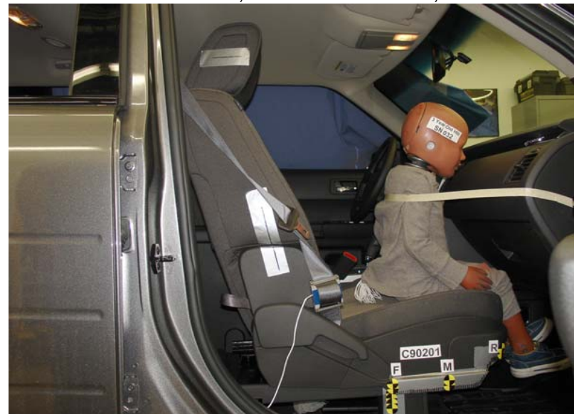
3-Year-Old Unbelted, Forward Seat Track, Position 4
