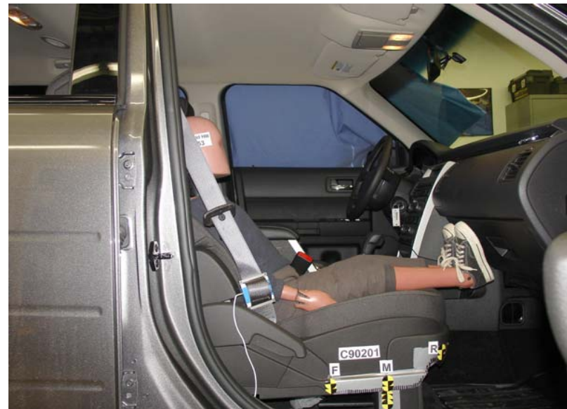
6-Year-Old Unbelted, Middle Seat Track, Position 2
