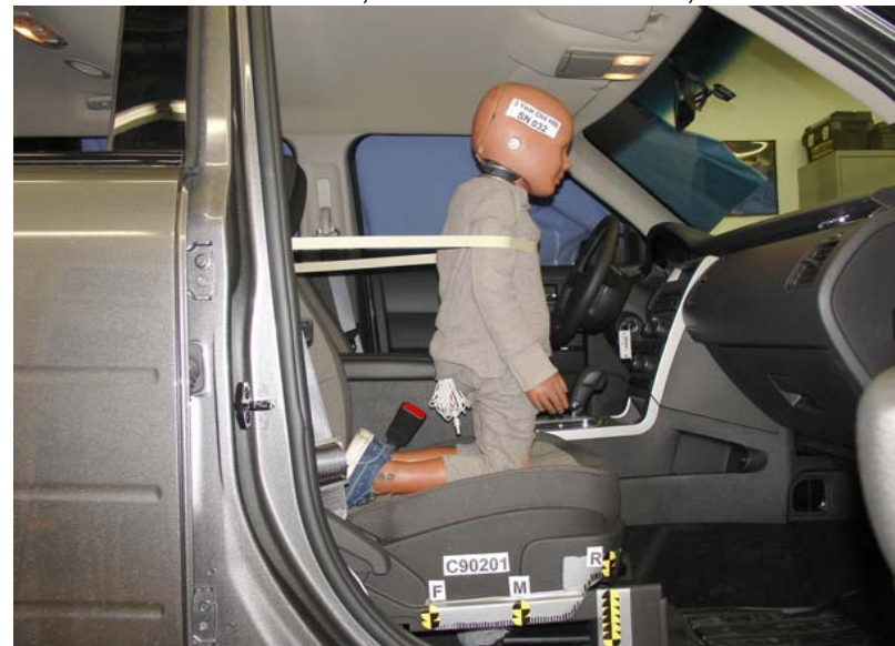
3-Year-Old Unbelted, Rearward Seat Track, Position 6
