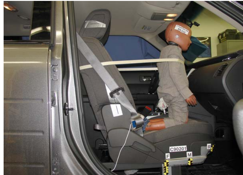
3-Year-Old Unbelted, Forward Seat Track, Position 6
