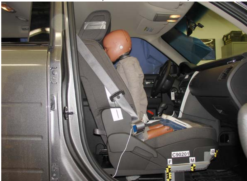
3-Year-Old Unbelted, Forward Seat Track, Position 7
