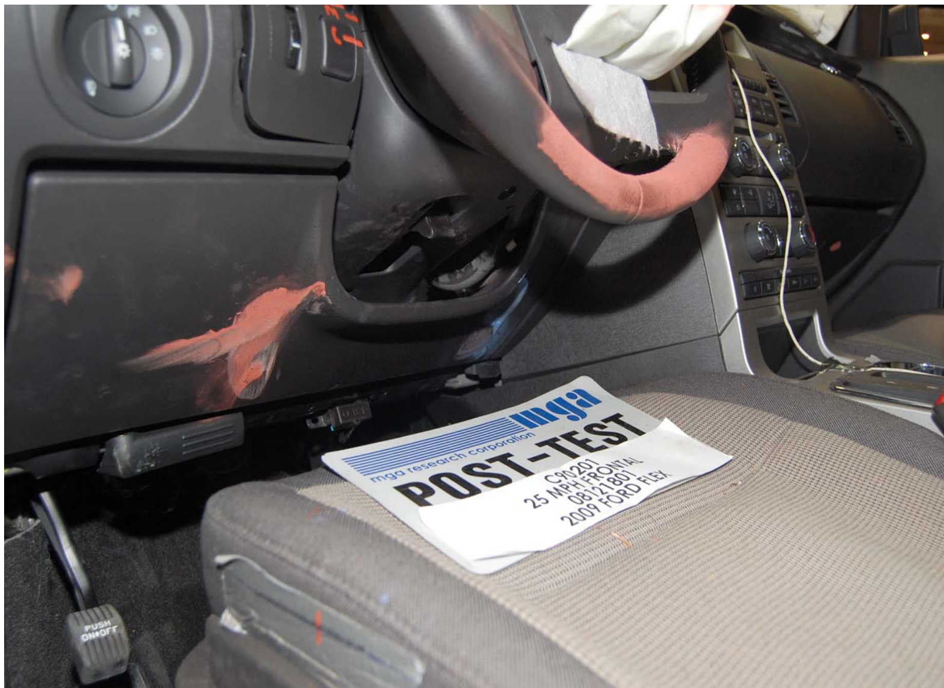
Post-Test Driver Dummy Knee Contact
