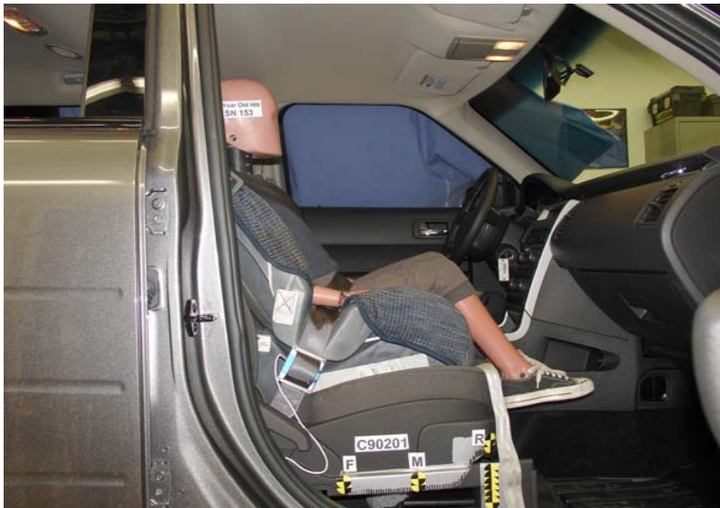
6-Year-Old Cosco High Back Booster Belted, Rearward Seat Track
