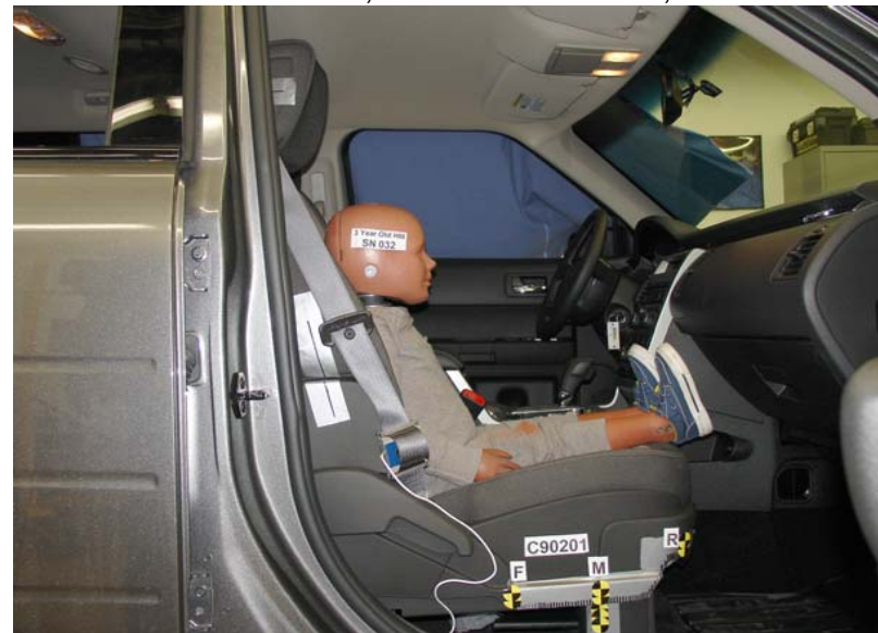
3-Year-Old Unbelted, Middle Seat Track, Position 1
