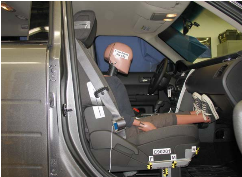
6-Year-Old Unbelted, Forward Seat Track, Position 1
