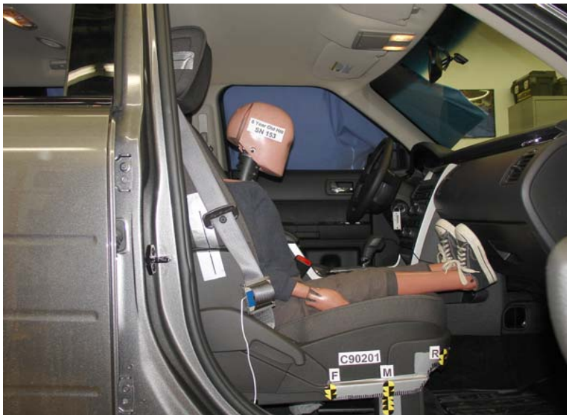
6-Year-Old Unbelted, Middle Seat Track, Position 1
