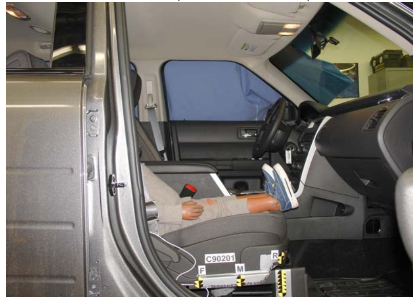
3-Year-Old Unbelted, Rearward Seat Track, Position 2
