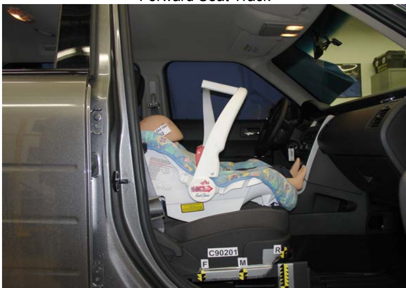
Evenflo First Choice 204 Forward Facing Unbelted, Rearward Seat Track
