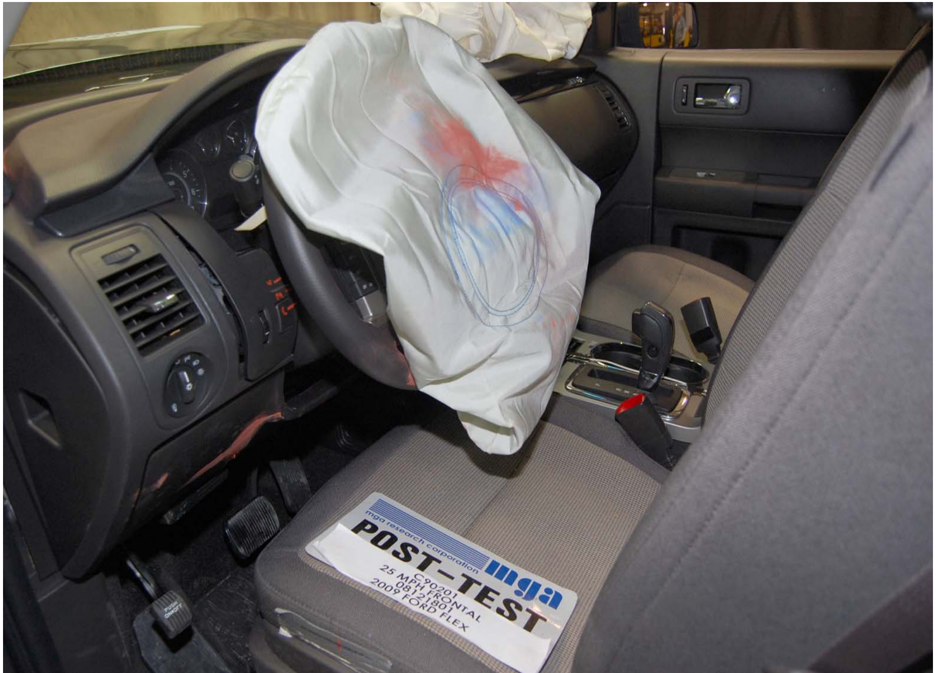
Post-Test Driver Dummy Airbag Contact
