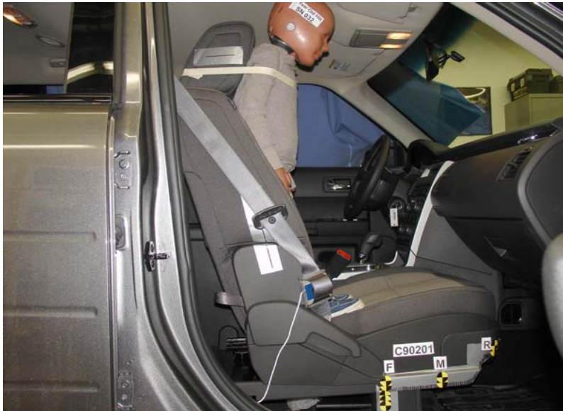
3-Year-Old Unbelted, Forward Seat Track, Position 5
