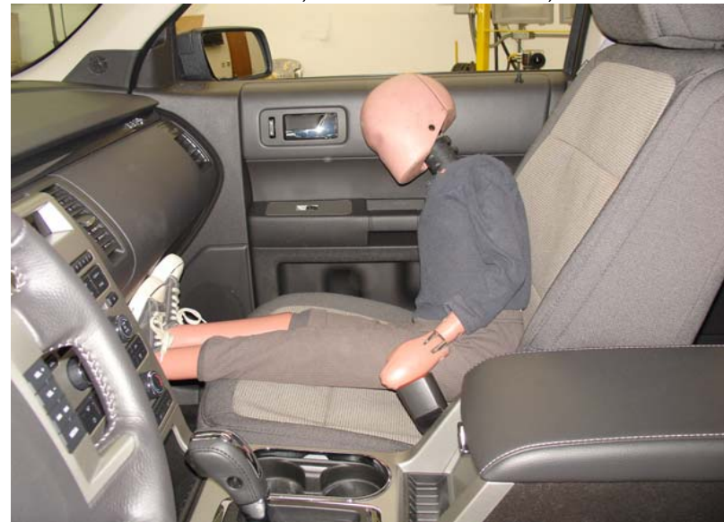
6-Year-Old Unbelted, Forward Seat Track, Position 4
