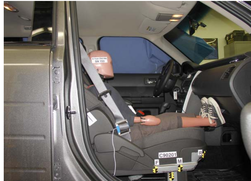
6-Year-Old Unbelted, Forward Seat Track, Position 2
