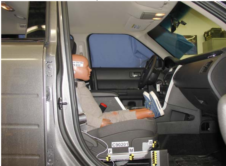
3-Year-Old Unbelted, Rearward Seat Track, Position 1
