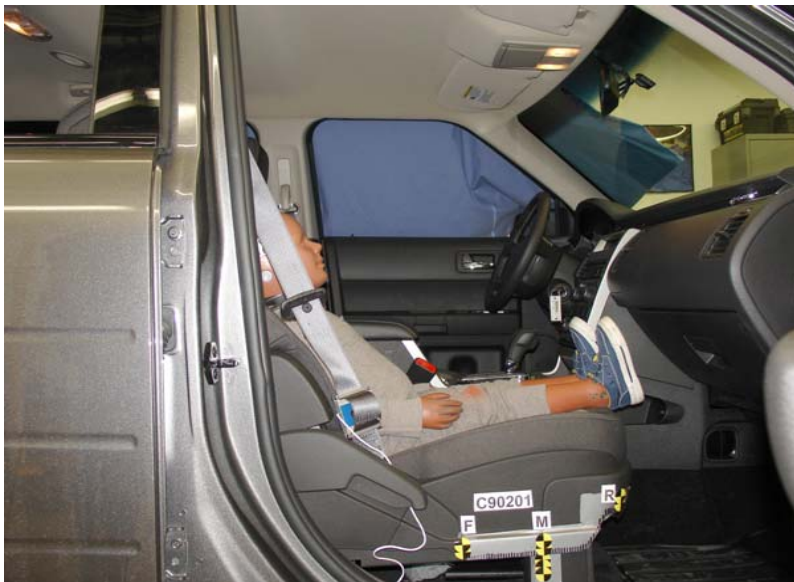
3-Year-Old Unbelted, Middle Seat Track, Position 2
