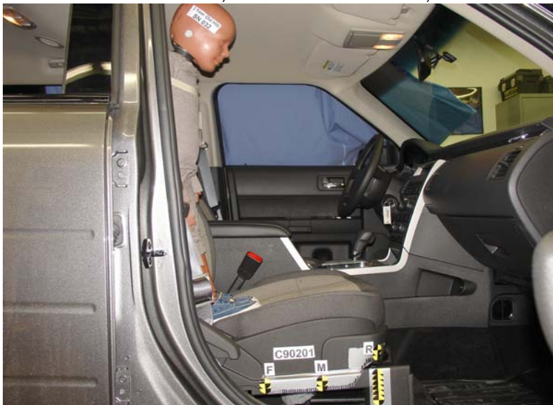
3-Year-Old Unbelted, Rearward Seat Track, Position 5
