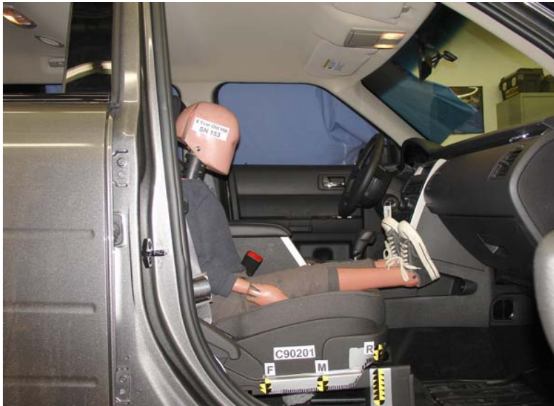
6-Year-Old Unbelted, Rearward Seat Track, Position 1
