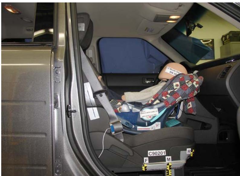
Britax Handle With Care 191 Unbelted, Middle Seat Track
