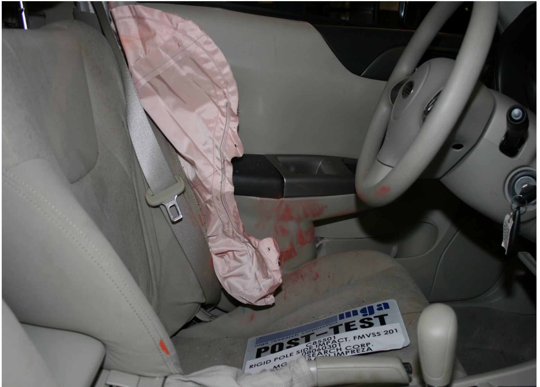
Post-Test Driver Dummy Upper Thorax Contact
