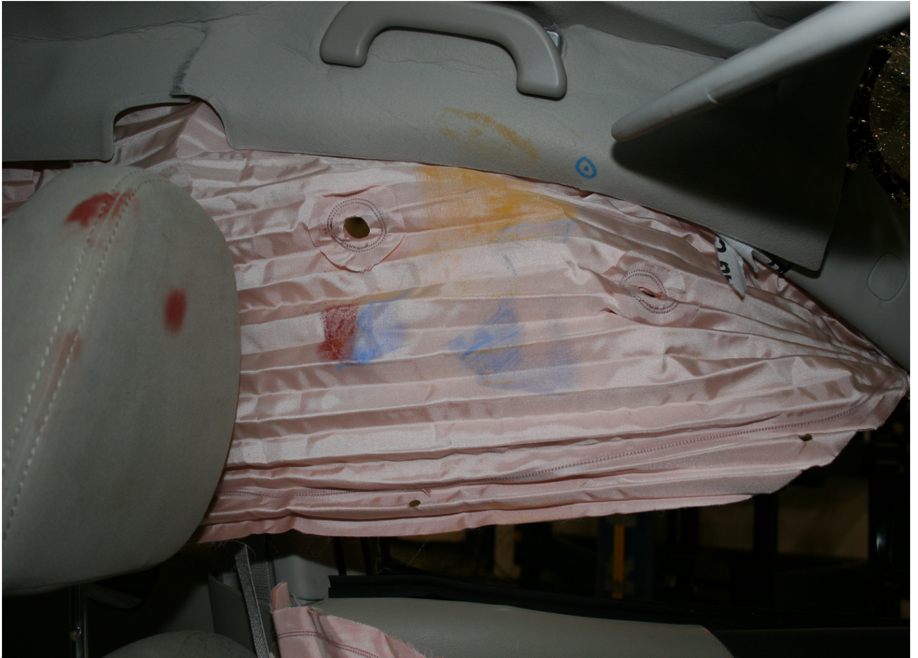
Post-Test Driver Dummy Head Contact (CAB & Headrest)
