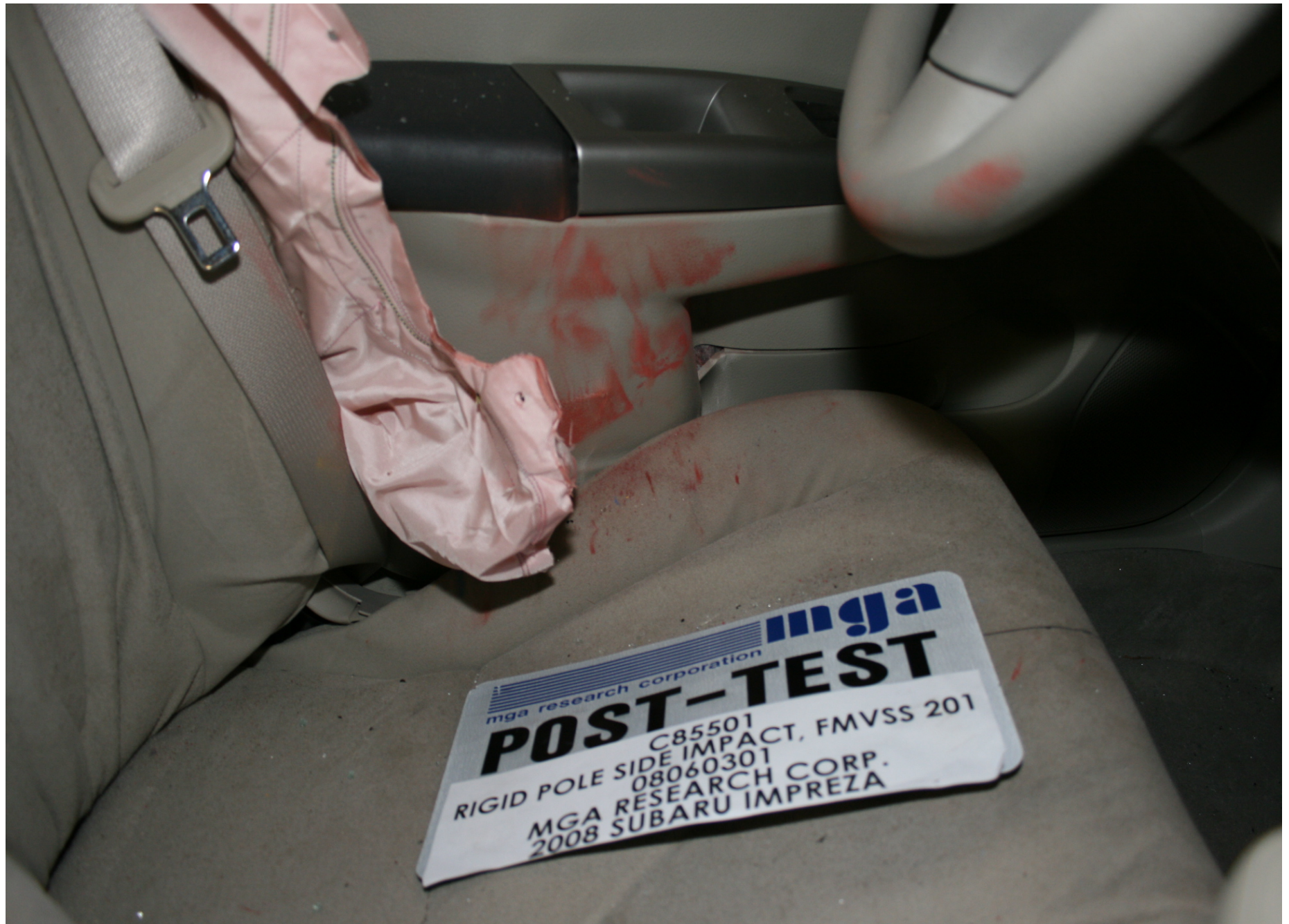
Post-Test Driver Dummy Lower Thorax Contact
