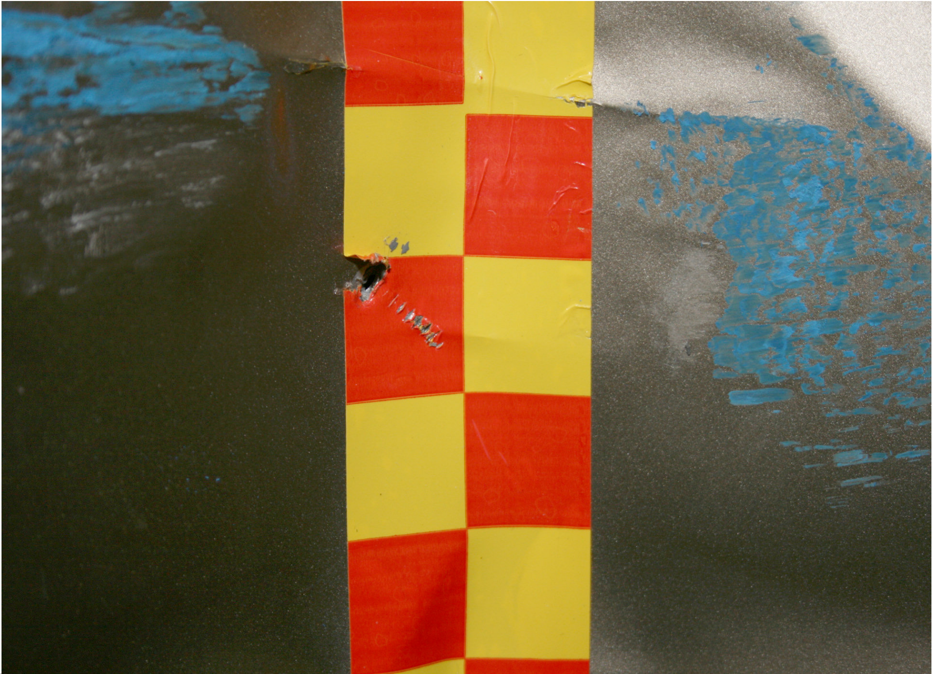
Post-Test Impact Point on Vehicle
