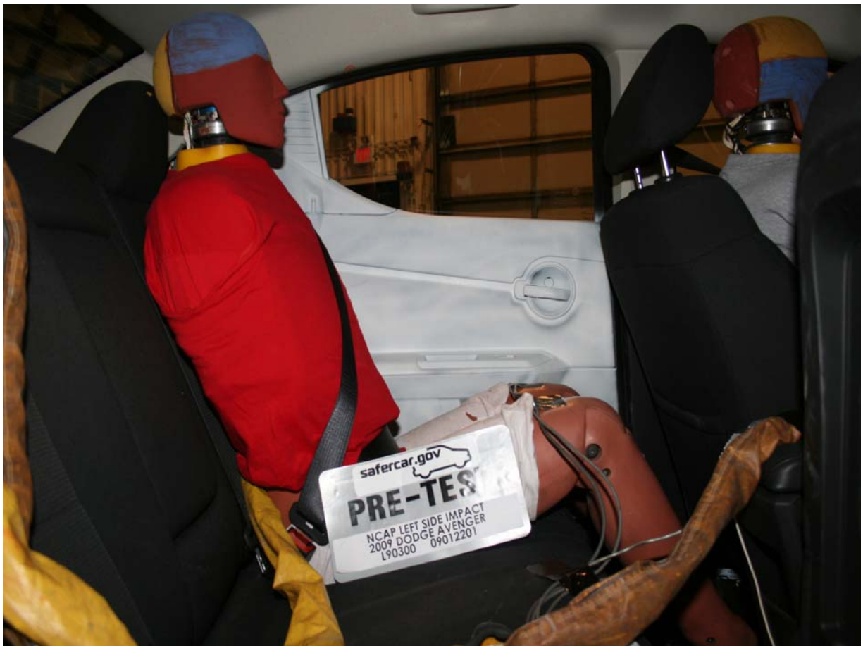
Pre-Test Passenger Dummy Right Side View
