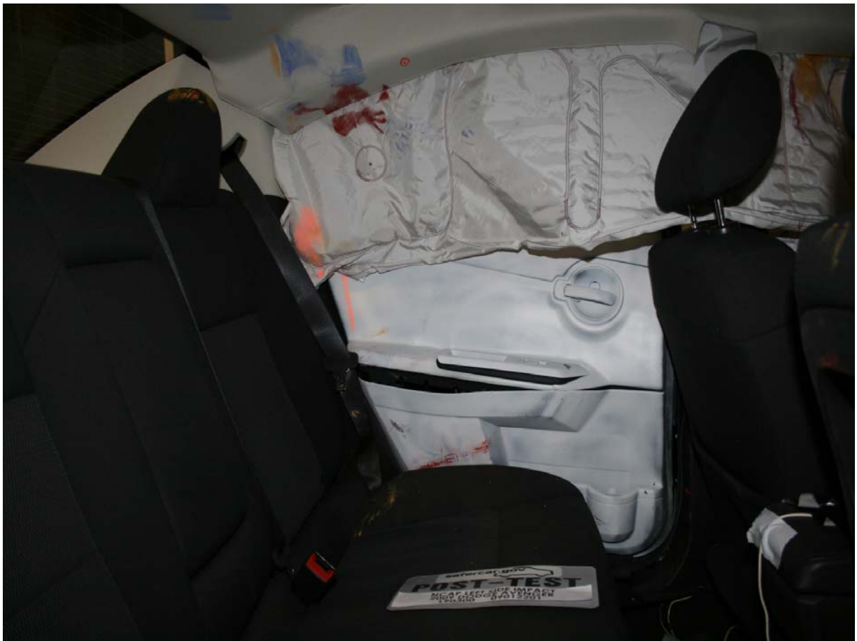
Post-Test Passenger Dummy Contact
