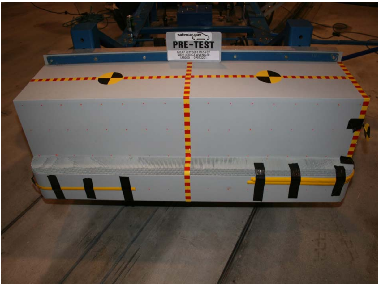
Pre-Test Front View of Deformable Barrier
