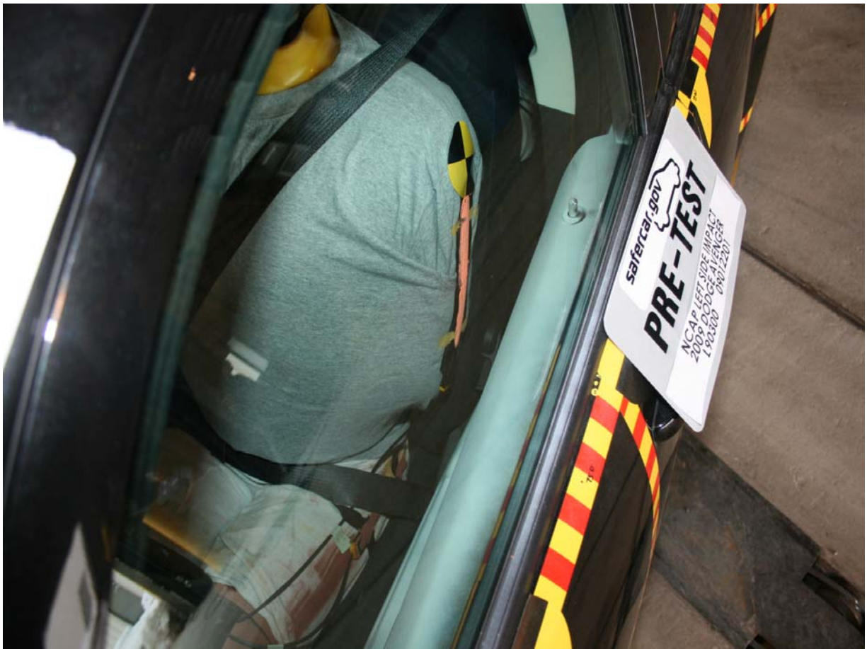
Pre-Test Driver Dummy Clearance From Door
