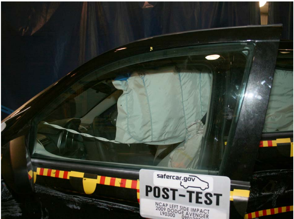
Post-Test Driver Dummy (Through Window)
