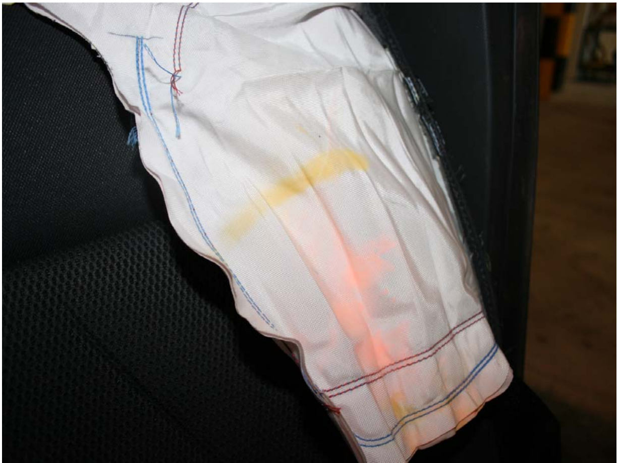
Post-Test Driver Dummy Upper Torso Contact
