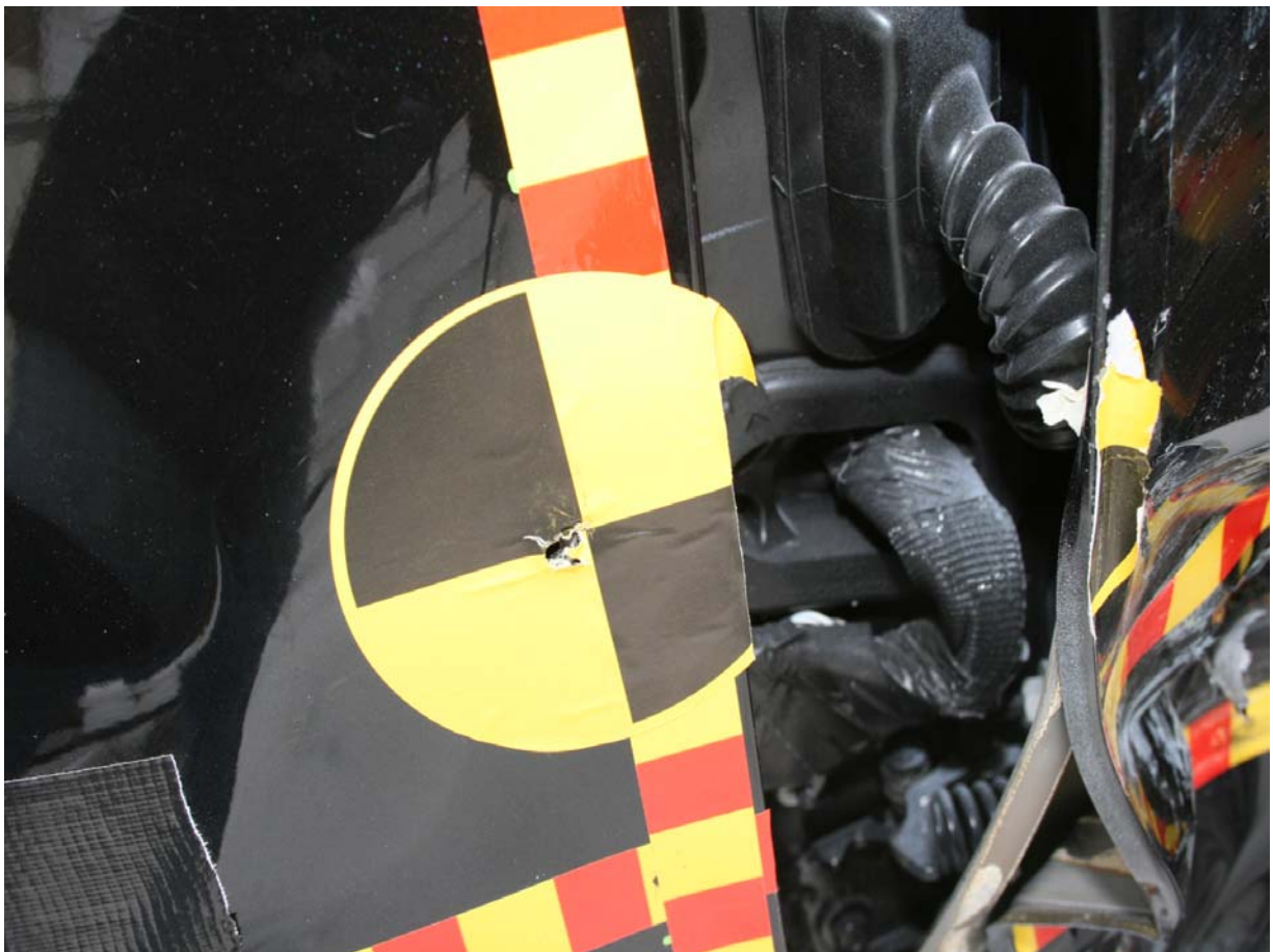
Post-Test Left Impact Point
