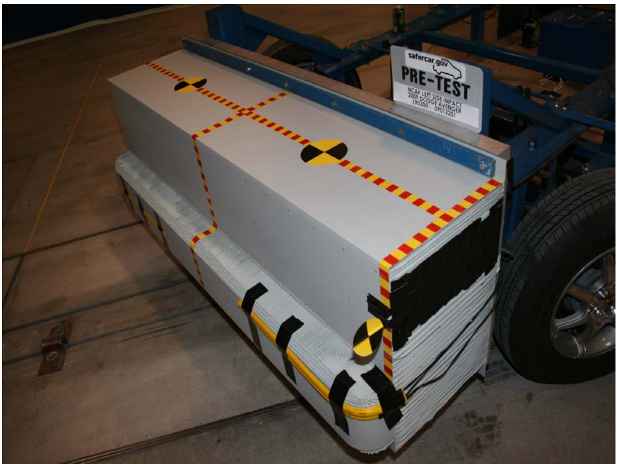
Pre-Test Left Side View of Deformable Barrier
