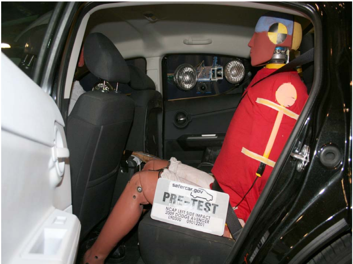
Pre-Test Passenger Dummy (Door Open)
