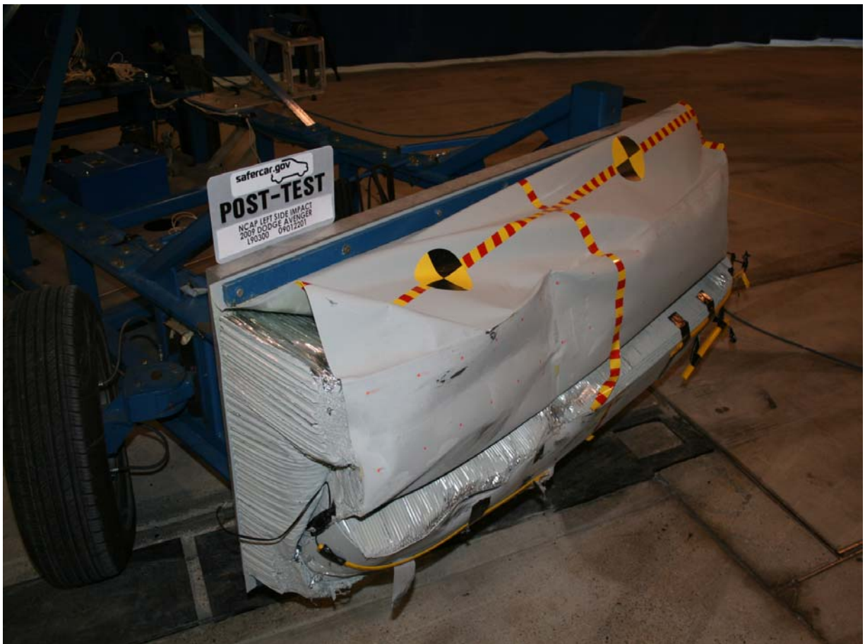
Post-Test Right Side View of Deformable Barrier
