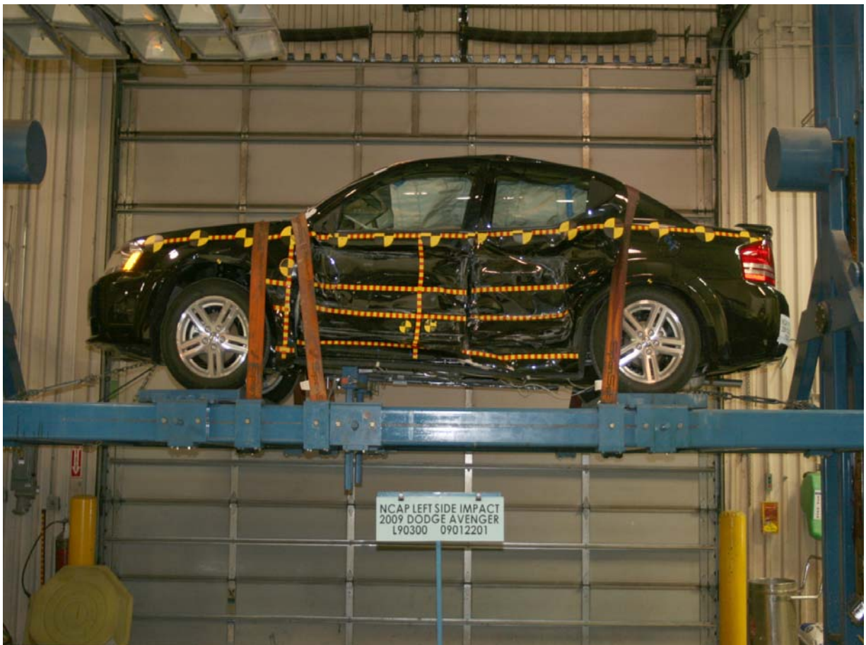
Vehicle on Rollover Device (360 Degrees)
