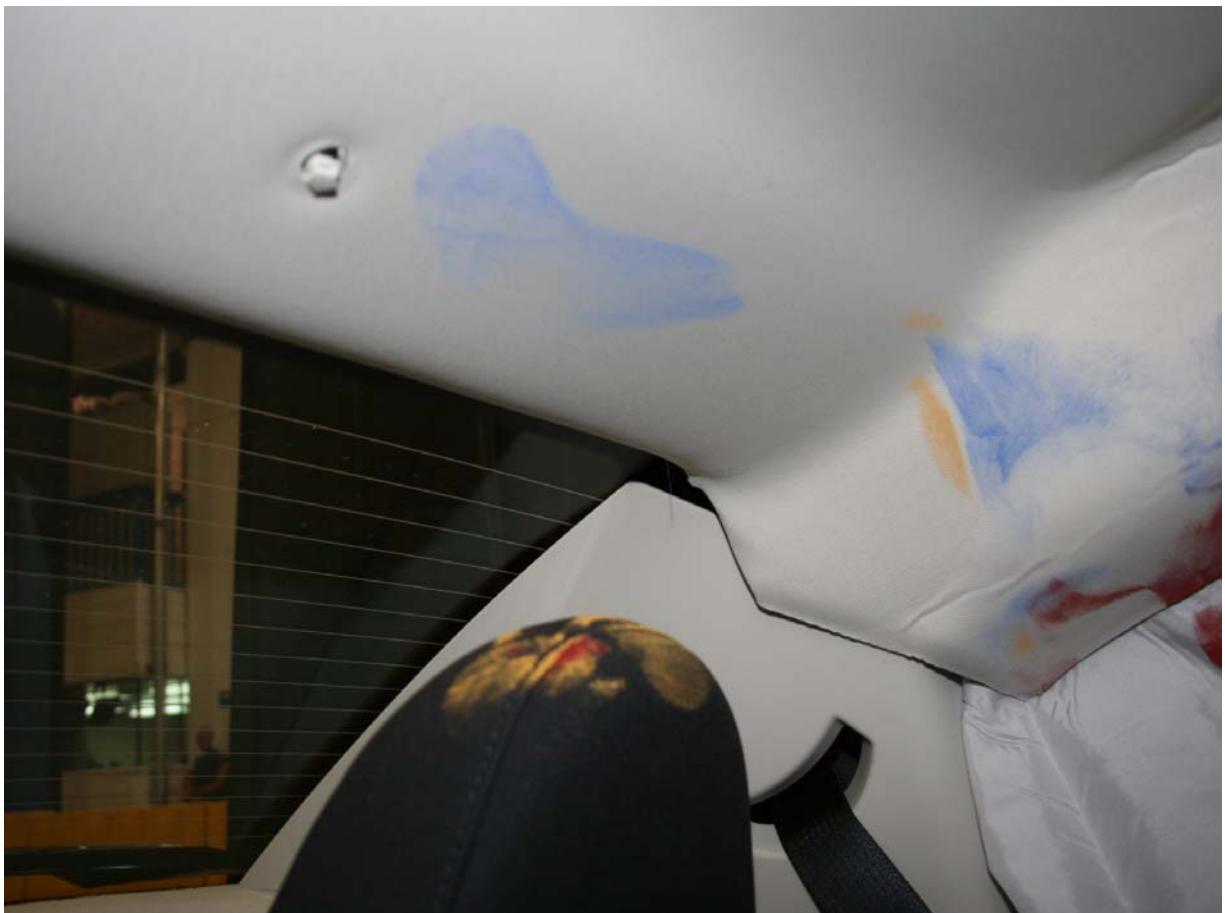
Post-Test Passenger Dummy Head Contact View 2
