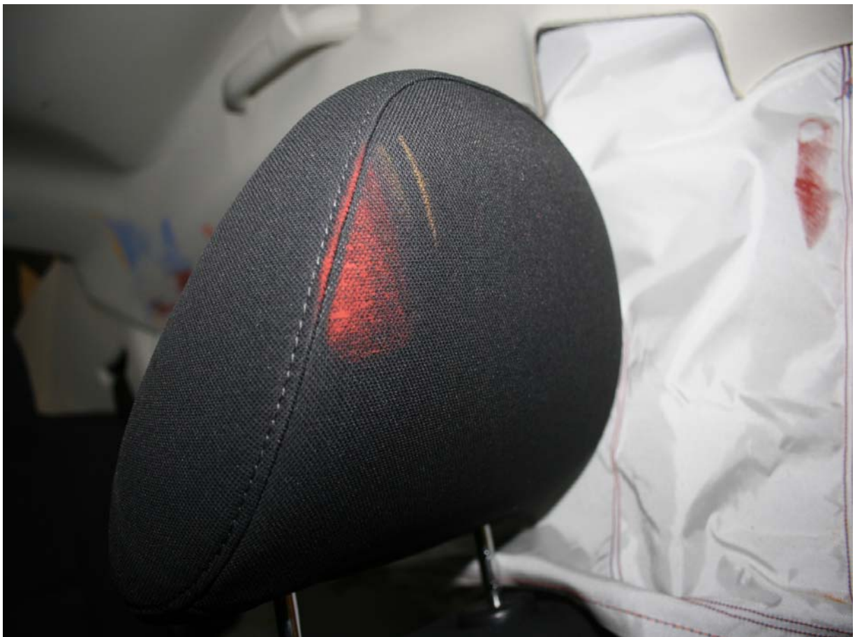
Post-Test Driver Dummy Head Contact View 2
