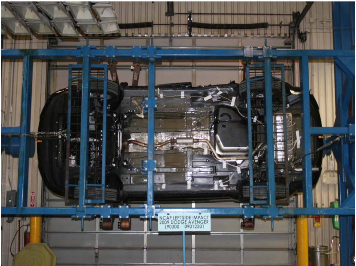
Vehicle on Rollover Device (270 Degrees)
