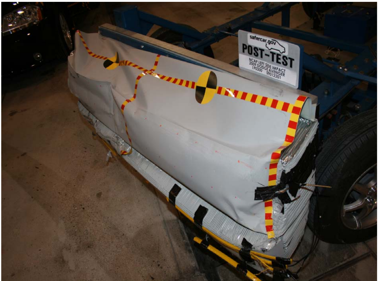
Post-Test Left Side View of Deformable Barrier
