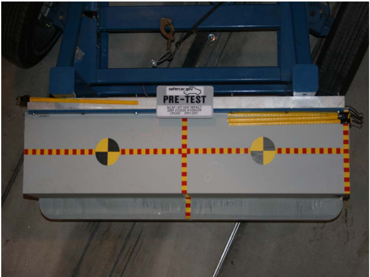
Pre-Test Top View of Deformable Barrier
