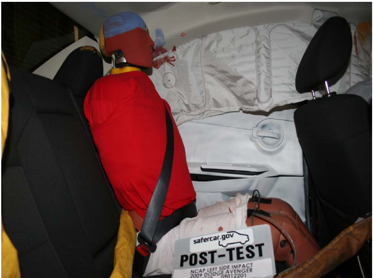
Post-Test Passenger Dummy Right Side View
