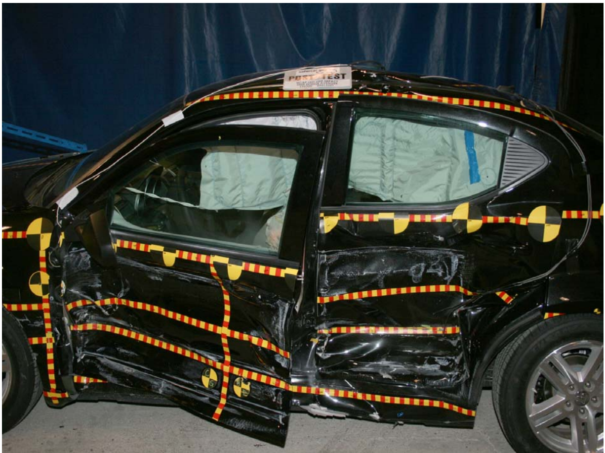
Post-Test Left Side Impact Close-up
