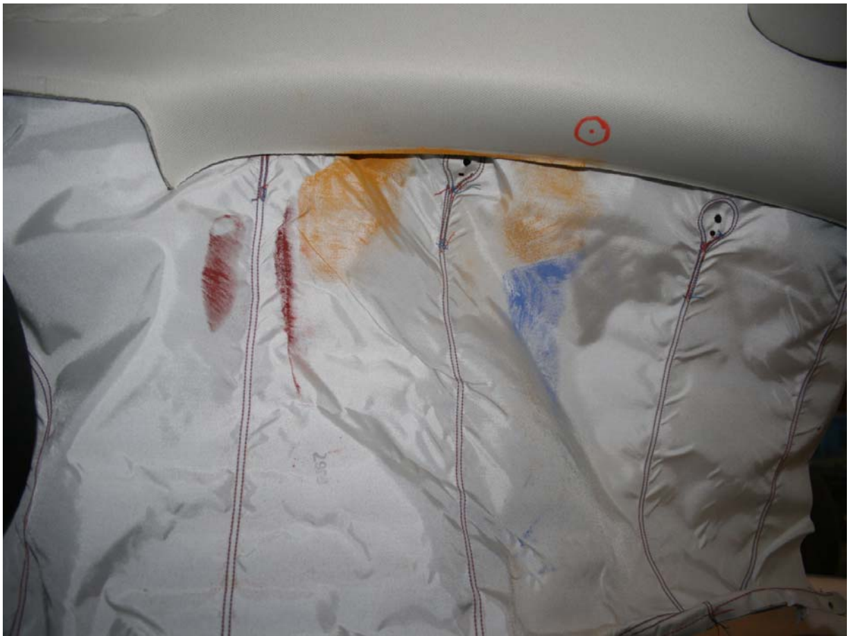
Post-Test Driver Dummy Head Contact View 1
