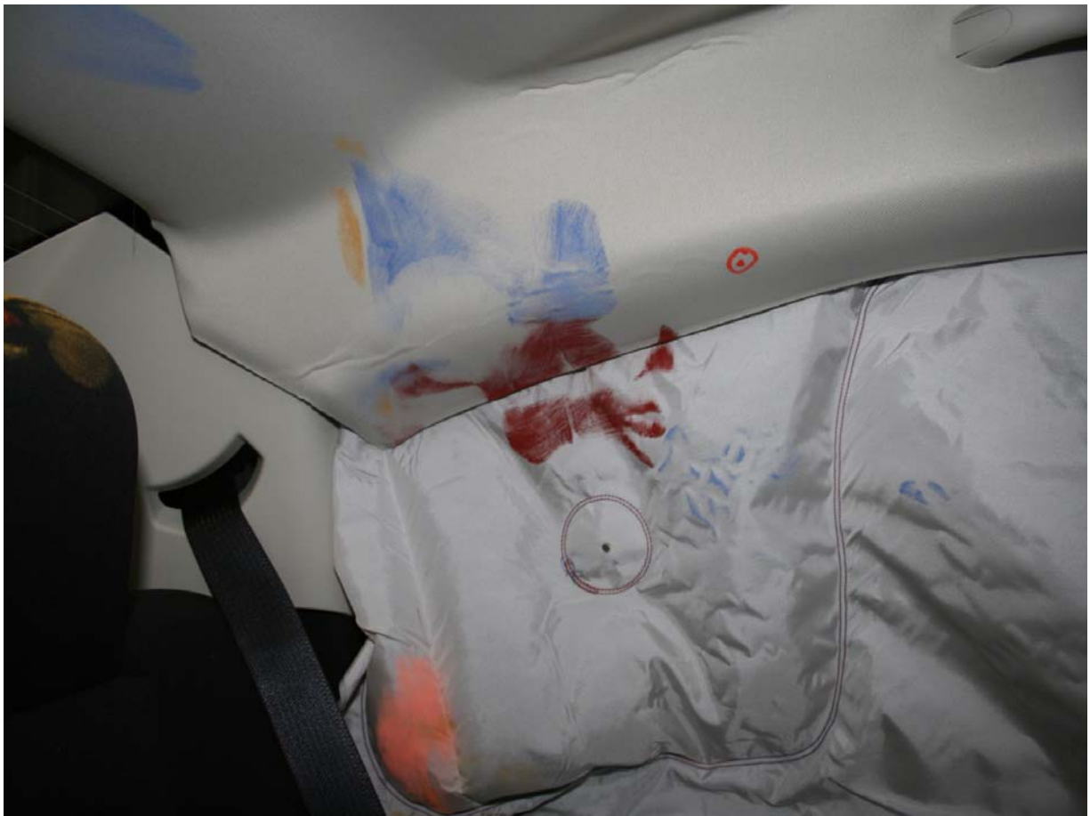
Post-Test Passenger Dummy Head Contact View 1
