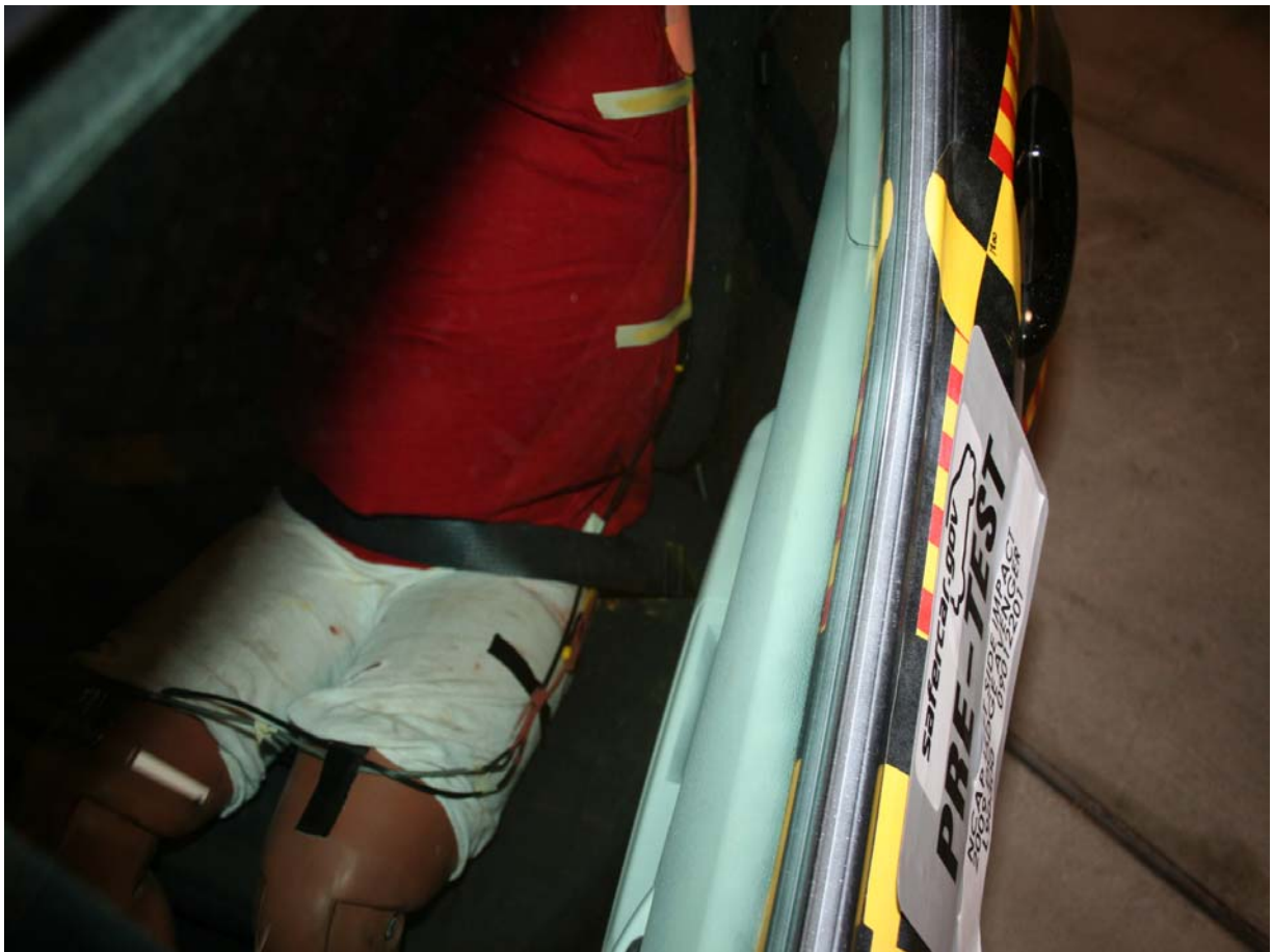
Pre-Test Passenger Dummy Clearance From Door
