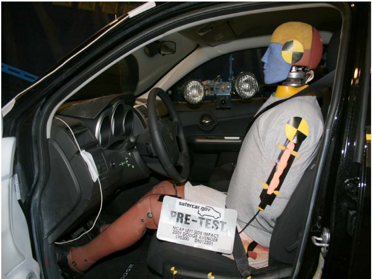
Pre-Test Driver Dummy (Door Open)
