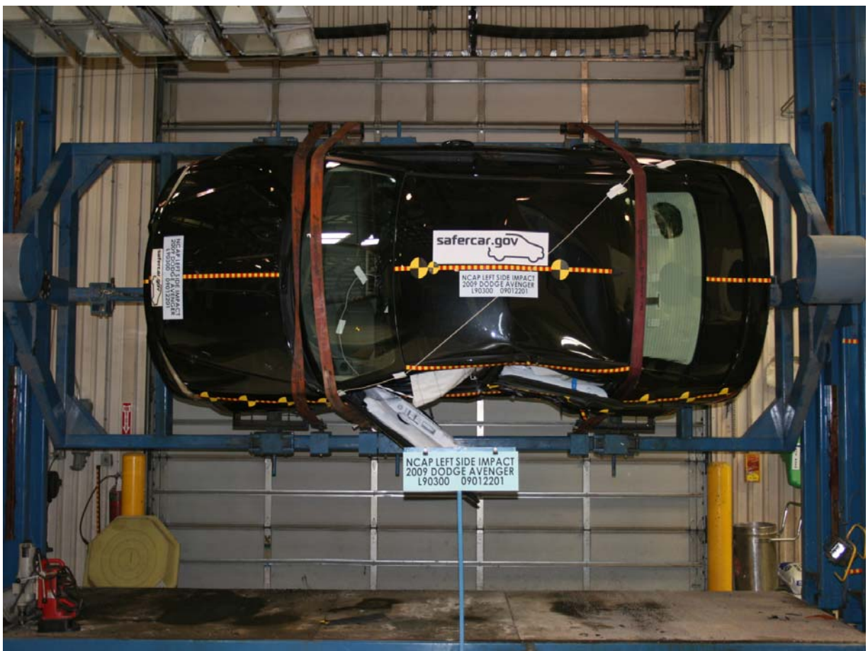
Vehicle on Rollover Device (90 Degrees)
