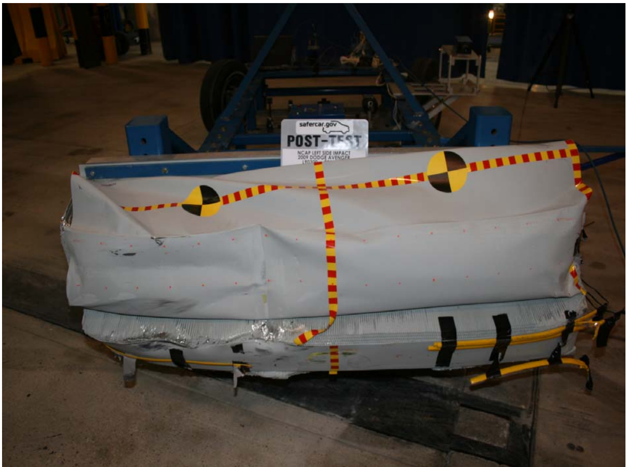
Post-Test Front View of Deformable Barrier
