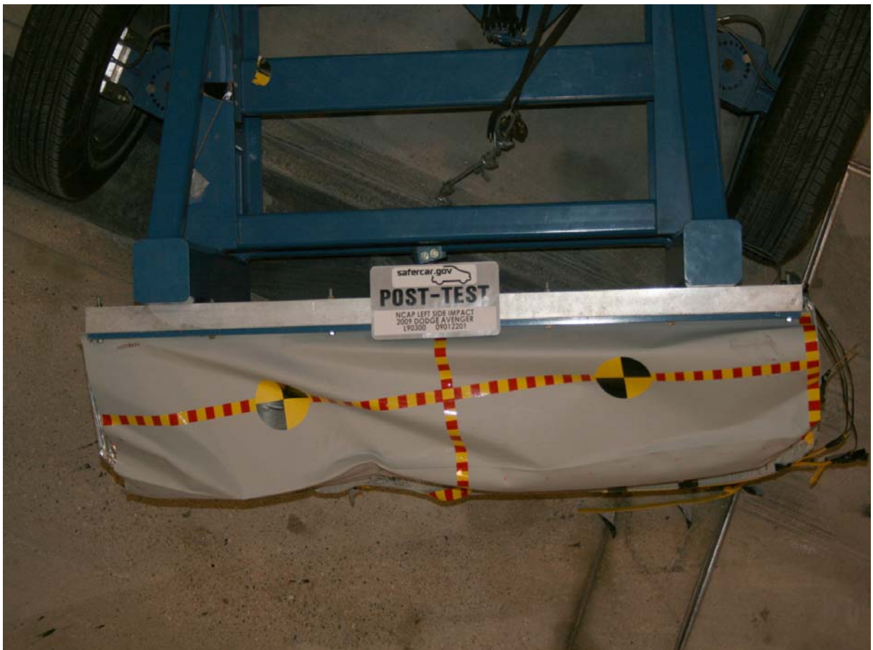
Post-Test Top View of Deformable Barrier
