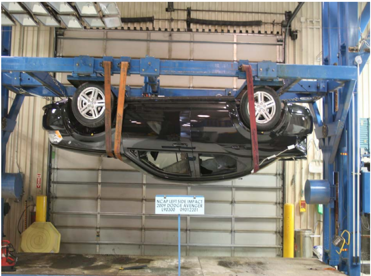
Vehicle on Rollover Device (180 Degrees)
