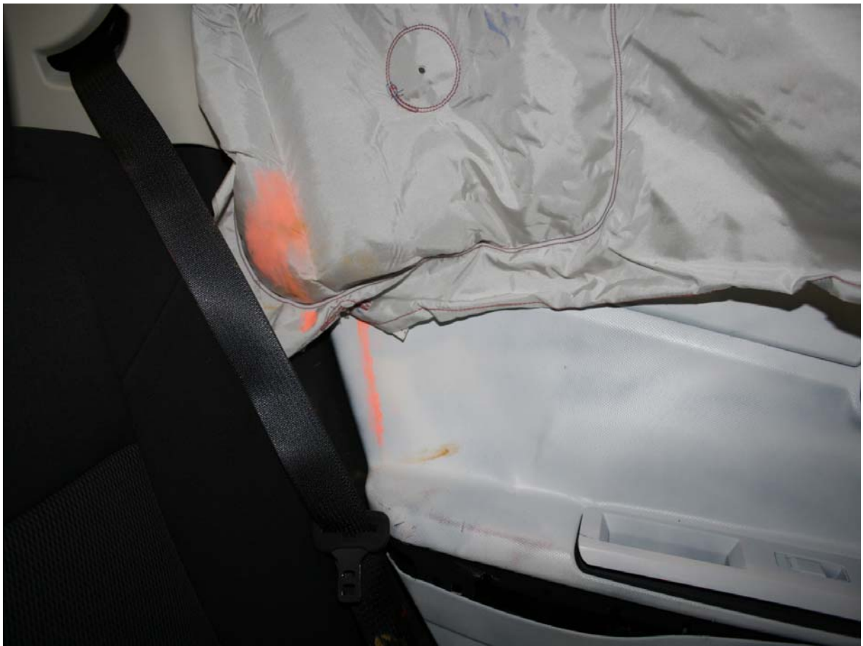
Post-Test Passenger Dummy Upper Torso Contact
