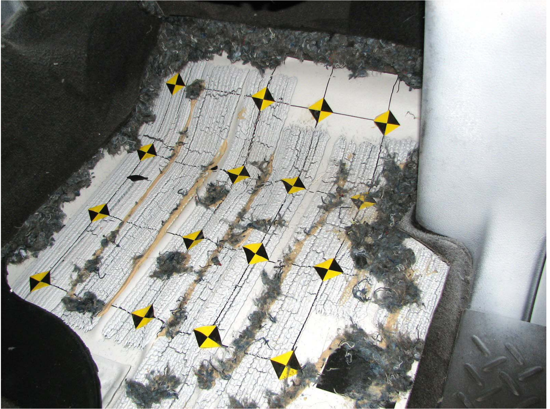
Figure A-55: Post-Test Passenger Side Floor Pan
