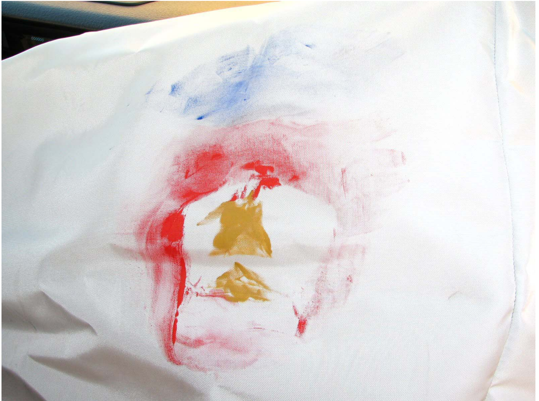
Figure A-57: Post-Test Passenger Dummy Airbag Contact
