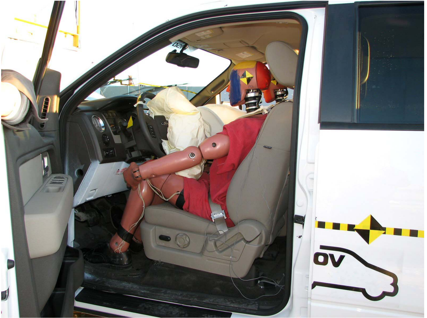
Figure A-35: Post-Test Driver Dummy (Door Open)
