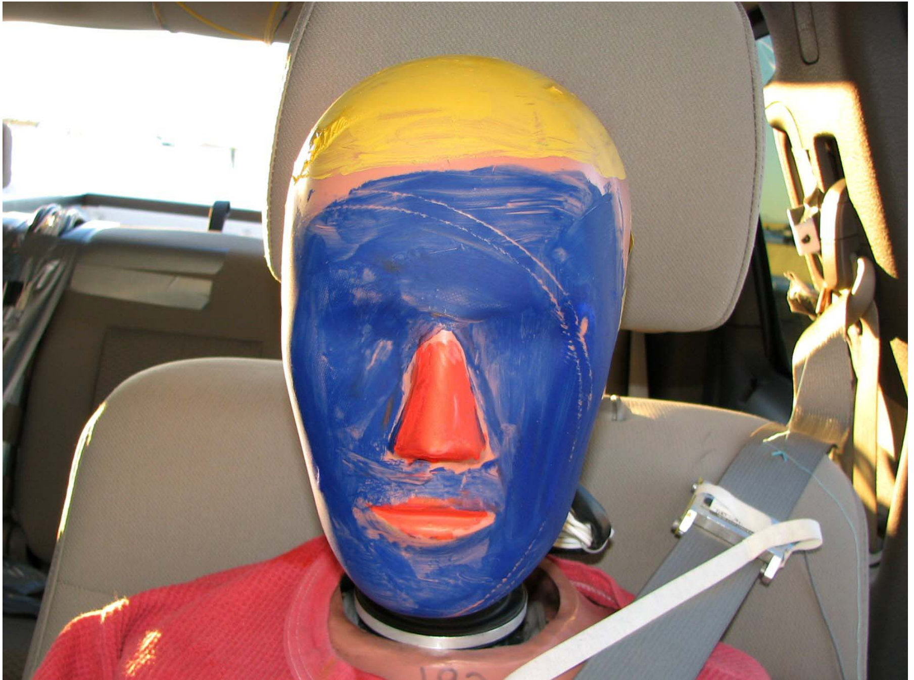
Figure A-42: Post-Test Driver Dummy Head
