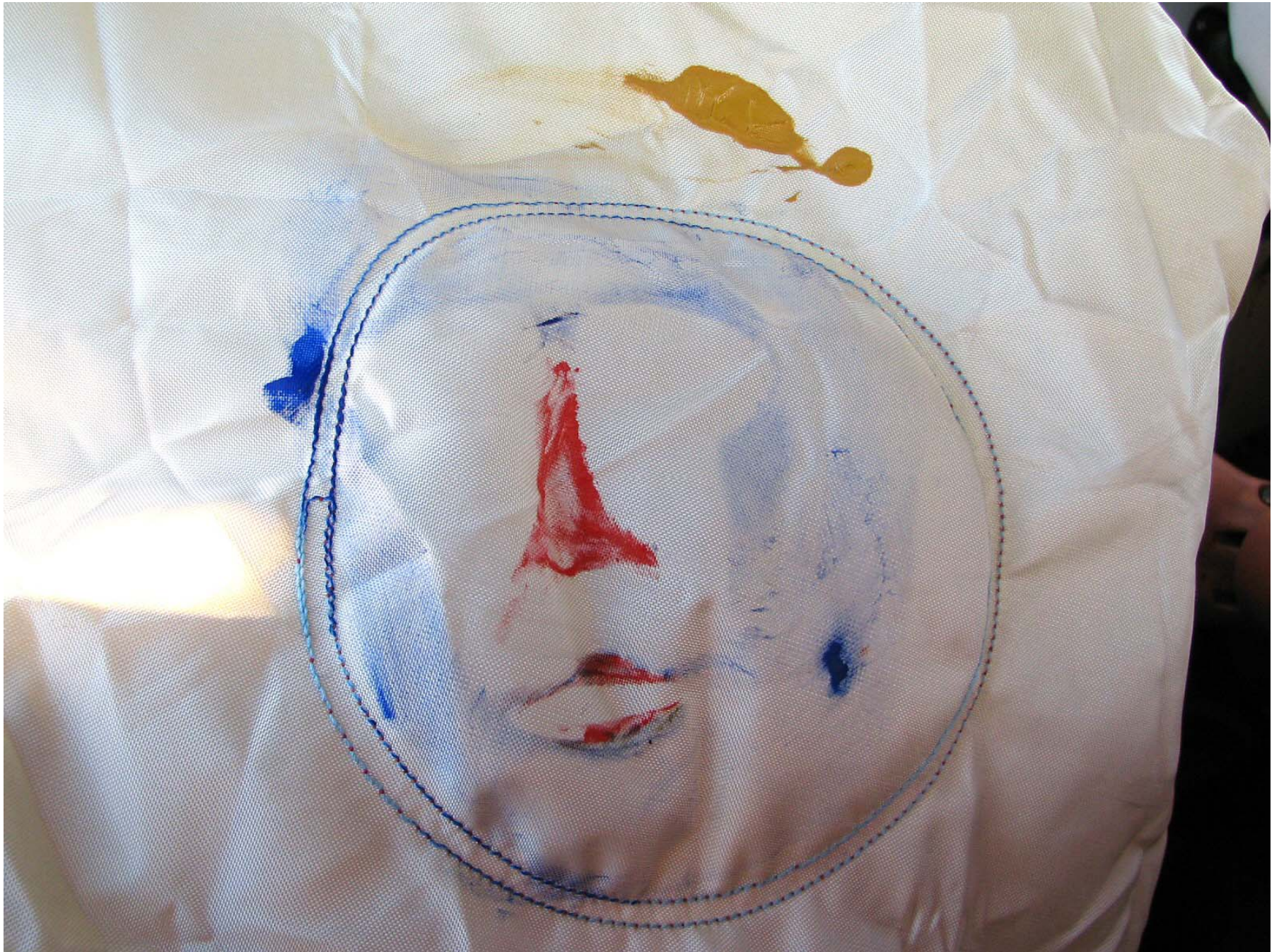
Figure A-43: Post-Test Driver Dummy Airbag Contact
