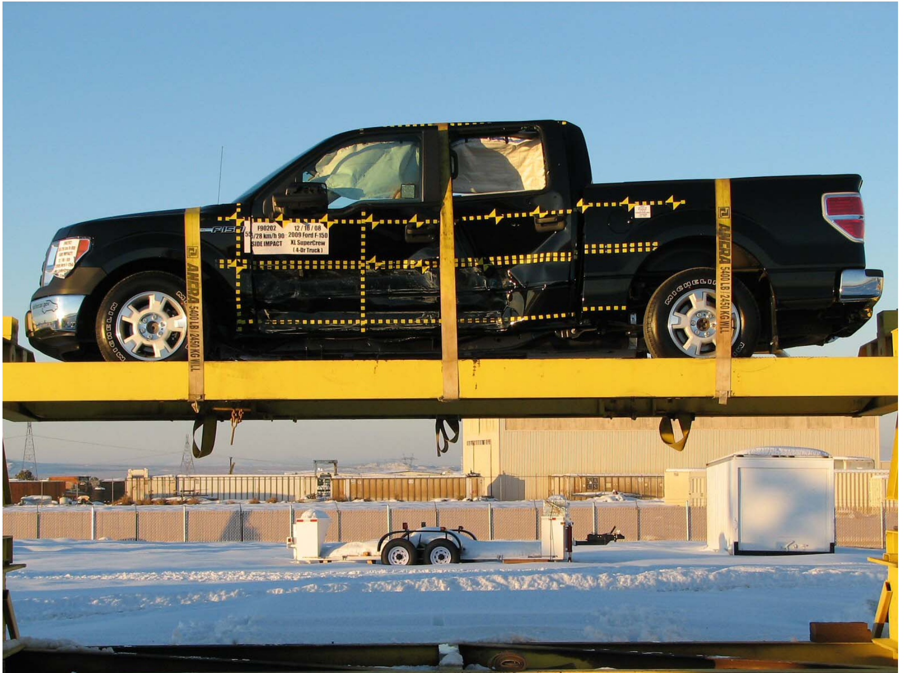
Figure A-61: Vehicle on Rollover Device (0°)
