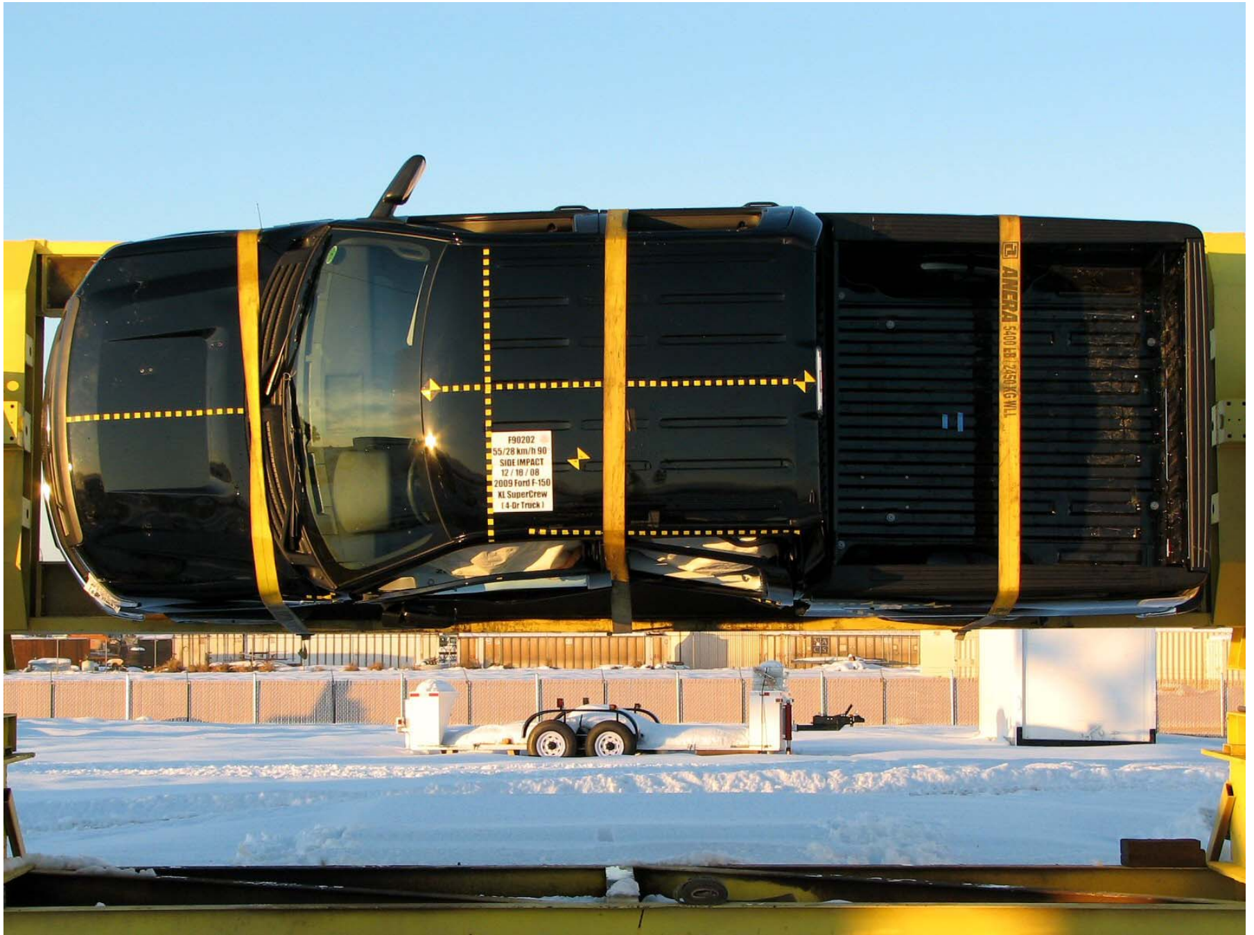
Figure A-62: Vehicle on Rollover Device (90°)
