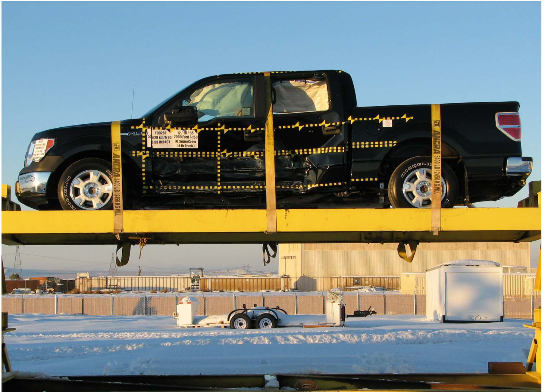
Figure A-65: Vehicle on Rollover Device (360°)
