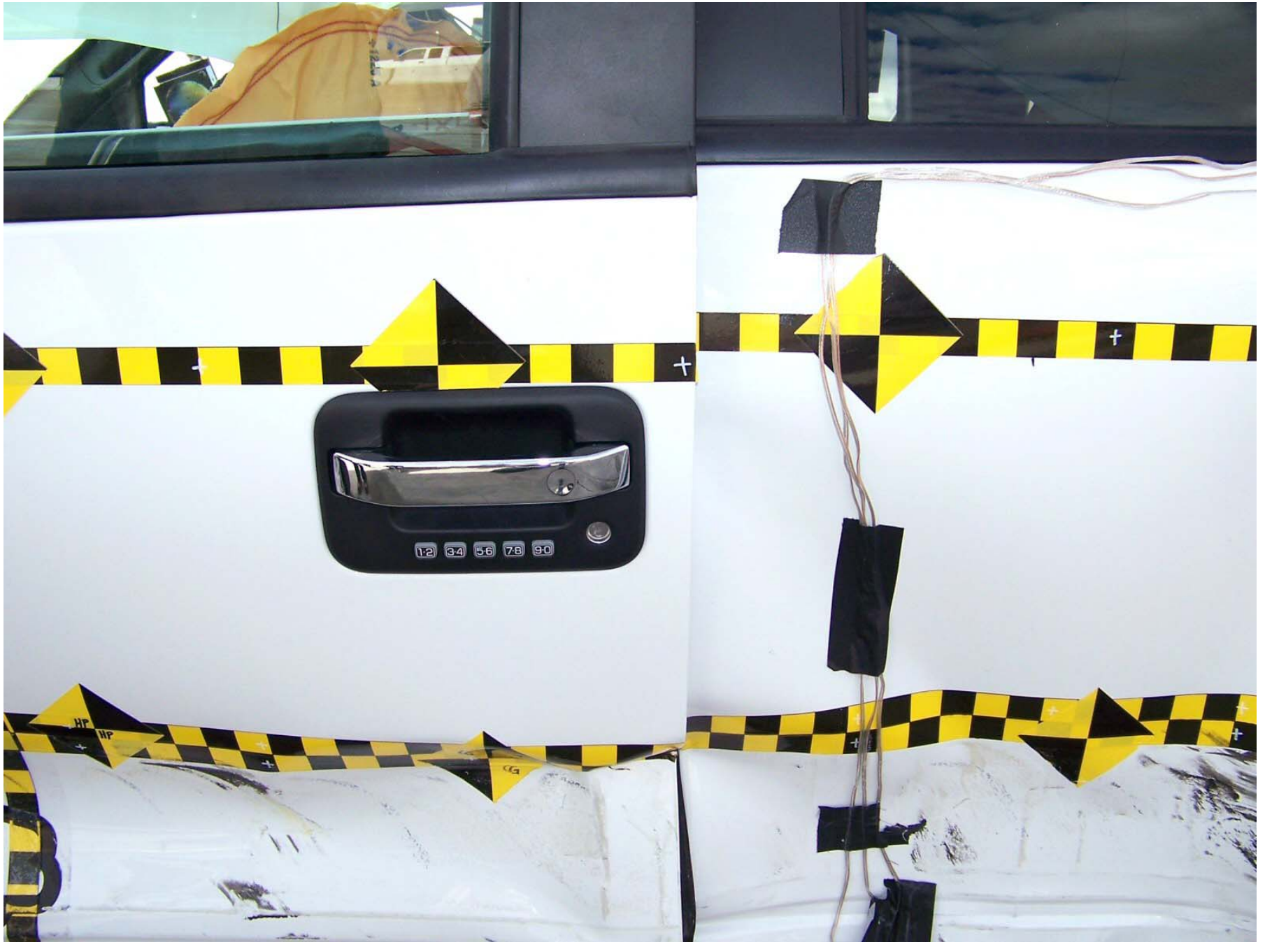
Figure A-32: Post-Test Left Front Door
