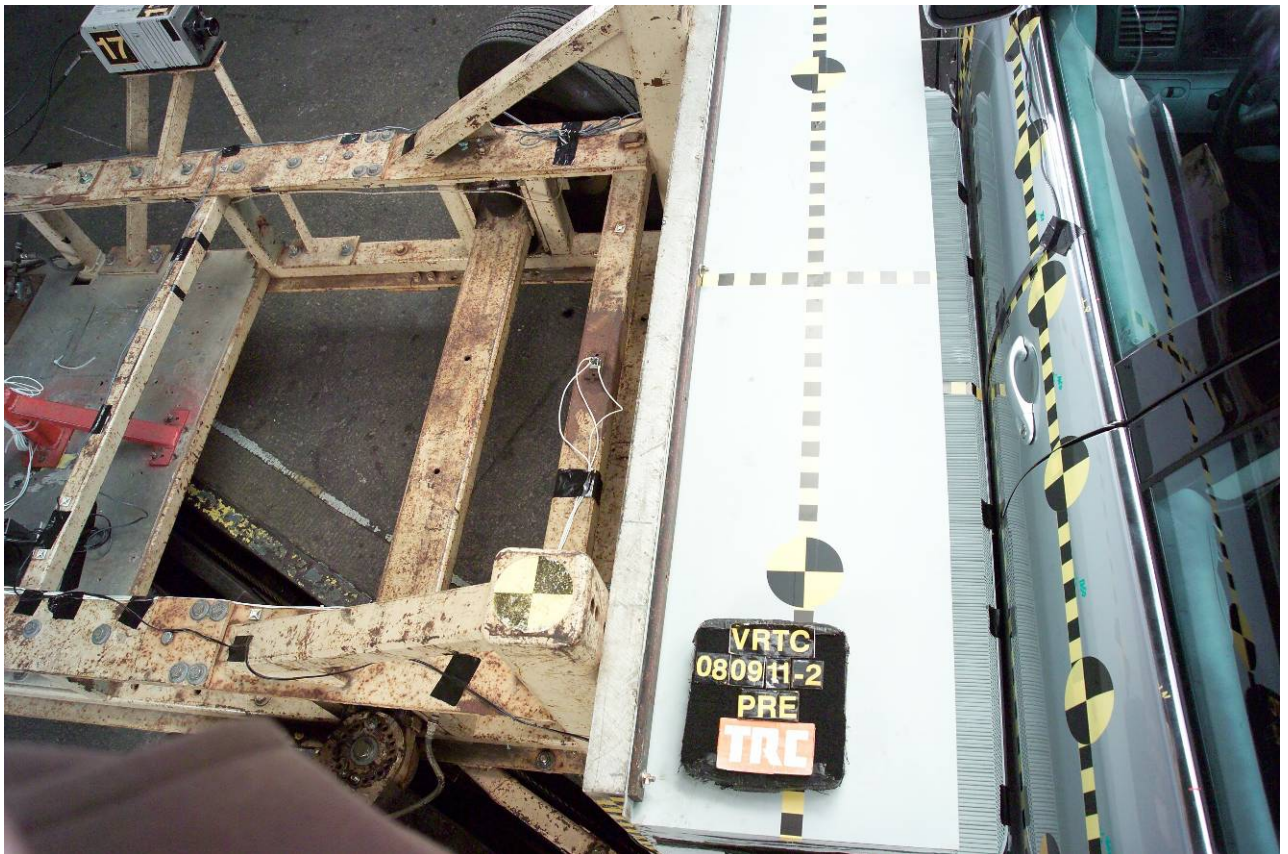
Figure A-39 Pre-Test MDB Alignment Overhead View
