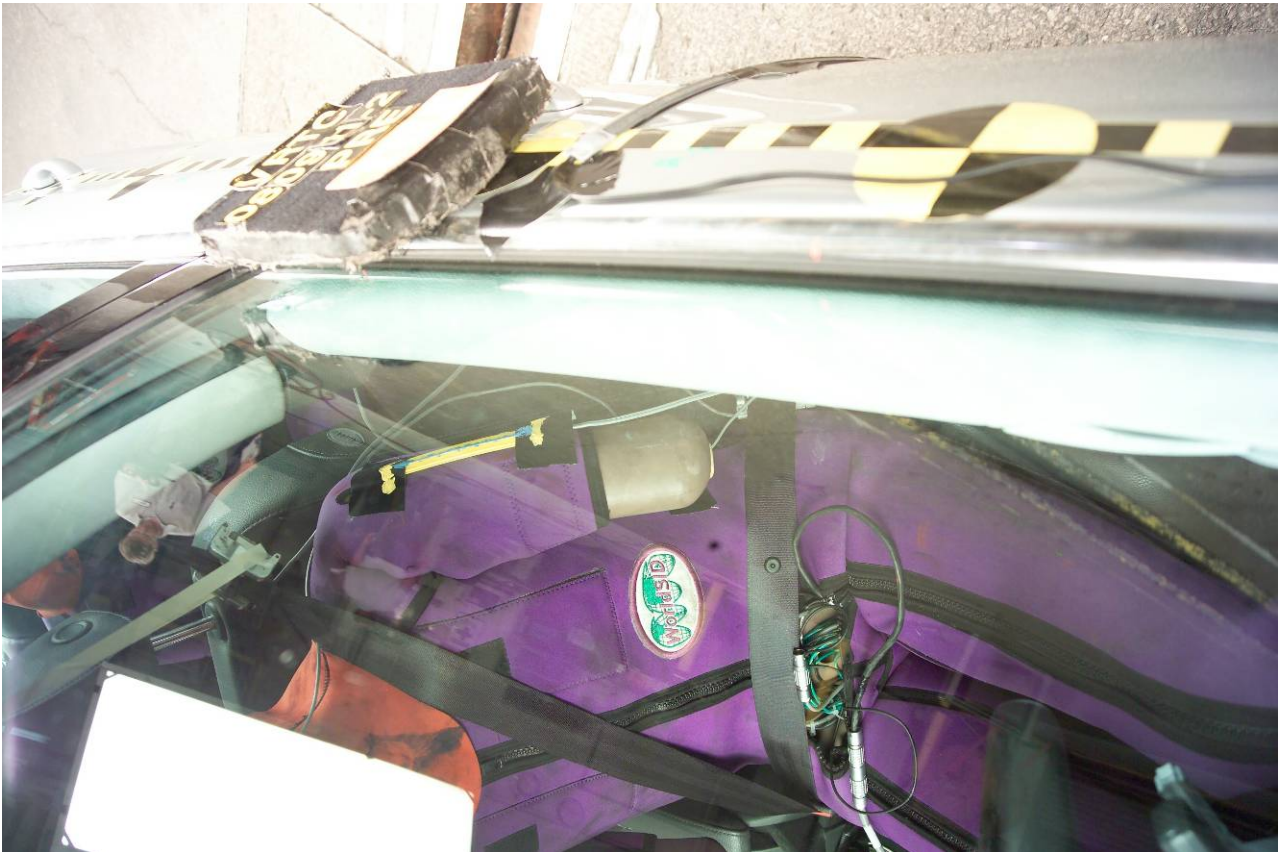
Figure A-56 Pre-Test Passenger Dummy and Door Clearance View
