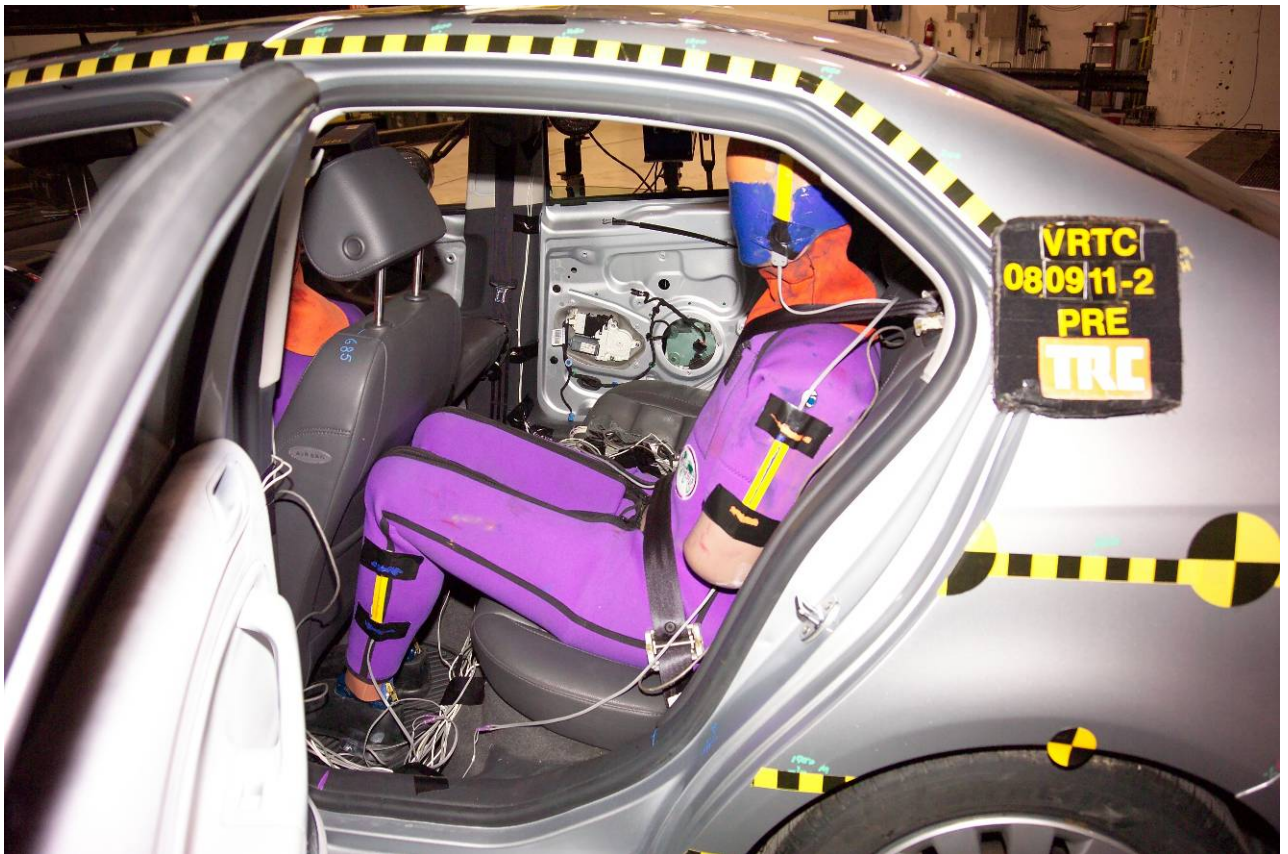
Figure A-58 Pre-Test Passenger Dummy Showing Belts, Chalking, and Contact Switches
