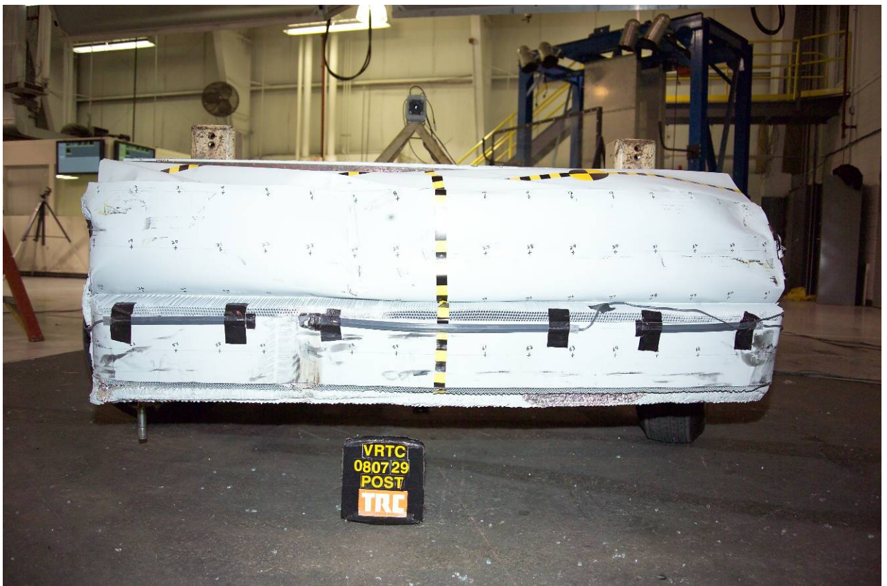
Figure A-26 Post-Test MDB Front View with Contact Switches in Place
