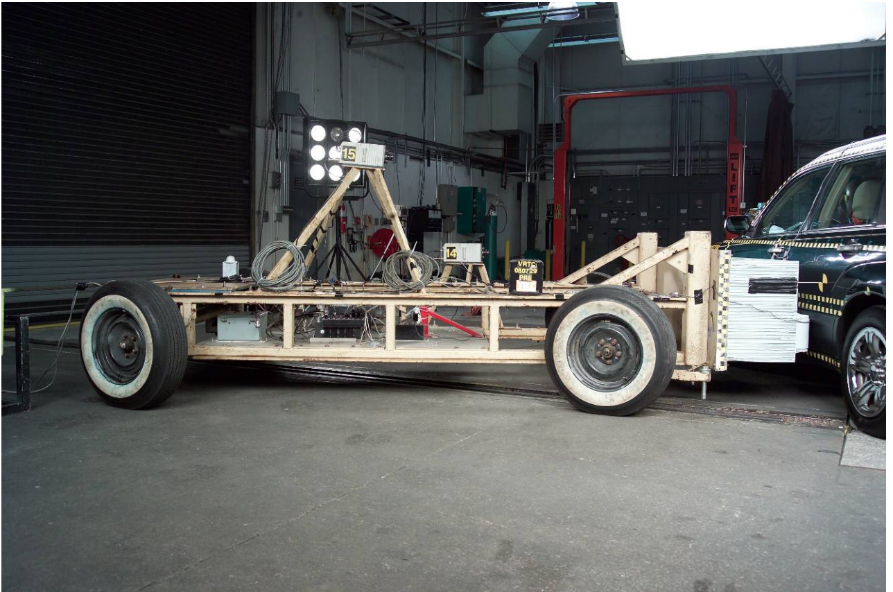
Figure A-33 Pre-Test MDB Right Side Overall View
