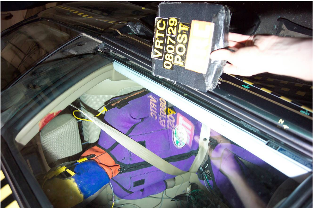
Figure A-53 Post-Test Passenger Dummy and Door Clearance View
