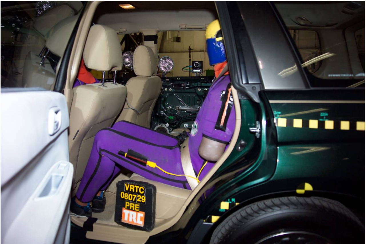
Figure A-54 Pre-Test Passenger Dummy Showing Belts, Chalking, and Contact Switches
