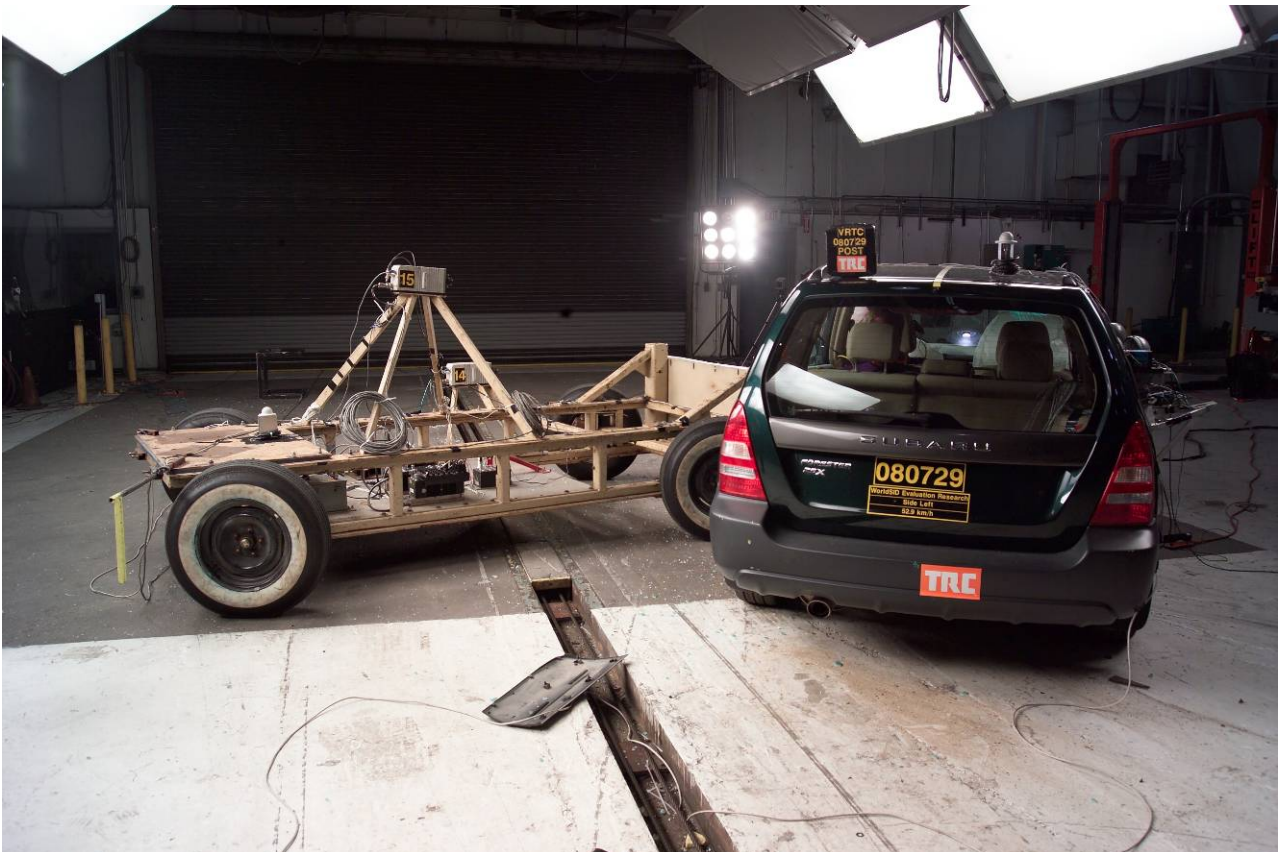
Figure A-30 Post-Test MDB with Vehicle Right Side Overall View
