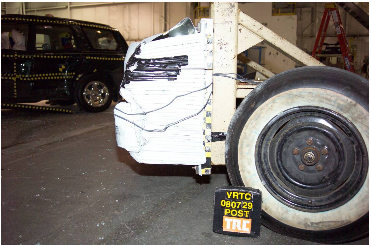
Figure A-20 Post-Test MDB Face Left Side View
