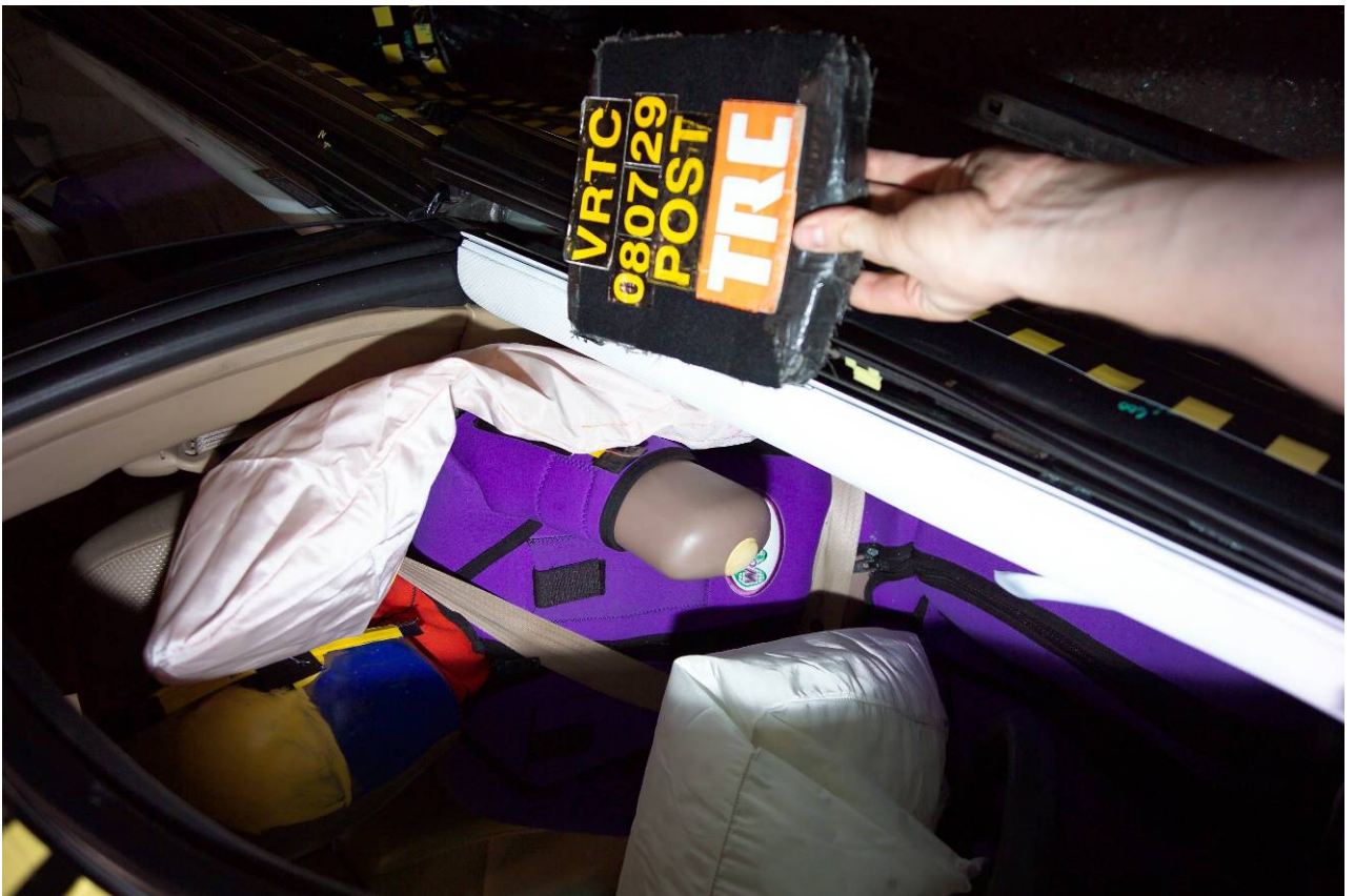
Figure A-41 Post-Test Driver Dummy and Door Clearance View
