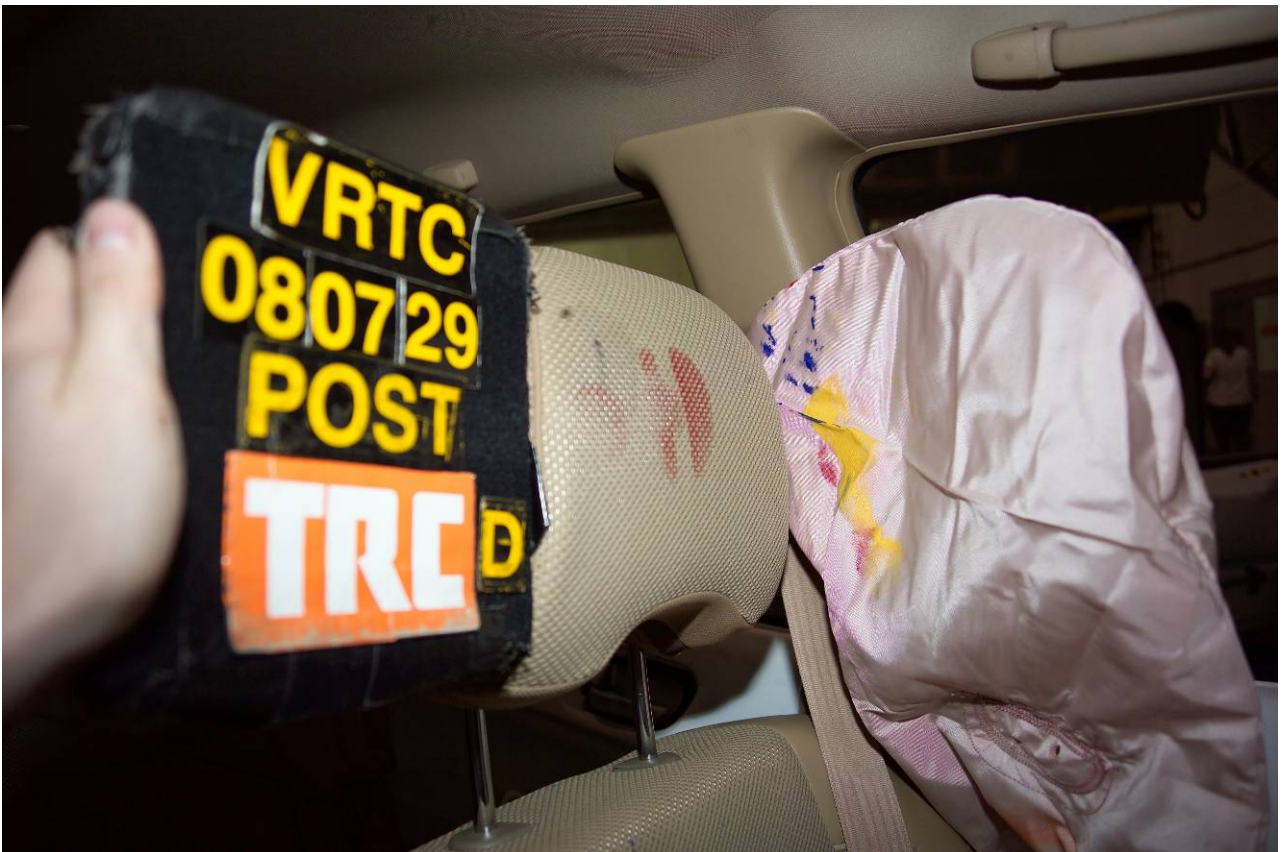
Figure A-46 Post-Test Driver Dummy Head Contact View
