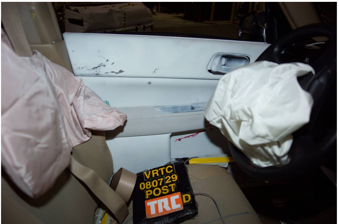
Figure A-44 Post-Test Driver Door Panel View
