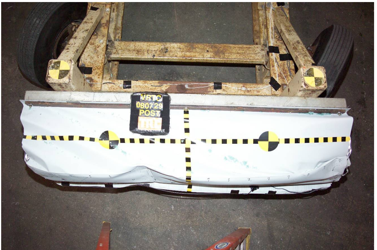
Figure A-24 Post-Test MDB Face Overhead View
