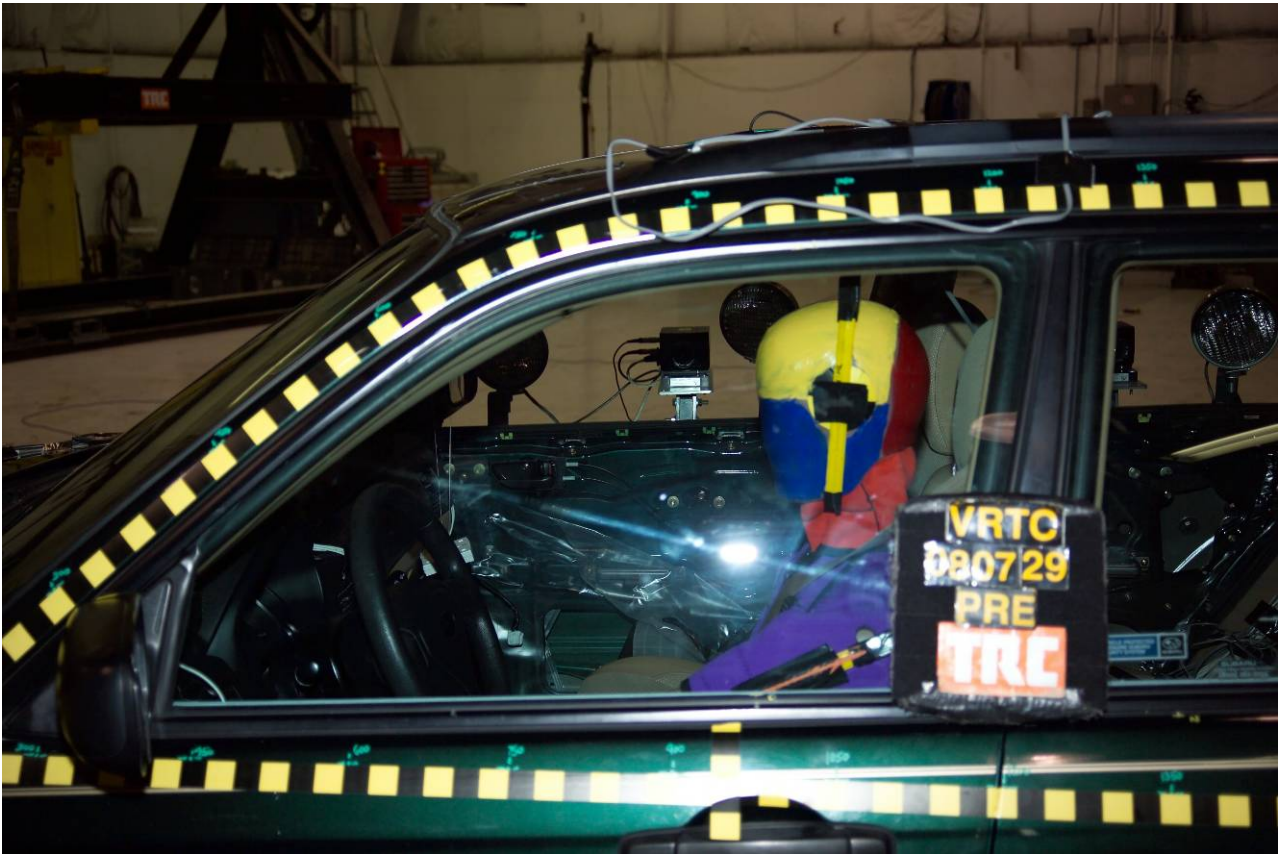
Figure A-36 Pre-Test Driver Dummy Side View
