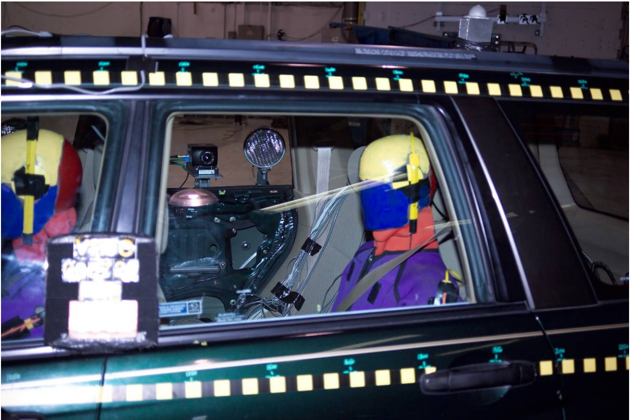
Figure A-48 Pre-Test Passenger Dummy Side View
