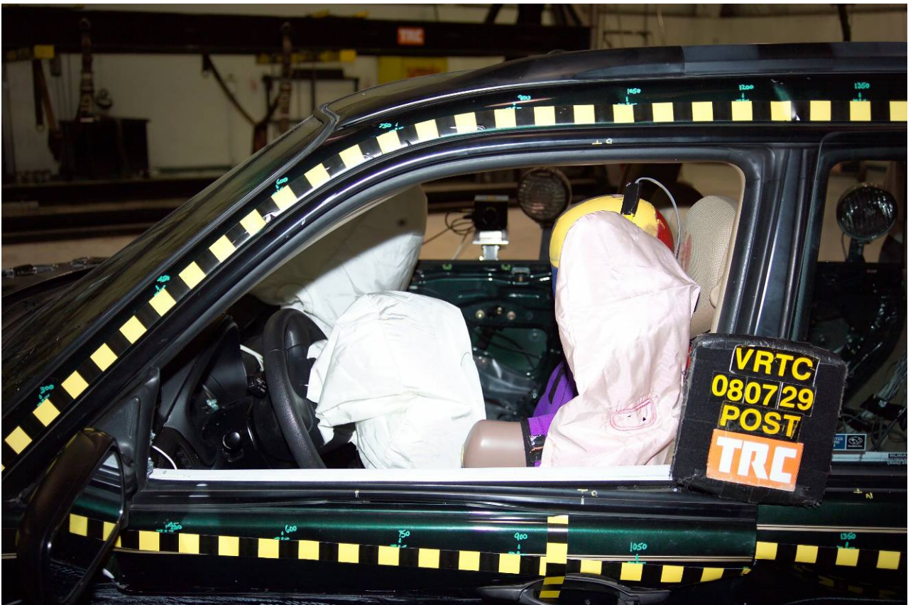
Figure A-37 Post-Test Driver Dummy Side View
