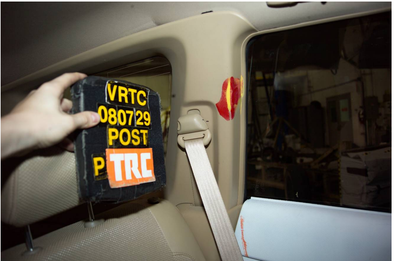
Figure A-58 Post-Test Passenger Dummy Head Contact View
