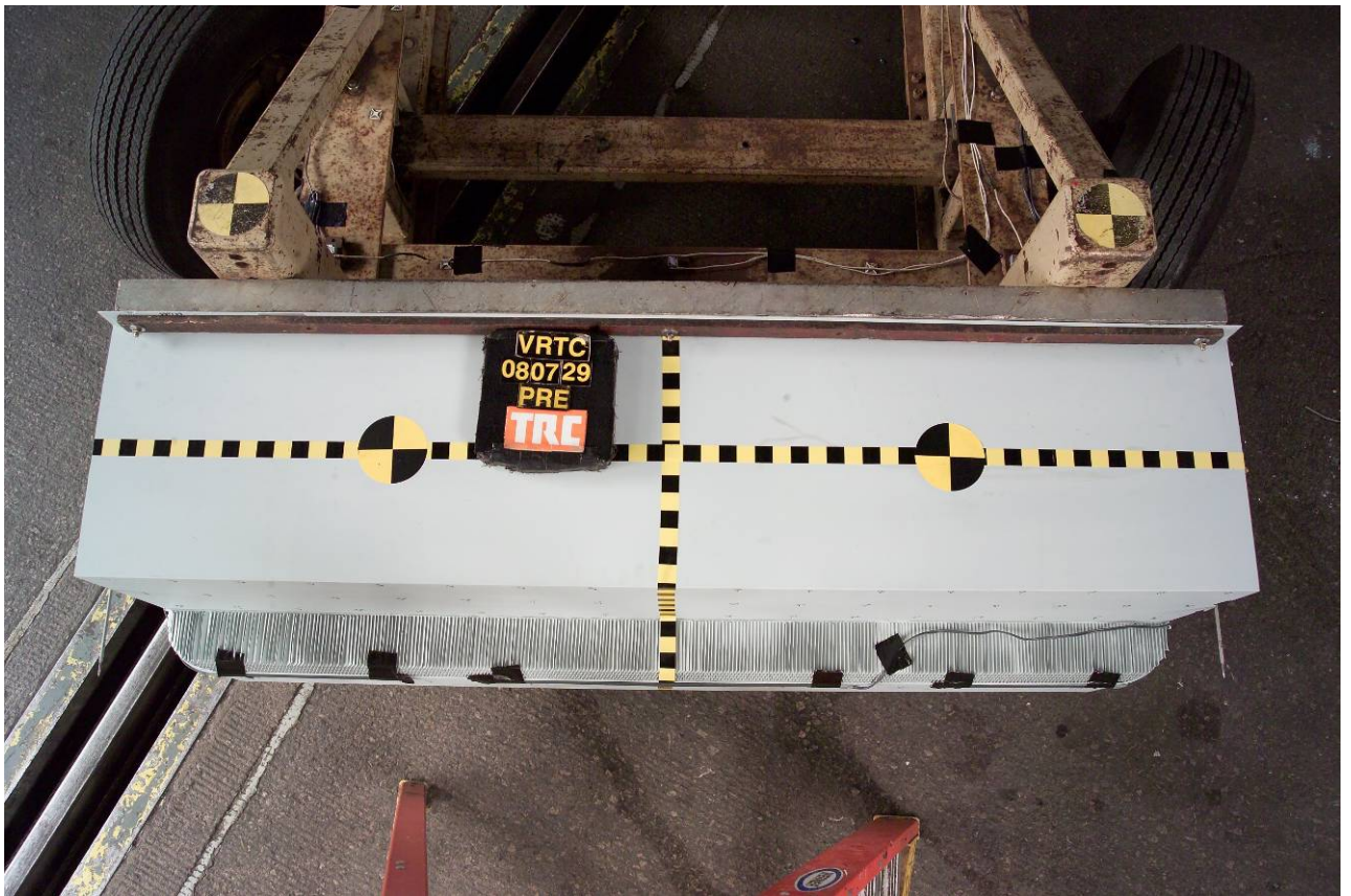
Figure A-23 Pre-Test MDB Face Overhead View
