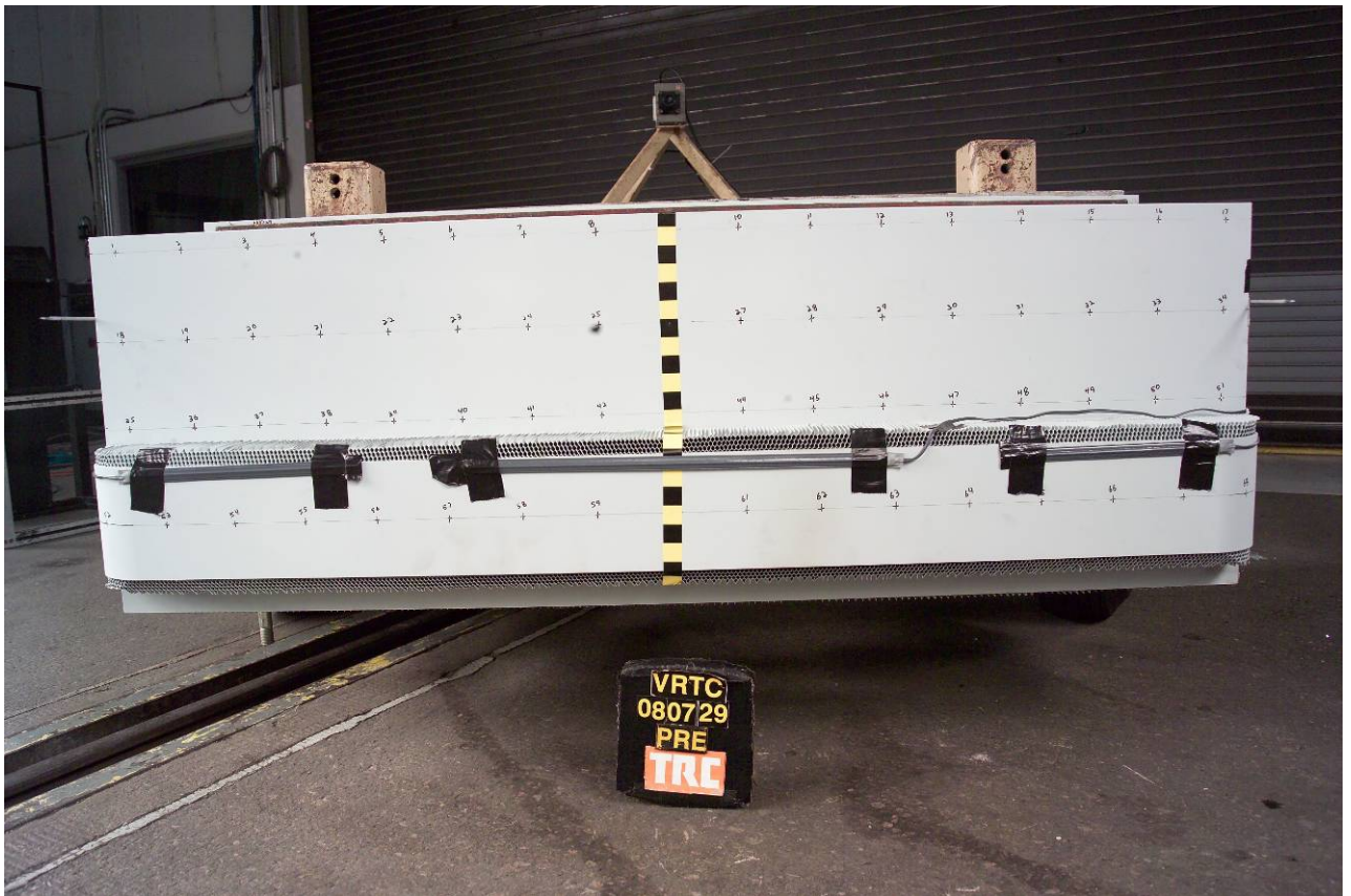
Figure A-25 Pre-Test MDB Front View with Contact Switches in Place
