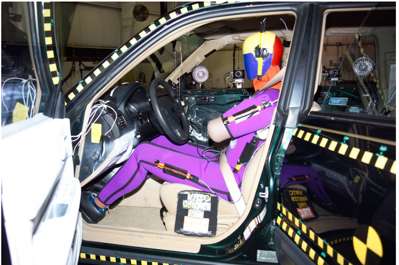
Figure A-42 Pre-Test Driver Dummy Showing Belts, Chalking, and Contact Switches
