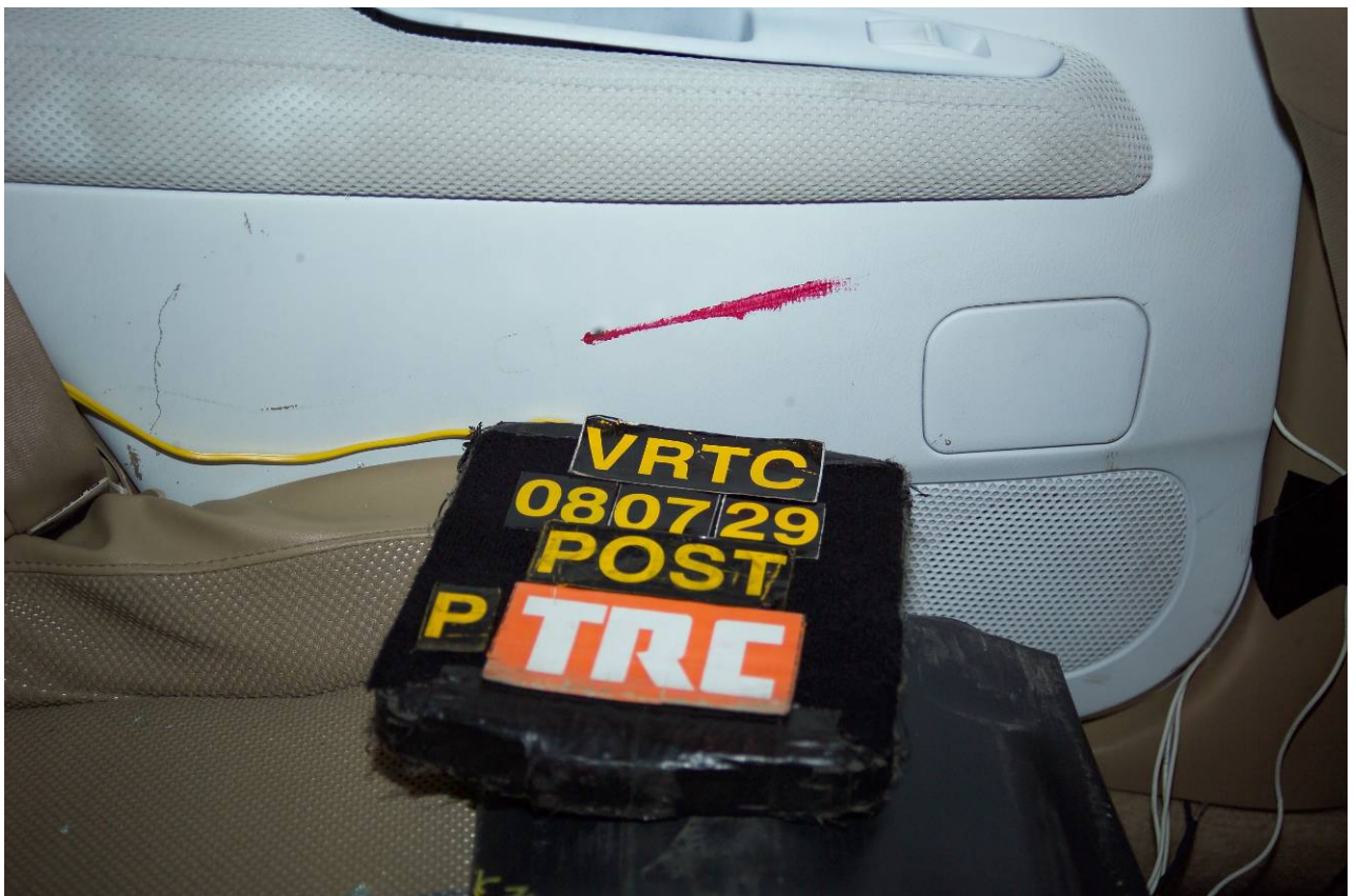
Figure A-60 Post-Test Passenger Dummy Torso Contact - View 2
