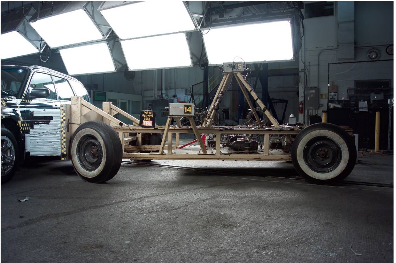
Figure A-31 Pre-Test MDB Left Side Overall View
