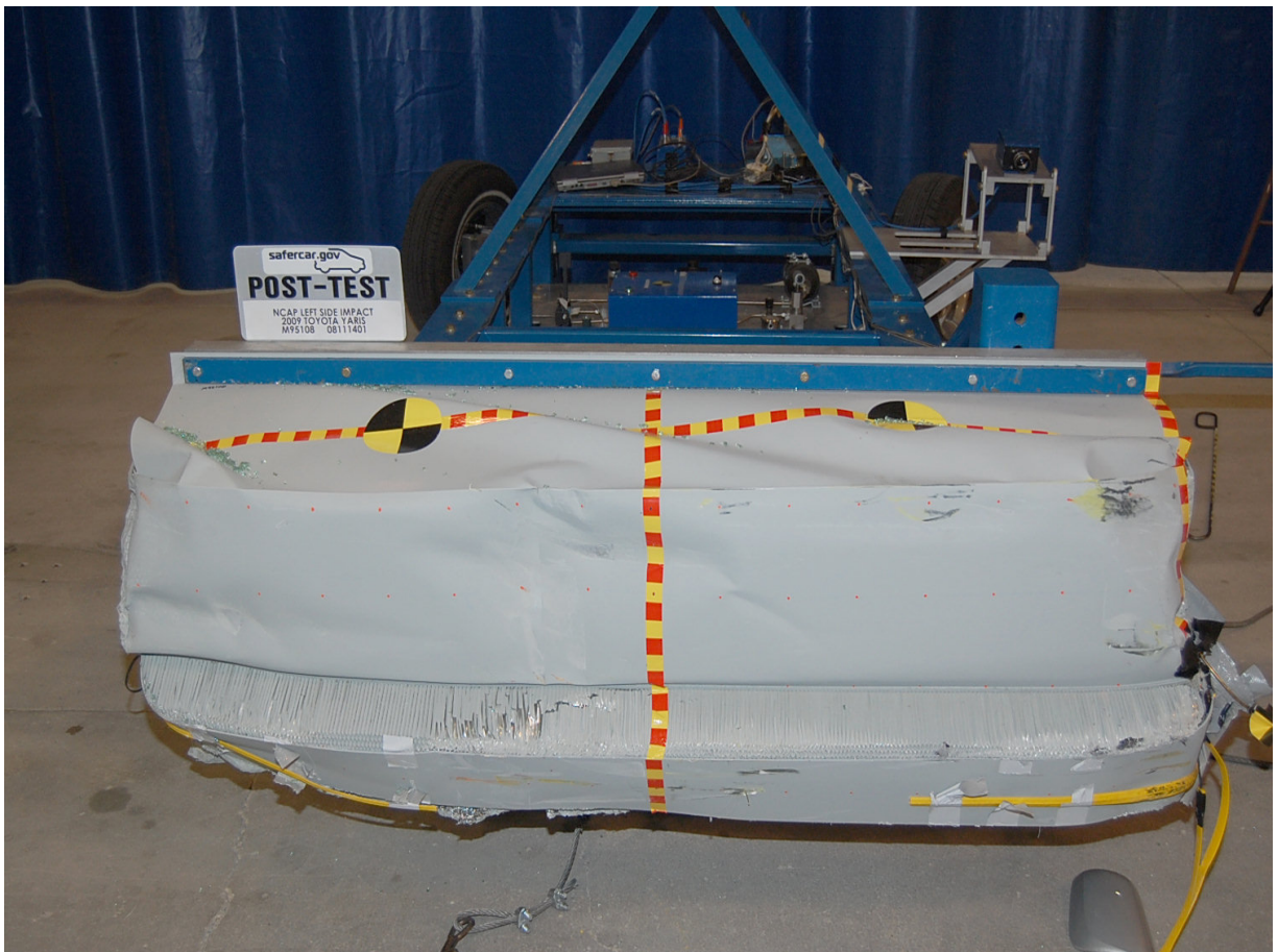
Post-Test Front View of Deformable Barrier
