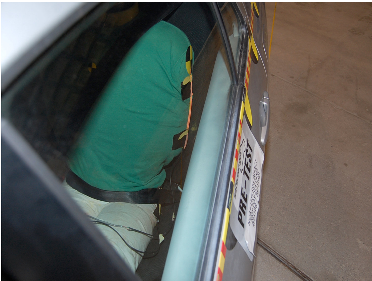
Pre-Test Passenger Dummy Clearance From Door
