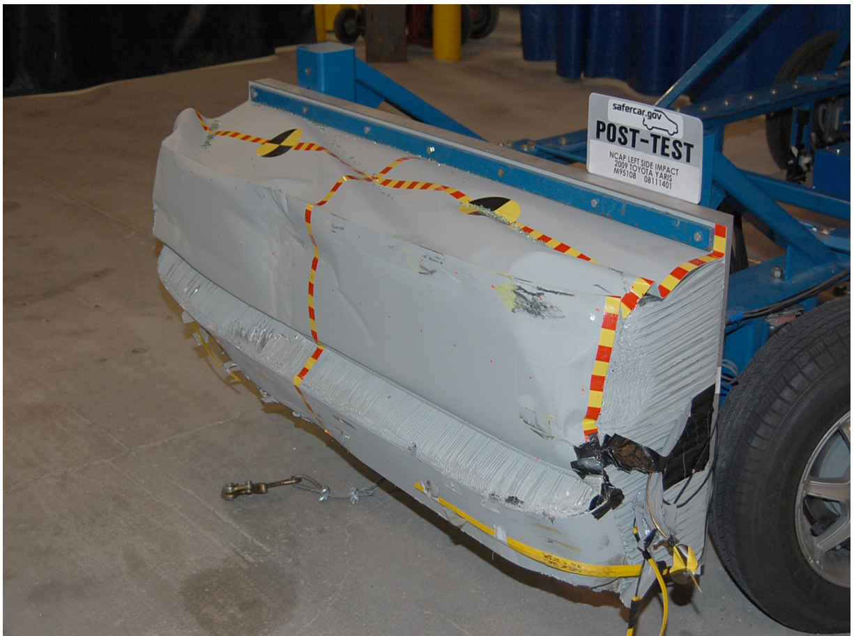
Post-Test Left Side View of Deformable Barrier
