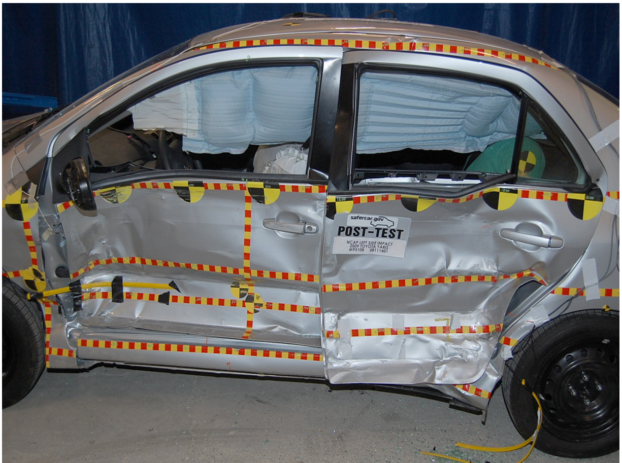
Post-Test Left Side Impact Close-up
