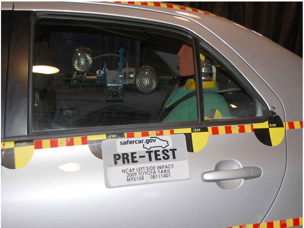
Pre-Test Passenger Dummy (Through Window)
