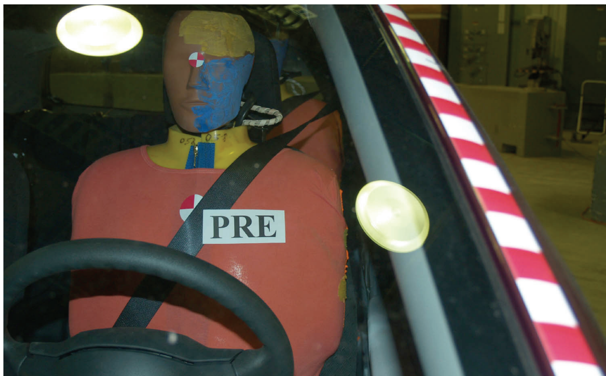
Figure A-33: Pre test driver shoulder clearance
