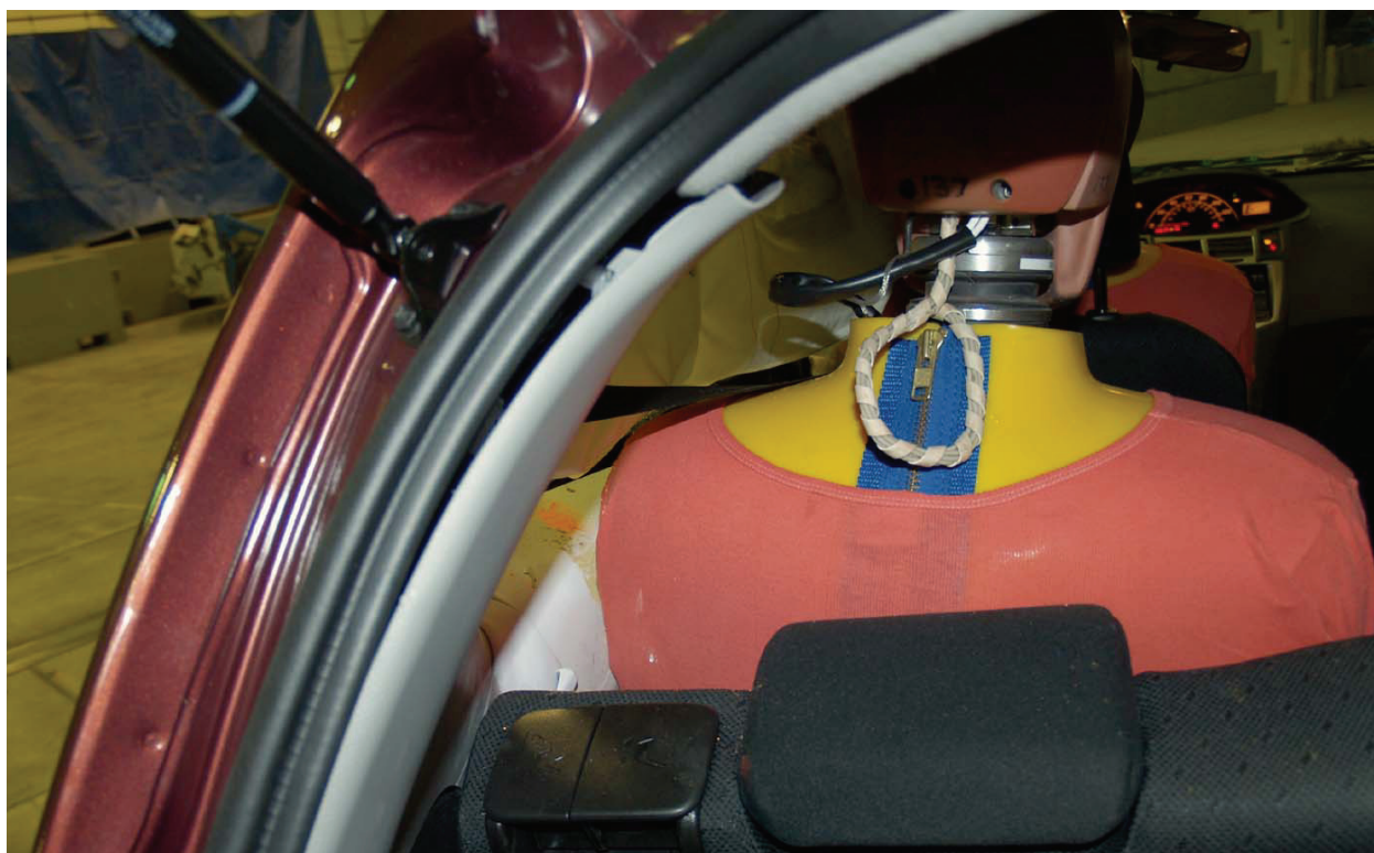
Figure A-42 Post test passenger shoulder clearance
