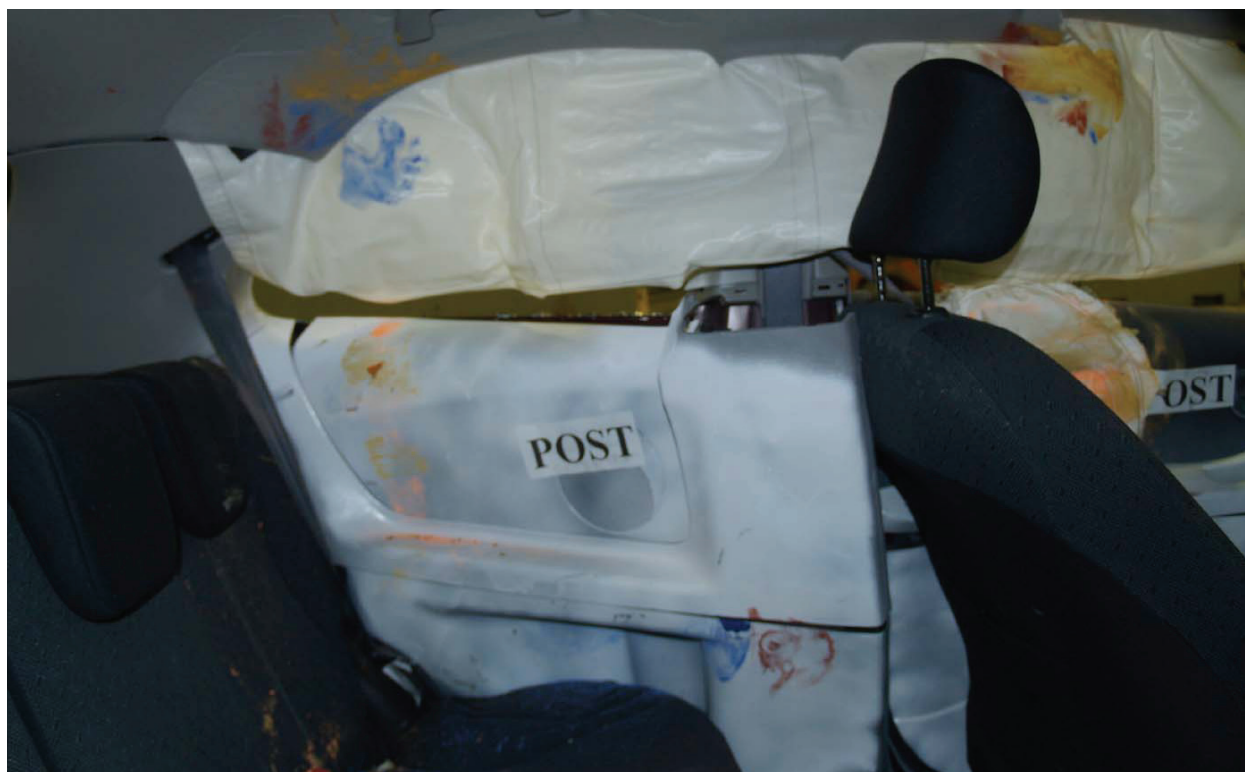
Figure A-45: Post test passenger contact locations (1)
