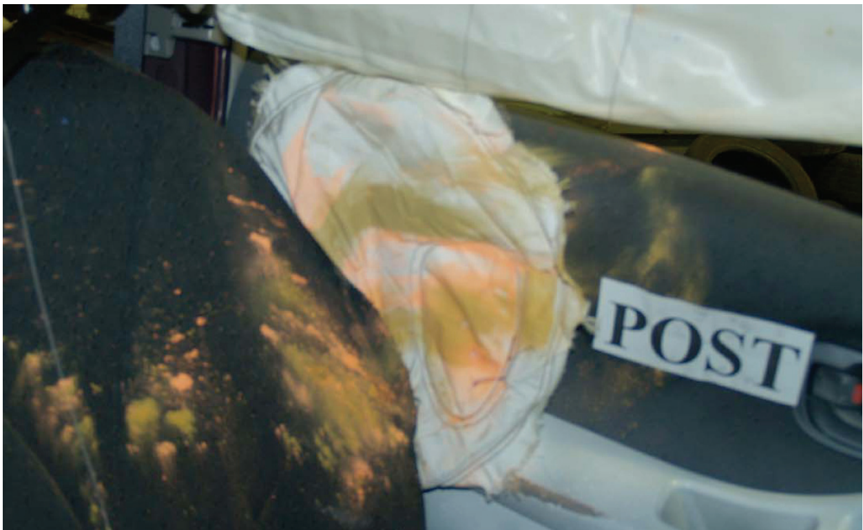
Figure A-38: Post test driver contact locations (2)
