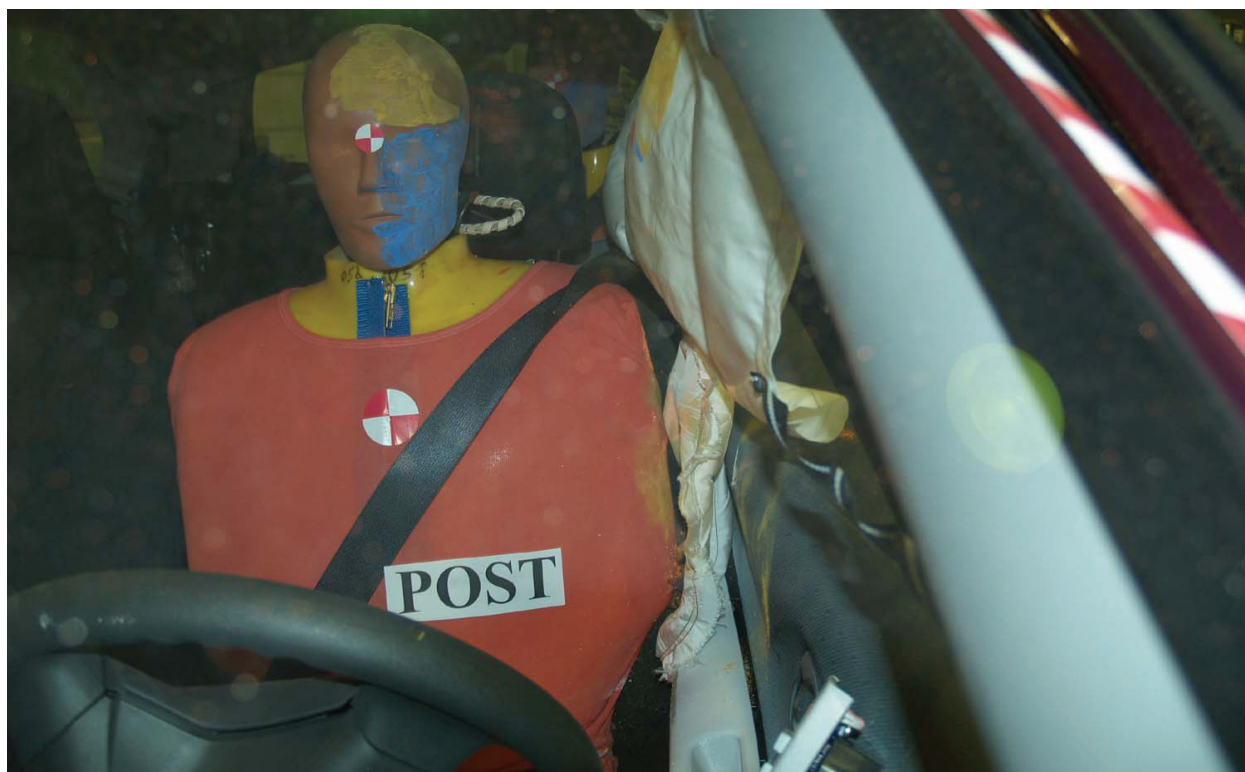
Figure A-34: Post test driver shoulder clearance
