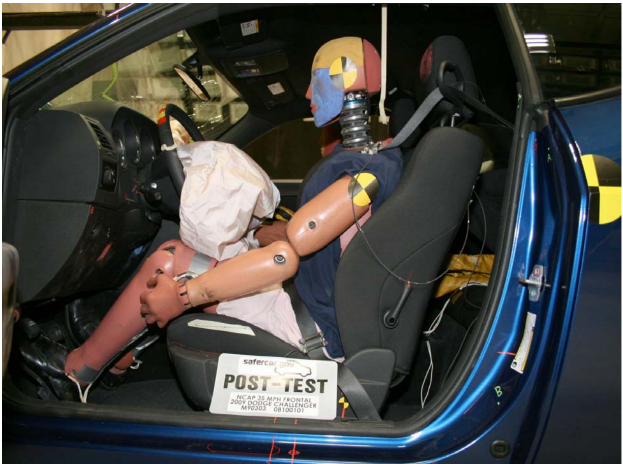
Post-Test Driver Dummy (Door Open)
