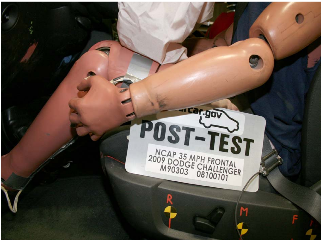
Post-Test Driver Side Knee Bolster
