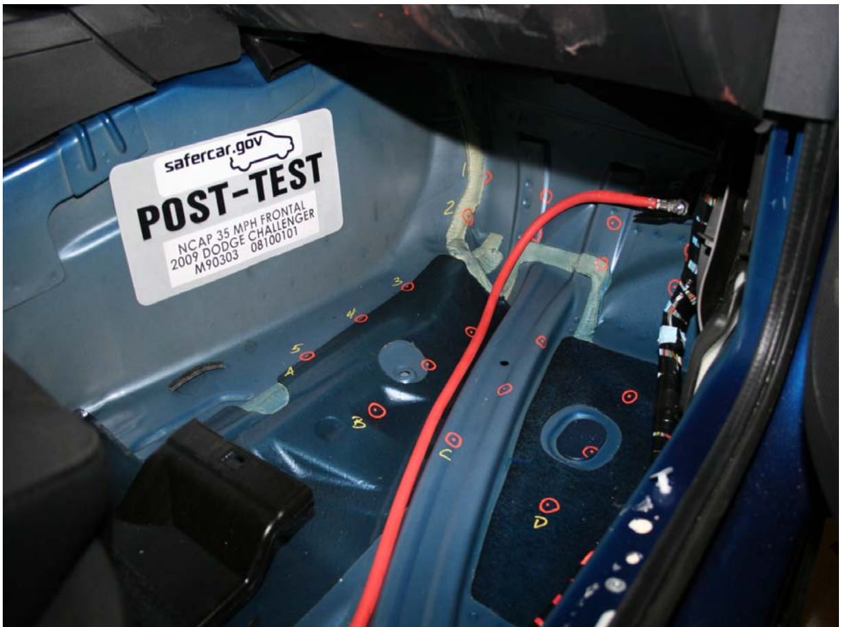
Post-Test Passenger Side Floor Pan
