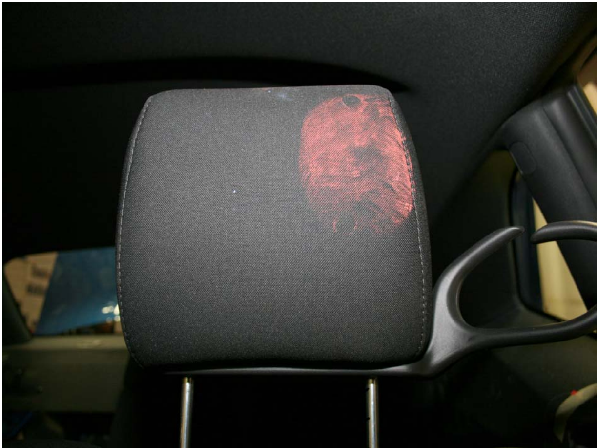
Post-Test Driver Dummy Head Contact
