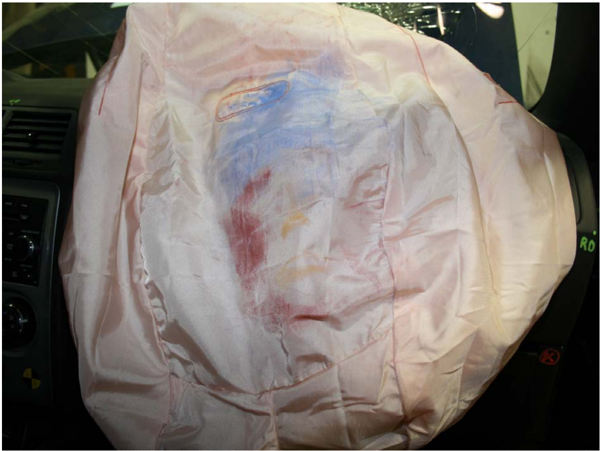
Post-Test Passenger Dummy Airbag Contact
