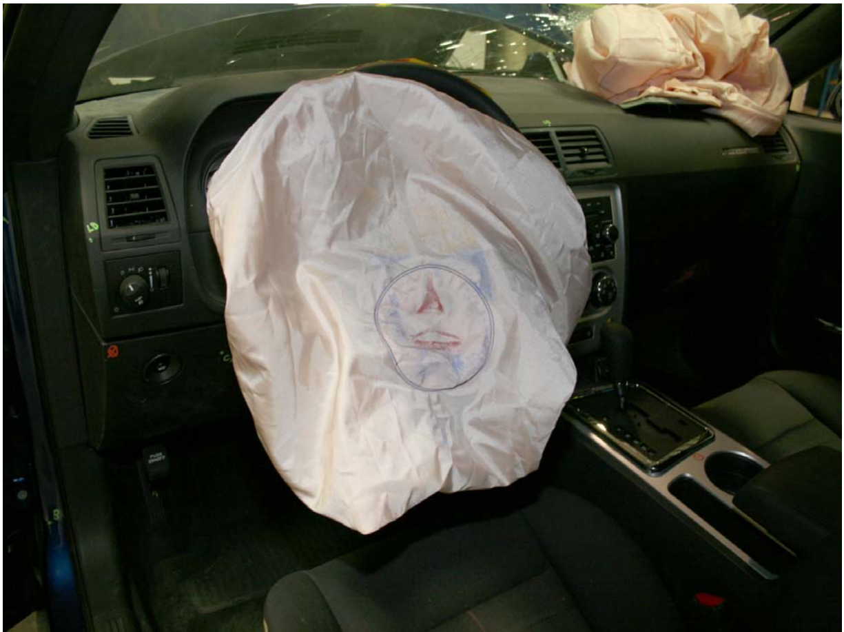
Post-Test Driver Dummy Airbag Contact
