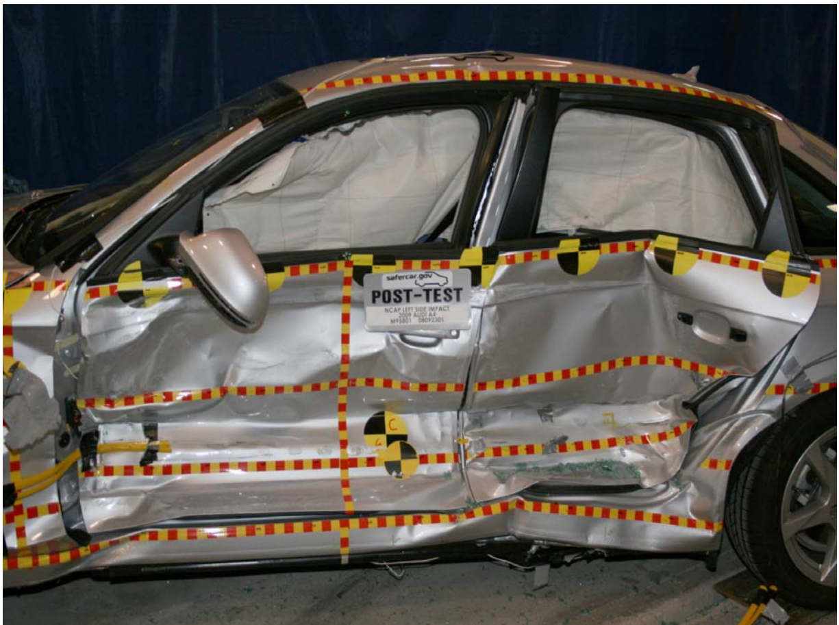
Post-Test Left Side Impact Close-up
