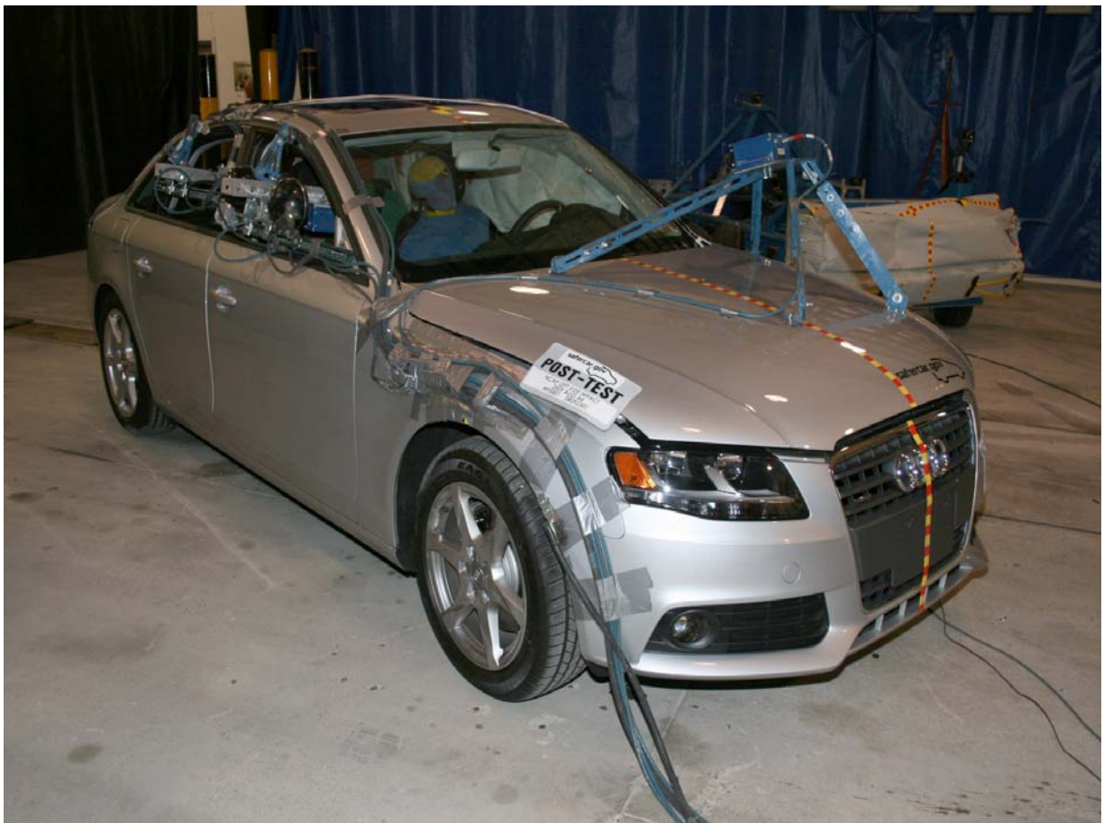
Post-Test Right Front 3/4 View
