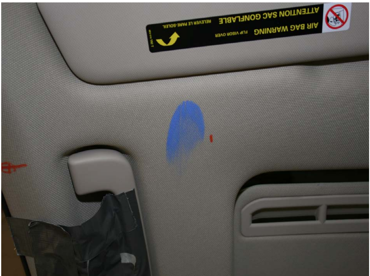
Post-Test Passenger Dummy Head Contact (headliner)
