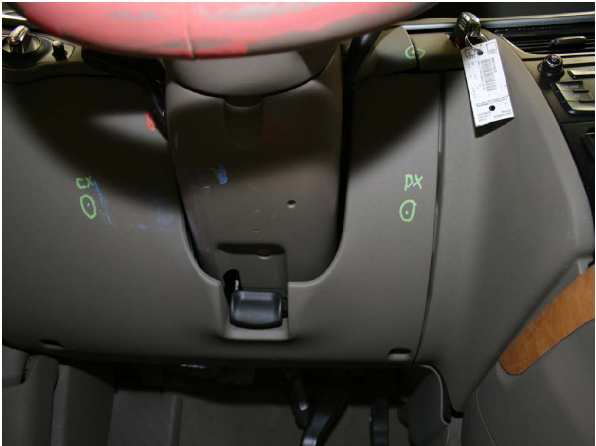
Post-Test Driver Dummy Right Knee Contact
