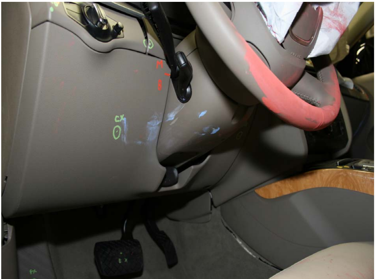
Post-Test Driver Dummy Left Knee Contact
