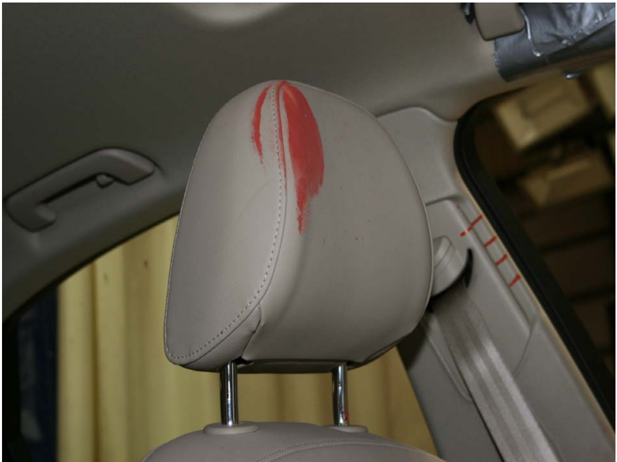
Post-Test Driver Dummy Head Contact
