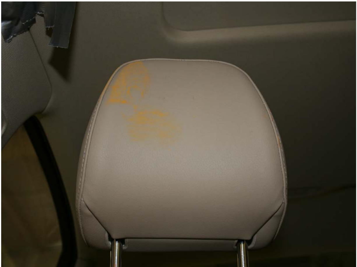
Post-Test Passenger Dummy Head Contact (headrest)
