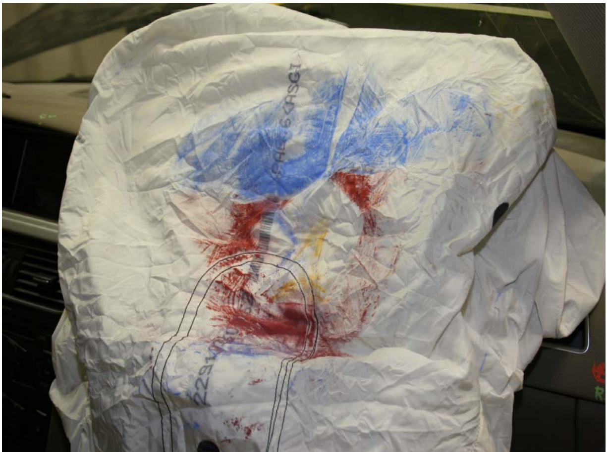
Post-Test Passenger Dummy Airbag Contact
