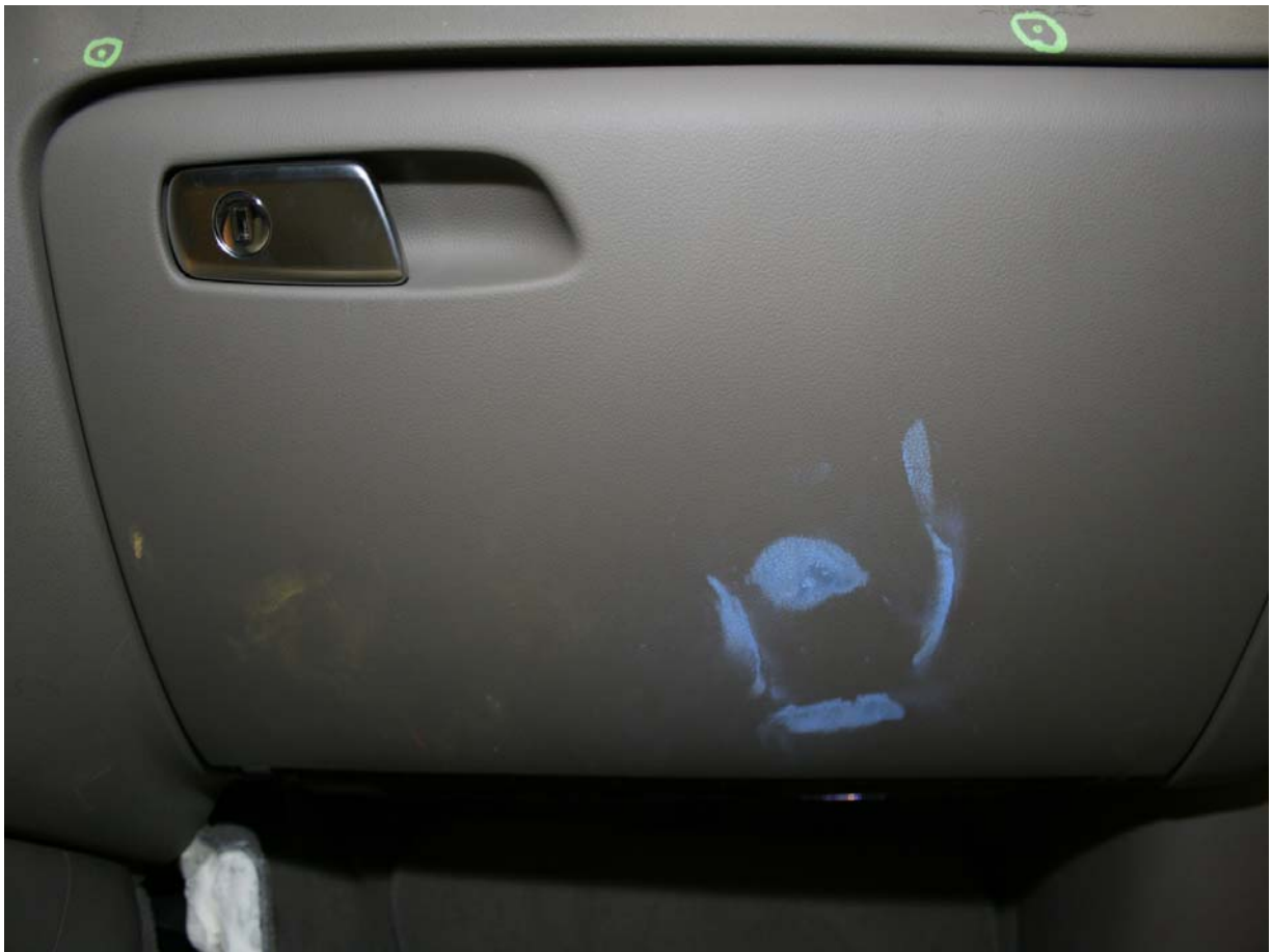
Post-Test Passenger Dummy Knee Contact
