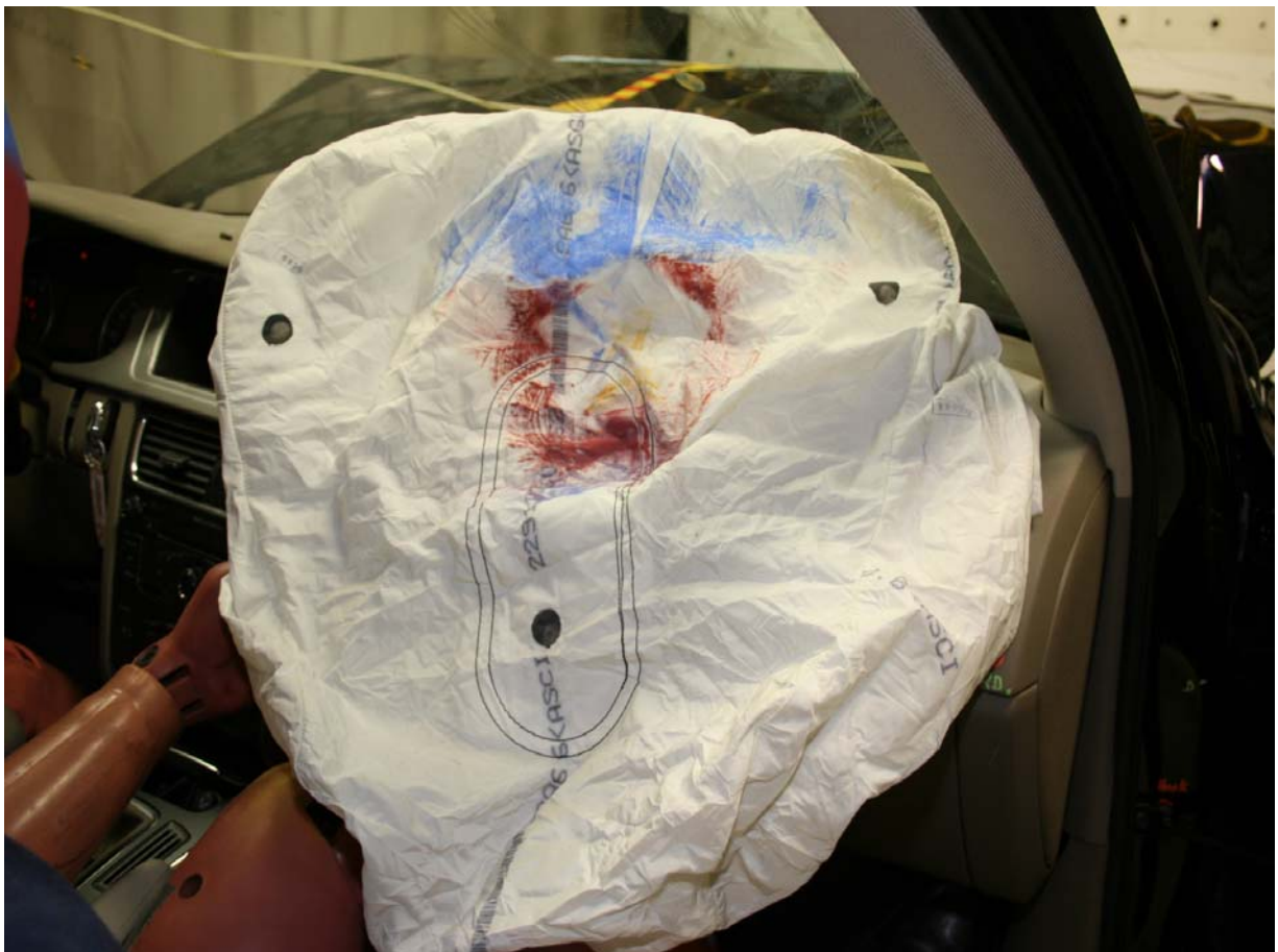
Post-Test Driver Dummy Airbag Contact
