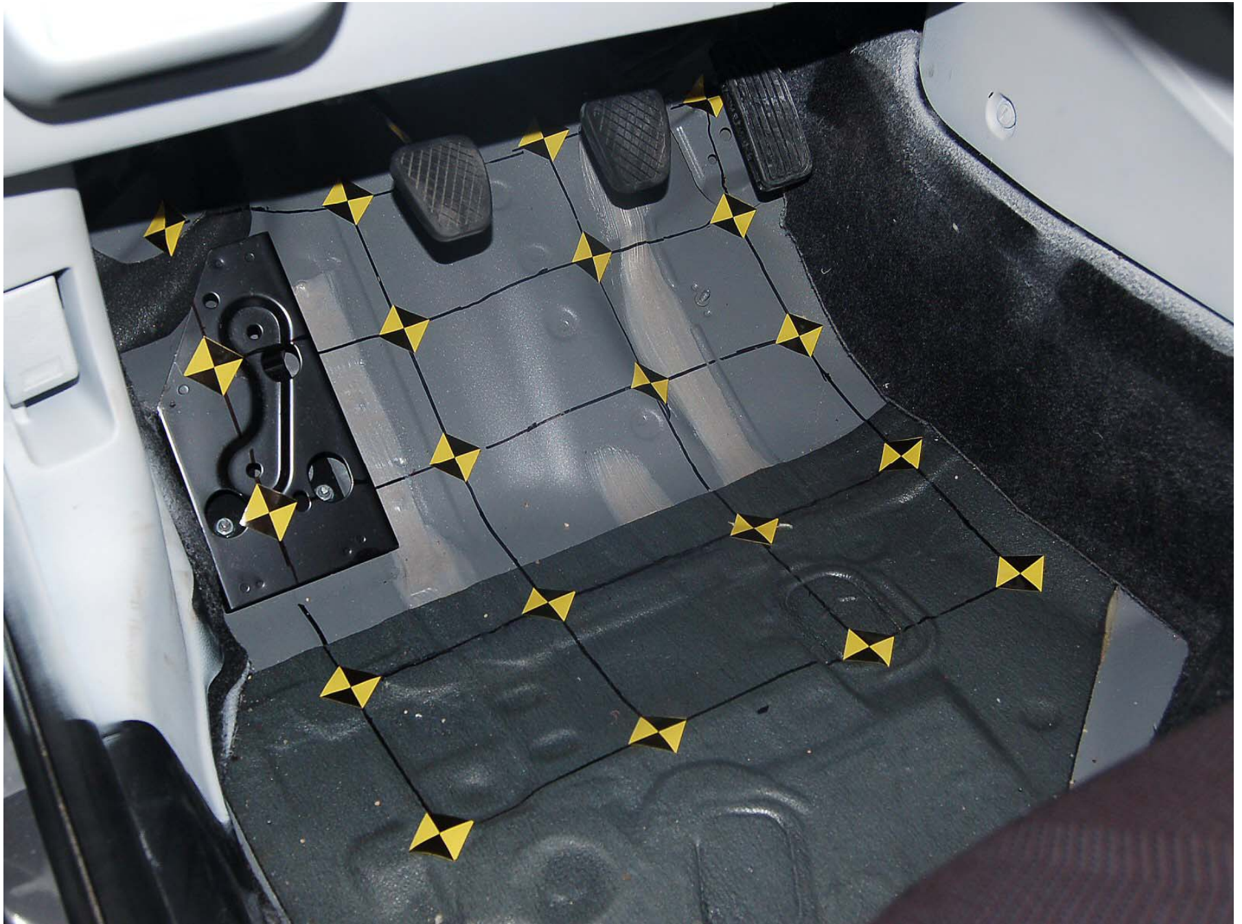
Figure A-40: Pre-Test Driver Side Floor Pan
