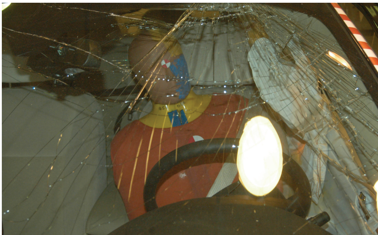
Figure A-38: Post test driver shoulder clearance
