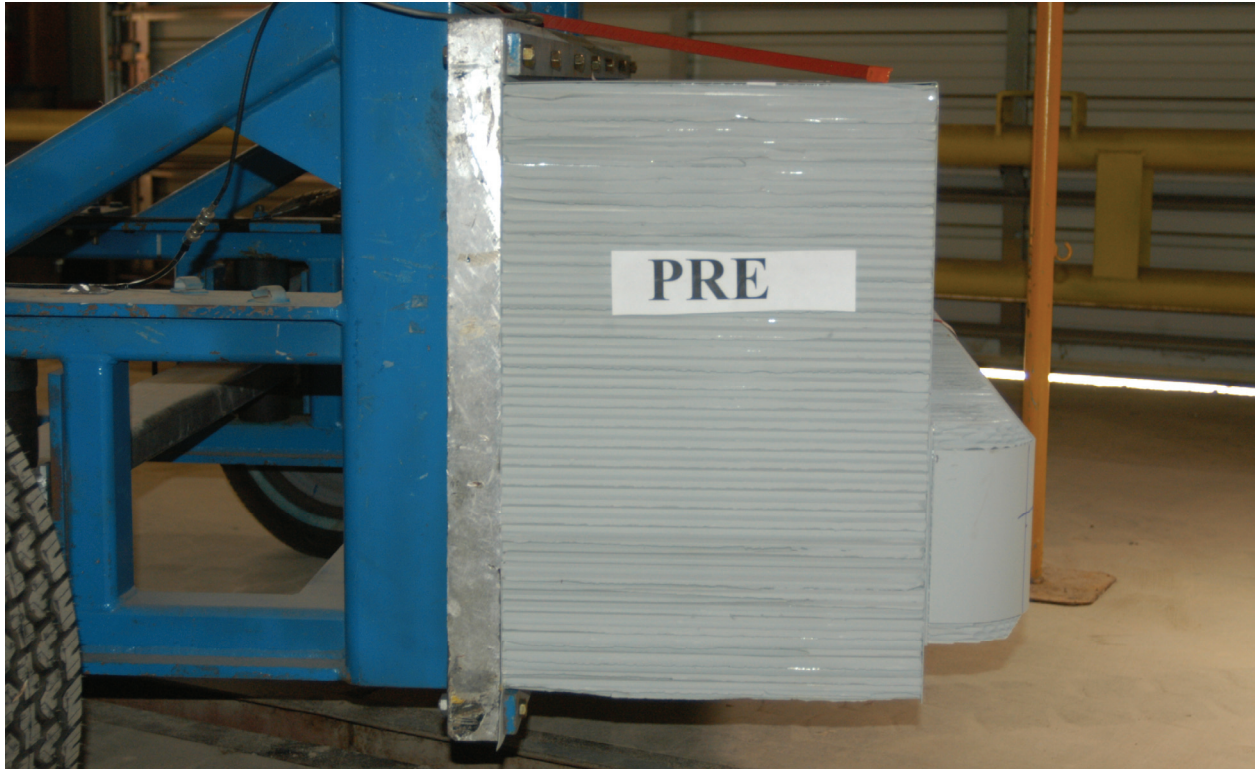
Figure A-55: Pre test right side view of MDB barrier face
