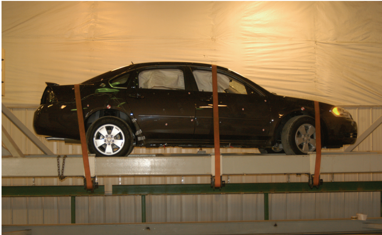
Figure A-63: FMVSS 301 360 degrees
