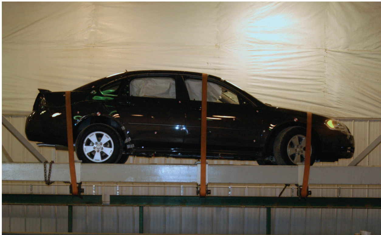
Figure A-59: FMVSS 301 0 degrees
