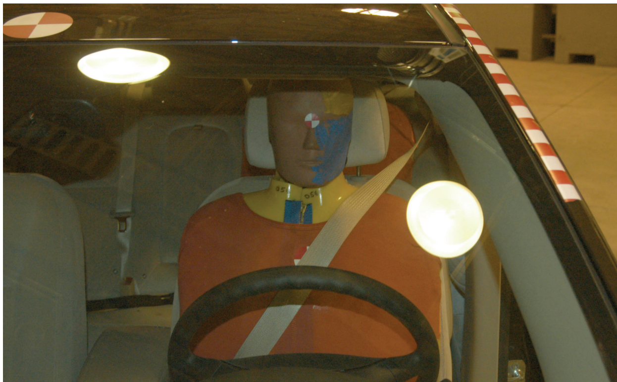
Figure A-37: Pre test driver shoulder clearance
