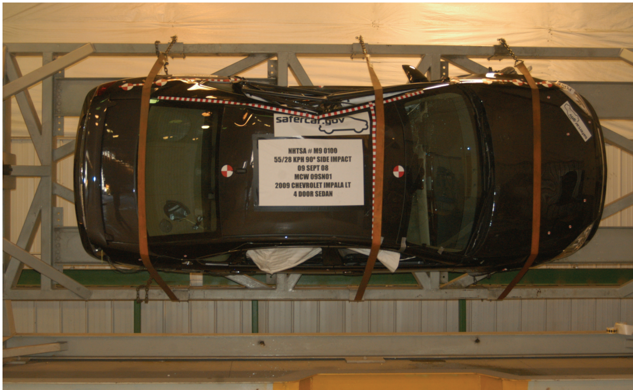
Figure A-62: FMVSS 301 270 degrees
