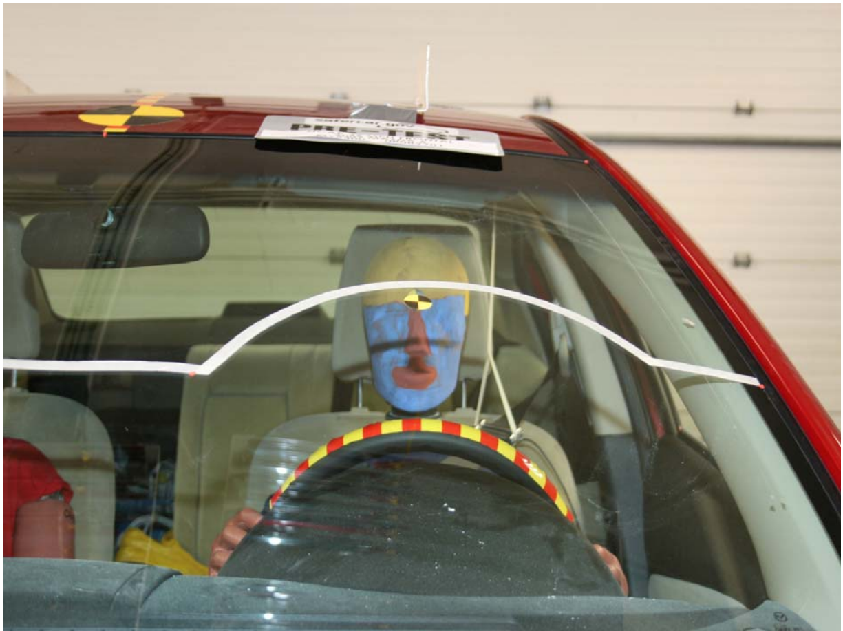
Pre-Test Driver Dummy Front View (Head Position)
