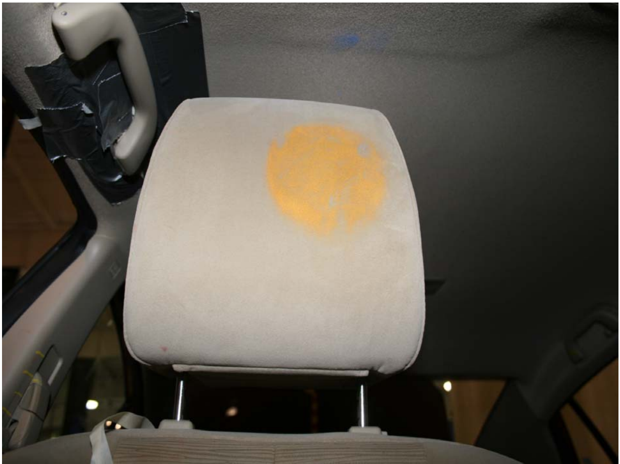
Post-Test Passenger Dummy Head Contact
