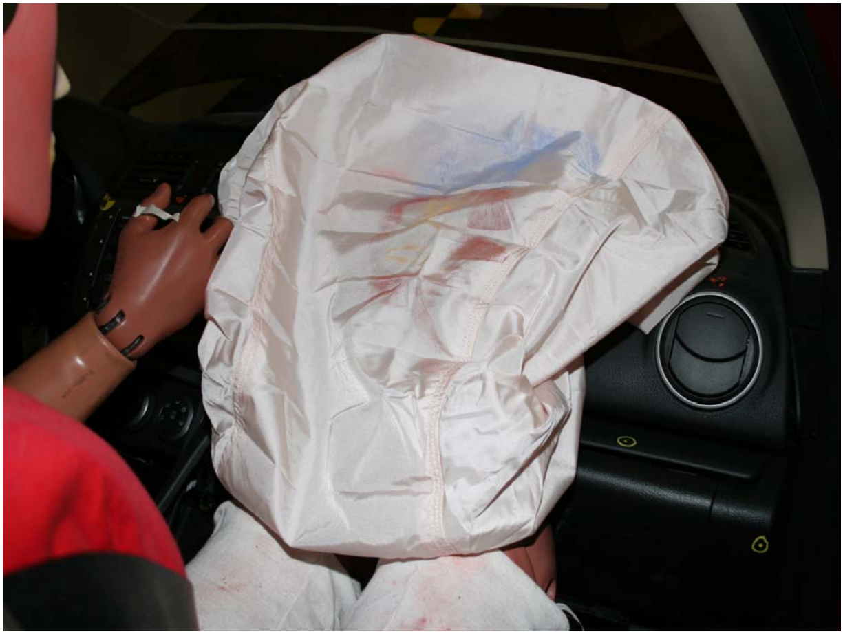
Post-Test Passenger Dummy Airbag Contact
