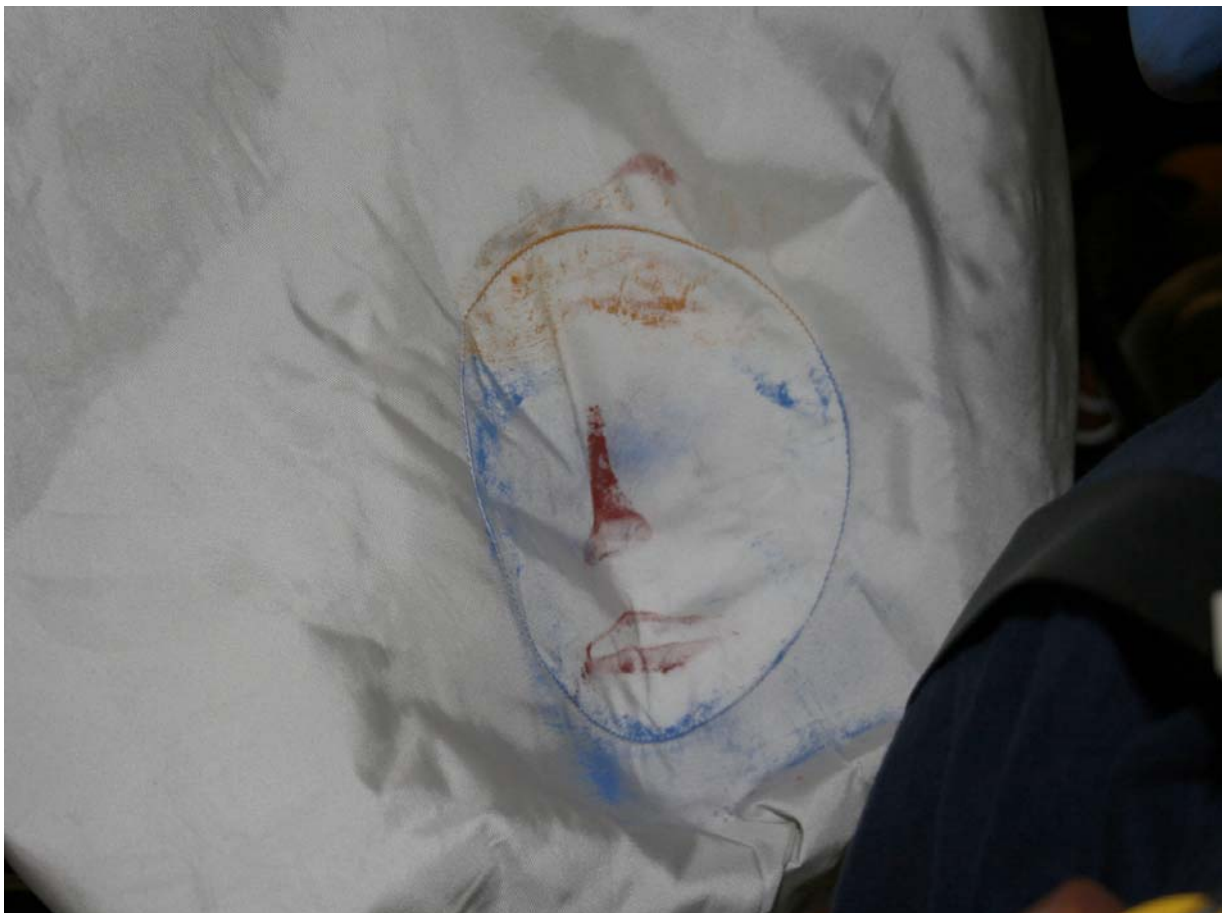
Post-Test Driver Dummy Airbag Contact
