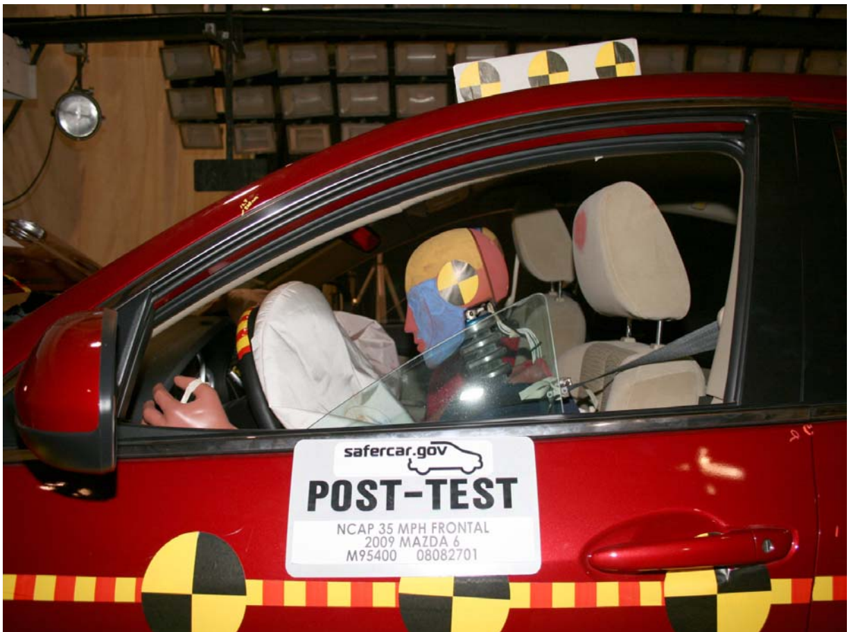
Post-Test Driver Dummy (Through Window)
