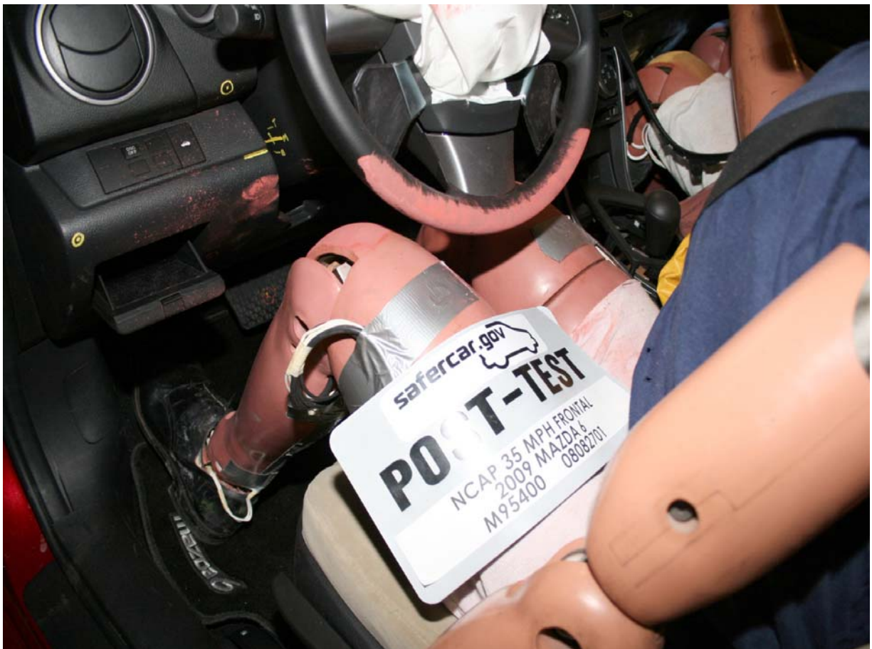
Post-Test Driver Dummy Left Knee Contact
