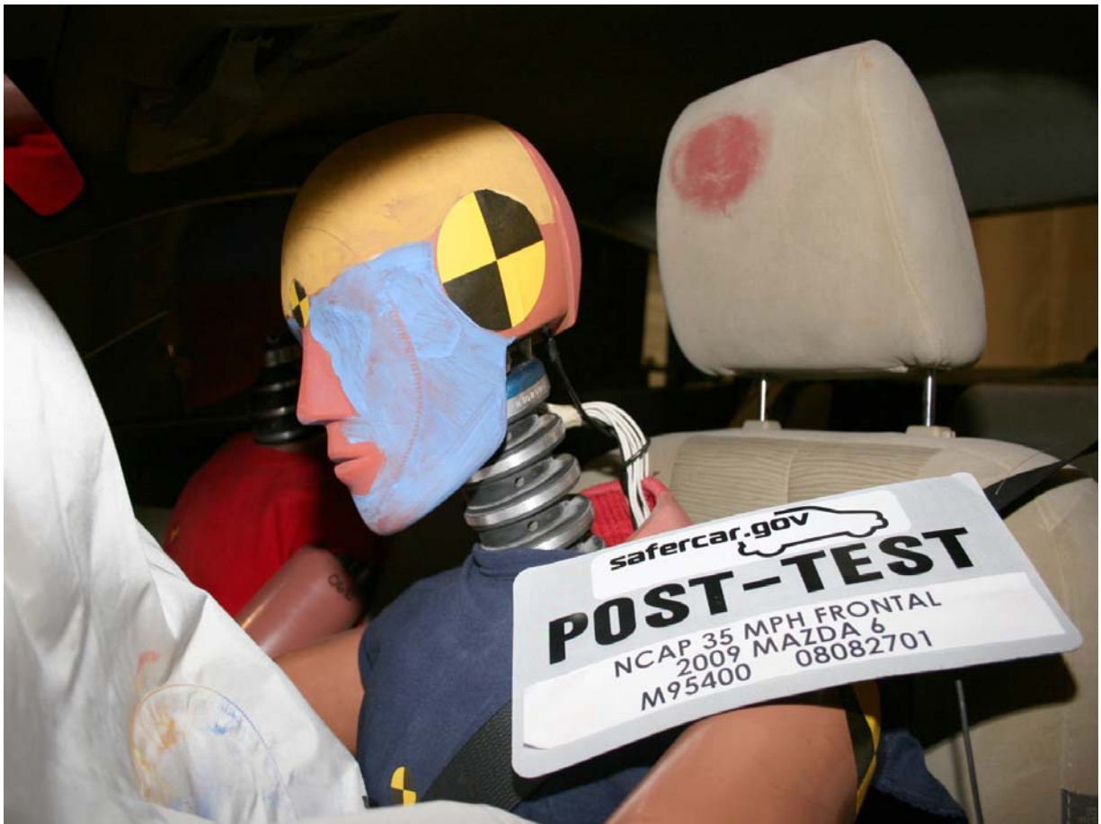
Post-Test Driver Dummy Head Contact
