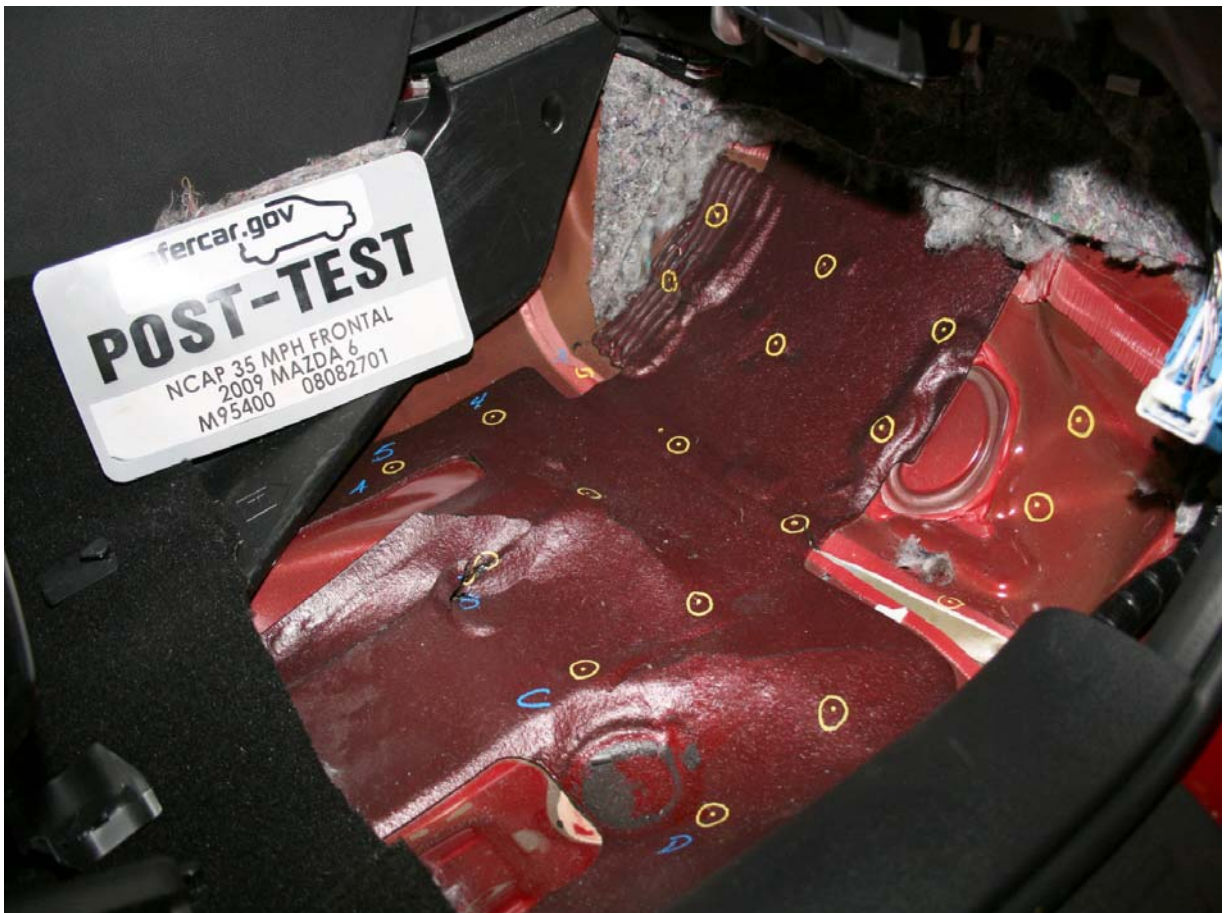
Post-Test Passenger Side Floor Pan
