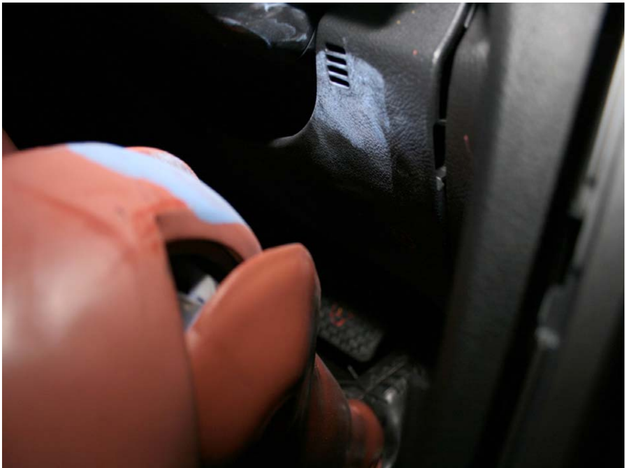
Post-Test Driver Dummy Right Knee Contact
