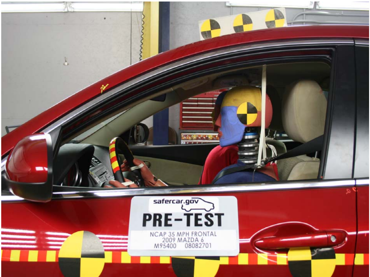
Pre-Test Driver Dummy (Through Window)
