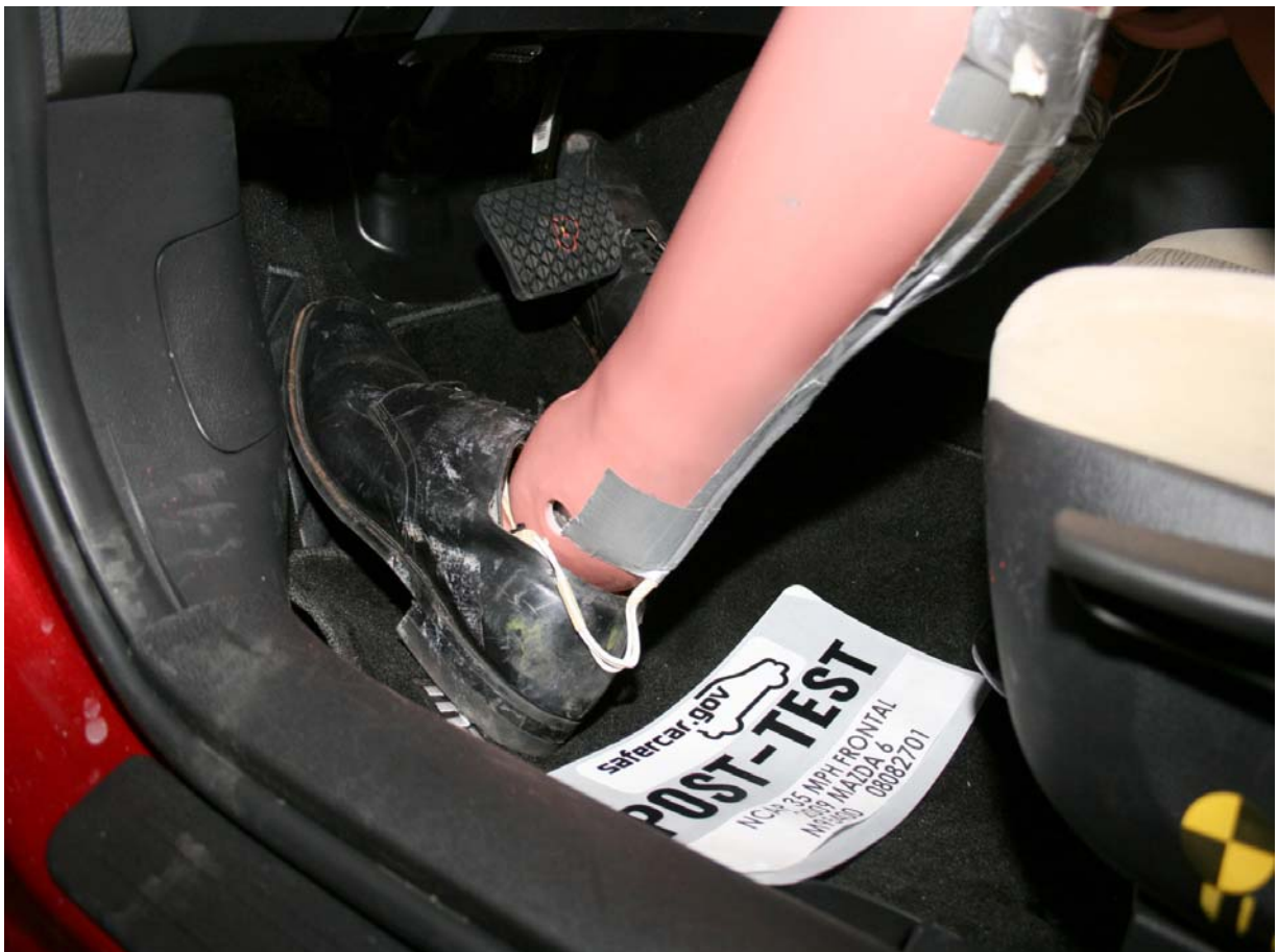
Post-Test Driver Dummy Feet
