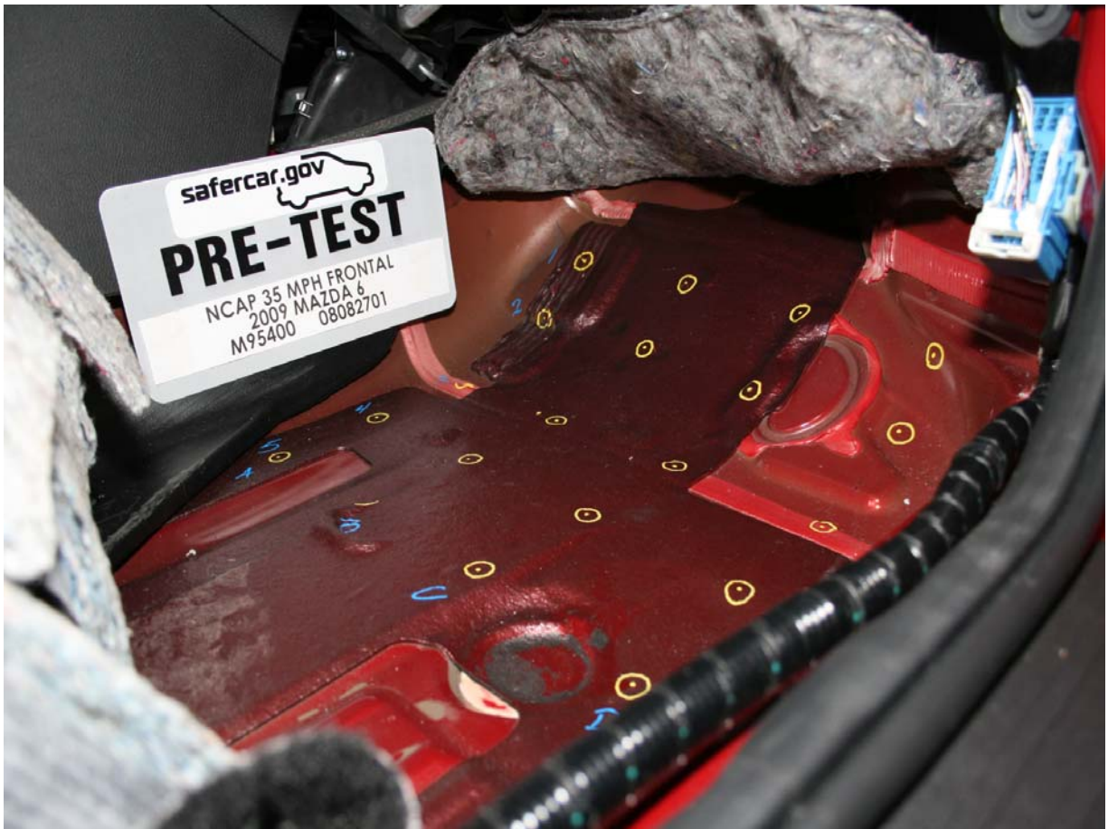
Pre-Test Passenger Side Floor Pan
