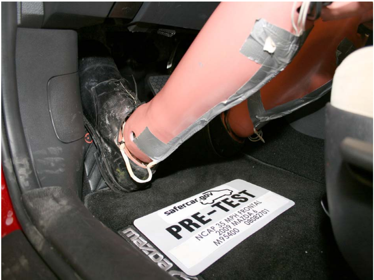
Pre-Test Driver Dummy Feet
