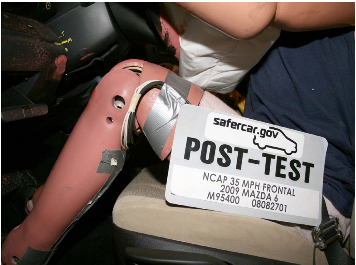
Post-Test Driver Side Knee Bolster
