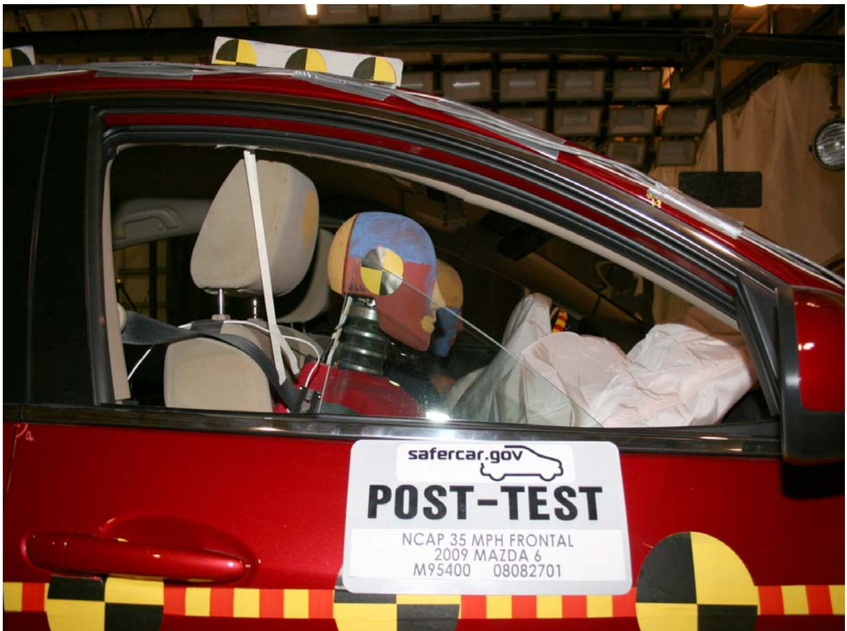
Post-Test Passenger Dummy (Through Window)
