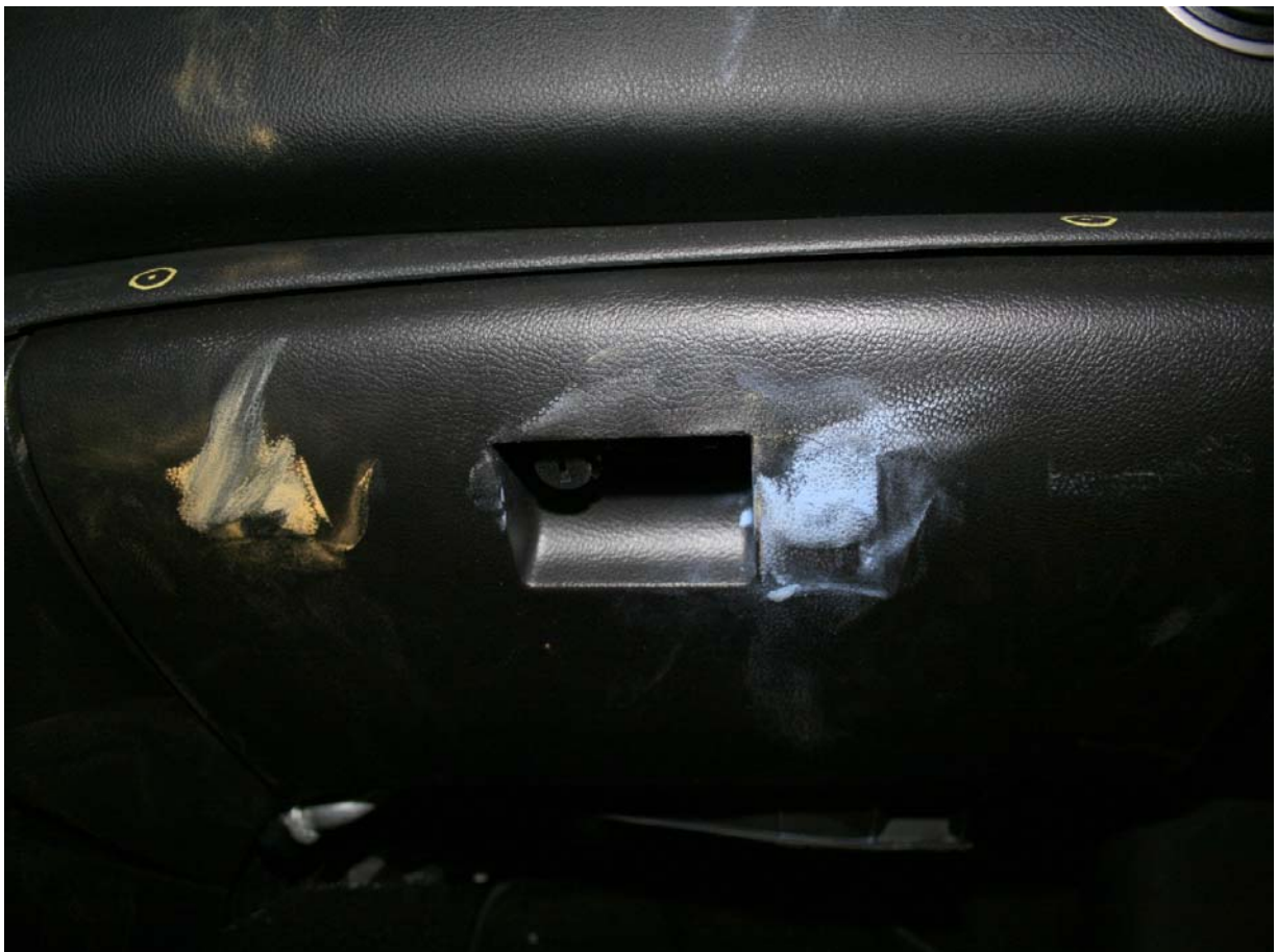
Post-Test Passenger Dummy Knee Contact
