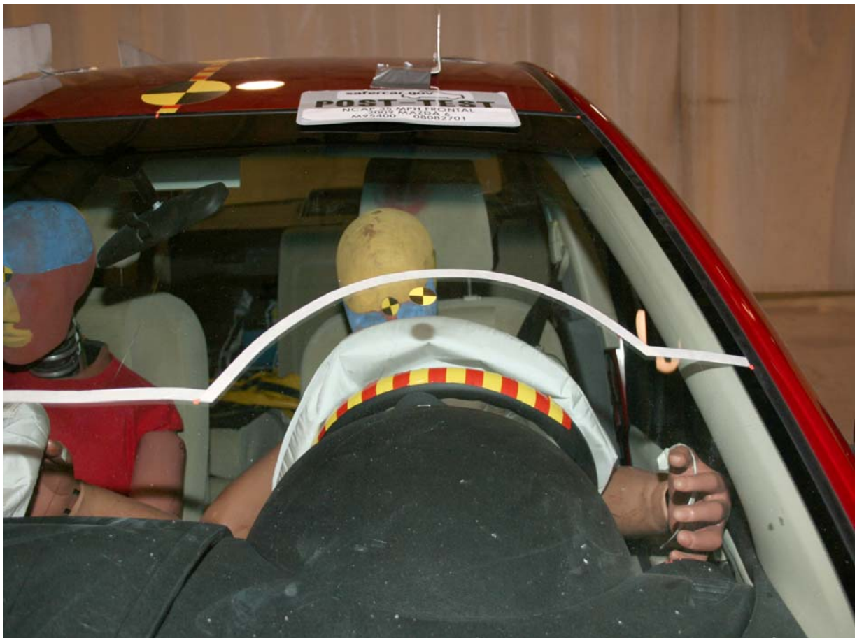
Post-Test Driver Dummy Front View (Head Position)
