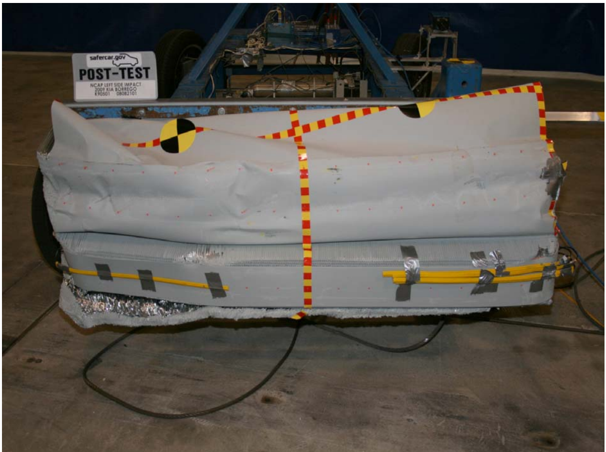
Post-Test Front View of Deformable Barrier
