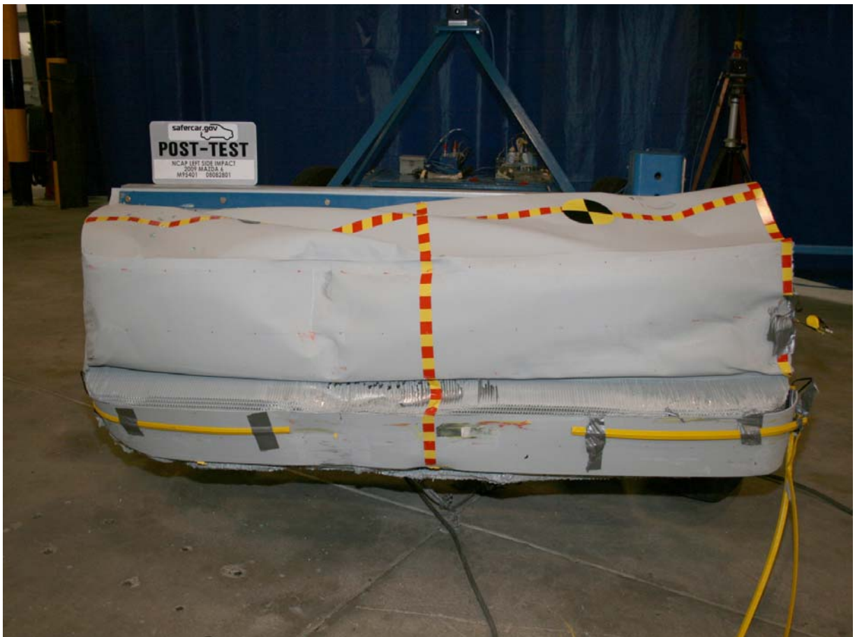
Post-Test Front View of Deformable Barrier
