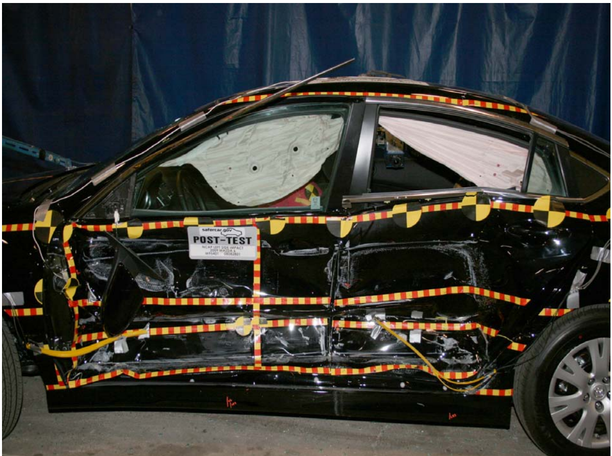
Post-Test Left Side Impact Close-up
