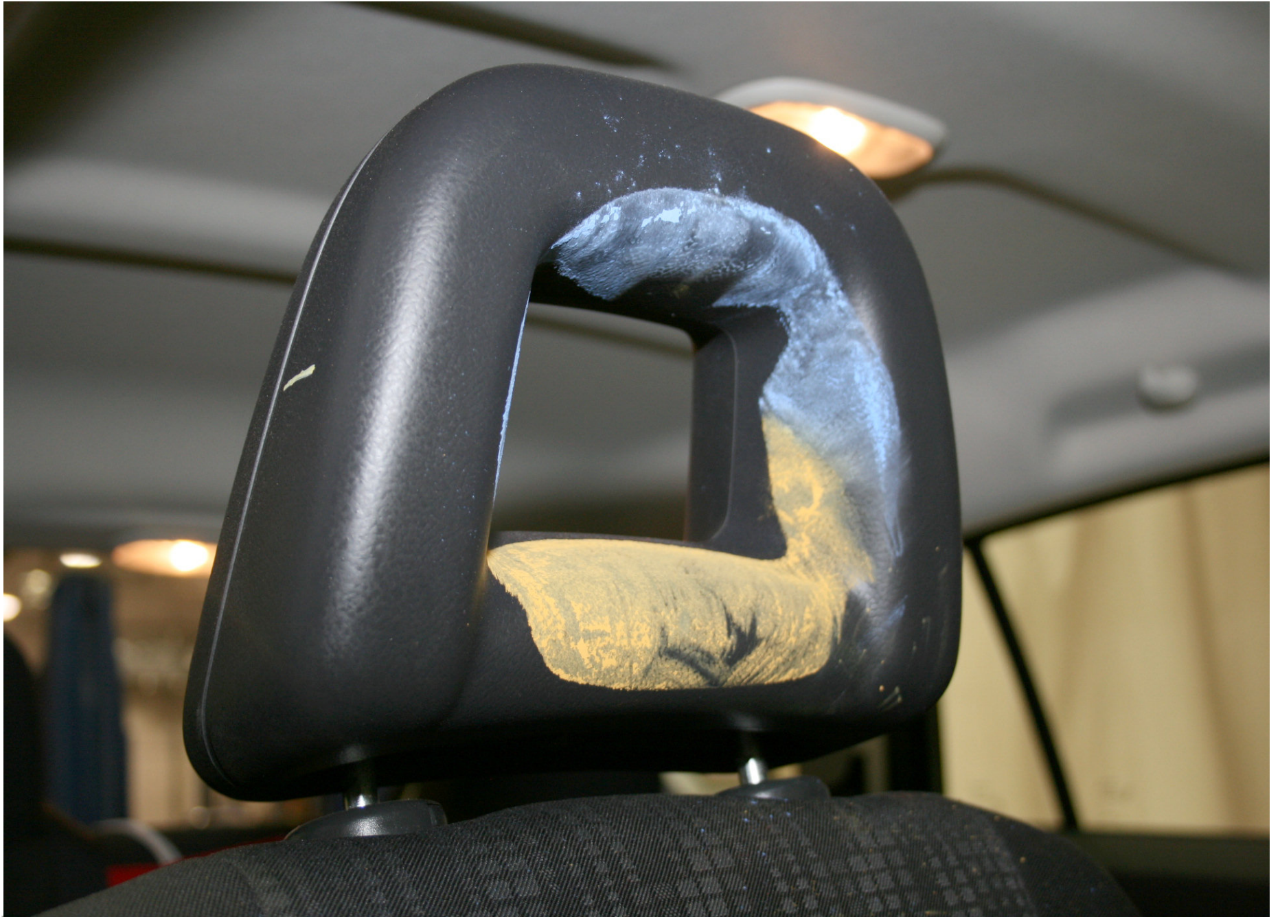
Post-Test Passenger Dummy Head Contact View (headrest)
