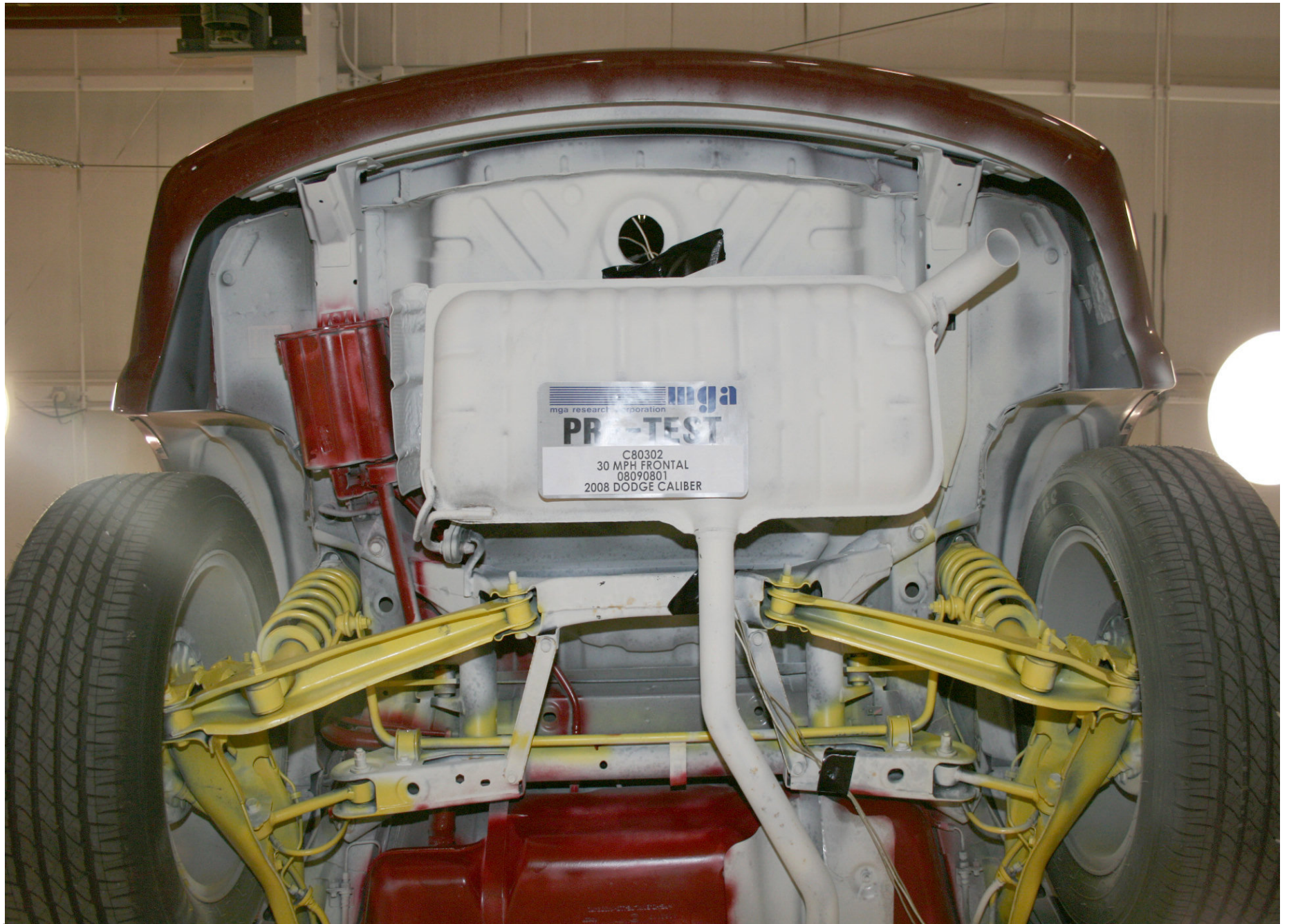
Pre-Test Rear Underbody View
