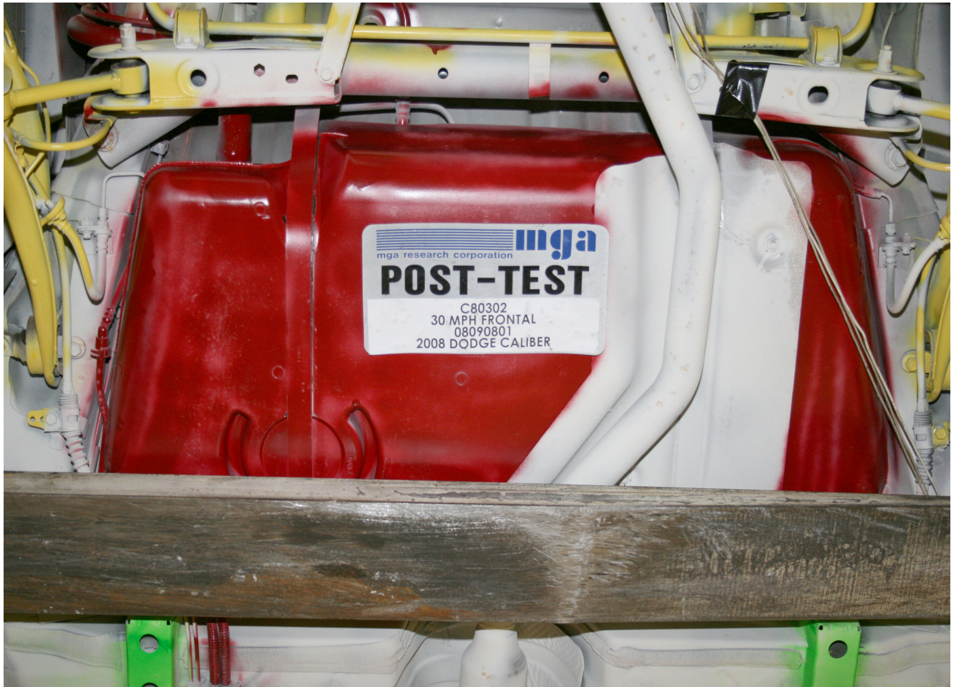
Post-Test Mid Rear Underbody View
