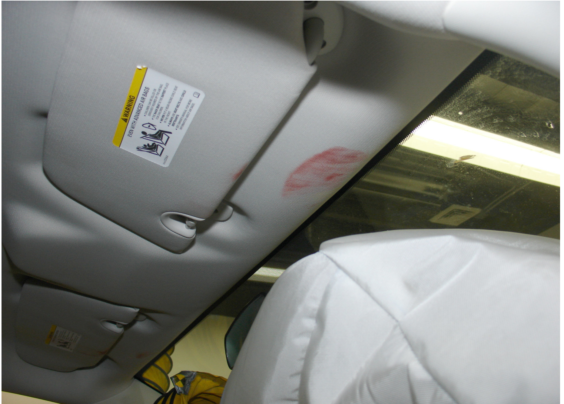
Post-Test 6YO P1 Passenger Dummy Head Contact (header) (Trial 2)
