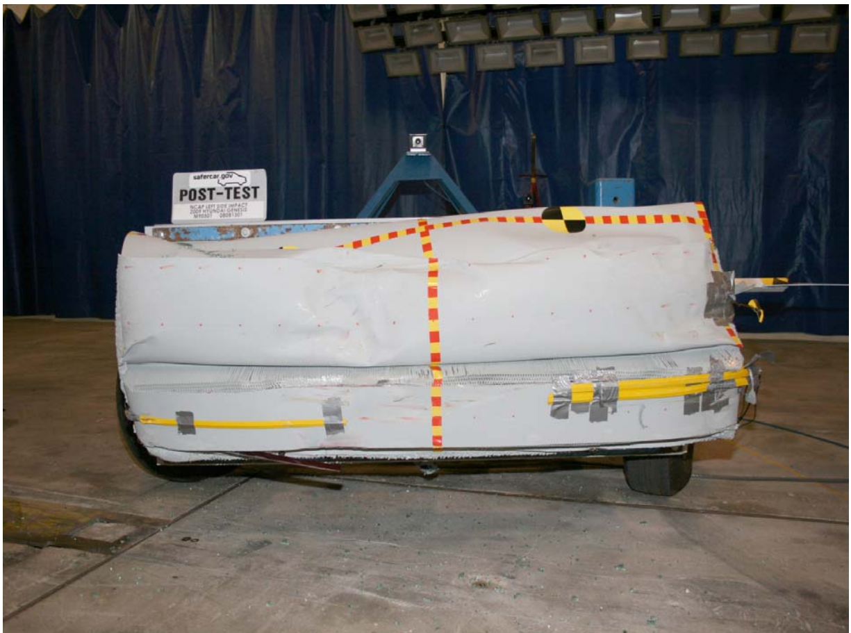
Post-Test Front View of Deformable Barrier
