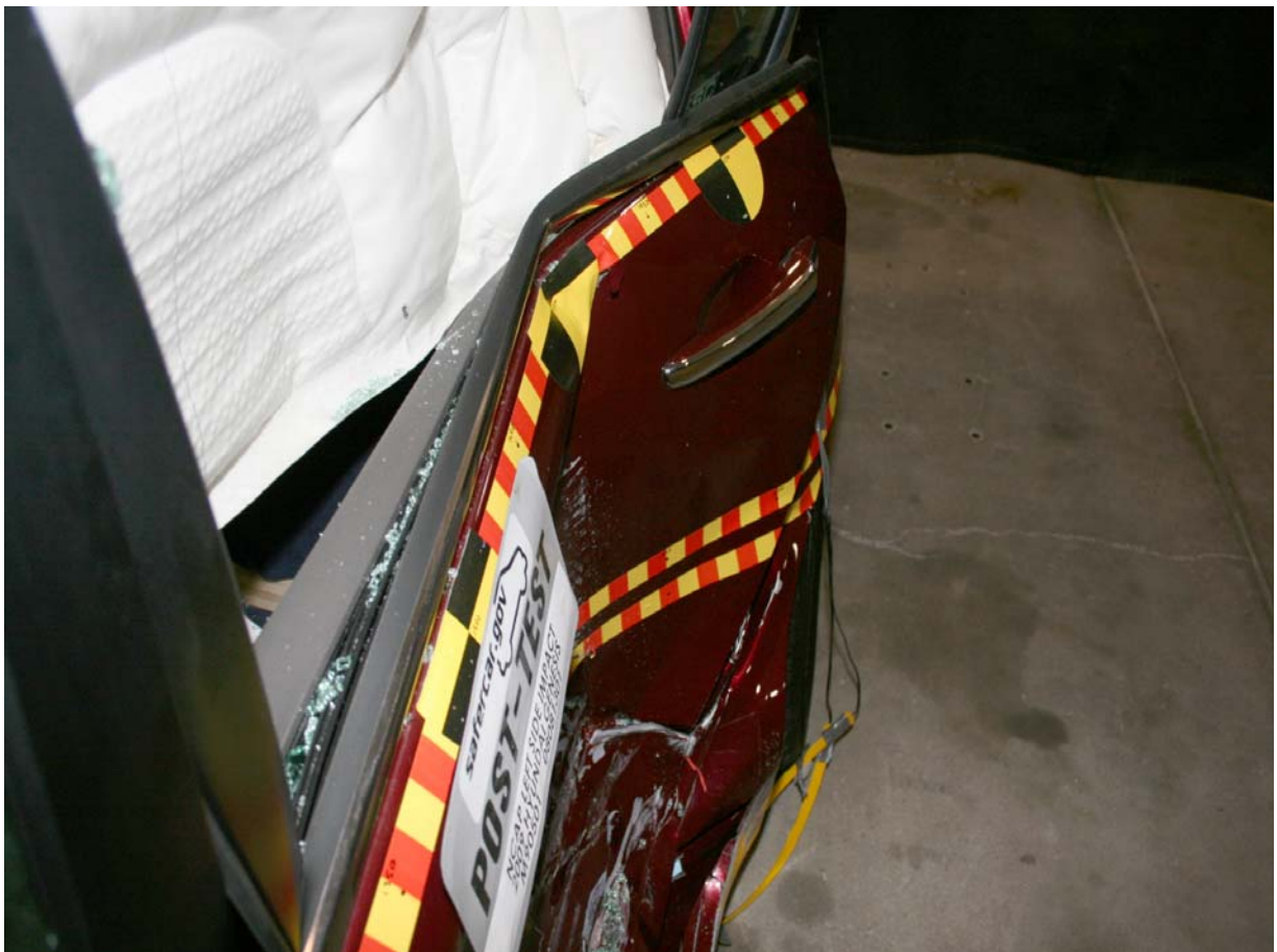
Post-Test Passenger Dummy Clearance From Door
