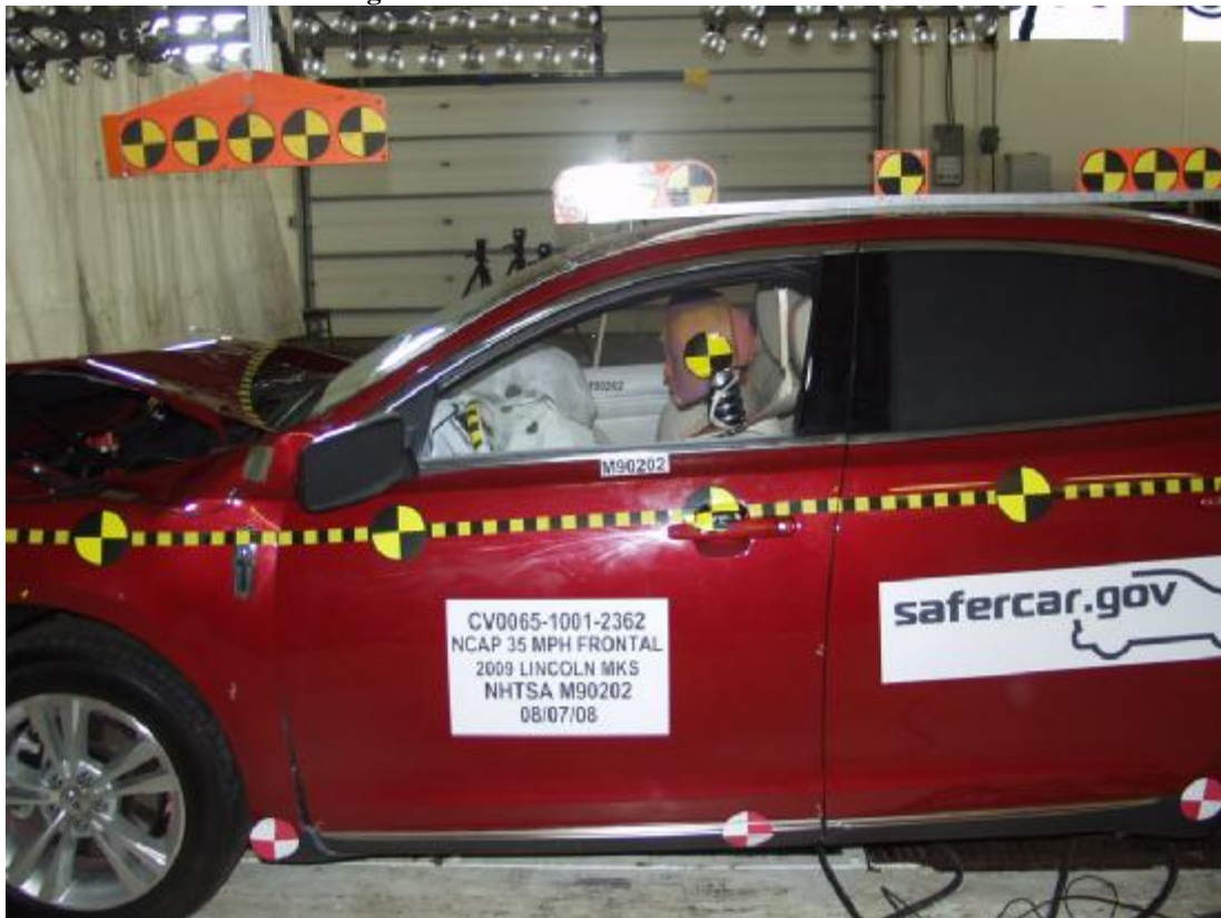
Figure A-33: Post-Test Driver Position View
