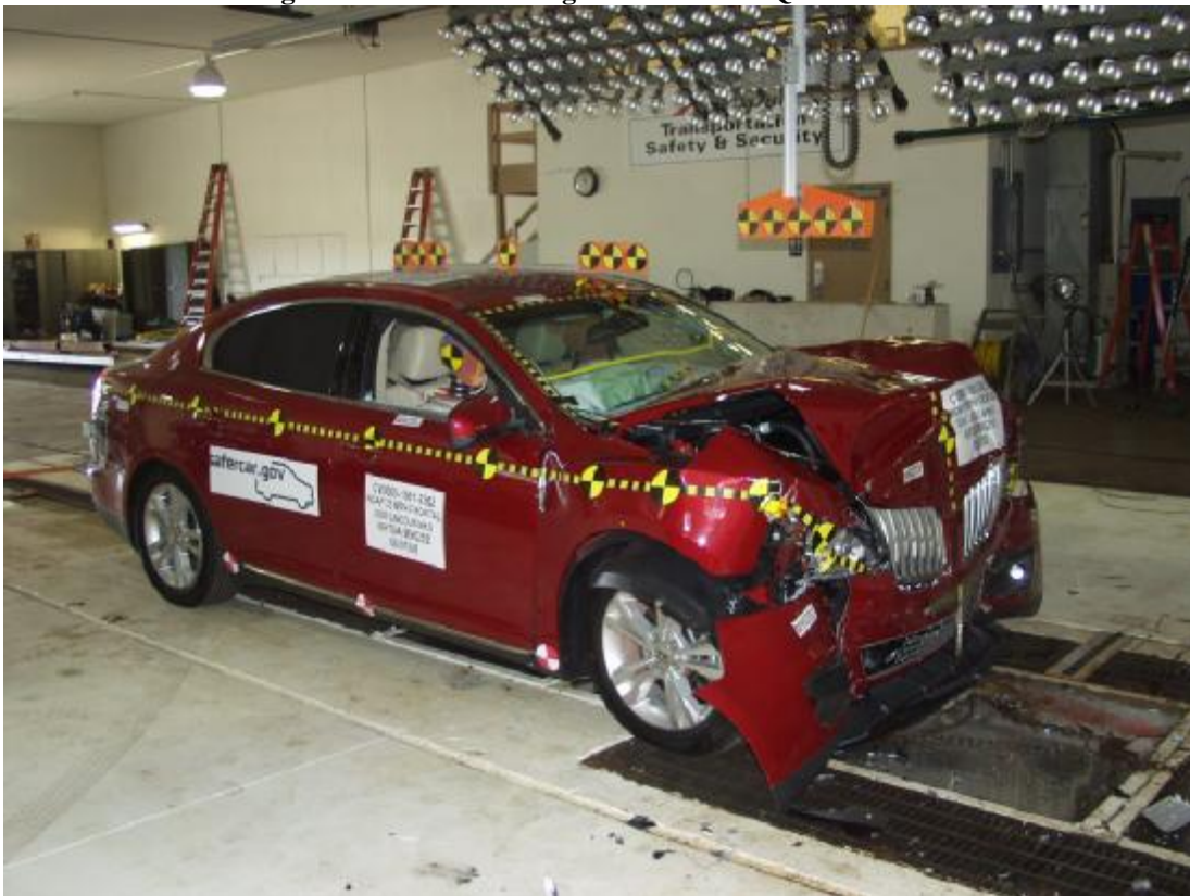
Figure A-13: Post-Test Right Front Three-Quarter View
