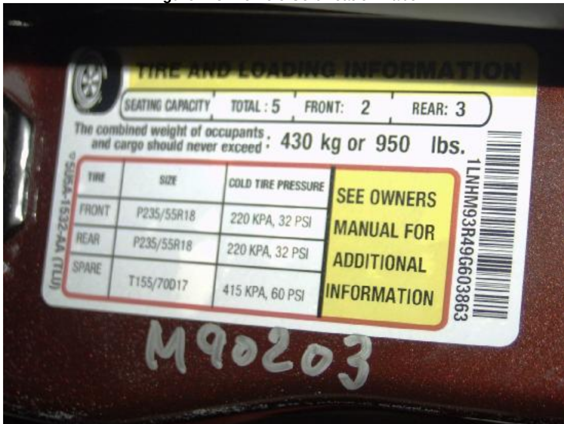
Figure A-4: Vehicle Tire Placard Label
