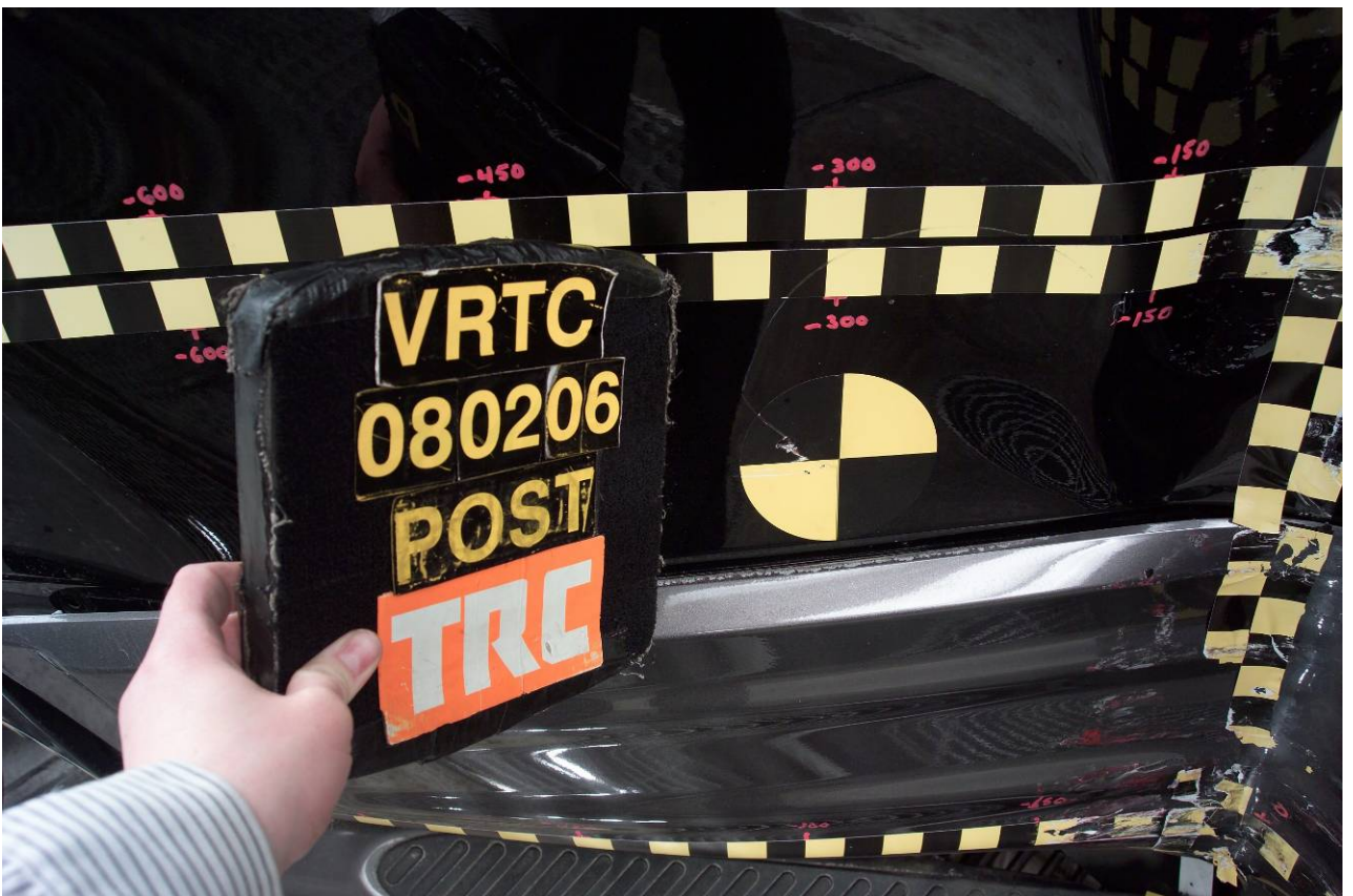
Figure A-22 Post-Test Primary Impact Point View
