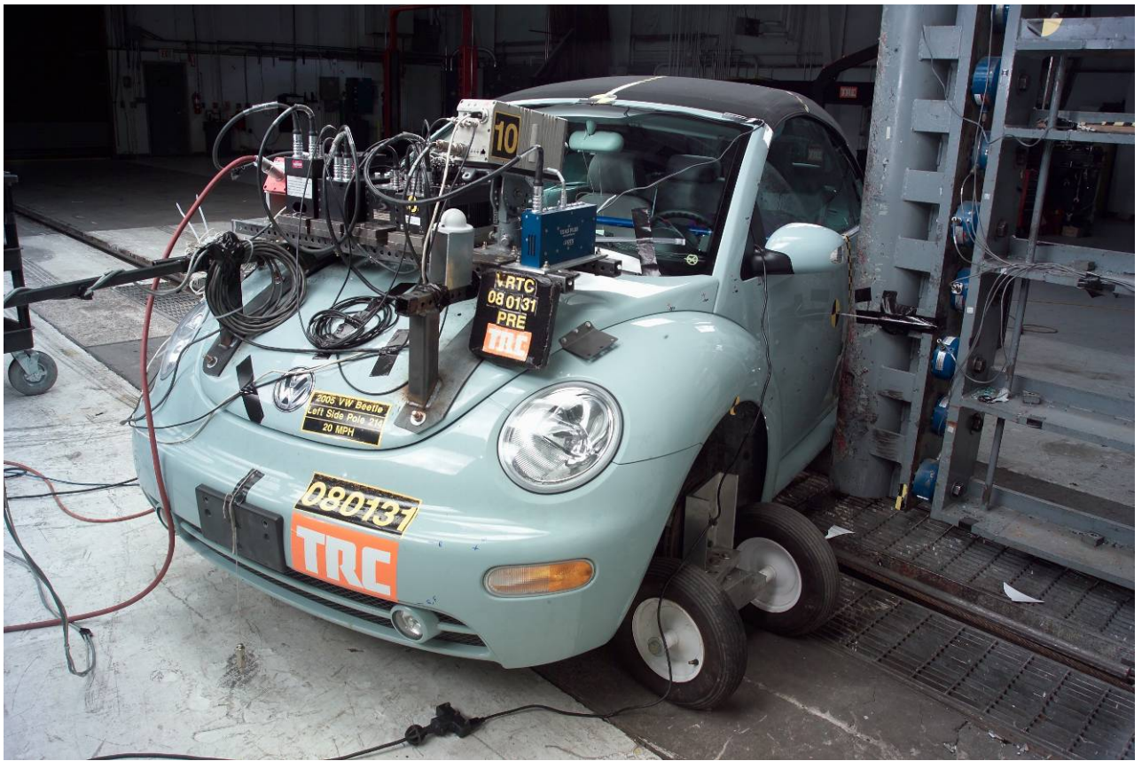
Figure A-19 Pre-Test Impact Alignment - View 1
