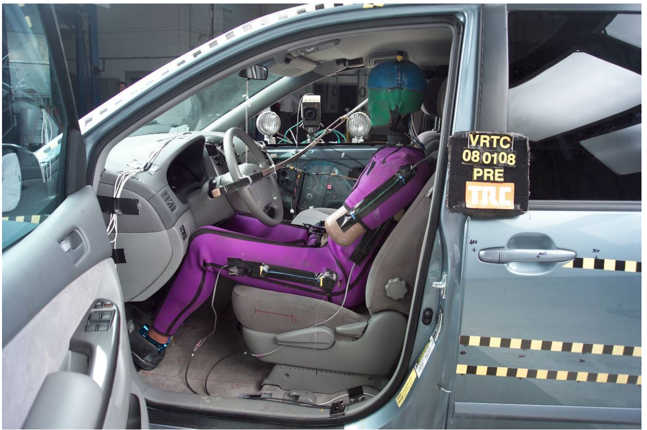
Figure A-22 Pre-Test Driver Dummy Showing Belts, Chalking, and Contact Switches
