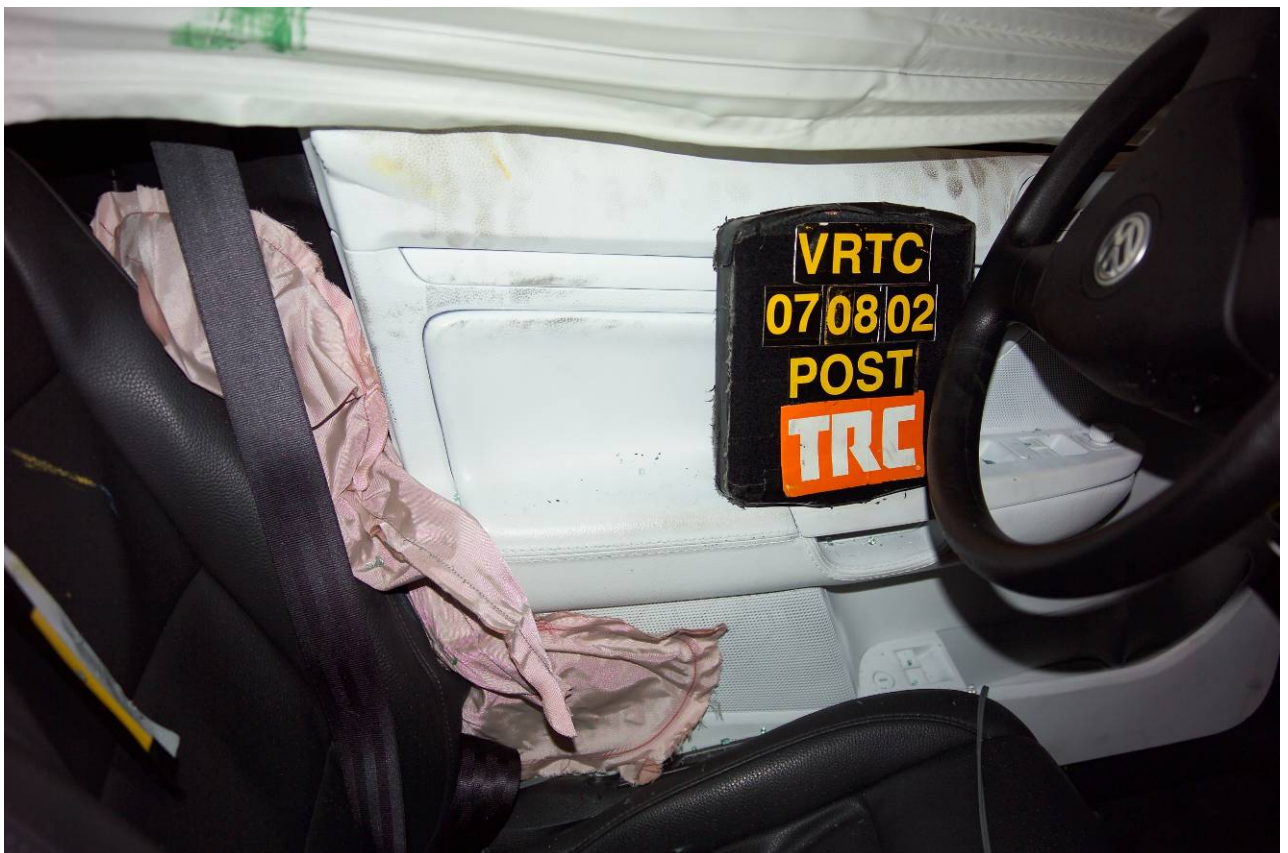
Figure A-34 Post-Test Driver Dummy Door Contact View
