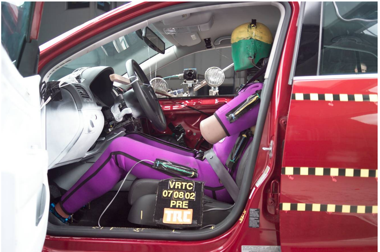
Figure A-30 Pre-Test Driver Dummy Showing Belts, Chalking, and Contact Switches
